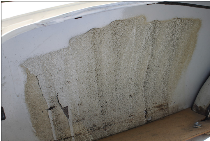
Typical sound deadener application onto the inner surface of the quarter panels.
