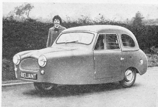
TWO NEW MINIATURES: On the left is the 1957 Bond Minicar, which will be in production next spring. Mechanically the car is as last year, main improvements being made in body styling. On the right is the Reliant Regal, in Grand Touring style with a hardtop. This car is powered by a four-cylinder side-valve engine, and has a four-speed synchromesh gearbox.
