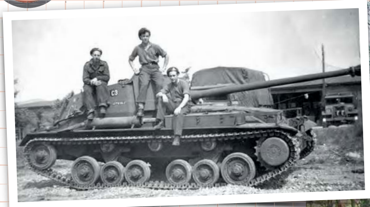
ABOVE The Archer self-propelled anti-tank gun – with rear-facing 17-pounder gun – was optimised for ambush tactics. A Bren gun was stowed on board for close defence.
