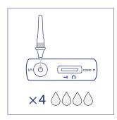
Add 4 drops of test sample into the test device sample window (S) by squeezing the sample extraction tube.
