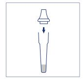
Insert the nozzle on to the sample extraction tube.
