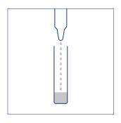
Add 0.3 ml (10 drops) of the sample extraction buffer into the extraction tube.
