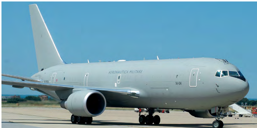
Above: The strategic transport and tanker missions are assigned to four KC-767As operated by 14° Stormo at Pratica di Mare. This type is able to refuel with both of the available systems: probe-and-drogue as well as the boom.
