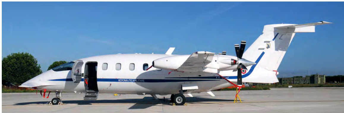
Above: A P.180RM from 14° Stormo on the ramp at Pratica di Mare. Four P-180s have been modified to this standard since 2011 and undertake navigation-aid calibration duties.
