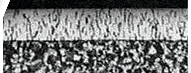
Traditional Single-Layer Chrome Plating Technology
