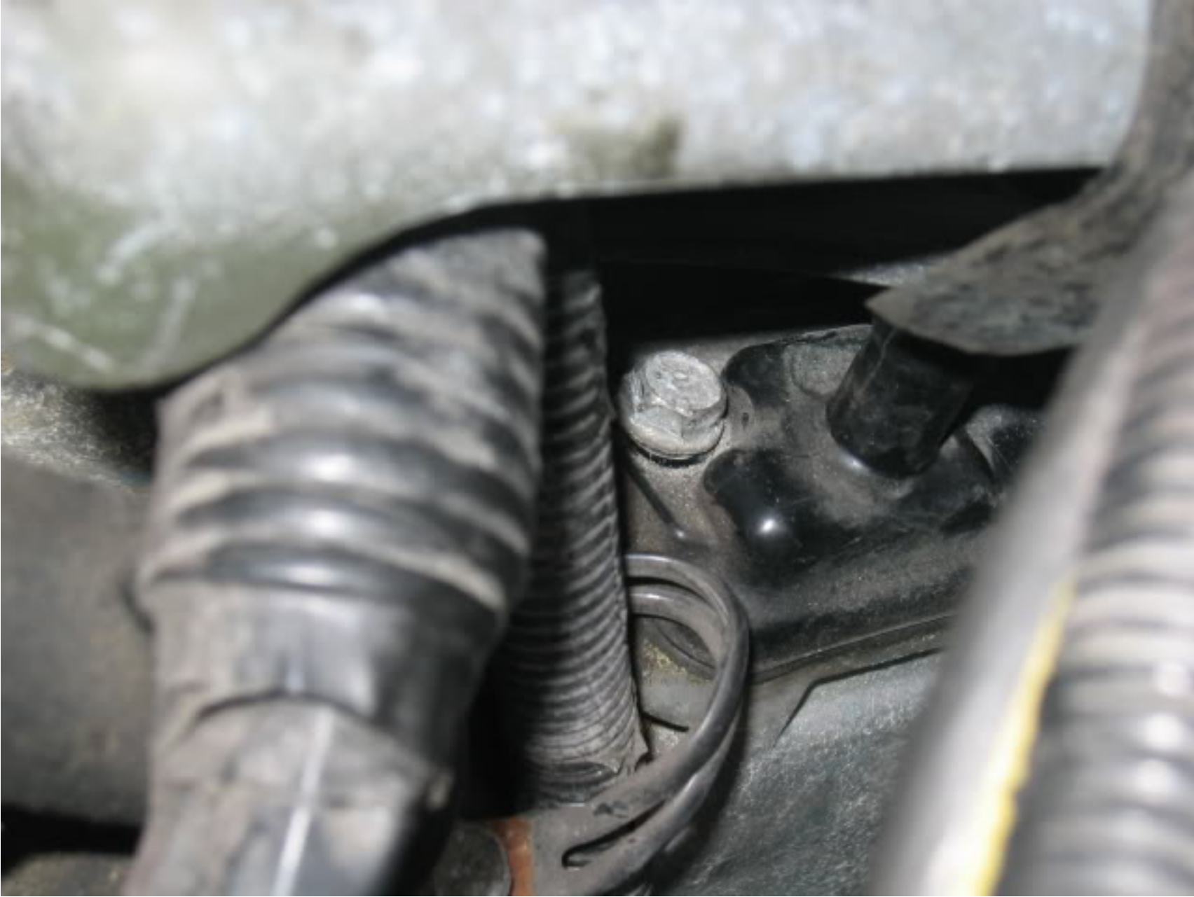
Picture of driver's side GBOD! Took me about 30 min to remove IC and GBOD. You will have to bend a AC line slightly to create enough room to wriggle out the bracket.
