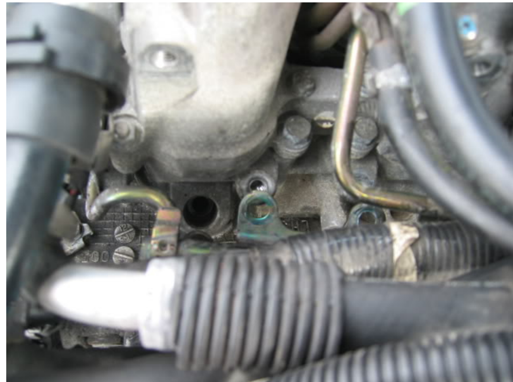
Picture of Pink injectors with o-rings correctly installed:
