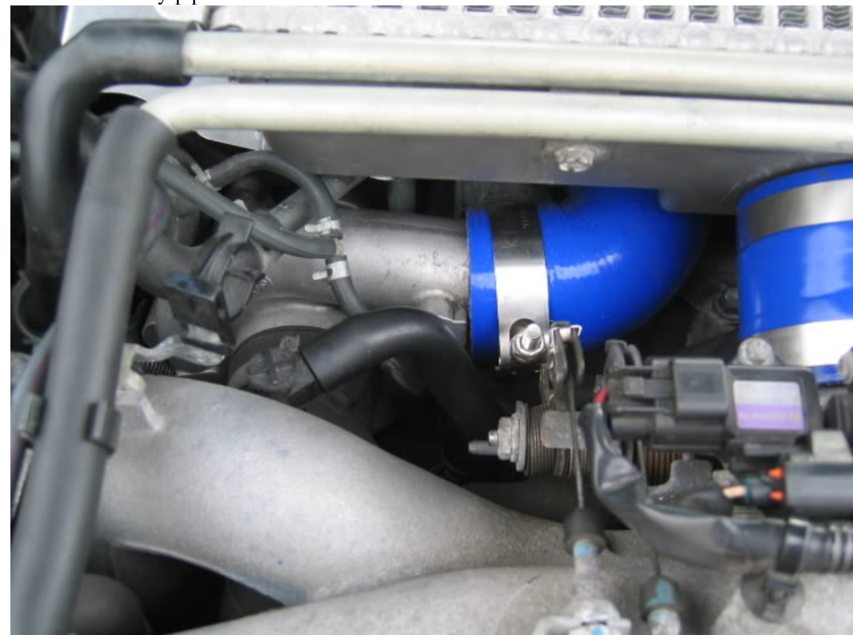
Remove two hoses (driver's side has one hose)
