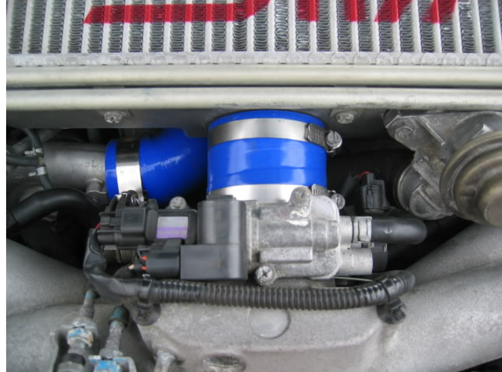
Remove turbo to y-pipe hose
