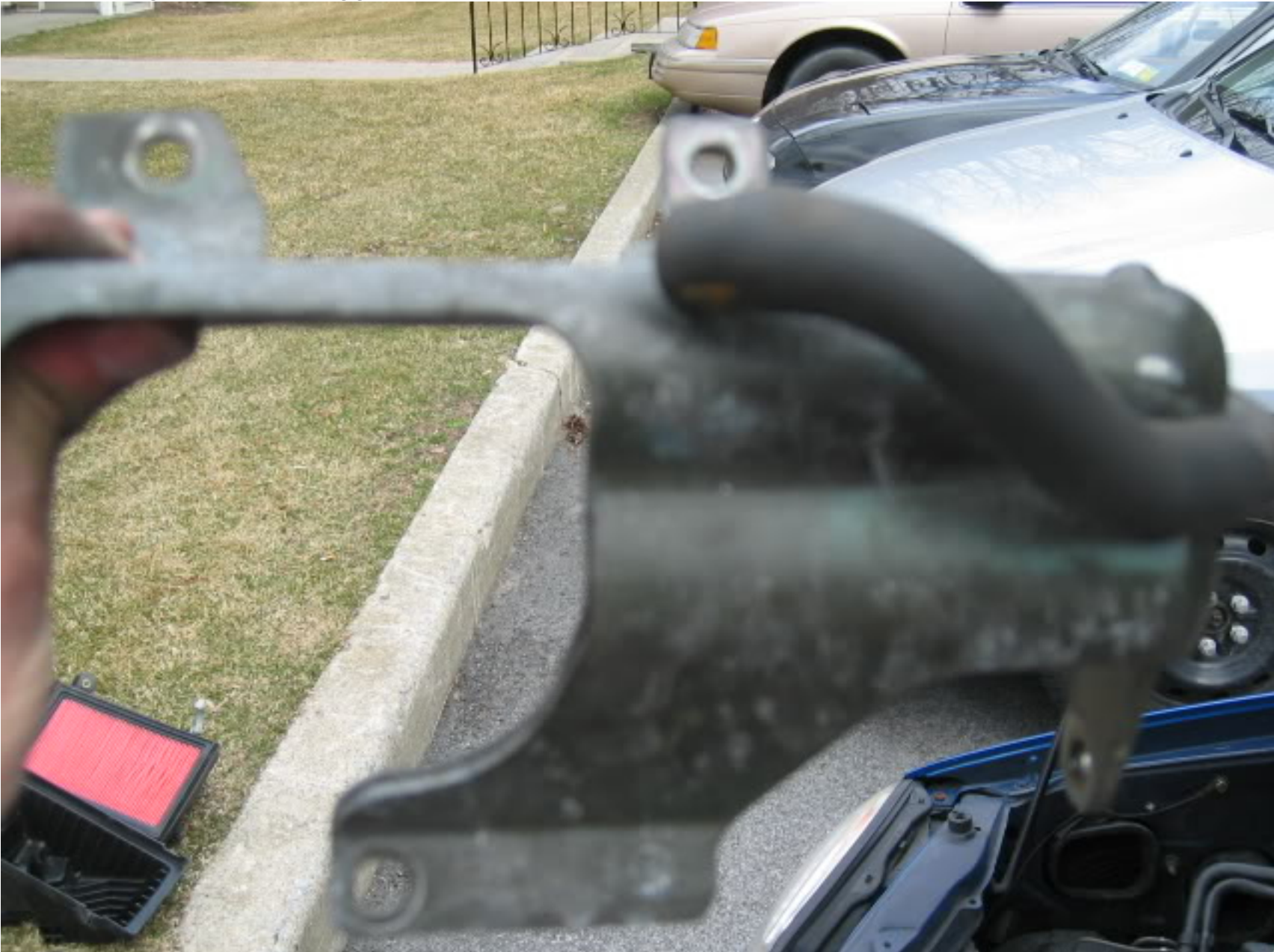
You will have to put this piece back on as hose off of breather cover is connected to a hose on GBOD. You have an option to cut this section off of GBOD and install it back on. I decided to put the bracket back on. :) You will have to bend a fuel line slightly in order to remove stock injectors. Be sure to use a gas to lubricate o-rings before
