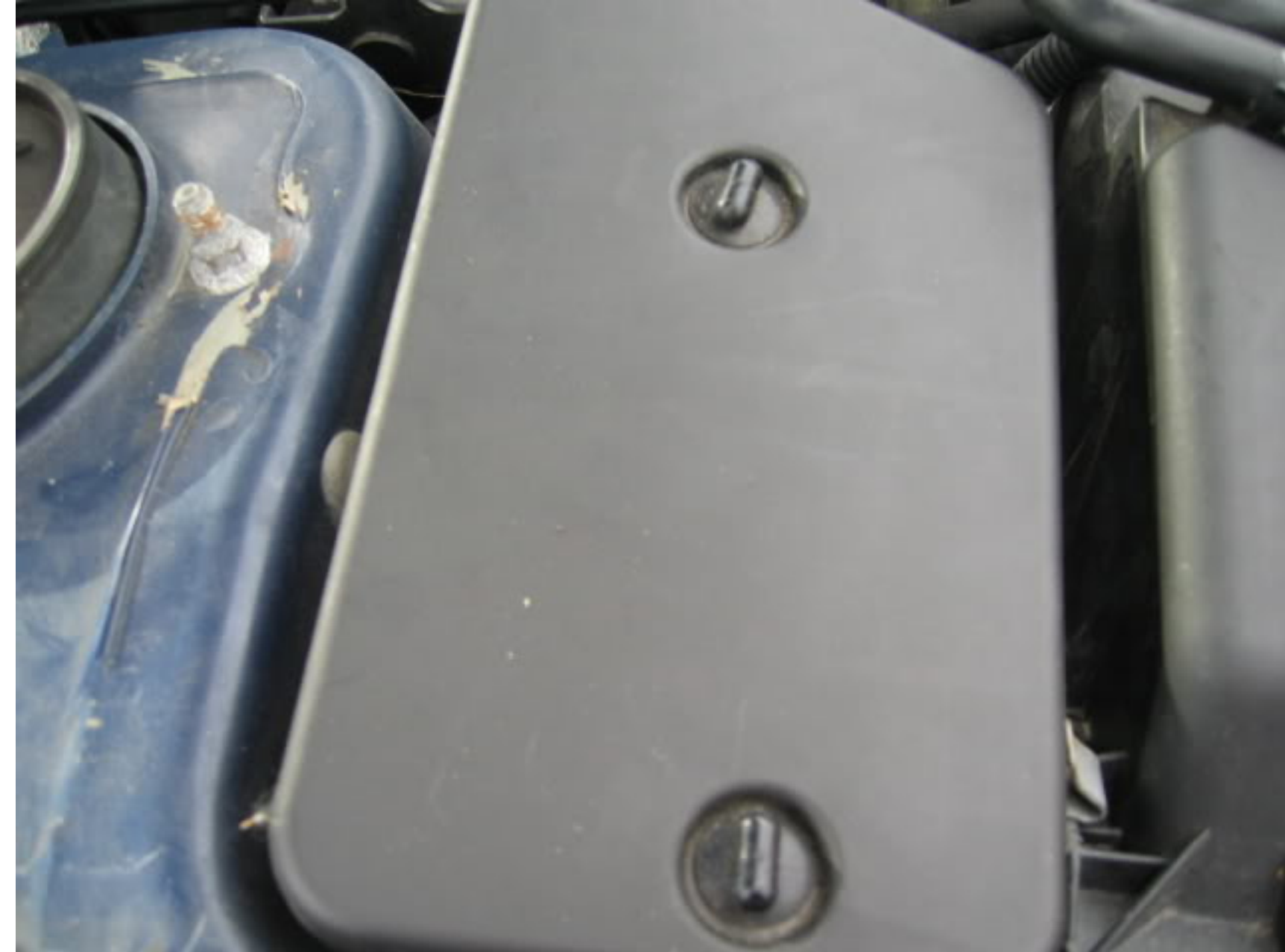
Remove the intake box (there are two bolts - you need a long extension to reach there)
