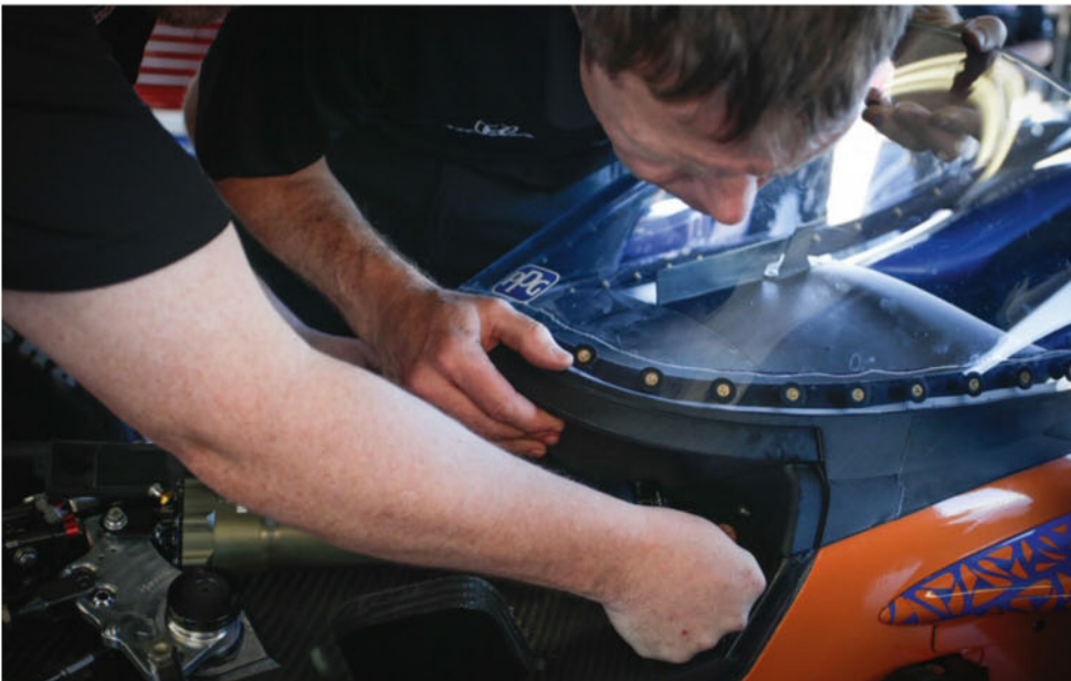
It will be retrofitted to the current chassis, as it was at the test, with a fitting flange incorporated into the Dallara monocoque
