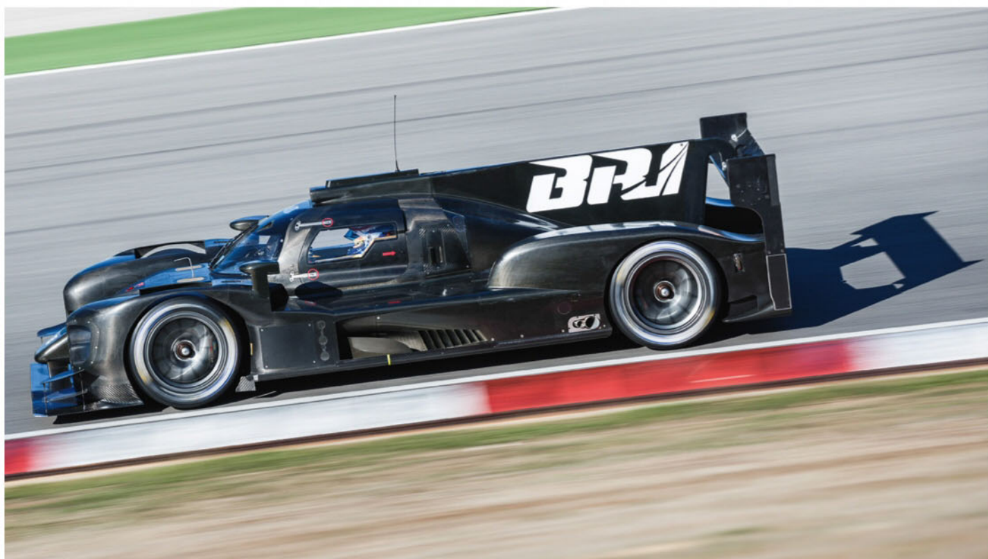
Three BR1s have been taken by SMP Racing while one has gone to Dragonspeed. It's been designed to take AER or Mecachrome turbo engines, or Gibson normally-aspirated units
