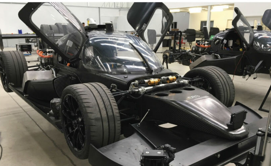
Roborace has used Devbots to prove and develop the AI hardware and software before integrating it into the Robocar. Based on an LMP chassis the cars have no bodywork so engineers can quickly and easily access all the systems during the testing
