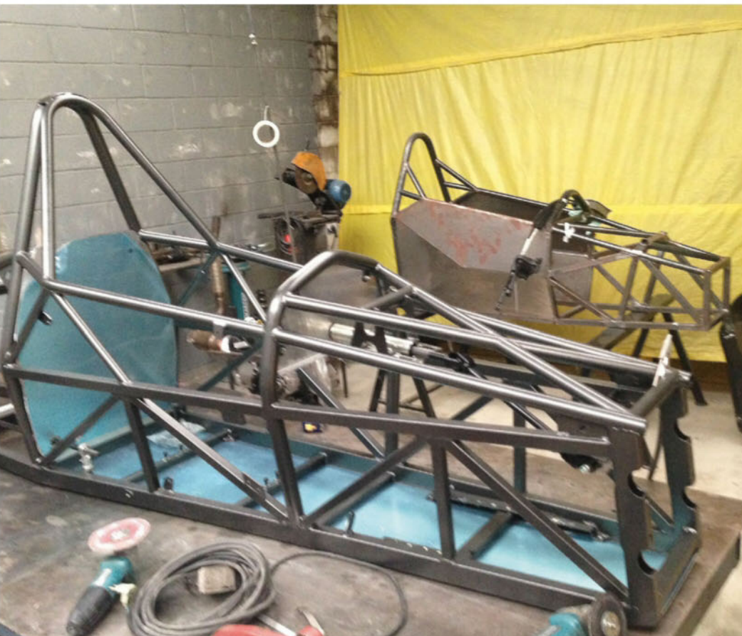
Left: Loom from the VW Up. It is a full throttle by wire, turbo control and double lambda ECU system. The immobiliser proved a headache for the team Above: A MacPherson strut from a VW Golf was inverted and machined to make an upright for the new racecar – an inspired and low cost solution Below: The current spaceframe design (in the foreground) with x-bracing, and original (behind) which will need the chassis tubes around the main hoop to be repositioned for strength. Note the rust!
