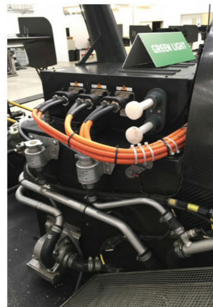
Batteries and inverter unit on the Devbot. On the Robocar the 540kW batteries will be mounted underneath, through the hollow base of the car
