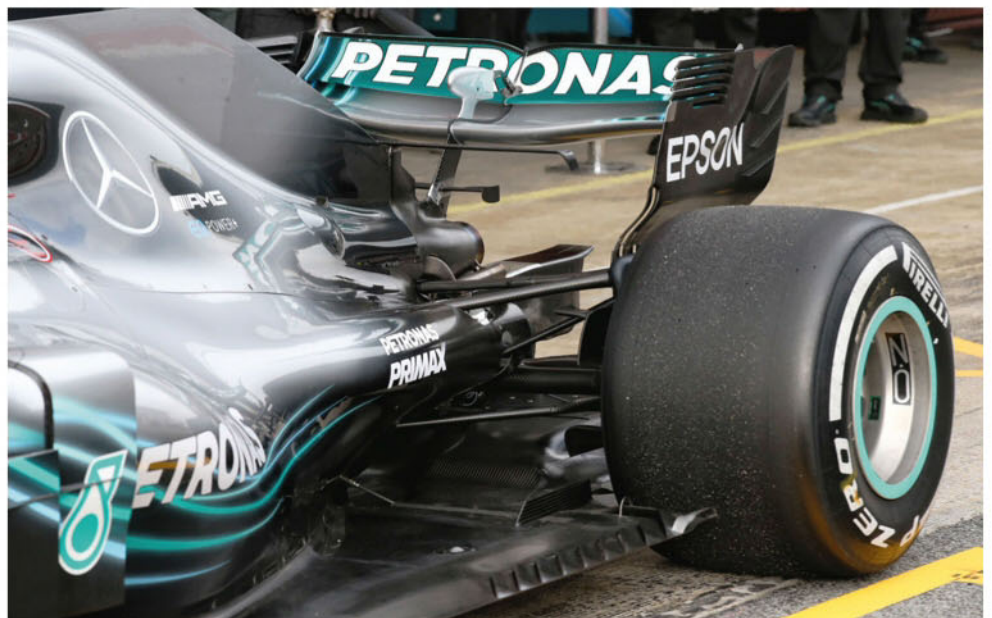
The loss of the T-wing is not total; some teams are trying to recover some of the effect with lower mounted winglets
