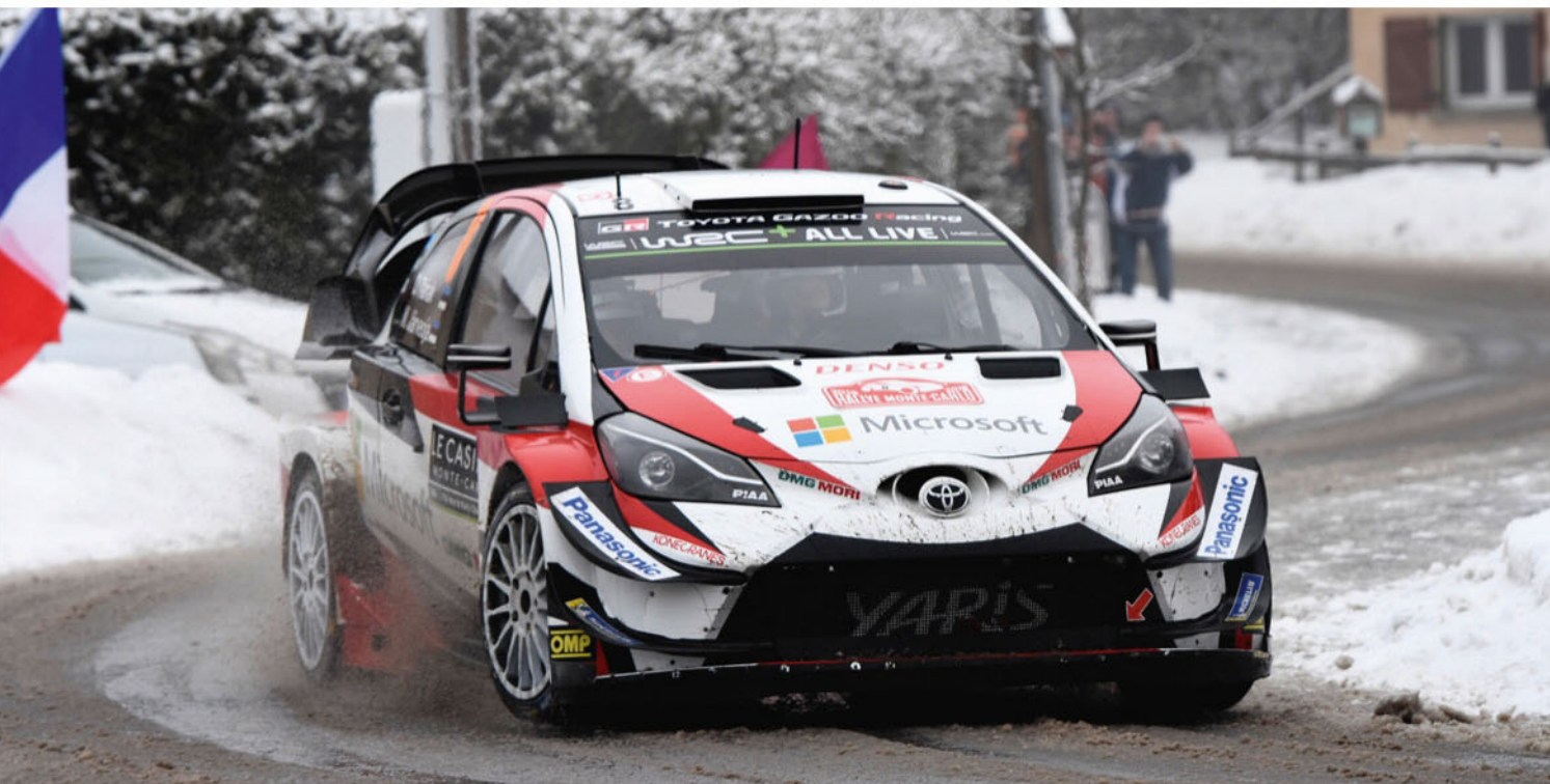
Toyota has worked on the front end aerodynamics and there are now two extra dive vanes. Revised front fenders help to improve the front downforce while also helping the cooling
