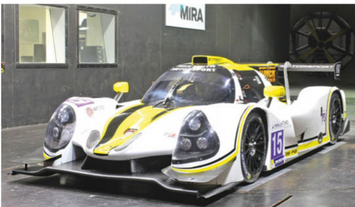
Ligier JS P3. Front end aerodynamic treatment is not dissimilar to that of an LMP2 car
