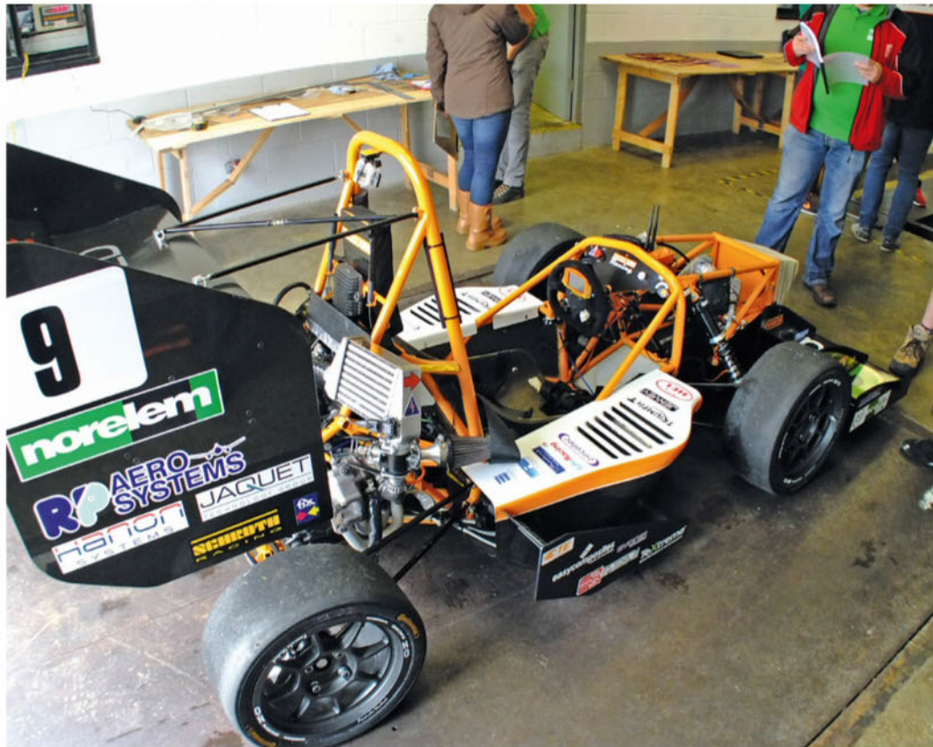
To achieve both high chassis stiffness and low mass with a tube frame there is a simple recipe to bear in mind: minimum of tube, minimum of nodes (ideally three tubes per node) and maximum of triangulation
