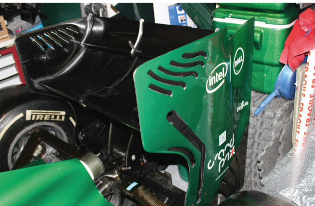
The rear wing assembly actually comes from a Force India but the pylons that support it are original Caterham components
