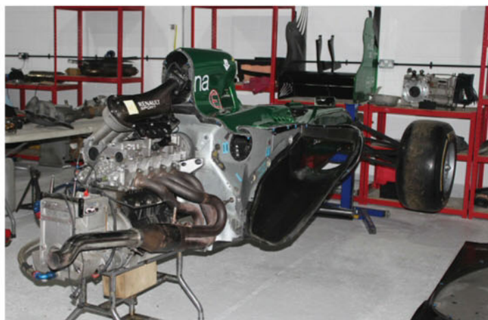
Formula Renault engine mounted in the back of CT05-1. A dose of realism meant any thoughts of a V6 hybrid were soon abandoned in favour of this 4-cylinder 2-litre engine
