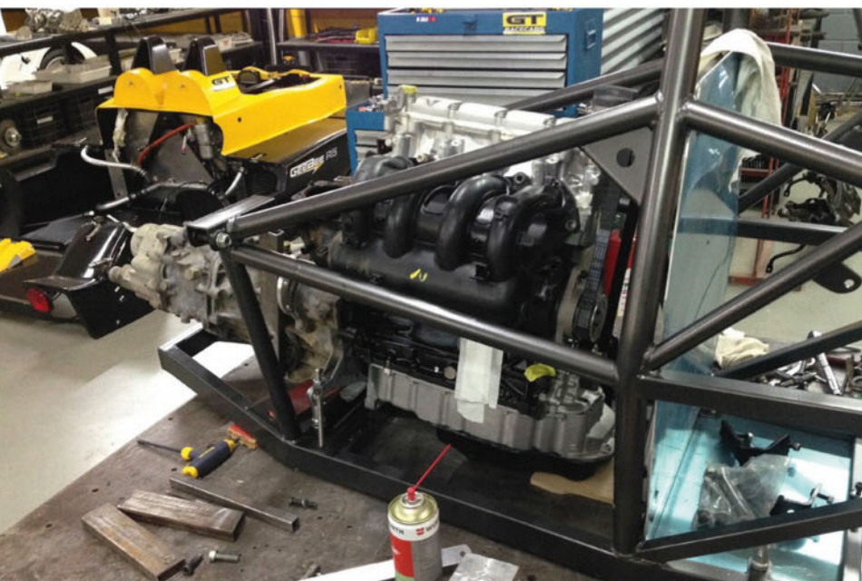
The original longitudinal-sited unit is a snug fit and in line with conventional single seater engine packaging
