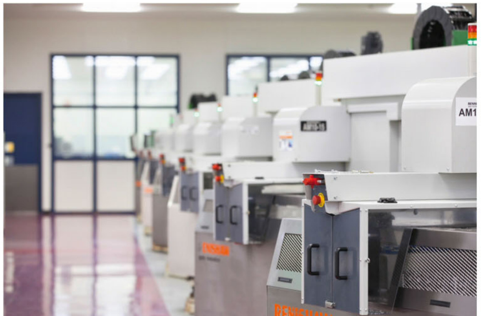
RAMTIC (Renishaw Automated Mill Turn Inspection Centre) consists of carousels that are plugged into each machine and automatically load the tools and materials. Up to 30 machines can be run by only two operators supported by kitting staff
