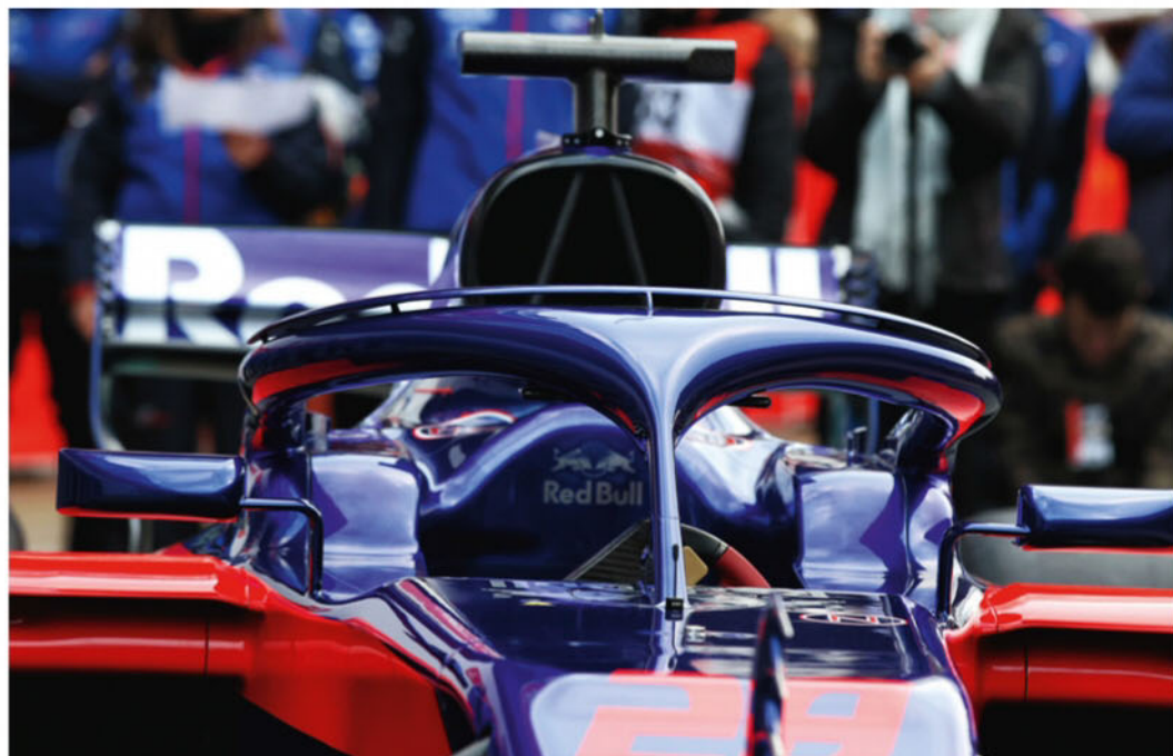
Toro Rosso is one of several teams to try to increase aero efficiency with its Halo design, one of many to choose this option
