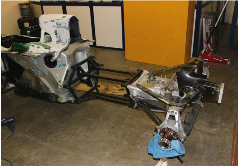
Frame for the Formula Renault engine and Sadev gearbox; fitted between the rear of the tub and the dummy transmission
