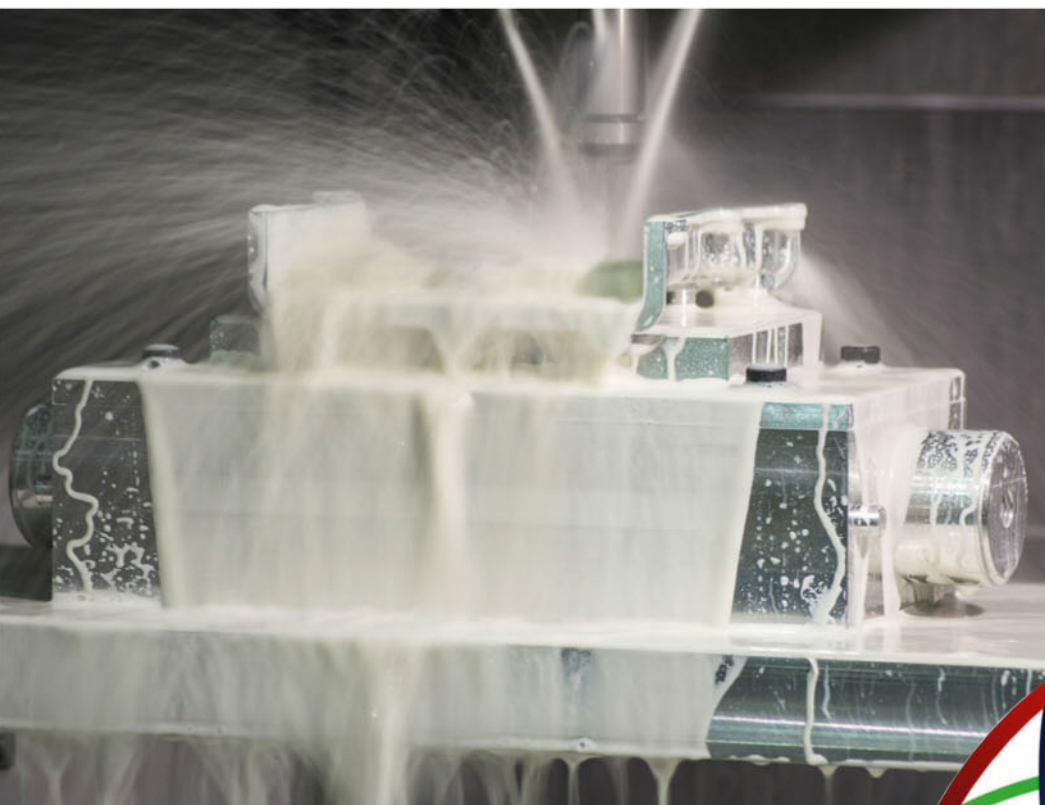
Liquid coolant is blasted at 1,000psi to the tip of the tool, reducing the temperature generated from friction. Coolant is also responsible for removing swarf which can sometimes weld itself to the part
