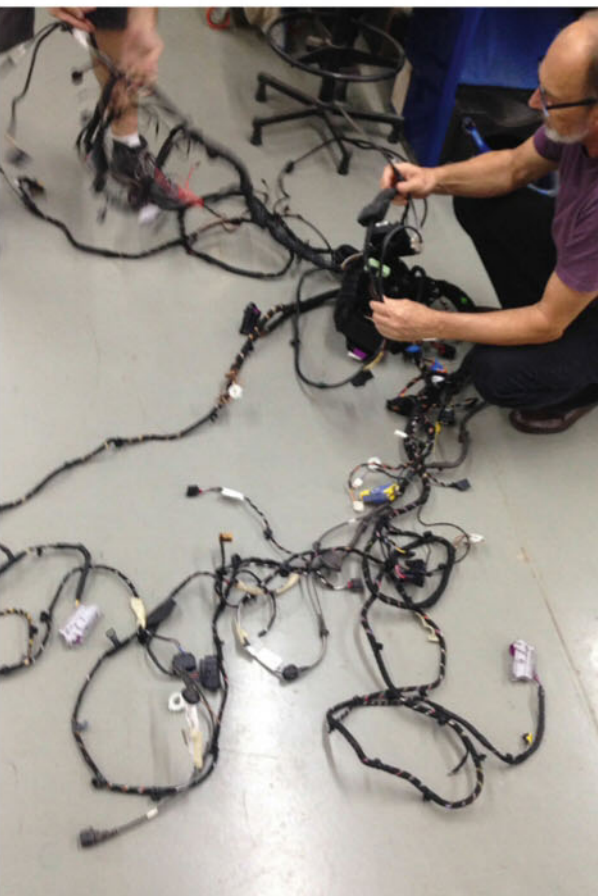
Left: Loom from the VW Up. It is a full throttle by wire, turbo control and double lambda ECU system. The immobiliser proved a headache for the team Above: A MacPherson strut from a VW Golf was inverted and machined to make an upright for the new racecar – an inspired and low cost solution Below: The current spaceframe design (in the foreground) with x-bracing, and original (behind) which will need the chassis tubes around the main hoop to be repositioned for strength. Note the rust!
