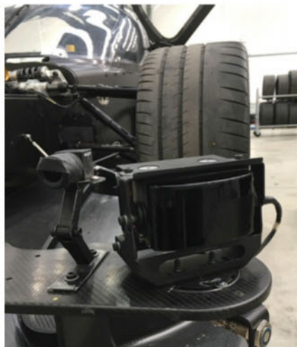
Similar to the set-up on the Robocar, the Devbot has five LIDARs, achieving a full 360-degree view around the car. A LIDAR on the front left corner along with a machine camera and an ultrasonic sensor underneath is shown on the left. On the right a LIDAR in front of the rear wheel, along with an ultrasonic sensor, is shown
