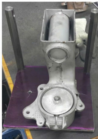
Left: Loom from the VW Up. It is a full throttle by wire, turbo control and double lambda ECU system. The immobiliser proved a headache for the team Above: A MacPherson strut from a VW Golf was inverted and machined to make an upright for the new racecar – an inspired and low cost solution Below: The current spaceframe design (in the foreground) with x-bracing, and original (behind) which will need the chassis tubes around the main hoop to be repositioned for strength. Note the rust!
