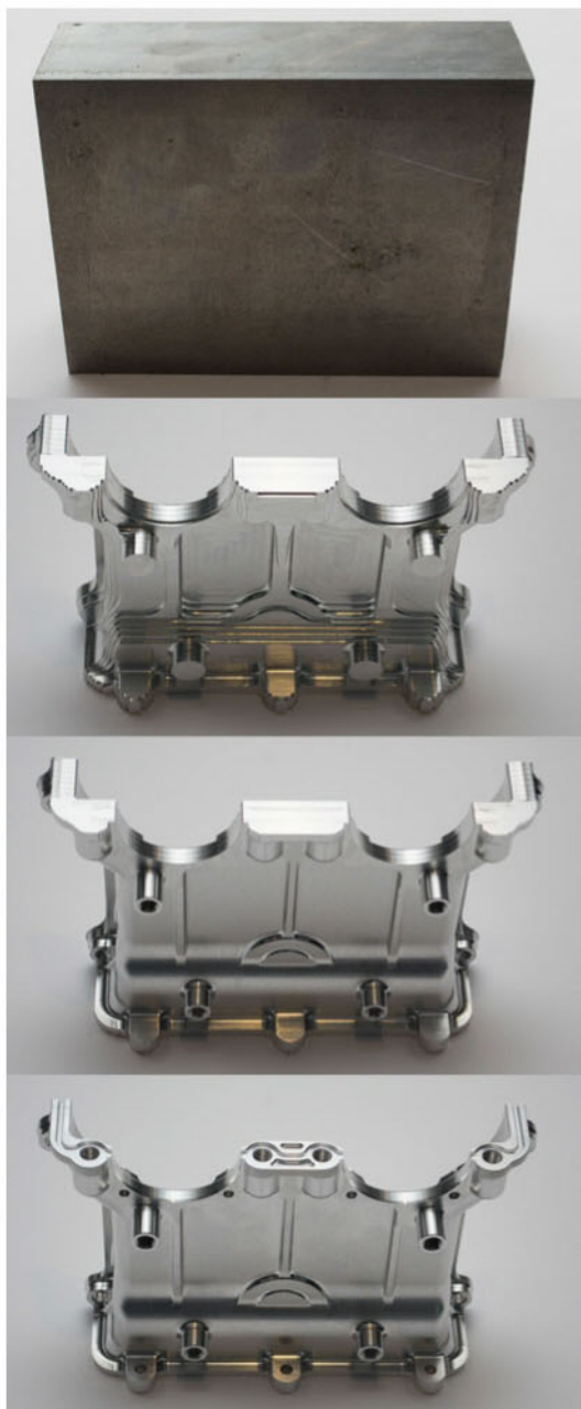
5-axis machines have the capability of machining a part from start to finish, creating intricate shapes out of a billet of material
