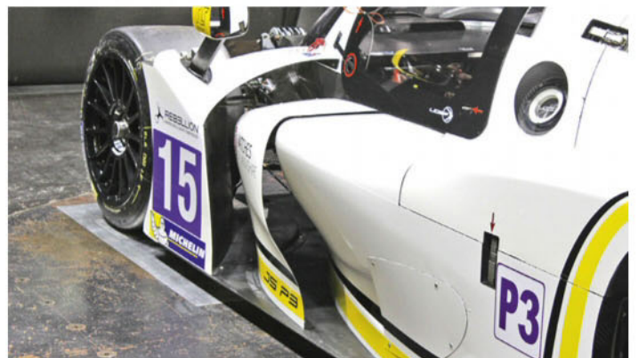
Clean exit for under-splitter air aft of front wheels; note the curved vane before sidepod
