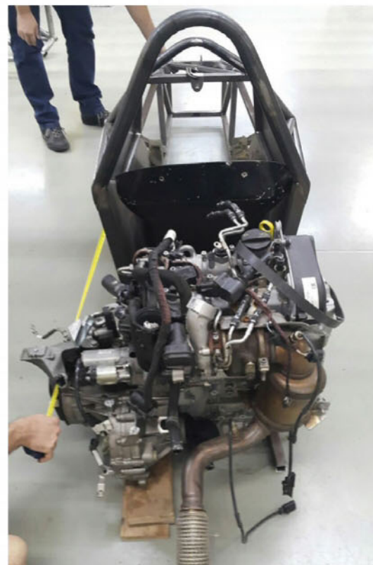
The extra width of the transverse unit from the VW Up is clear, but that was just the start of the problems for the team. The engine switch meant many changes, particularly to the rear suspension
