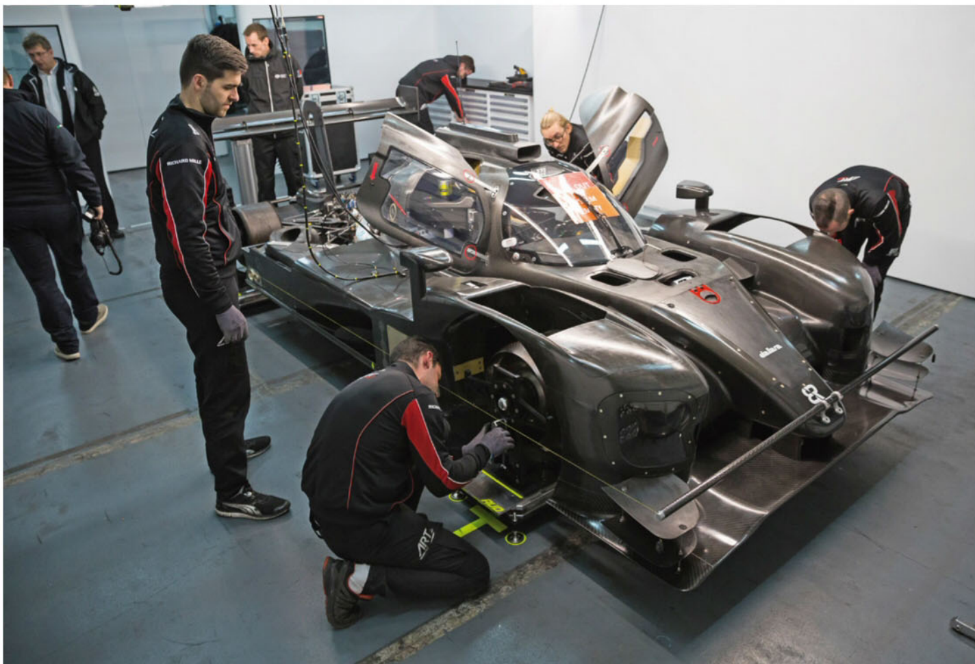
The front suspension has been changed from the LMP2 spec because of the narrower monocoque at the front, the different sized tyres and the shedding of weight from the chassis
