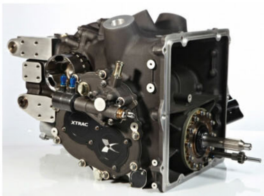
The Xtrac gearbox is carried over from the Dallara LMP2. The casing, and therefore the rear suspension design, is similar regardless of the engine installation that's chosen for the BR1
