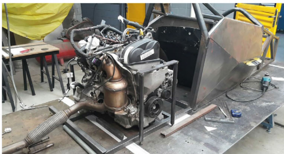
A frame was built to mount the engine/gearbox unit so it could be fired up and tilted 65 degrees to check oil pump pick-up
