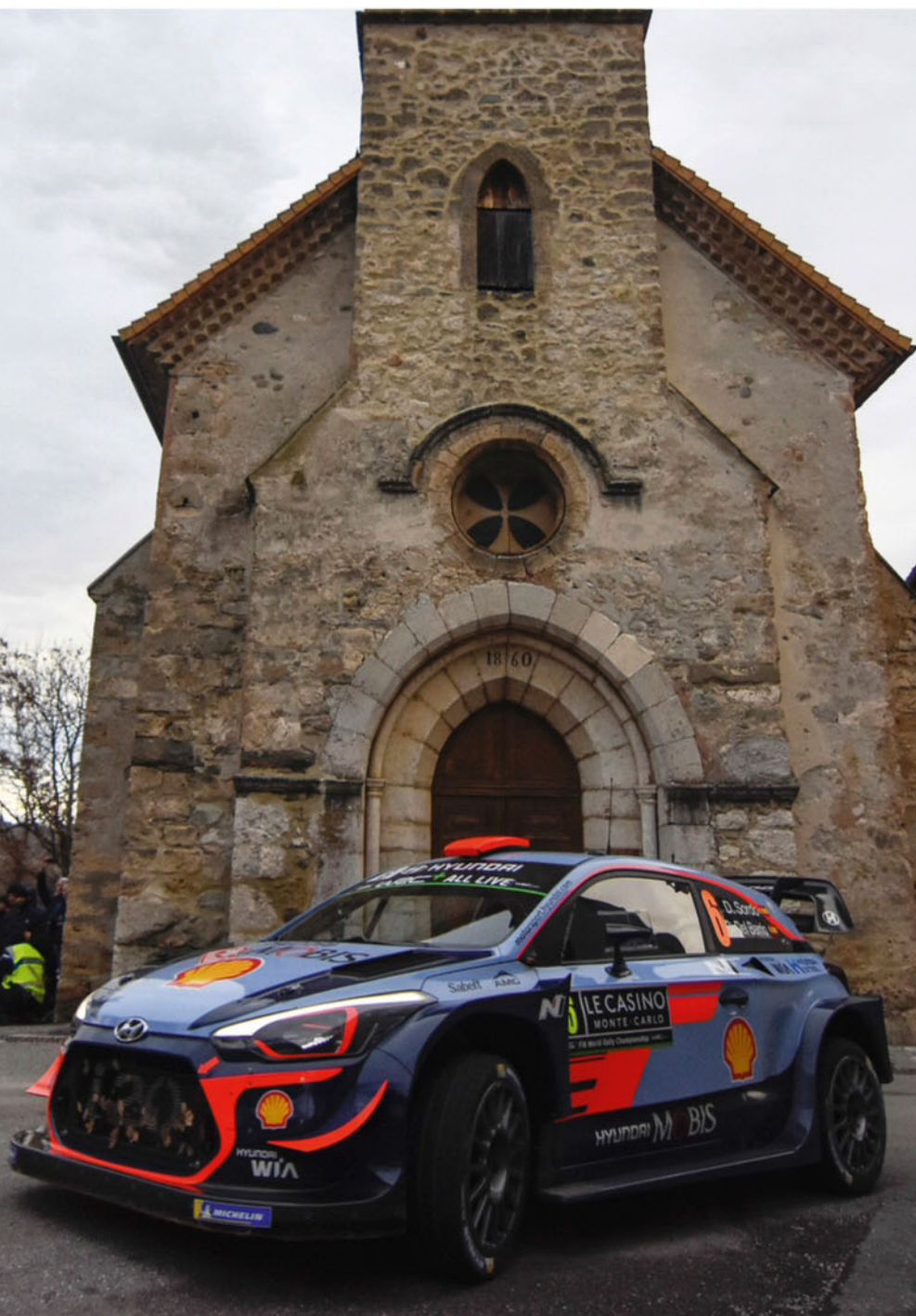
The Hyundai's splitter design is similar to the 2017 version but is now integrated into the front bumper. The i20's engine has a modified exhaust manifold, after the first iteration experienced problems with cracking, plus new fuel injectors and pistons
