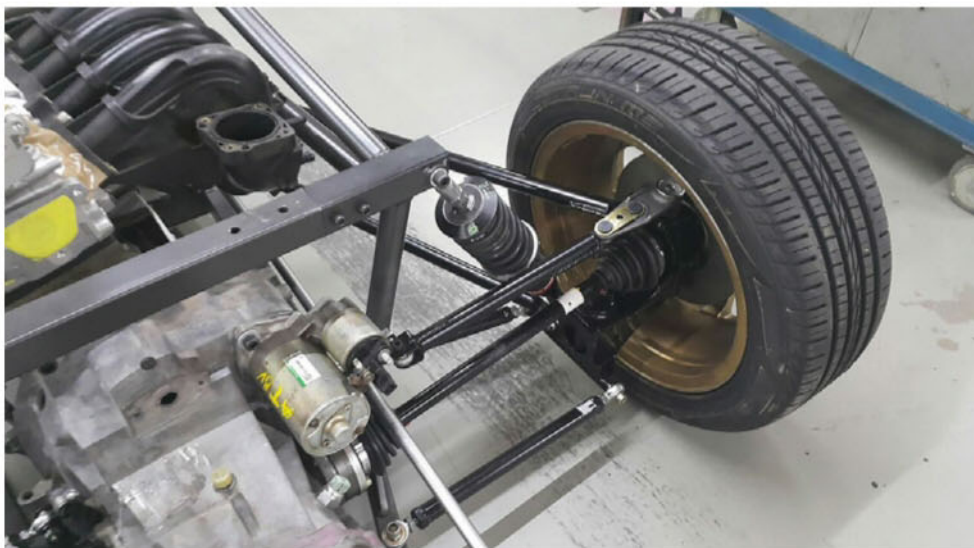
Fuse brackets have now been incorporated into the chassis design to help protect the spaceframe from damage in a crash
