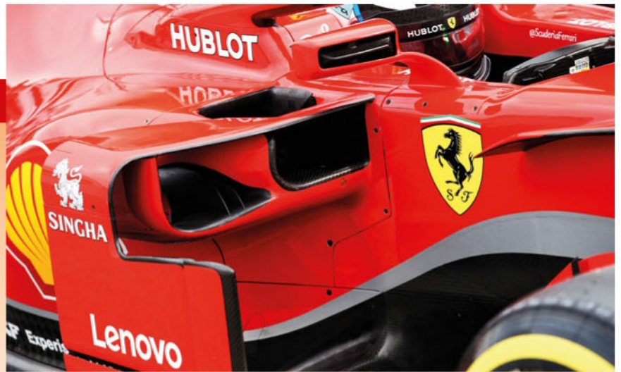
Sidepod design seems to be led by Ferrari, with impact structure relocation for efficient aerodynamic effect
