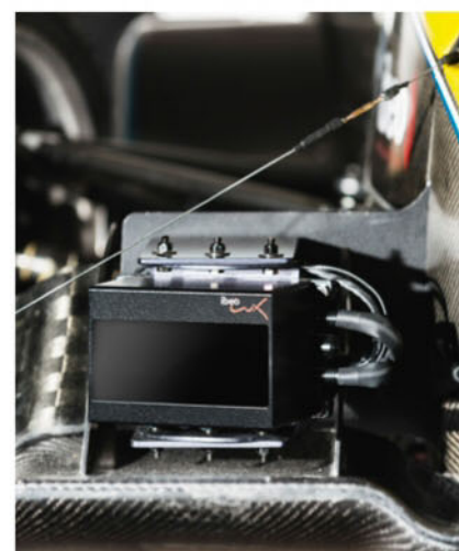
This year's car from KA-Racelng features three LIDARs at the front to increase the field of view. The team also removed some aero devices to minimise obstructions – because of the rather steady speeds of these cars they do not require much downforce
