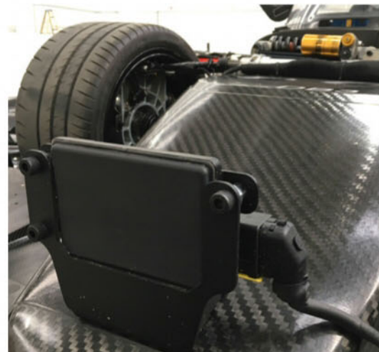
Both the Robocars and the Devbots benefit from two radars, one of which is at the front while the other one is at the rear; to give spatial information on the car's position within the environment
