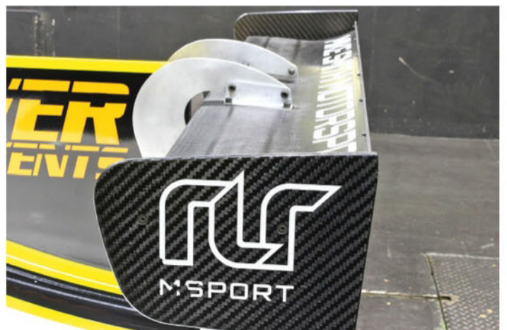
The rear wing features modest camber and is fitted with a mandatory 25mm Gurney flap
