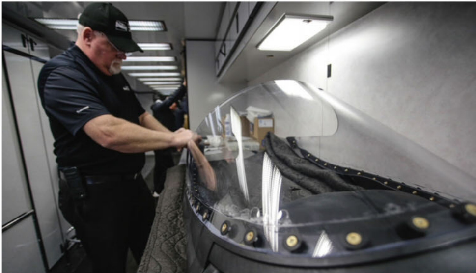
The screen is made from the same high-spec transparent material that its maker usually uses for the canopies of jet fighters
