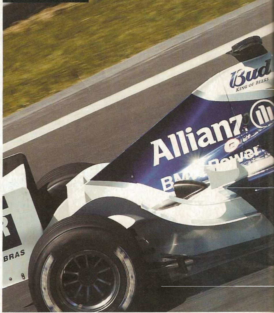
The brake ducts on Ralf's car were 30mm outside the limit
