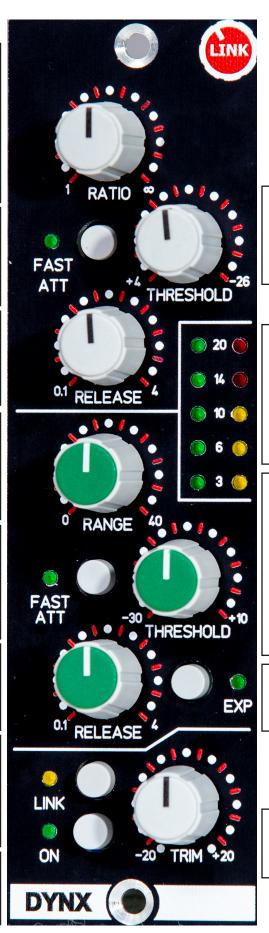
Whenever a signal exceeds the level set by this control, the compressor will start to act at the ration set by the RATIO control
