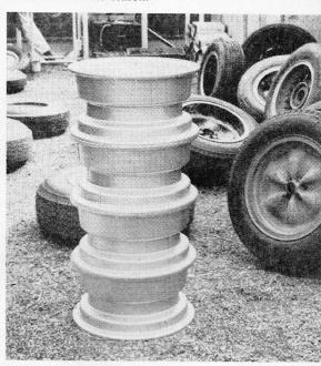
NEVER BE WITHOUT A CAPSTAN. A pile of 7½ in. rim, magnesium alloy Dunlop wheels as used at Aintree by B.R.M. and also destined for the Lotus-Ford "Indy" car.
