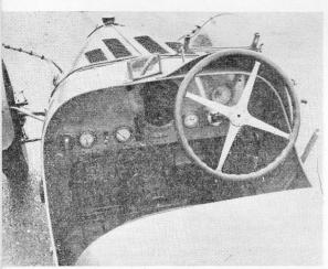
THE RIDING MECHANIC had the pressure pump on his left and the ignition advance and retard on his right. The magneto is just behind the large hole in the centre of the instrument panel.
