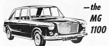
With transversely mounted twin carburetter, 1100 c.c. engine and frontwheel drive, the revolutionary MG 1100 achieves a masterly combination of performance, economy and spacious comfort. Many special features include entirely new hydrolastic 'fluid-smooth' suspension; front-wheel disc brakes; rubber-mounted body; wide vision; luxury finish; large boot capacity. See this most advanced MG of all time at University NOW. £714 inc. P.T. (4-door saloon). Part exchange, hire purchase, gladly
