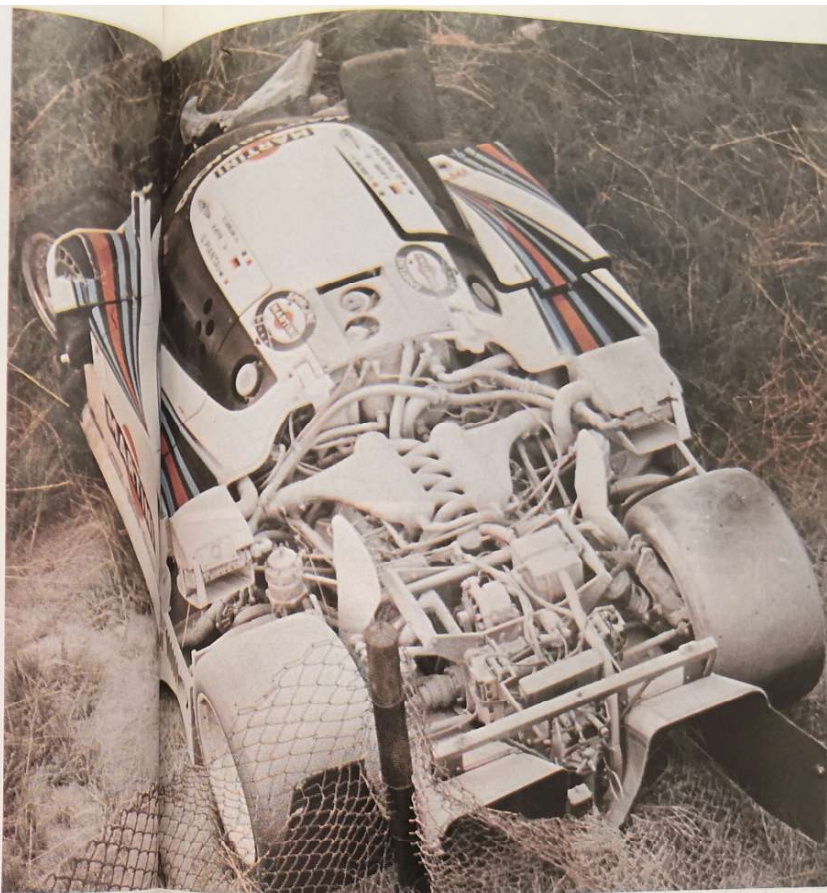
The wreck of the Ghinzani/Heyer/Pianta Lancia LC/2. The Italian car had a violent accident in the closing stages of the race while it was being driven by Heyer: first reports suggested that the cause was a steering failure. (photo: Asset)
