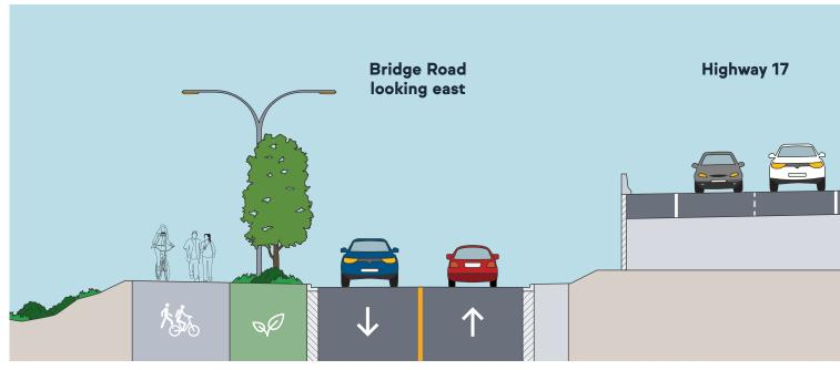
Cross-section illustration of two-way Bridge Road.
