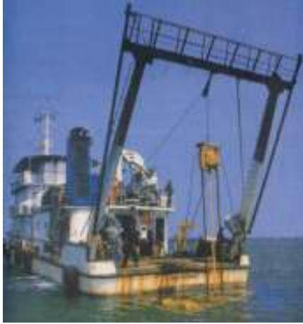
Fig.2: Vibro-corer being lowered from the aft-deck of RV Samudra Shaudhikama Fig.3: electrical motor of Vibro corer
