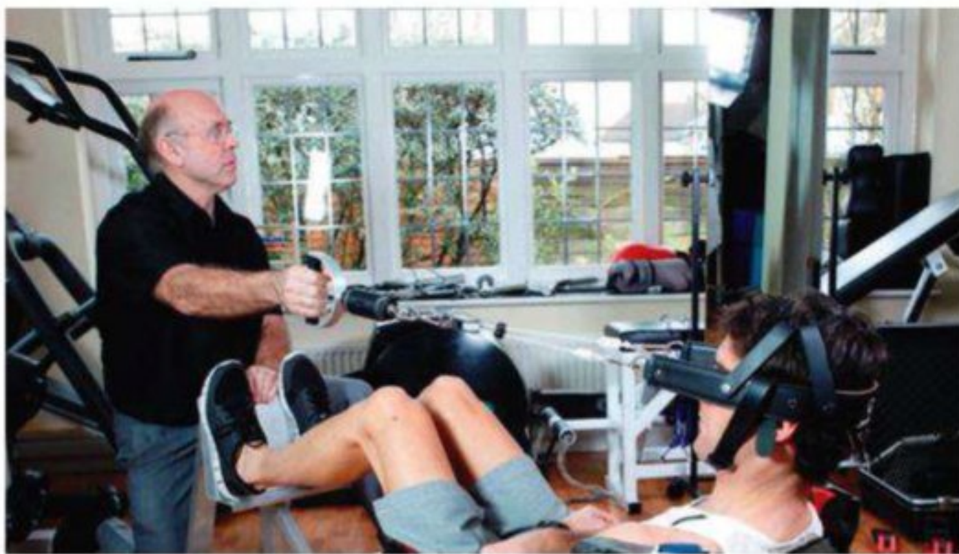
Neck muscles are particularly important for racing drivers, so tests have been designed to measure the muscles' resistance to an applied load. The subject resists as long as possible, and a graph of the results is produced
