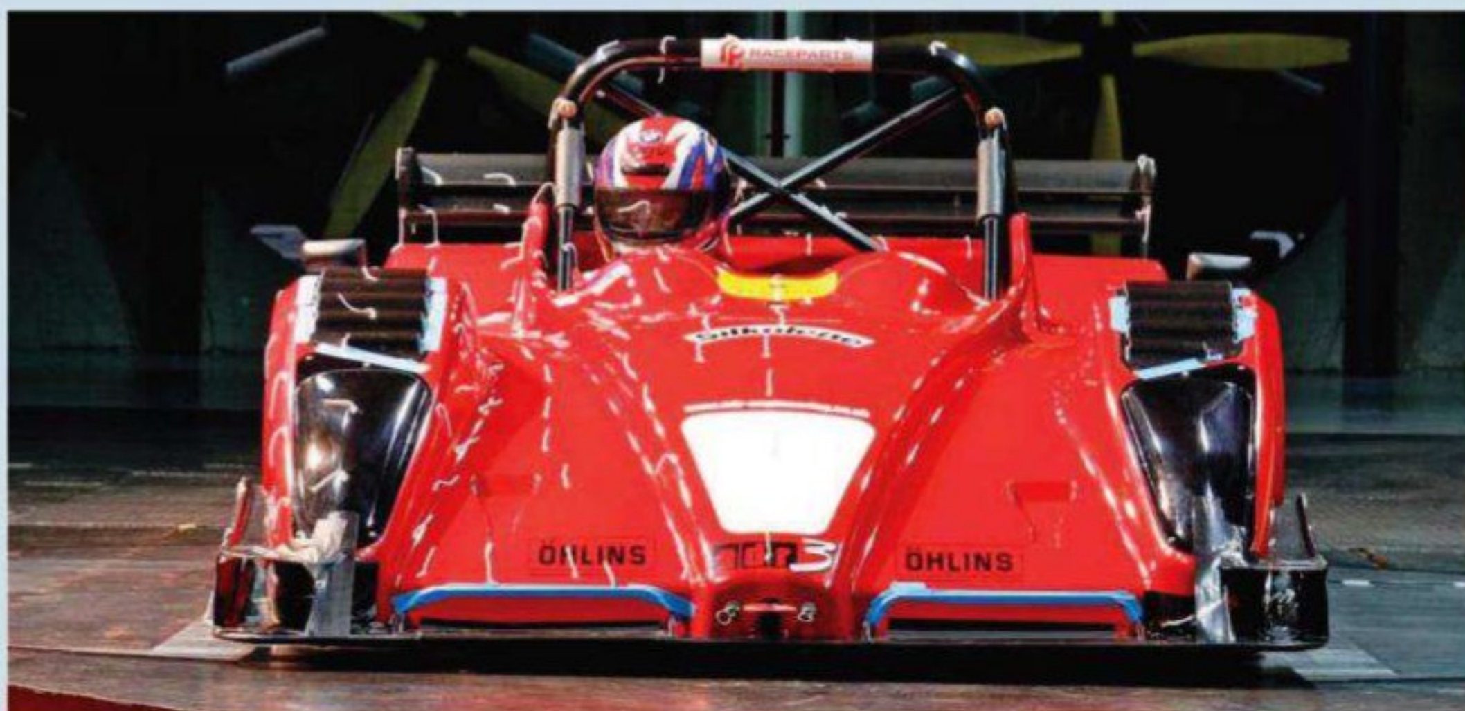
The ADR3 showed some interesting balance shifts when yaw angle was applied to the car in the wind tunnel
