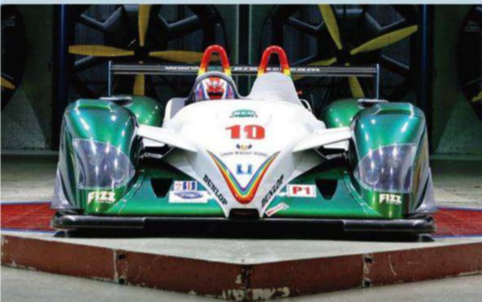
Figure 1: The ADR3 demonstrated a decrease in front downforce with yaw angle, whereas rear downforce increased
