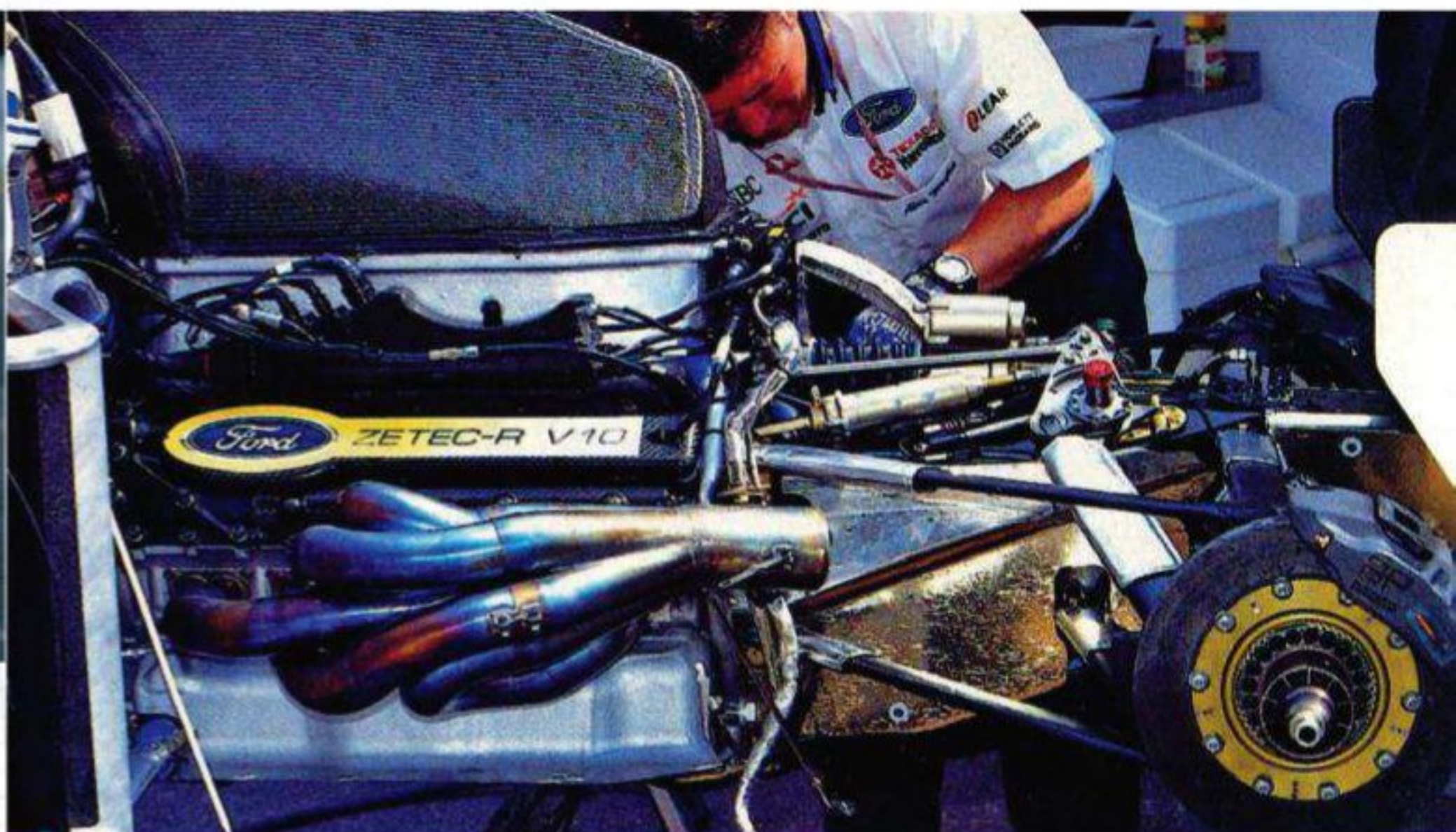
The Stewart-Ford SF2 featured a revolutionary carbon fibre gearbox, but it proved to be a massive resource drain and was dropped for the following season, which saw the SF3 win at the Nürburgring
