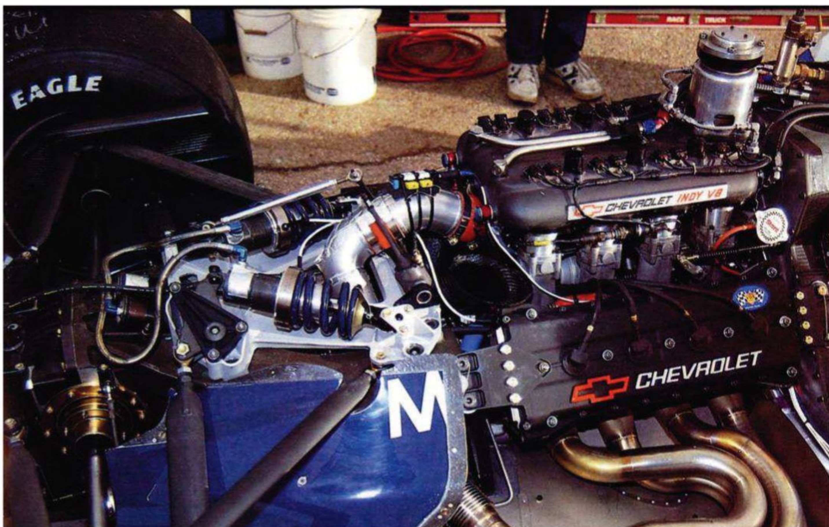
The Indy 500-winning Galmer, which has a single turbo mounted in the bellhousing behind the engine - a layout likely to appear in F1 in 2014
