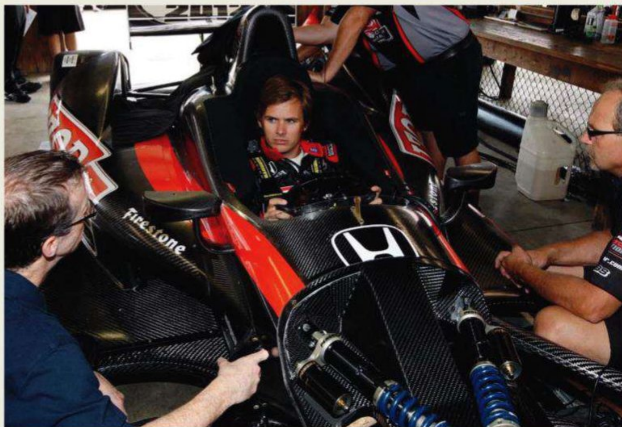
Increased cockpit size is a bonus for bigger drivers, but steering wheel-mounted hand clutch is the biggest change
