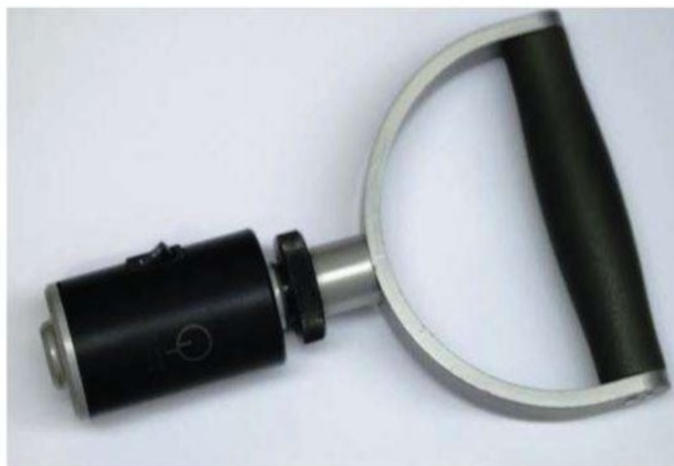
The load cells used by Gatherer are supplied by Beru F1 and are the same as the ones used on the suspension of Formula 1 cars
