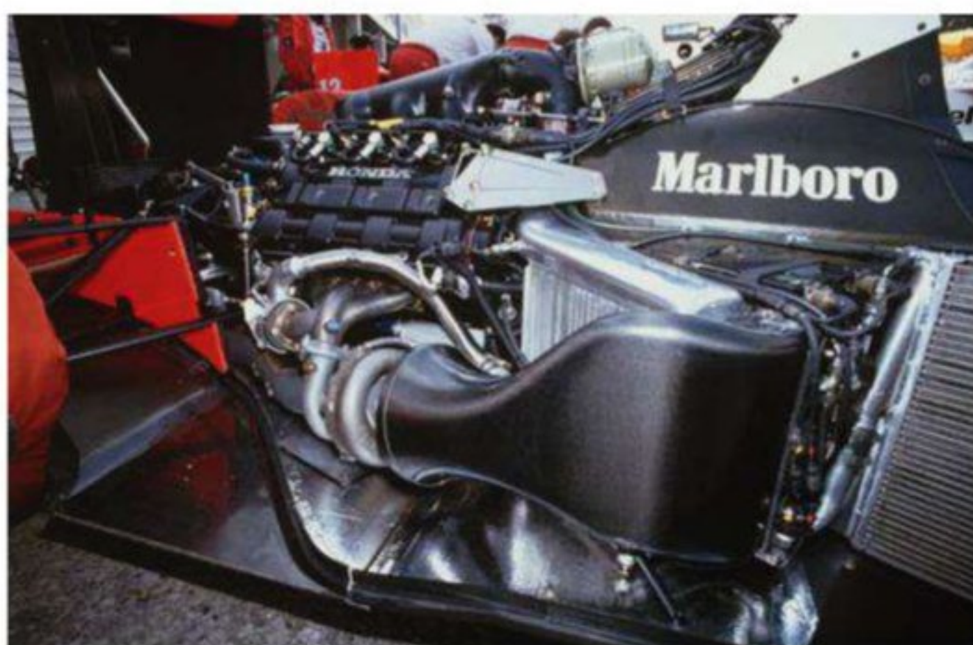
The last time forced induction was used in Formula 1 was in 1988, when McLaren dominated the formula with twin-turbo Honda power
