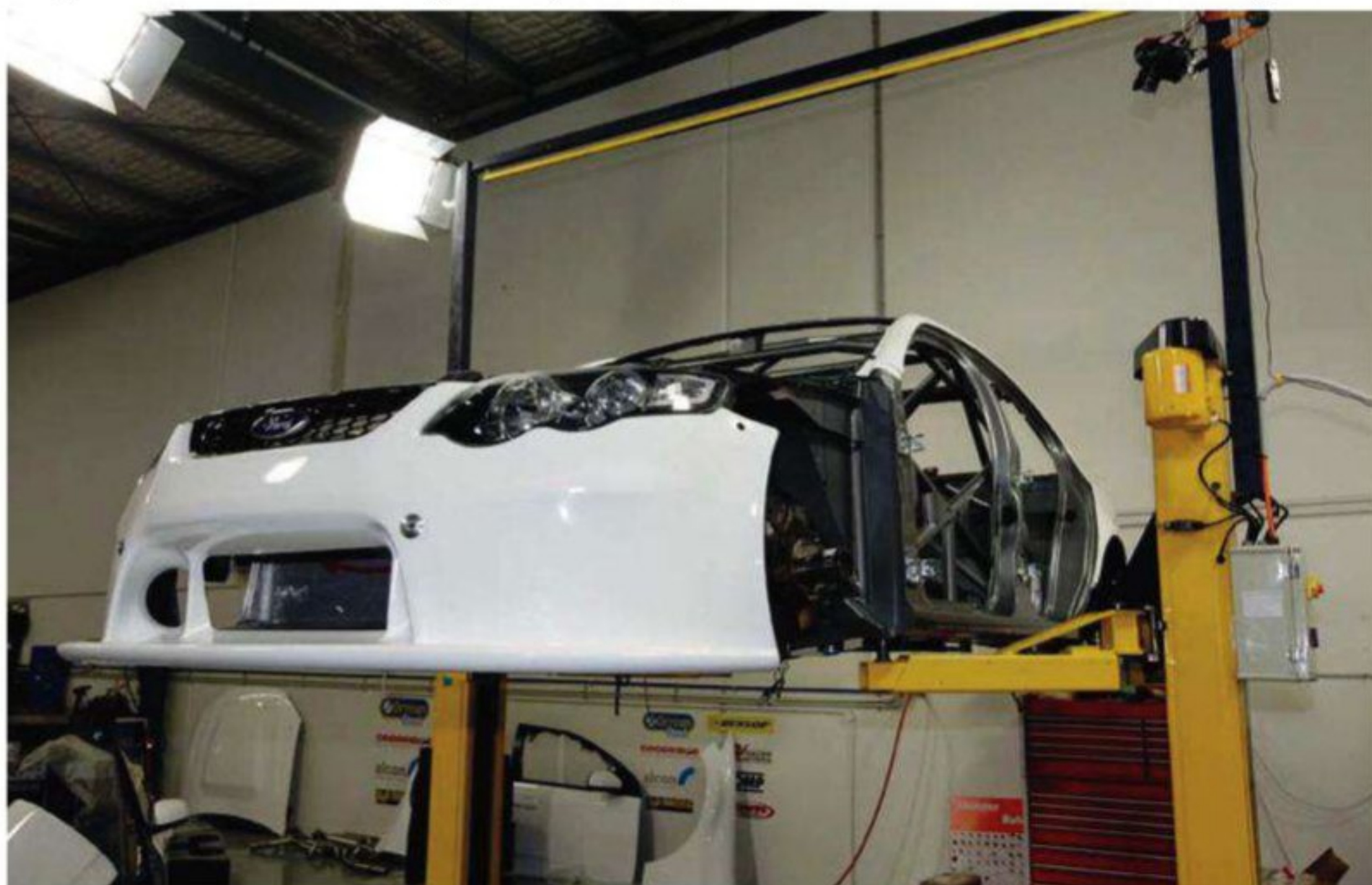
The current carbon / Kevlar front splitters and adjustable rear wings which be retained for the time being, keeping downforce and drag levels at a similar level to the current cars, and the aero balance the same at around 53 per cent
