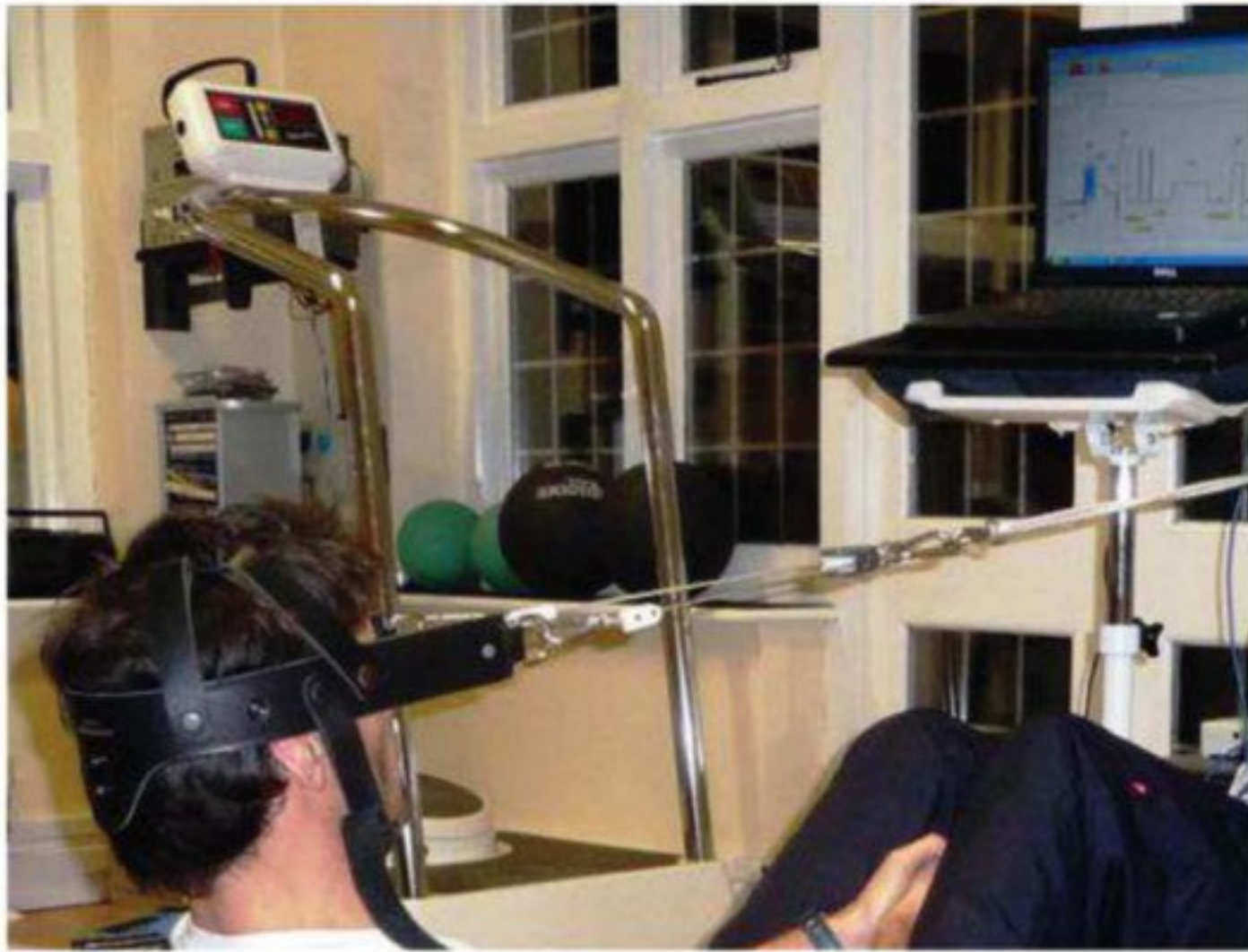
The load cell is incorporated into a device that allows measurements to be taken in either tension or compression. An endurance test using a constant load can be used to measure a subject's stamina
