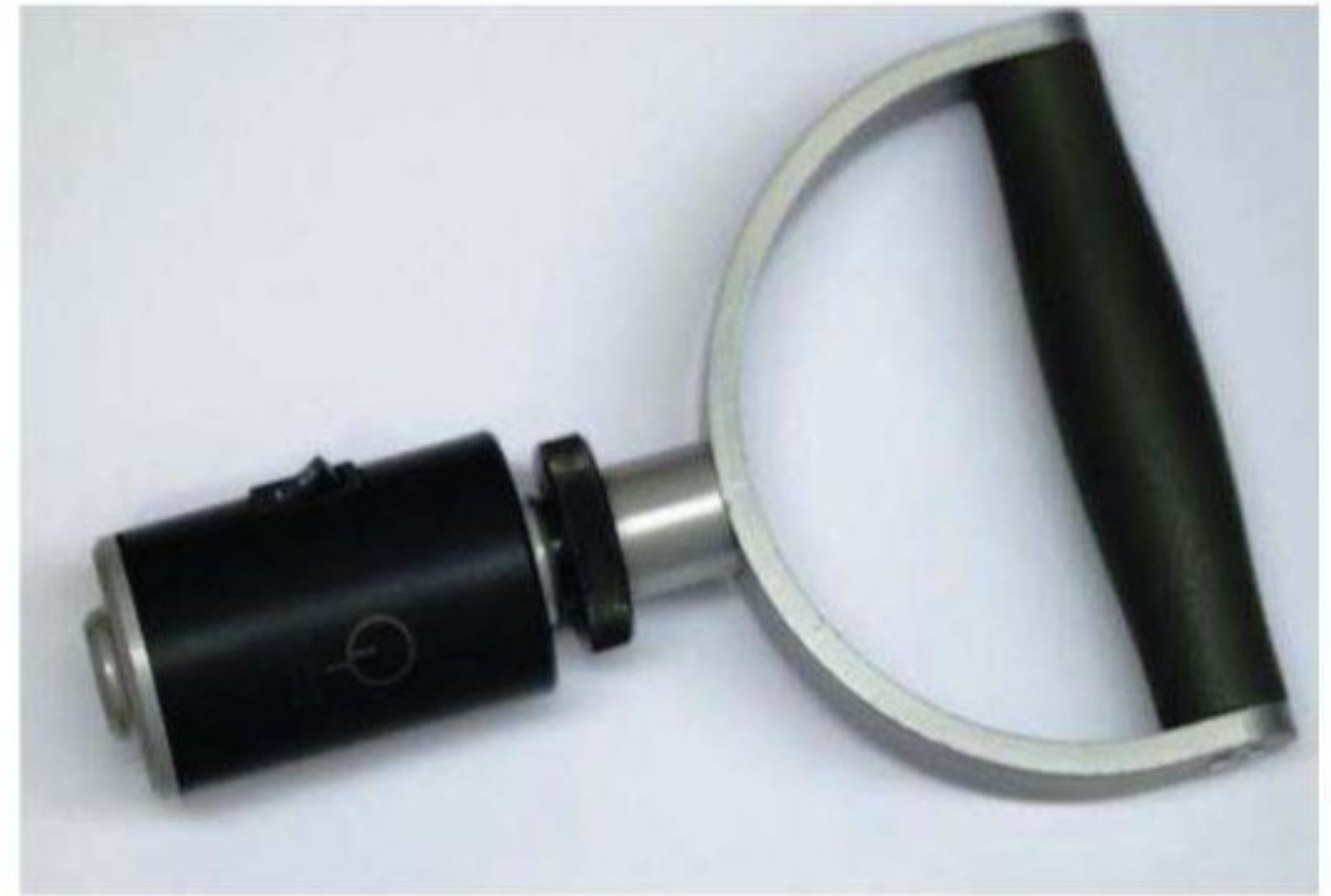
The load cells used by Gatherer are supplied by Beru F1 and are the same as the ones used on the suspension of Formula 1 cars
