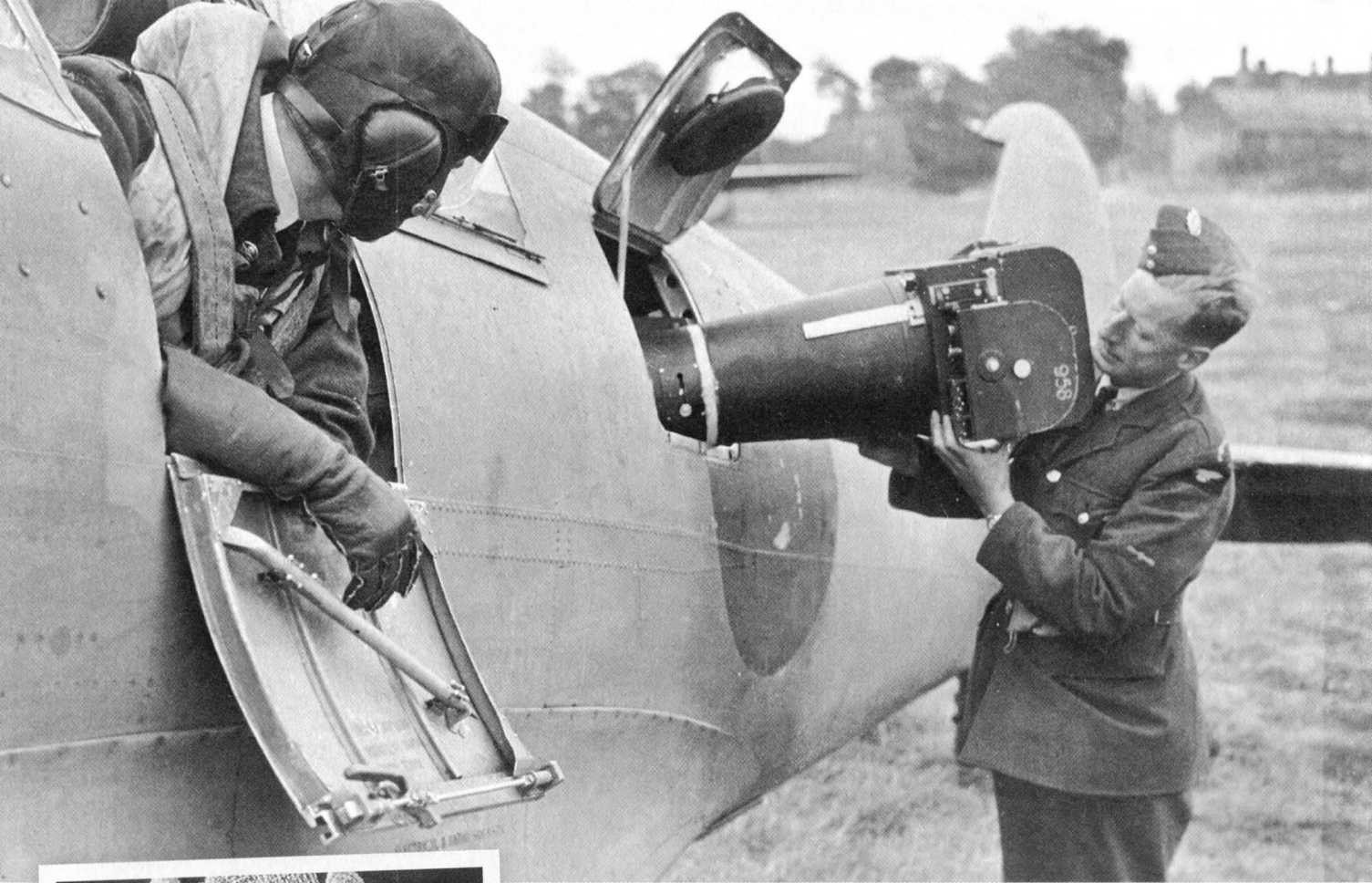
PR (Photo Recon) Spitfires were fitted with one, but usually two, long focal length, very large format cameras. From as high as 30,000 feet, they shot overlapping, fine-grain film strips that when viewed through a pair of special magnifying "glasses" gave a slight three-dimensional effect. (Photo courtesy of Joe Gertler)
