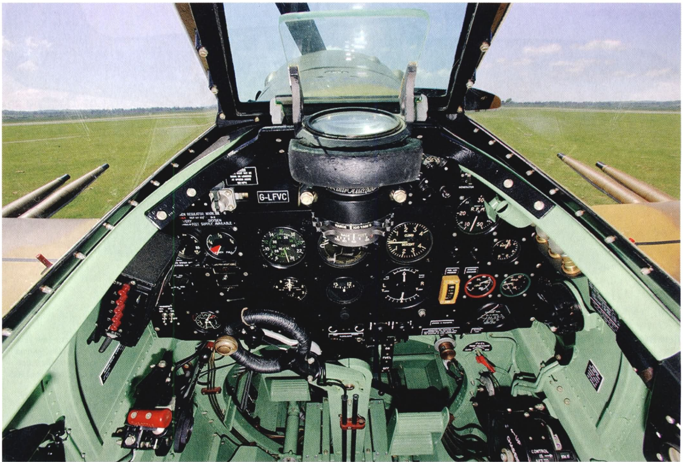
Spitfire LF Mk Vc JG891's cockpit. The majority of Mk Vcs were sent overseas, with many serving in North Africa or the Mediterranean. Usually fitted with two wing-mounted cannons, four cannons are visible here. The extras were fitted to Malta-bound Spitfires: an ingenious way of importing spares to the besieged island. (Photo by John Dibbs/planepicture.com)
