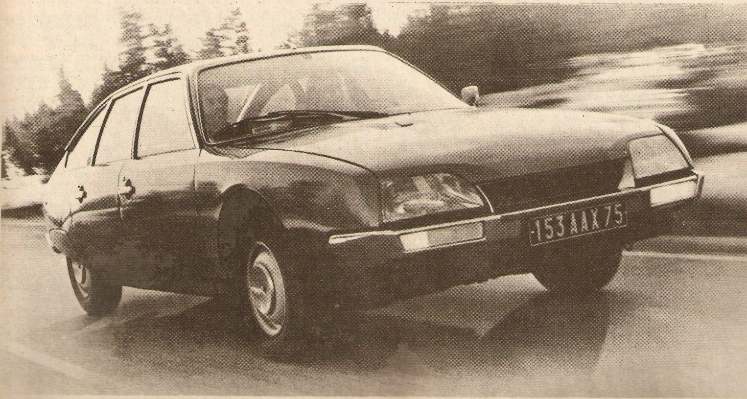
The Citroën CX exemplifies many of the desirable features described in the text. The airflow beneath the car and through the radiator have received particular attention, two areas which have been totally neglected by most manufacturers.
