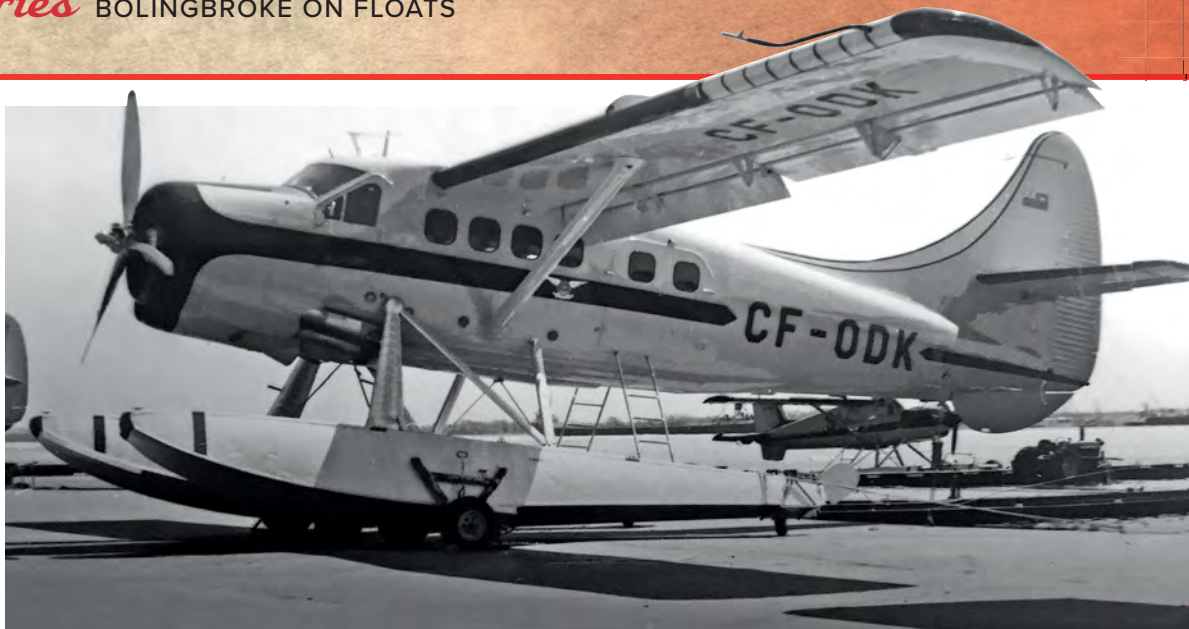
RIGHT De Havilland DHC-3 Otter CF-ODK at Sault Ste. Marie, Ontario, has been pushed from hangar to river side on the same beaching gear used for the 717 'Water Bolly'.
