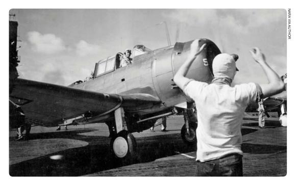
ABOVE Even in the heat of battle the US Navy made sure official war photographers were on hand to document the action. One of numerous excellent images captured during the raid on Truk, this example shows a deck handler directing forward a VB-10 Dauntless with a 500lb bomb under the fuselage, for launch from the Enterprise.
