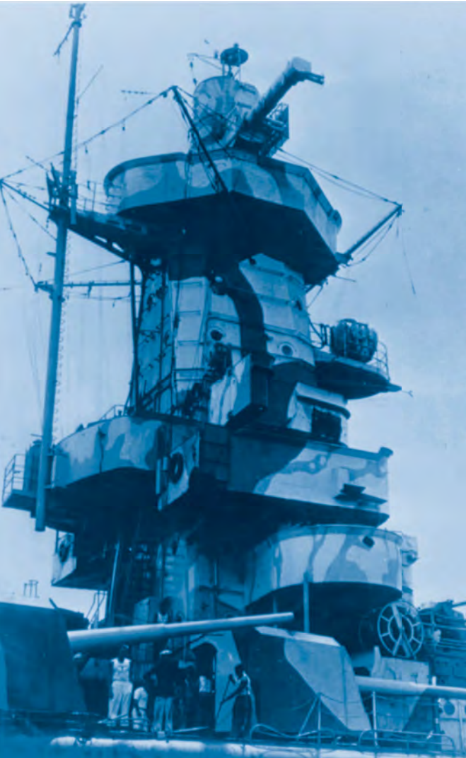
ABOVE: Graf Spee's Seetakt radar antenna and 15cm broadside guns. (USNHHC)
