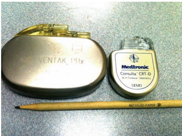
FIGURE 18-42 ▲ Implantable cardioverter–defibrillators (ICDs), old and new models. Note the decrease in size and weight that has been achieved with the newer generation, allowing prepectoral implantation. (Courtesy of Medtronic Inc. Minneapolis, MN.)
