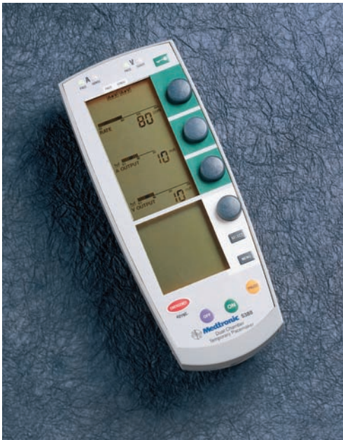
FIGURE 18-33 ▲ A dual-chamber temporary pacemaker. (Courtesy of Medtronic, Minneapolis, MN.)
