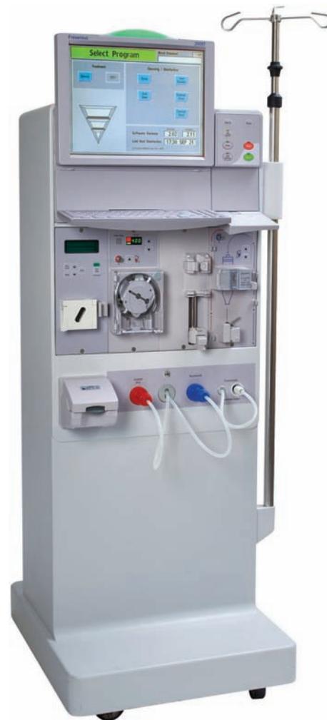
FIGURE 30-2 ▲ Hemodialysis delivery unit, which includes an automatic blood pressure cuff, heparin infusion pump, and blood pump. This machine displays a continuous readout of ultrafiltration goal, rate, and total fluid removed and monitors dialysate temperature and conductivity. It can vary the sodium concentration of the dialysate. (Courtesy of Fresenius 2008T Fresenius VSA, Inc., Concord, CA.)
