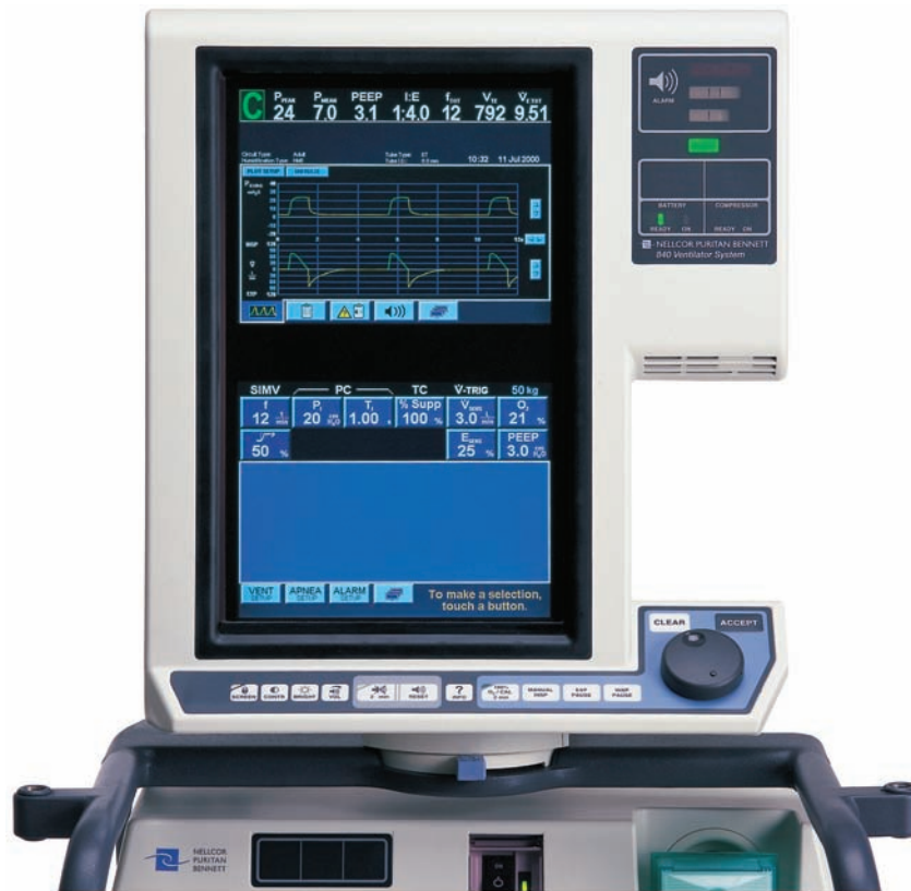
FIGURE 25-8 ▲ The Puritan-Bennett 840 (PB 840) Ventilator System. The close-up photos of the screens and controls are an example of the type of controls used with computer-controlled ventilators.
