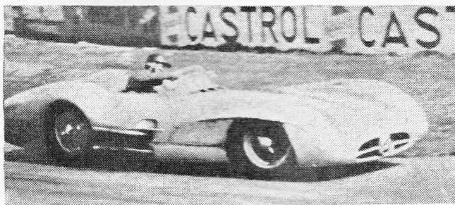
ILL-FORTUNE for Hans Herrmann, testing the new Grand Prix Mercedes-Benz at Hockenheim. Hot oil from a burst pipe caused him to lose control, and to avoid two small girls he crashed into a wall. What appears to be an inboard front brake is exposed in the wreck.
