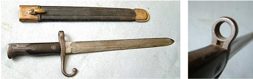
Vettereli shortened and bushed for an unknown rifle. Possibly for UK Home guard.
