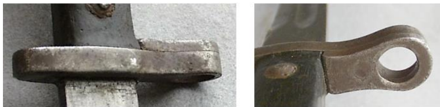
M1935 modified for M1 Garand rifle. Modified by adding an additional plate onto the existing crossguard of a M1935, this new plate has a smaller off centre hole designed to mate with the Garand flash hider.
