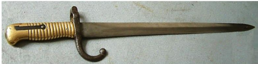
Defense Nationale bayonet using an 1866 style hilt and a re-used double edged sword blade. Chassepot style muzzle ring with cut out, and Remington style un chamfered slot. Bottom rivet is missing and shows only a dimple where the hole would be drilled
