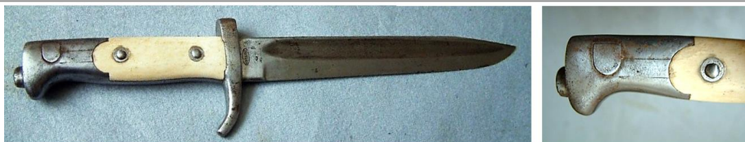
M1870 shortened and with replaced grips (ivory, bone or a pale composite). The original spring has been removed.
