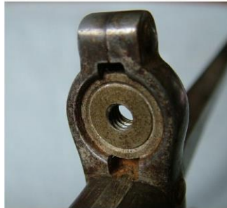
1874 Gras with muzzle ring filled with brass threaded plug. Stud is permanently fixed as adjustment screw on top of muzzle ring has been riveted. This conversion is to allow the bayonet to be used as an earth for telegraphers.
