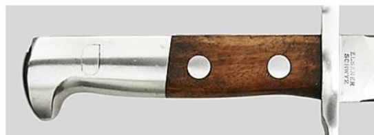
Elsener began producing the M1918/55 variant that combined the M1914 hilt with the M1918 blade. Hilt on the M 1918/55 (left) is 1-3mm thicker compared to the standard M1918 (right).
