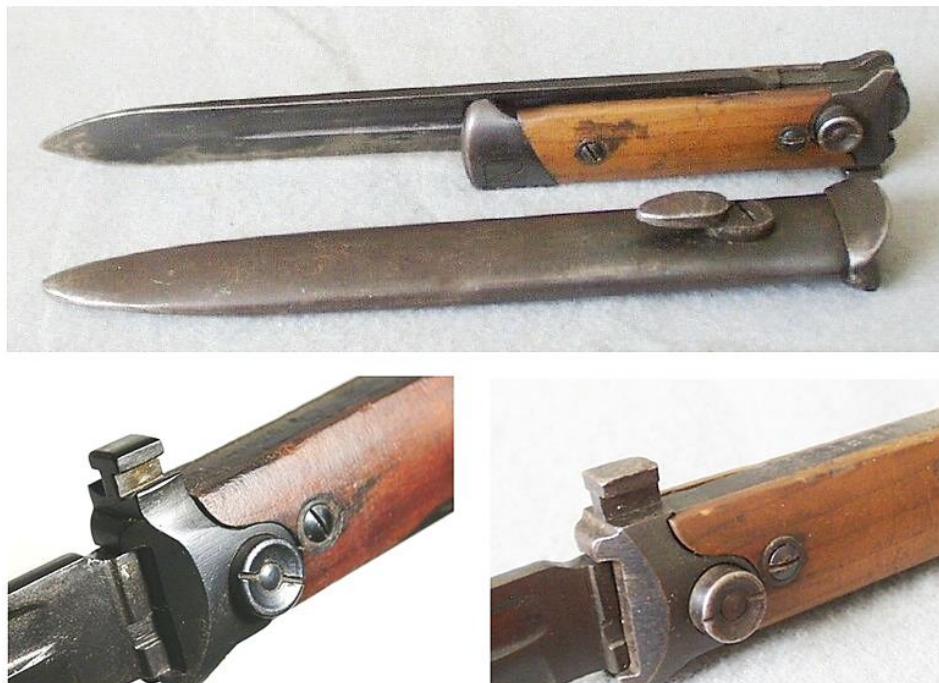
Folding bayonet for Beretta Model 38 submachine gun. It has a T-shaped attachment stud, compared to the Carcano M38 muzzle ring. Very rare bayonet.
