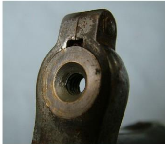
1874 Gras with muzzle ring filled with brass threaded plug. Stud is permanently fixed as adjustment screw on top of muzzle ring has been riveted. This conversion is to allow the bayonet to be used as an earth for telegraphers.
