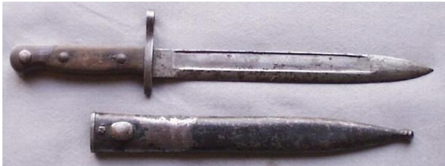
M1935 with squared fuller (blade from unknown bayonet).
