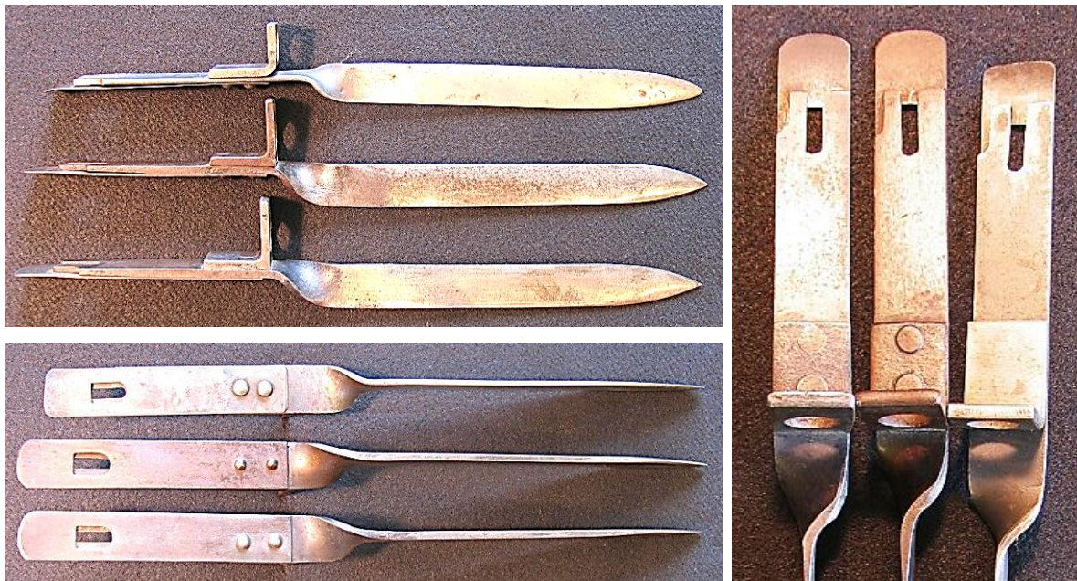
Different variations. Size, rivets position and size, muzzle ring shape varies.
