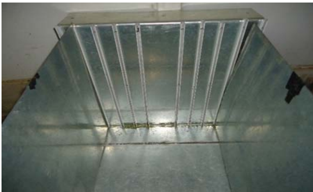
Figure 2. The actual picture of the chamber showing aluminum studs and capacitor plates in the chamber chamber
