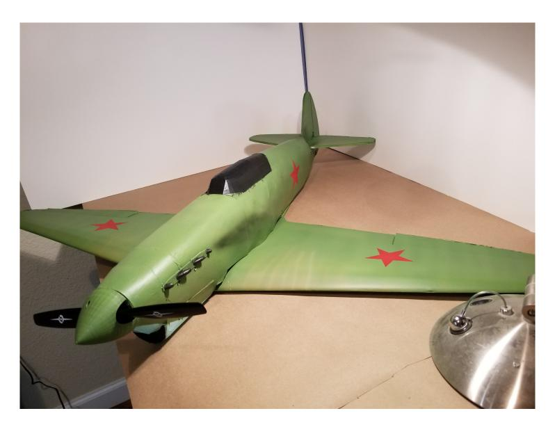
Note that the hole for the motor mount is measured for a flite test C-Pack motor, the GT2215/09. Also, be aware that your skin stencils may vary due to build imperfections so always cut bigger than your need and trim down after gluing.
