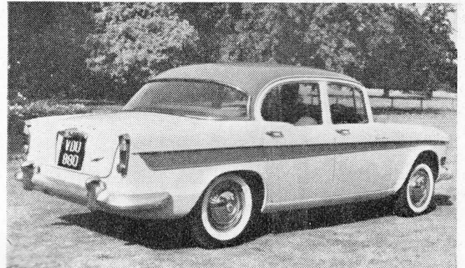
HUMBER: The Super Snipe now has a 3-litre engine and vacuum-assisted brakes, discs being employed in front. Stiffer anti-roll bar improves stability and maximum speed is over 100 m.p.h.
