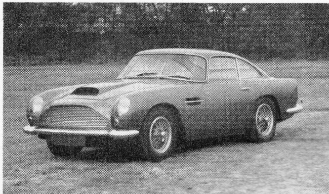
ASTON MARTIN: The new DB4 G.T. model was announced last month. A 3.7-litre engine produces 302 b.h.p., which is transmitted through a 9 in. twin-plate clutch and Salisbury "Powr-Lok" differential.
