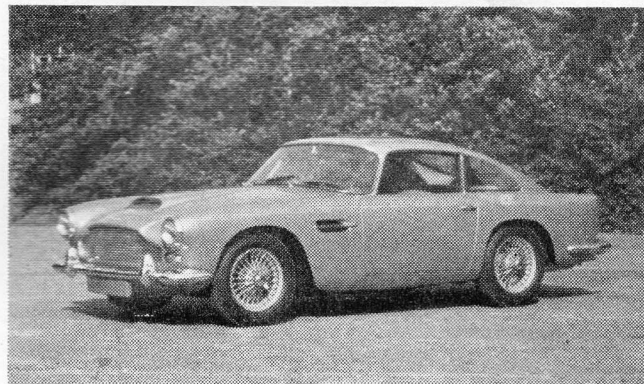
ASTON MARTIN: First shown last year, the normal DB4 3.7-litre coupé has a 240 b.h.p. engine, with four-speed all-synchromesh gearbox and Dunlop disc brakes on all four wheels.
