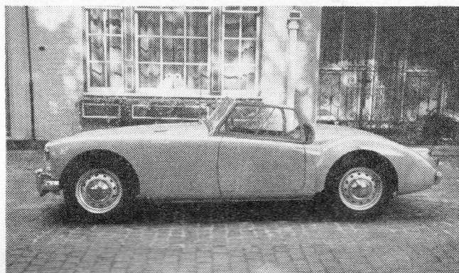
M.G.: High performance from Abingdon is represented by the new M.G.A 1600, with "B" series engine enlarged to 1.589 c.c. and giving 78 b.h.p. Lockheed disc brakes are fitted to the front wheels.
