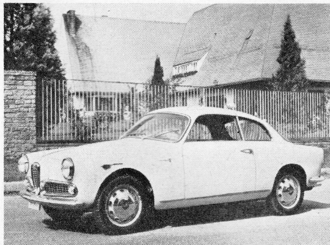
ALFA ROMEO: Giulietta Sprint coupé, a four-cylinder, 1,290 c.c. thoroughbred with a maximum speed of over 100 m.p.h., its engine developing 80 b.h.p. at 6,000 r.p.m. A four-speed gearbox is fitted.
