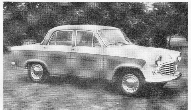
STANDARD: The Vanguard has a 68 b.h.p., 2-litre engine and a maximum speed of 84 m.p.h. Fuel consumption is in the 28-34 m.p.g. bracket, and the car is famous for its reliability.
