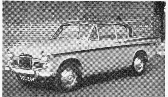
SUNBEAM: The new Mark III Rapier now has a 78 b.h.p. engine, disc brakes on the front wheels and a new, close-ratio gearbox, and revised interior trim and greater comfort.
