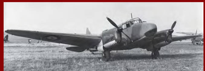
ABOVE: Oxford AS504 looking somewhat ungainly with its two Gipsy Queen IV in-line engines. AEROPLANE
