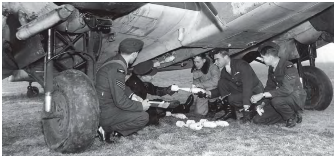
ABOVE: Practice smoke bombs being fitted to an Oxford's under-fuselage bomb rack. AEROPLANE
