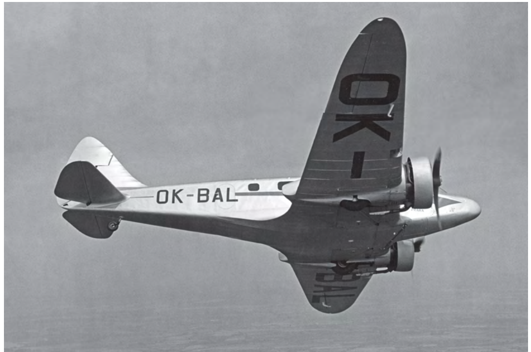
ABOVE: The first of the four Walter Castor-engined Envoys for Czechoslovak carrier CSA was OK-BAL, pictured pre-delivery in 1935. AEROPLANE
