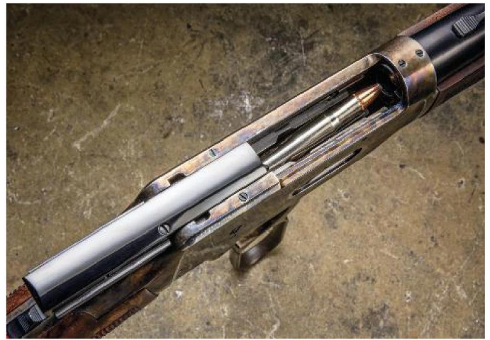
As Browning intended it, the new '94 features top ejection. This isn't ideal for mounting a scope, but the receiver is threaded anyways.
