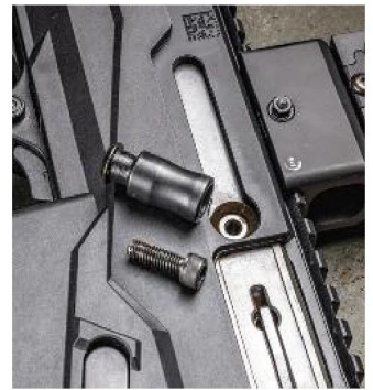
The charging handle is easily removed and can be repositioned to either side. The barrel is also suppressor ready.
