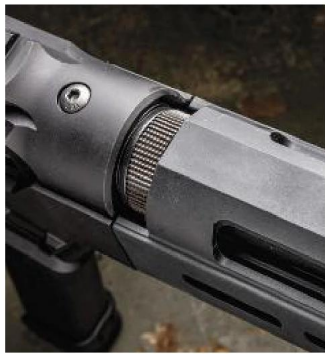
A knurled nut sets the proper distance between the barrel's breech face and the lug abutments in the receiver.
