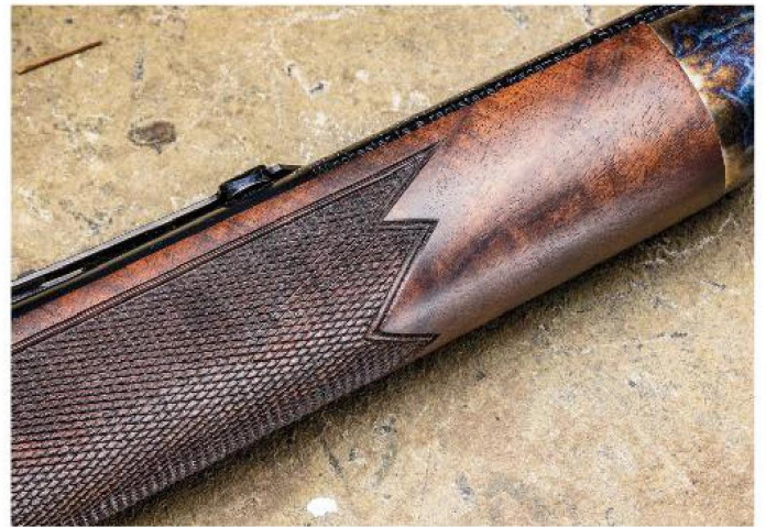
Though laser cut, the 18 lines-per-inch diamond checkering is both classic and functionally tactile.
