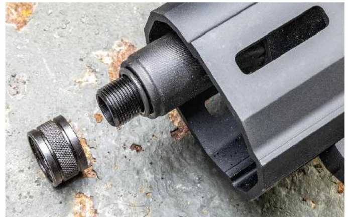
The charging handle is easily removed and can be repositioned to either side. The barrel is also suppressor ready.
