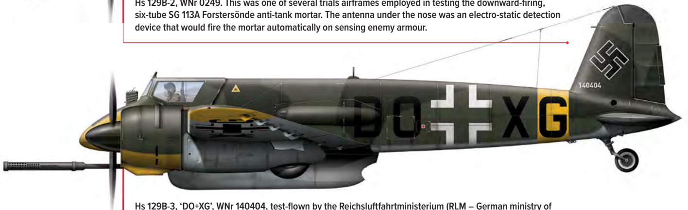
Hs 129B-3, 'DO+XG', WNr 140404, test-flown by the Reichsluftfahrtministerium (RLM – German ministry of aviation) to employ the BK 7,5 cannon. The aircraft was eventually fitted with an enlarged rudder.
