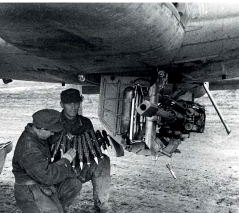
LEFT The muzzle break of the MK 103 30mm cannon was rectangular, compared with the circular muzzle of the Mk 101. This MK 103 has been swung down from the lower fuselage of an Hs 129B-2 of 10.(Pz)/SG 9 on the Eastern Front, for re-arming.
