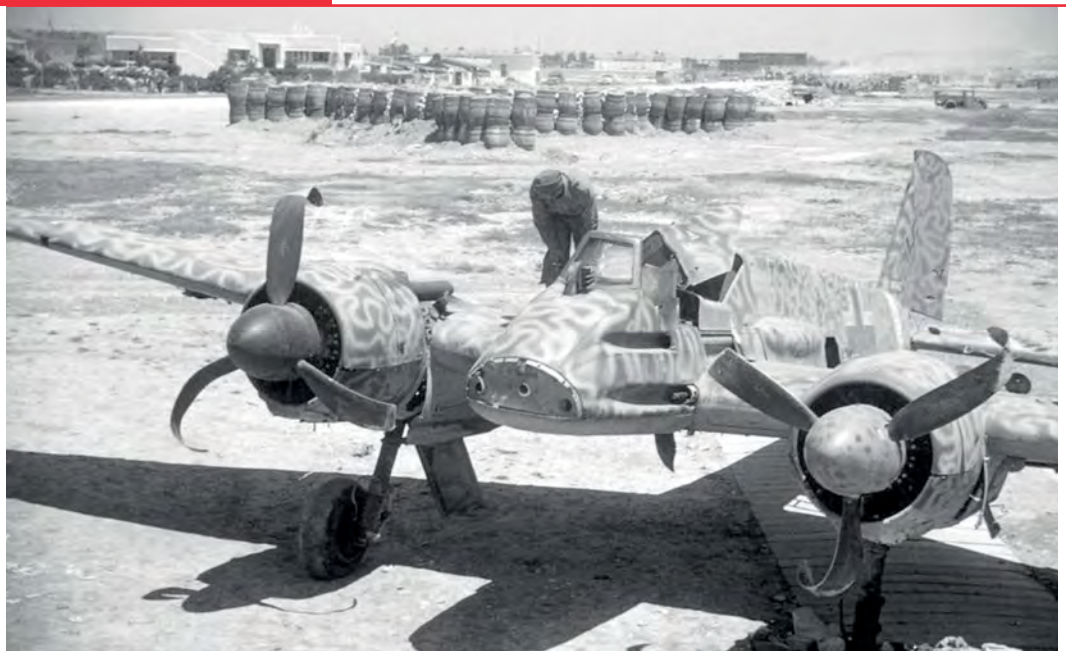
The extraordinary cockpit area of the Hs 129A-series aircraft, with the small, heavily armoured vision panels including the V-shaped windscreen, which proved totally inadequate. The external structure ahead of the cockpit was intended to house the weapons sight.
