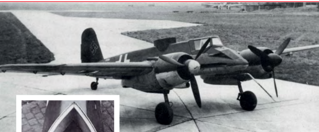
LEFT Among the many types of weaponry trialled on the Hs 129 was the curious Rheinmetall-Borsig SG 113A Förstersonde downwards-firing anti-tank mortar system. This Hs 129B-0 was one of several that tested the weapon, the mortars being mounted mid-fuselage.
