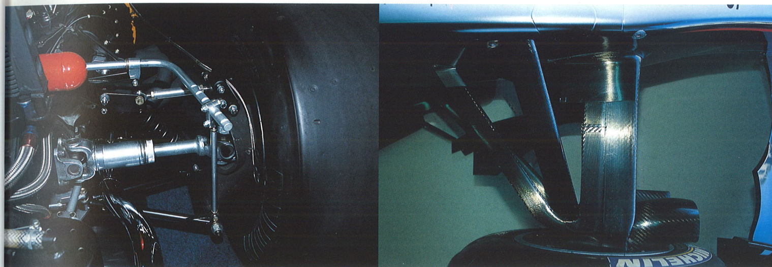
The McLaren M7 used its engine as a 'stressed member' (above) meaning that it worked as part of the chassis. The suspension (below) used a simple, effective wishbone layout
