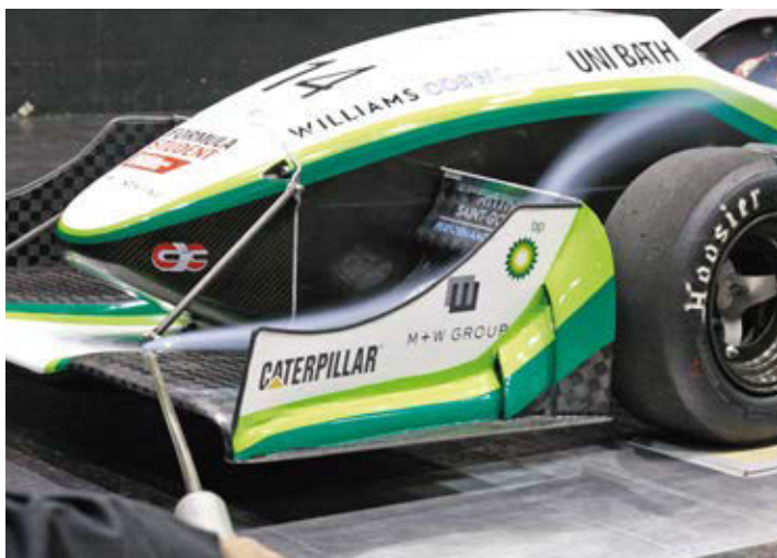
Figure 7: The front wing deflected air over the top of the tyres
