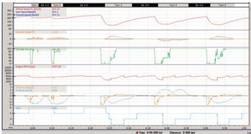
Figure 4: A plot of Speed, Throttle and RPM for a lap
