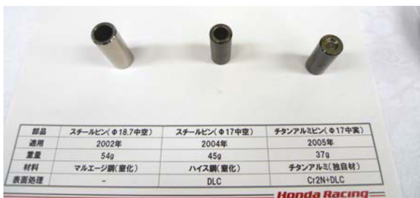
Increasingly lightweight piston pins could survive F1 conditions with the addition of DLC coatings
