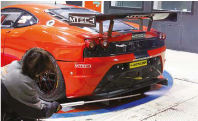
Figure 10: The Ferrari F430's diffuser showed 'clean' flow emerging from its centre...
