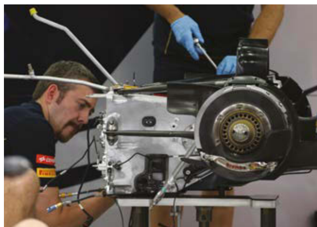
Toro Rosso gearbox shares internals with other Renault F1 cars, but features a unique aluminium casing. Other teams have opted for all carbon designs
