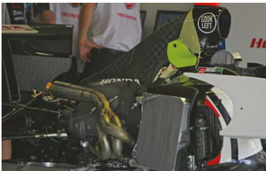
Honda's engineers experimented extensively with exhaust system design and pulse tuning
