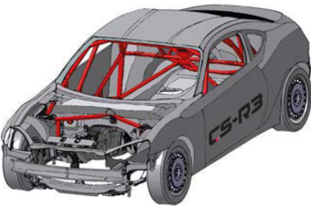
TMG's welded-in rollcage and stiffening structures for the rear-wheel-drive GT86 CS-R3 are shown in red
