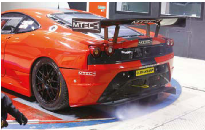
Figure 11: ... but disturbed, and even reversed, flow aft of the outer sections
