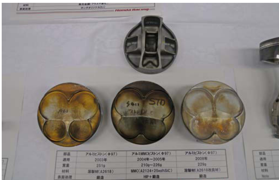
Weight of the reciprocating assembly was progressively reduced to achieve 20,000rpm+ reliability
