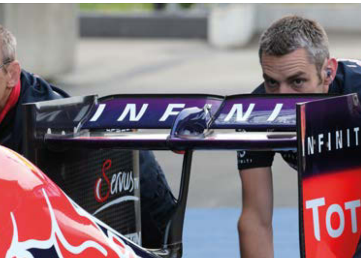
Rear wing set almost flat, Red Bull found some speed at the expense of downforce...
