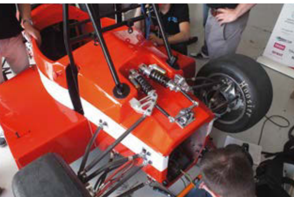
Pushrod suspensions transfer the same forces as other designs. The important thing is balancing the car's response to them
