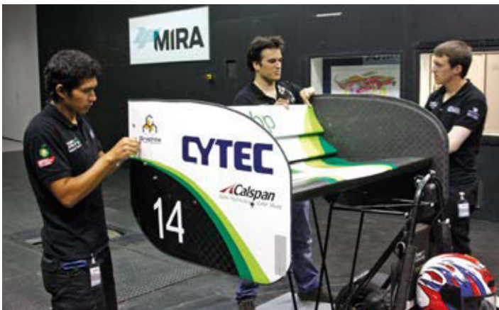
Figure 3: Rear wing was a conventional large chord triple-element design
