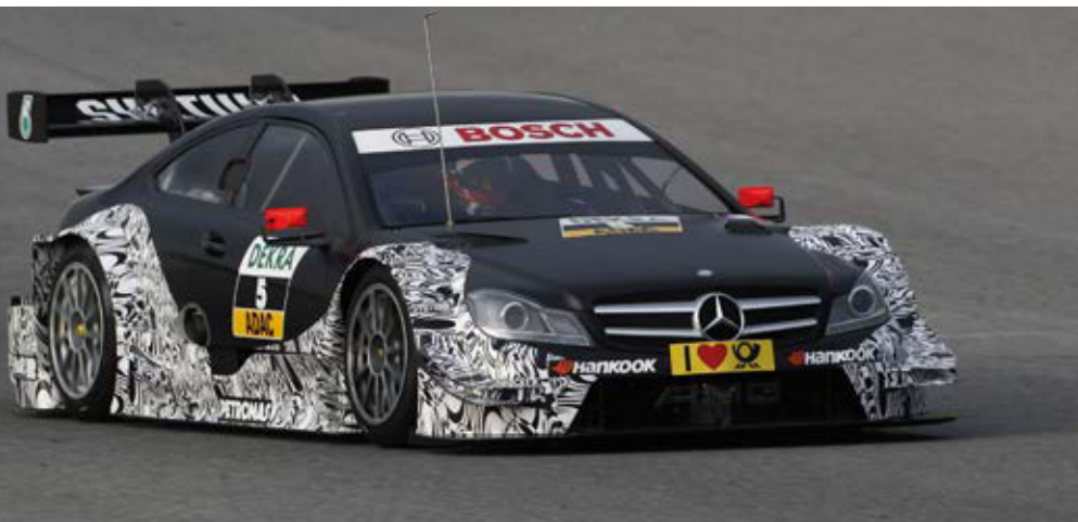
Mercedes livery in testing serves to indicate the body areas of the cars that are allowed to deviate from the base car template. Dazzle camouflage may be to deter eyeball analysis of aero elements by opposition
