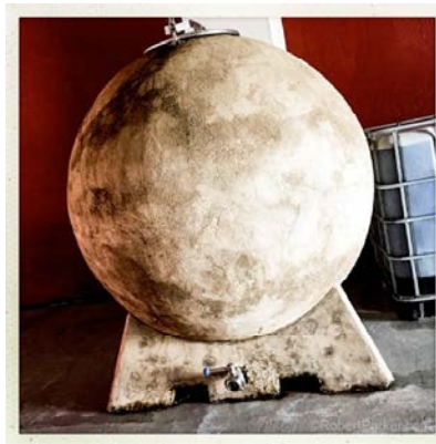
I saw some experimentation with the shape of concrete vats, like these spherical ones. Beyond the egg...
