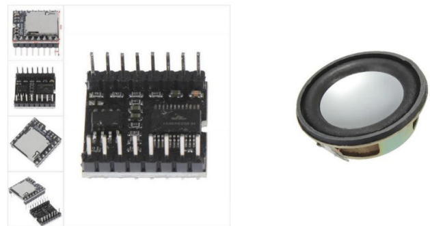
Figure 5. DFPlayer Mini MP3 Player and 5Ohm speaker
