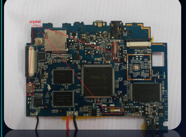
A crystal oscillator is an electronic oscillator circuit that uses the mechanical resonance of a vibrating crystal of piezoelectric material to create an electrical signal with a precise frequency. This frequency is commonly used to keep track of time, as in quartz wristwatches, to provide a stable clock signal for digital integrated circuits, and to stabilize frequencies for radio transmitters and receivers
