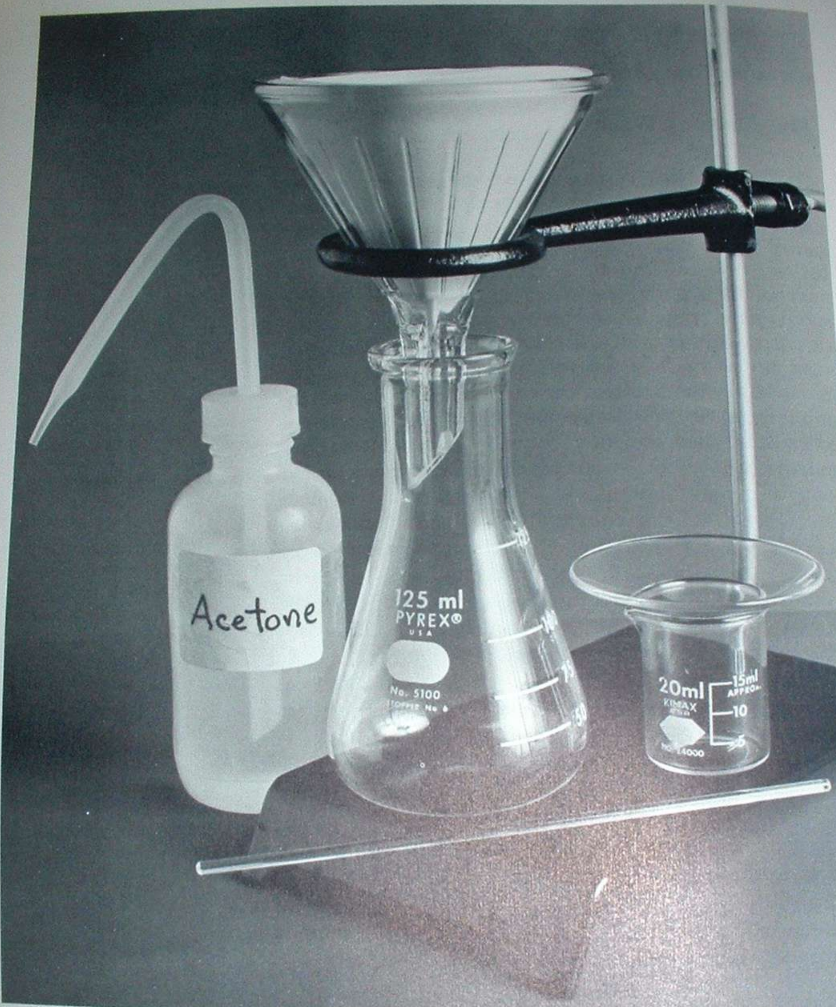
96. The equipment used for the acetone wash includes: acetone in a plastic wash bottle, a 125ml Erlenmeyer flask, a ribbed funnel with a medium-speed filter paper, a 20ml beaker with a watch-glass cover, a glass stirring rod, a lab stand.
