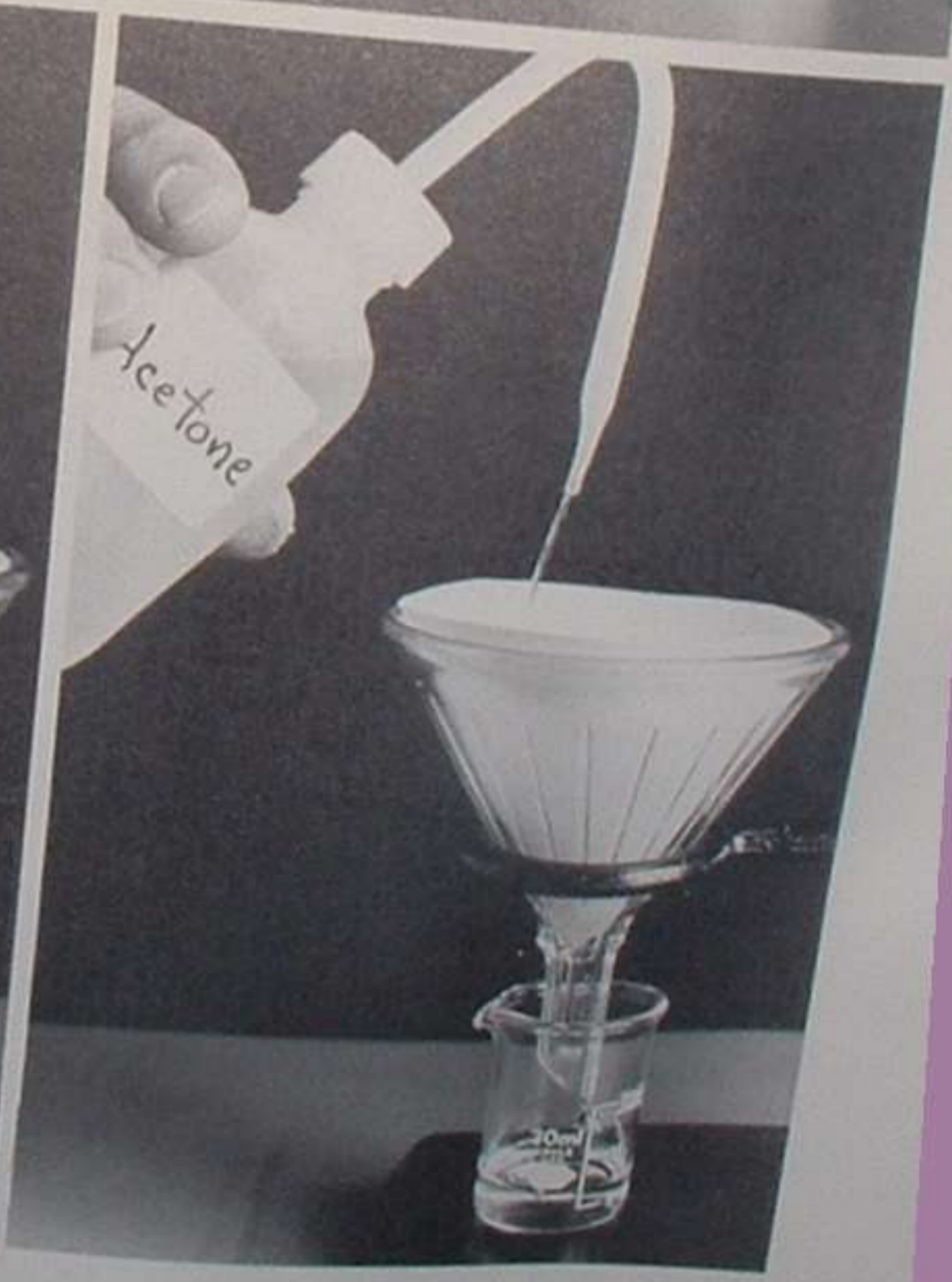
bottom: 113. The acetone is stirred until the base is dissolved. 114. The liquid is filtered to obtain a clear solution. 115. The filter is rinsed to minimize any loss of the base and to increase the total volume of the solution to 15-20ml.
