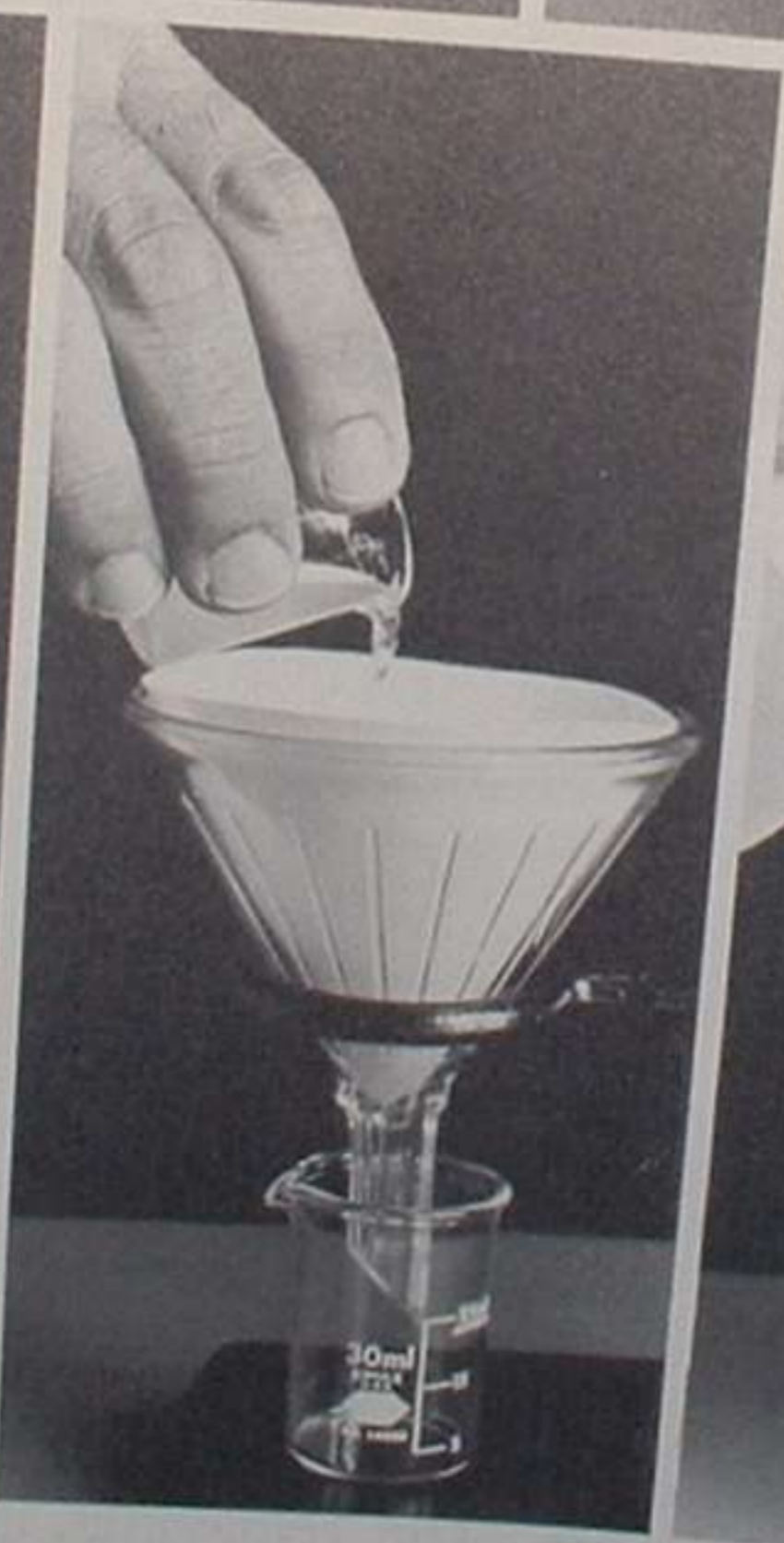
bottom: 113. The acetone is stirred until the base is dissolved. 114. The liquid is filtered to obtain a clear solution. 115. The filter is rinsed to minimize any loss of the base and to increase the total volume of the solution to 15-20ml.
