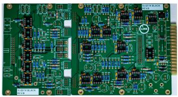
After that Step solder all Wima Capacitors and Board Connectors like on the pictures. On the Small Board, the short pins are soldered as close as possible to the board. Its important that you press them flush in place during soldering. We need them to sit flush and straight for the mechanical assembly later.
