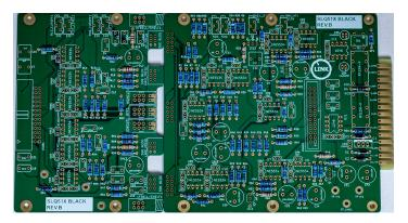
After Placing and Soldering all Resistors, we solder the next bigger parts like IC-Sockets and small Capacitors, like 37x100nF and 16x22pF
