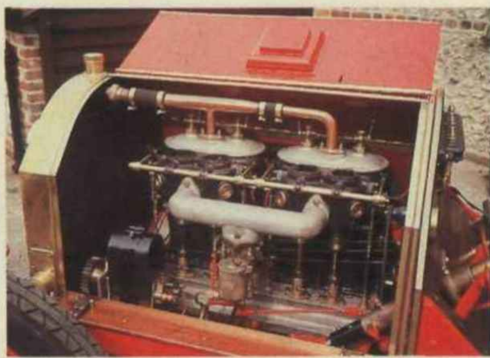
The four-cylinder motor has paired blocks; the igniter push-rods are plainly visible. Bottom left, the man-sized pump keeps fuel pressure up. Tachometer, air-pressure gauge and a battery of drip-feeds stock the dash, bottom right.
