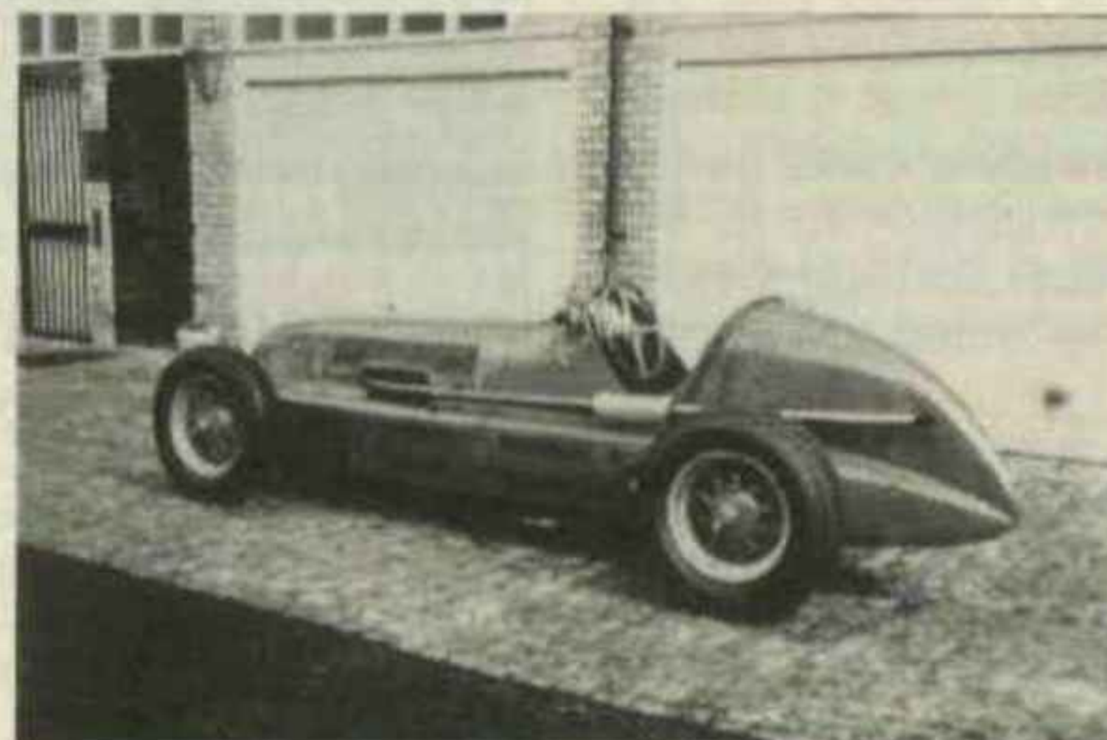
1938 MASERATI 4CM. 1 1/2 litre, twin supercharged 16 valve 4 cylinder Grand Prix car. Chassis and engine to 4CL specification. Fully race prepared, FIA papers and VSCC blue form.
