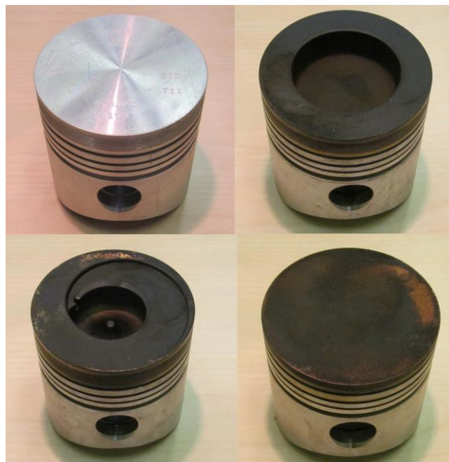
Figure 1. Chamber Geometries: a) Rough piston (top left), b) Heron type geometry (top right), c) MR type geometry (bottom left) and d) Disc type geometry (bottom right)
