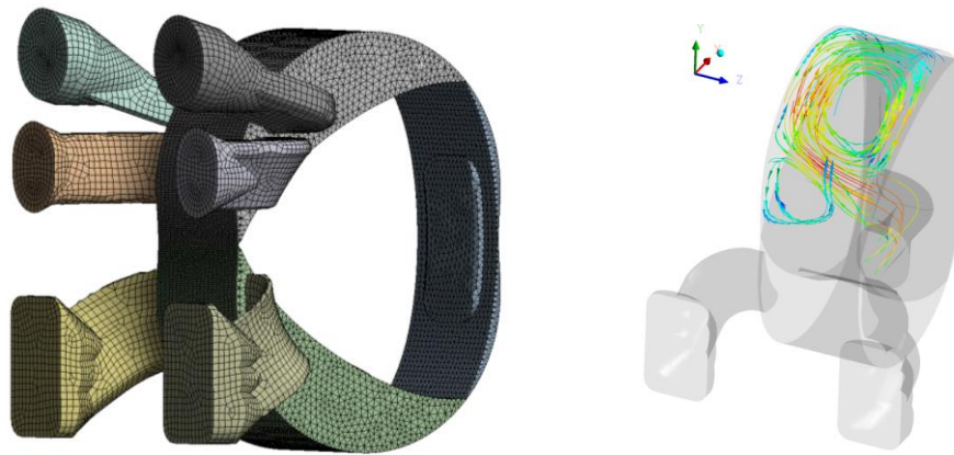
Figure 1. Numerical model of the single rotor 13B- Renesis engine (right side), air motion during intake from single side port (left side)
