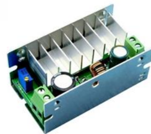
Figure 8. K101 200W adjustable dc-dc voltage regulator card [13]
