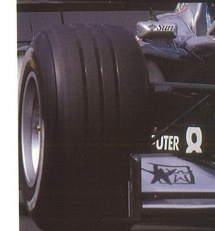
The Bridgestone front (above) was wider than the Goodyear (top), and had been expected to confer an advantage. On the day, Goodyear dominated
