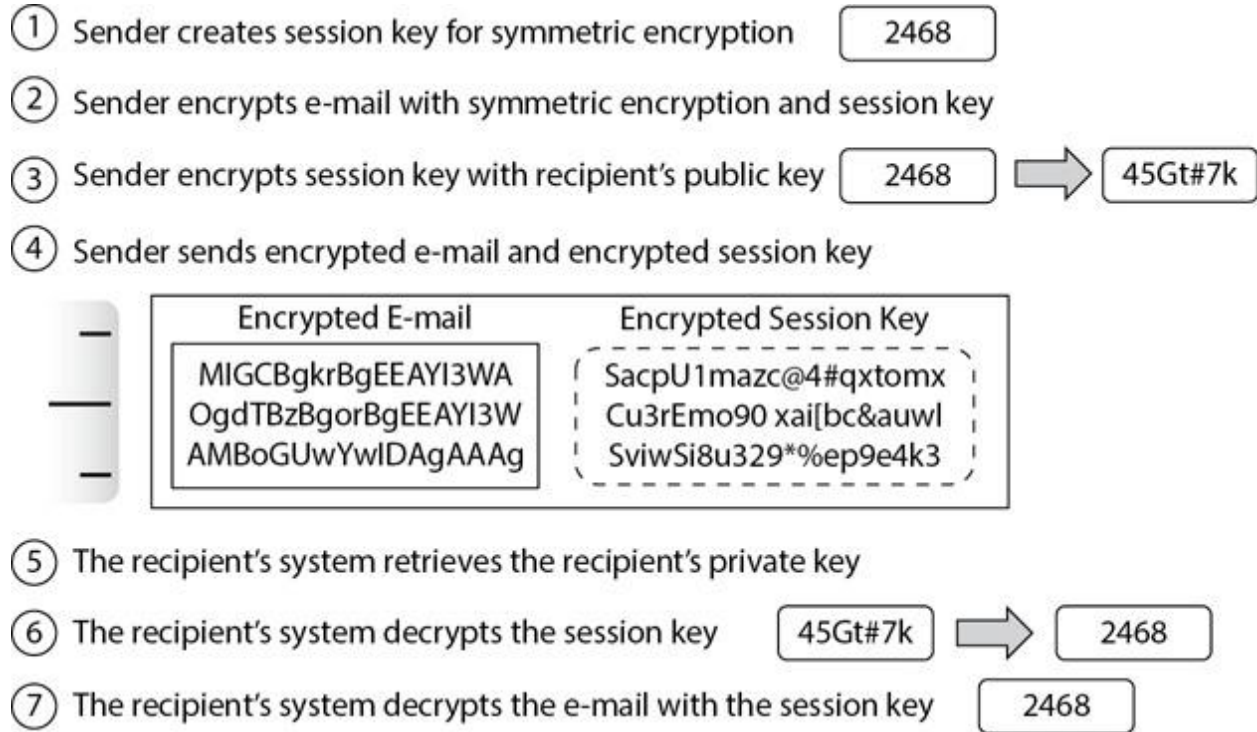
Figure 14-10 Encrypting an e-mail with symmetric and asymmetric encryption
