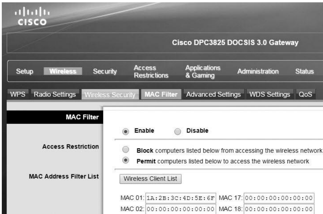
Figure 3-18 Enabling a MAC address filter
