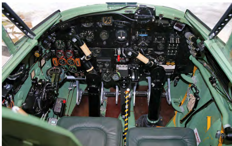
RIGHT: The completed cockpit, showing well the TIII's seating arrangement and dual controls.
