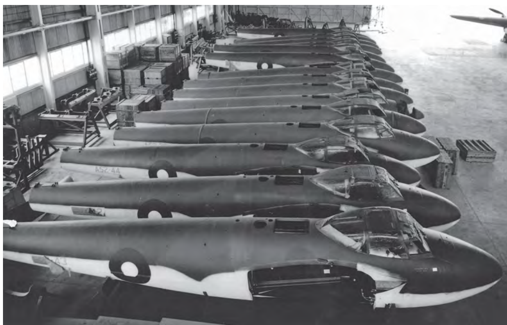
TOP: The fuselage production plant, on the upper floor of a disused mill building in a Sydney suburb, was somewhat primitive. VIA HARS
