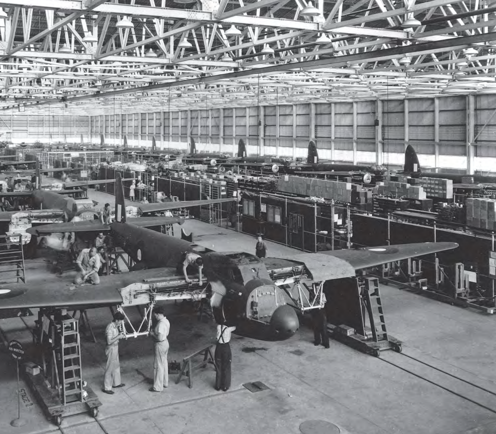
ABOVE: Bankstown's final assembly facility, with wings produced by General Motors Holden being mated to fuselages.
