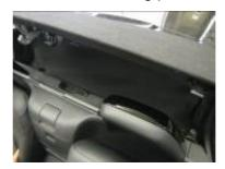
2). Install the resin edge of the tension cloth into the J-hook.
