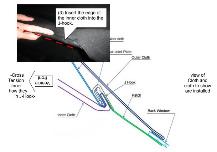
4). Lightly pull the inner cloth and verify that the inner cloth does not come off easily.
