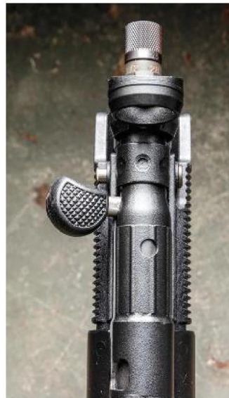
Pull the handle and lift to lock the bolt to the rear. The bolt handle can be slapped to send the bolt forward into battery.
