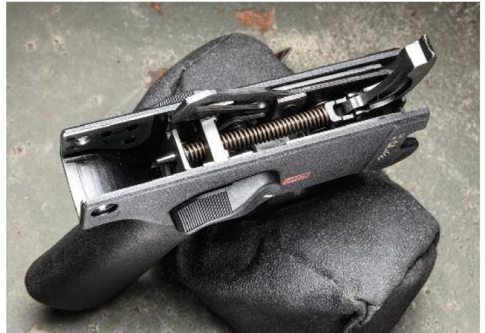
Inside the trigger housing is a 9mm semiautomatic-only trigger pack that cannot be converted to automatic or burst modes.
