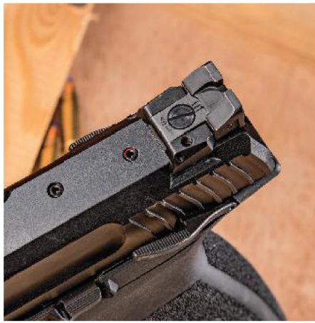
The rear sight is adjustable for windage and elevation, but it requires a thin-bladed flat-head screwdriver tip.
