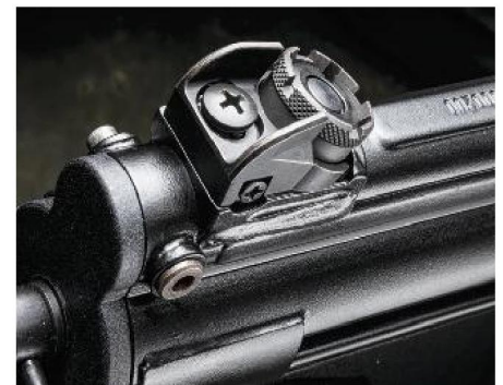
The adjustable rear drum sight features four progressively wider notches. Sights were zeroed in a machine rest at 25 meters. One-quarter turn equals .55 inch at 25m.
