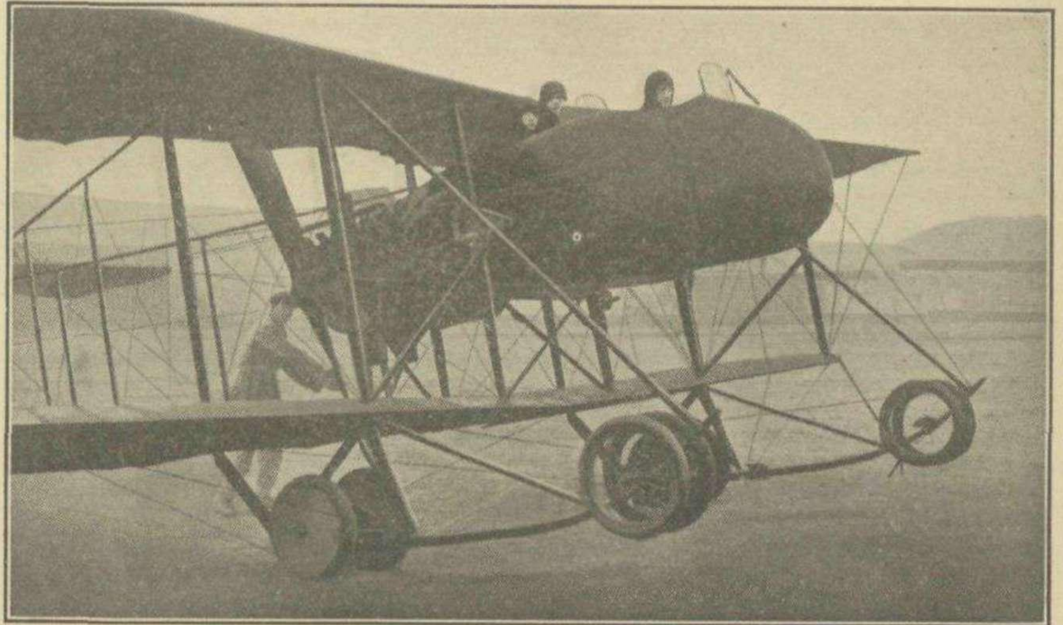
A "flying birdcage" which was the precursor of present day twin engine machines, the Farman F.40 of 1913.
