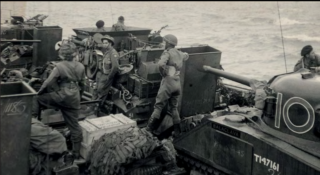
LEFT: British Shermans, and a Sherman ARV (carrying two BSA motorbikes), all with wading gear, wait in their LCT (Landing Craft, Tank) ahead of their landing on Normandy's beaches. (HMP)
