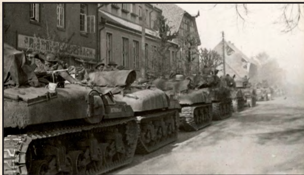
ABOVE: Ram Kangaroo personnel carriers of 4th Armoured Brigade in Rethem, 16 April 1945. The Kangaroo was one suggestion made by O'Connor and others, such as the Canadian Guy Simmonds, to give infantry protected mobility when supporting armoured operations. They would not be used during Goodwood, but were a common feature of subsequent operations. (HMP)
