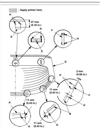
Attach the fasteners (A) to the tailgate as shown.
