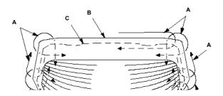
rear window. Clean the inside face and the edge of the rear window with alcohol where new adhesive is to be applied. Make sure the bonding surface is kept free of water, oil and grease.
