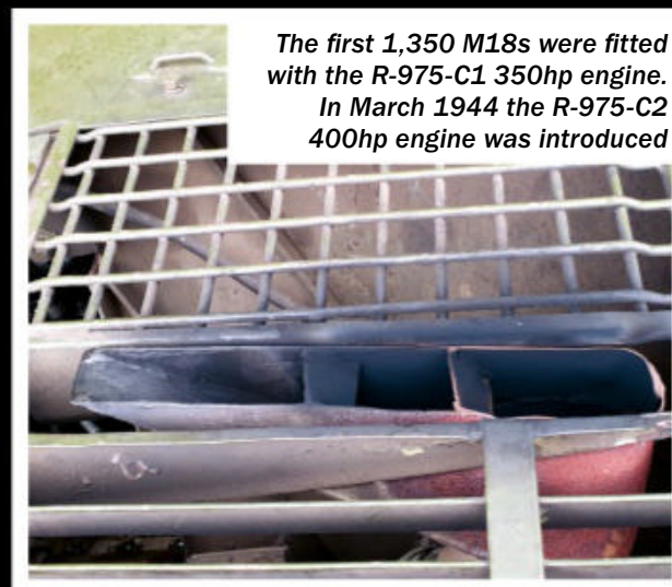
The exhaust pointed vertical out of the engine deck to reduce the amount of dust produced by the M18
