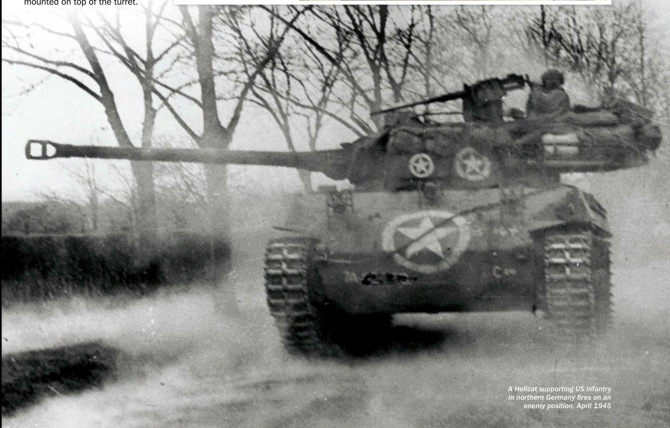
On the left of the main gun was the gun sight. A canvas dust cover protected the mantlet and gun
