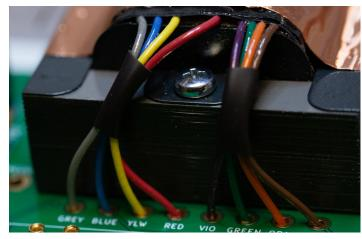
Place the Input Transformer with a gap between PCB and transformer. You can use a space or just solder one pin and later the other pins.
