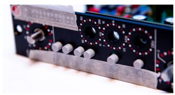
Now we will cut the LEDs legs. Make sure you have the right leg for + and - (Long leg is + and short leg is -). I usually don't cut them straigt and keep two different size legs, so you still know which leg is + and which is -. For the Mainboard we need LEDs with long leg measured cut to 8-10mm (5/16 to 6/16)
