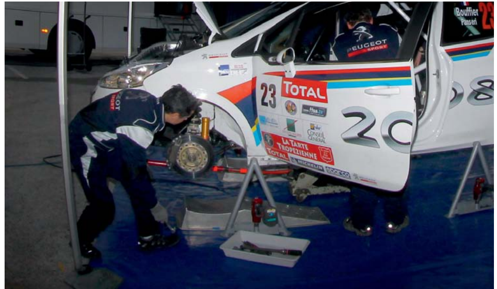
A Peugeot 208 Group R rally car, an example of a vehicle which features strut suspension
