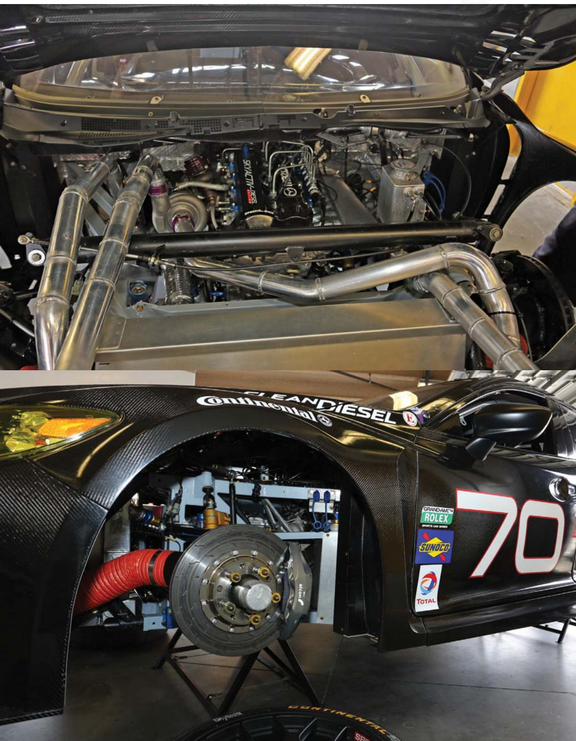
The engine was the real key to the car's development, and indeed is the reason the car even exists (top). A new Alcon brake package was fitted to the car further reducing weight (above)
