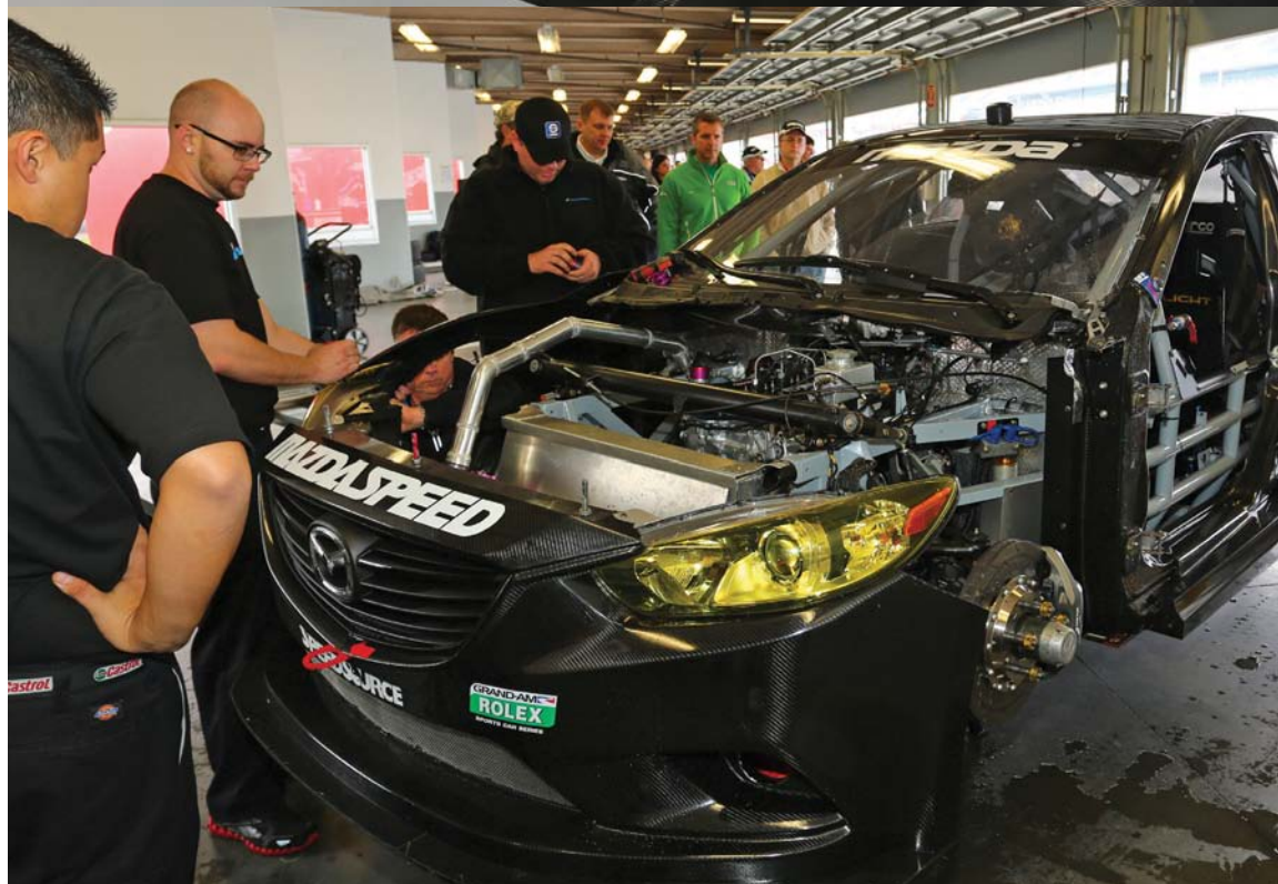
The tubular steel chassis of the '6' is essentially the same as the Riley MK XXIV Mazda RX8 which won its class in the Rolex 24 in 2010. The first of the new cars was built 22kg underweight with later versions even lighter, partially due to a lightweight composite body. Note the NASCAR style door bars
