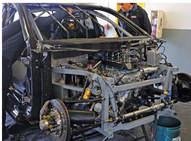
The turbo diesel engine replaces the RX8's triple rotor, a first for Grand-Am. The drivers shift through the EMCO gearbox at just 5,000rpm.
