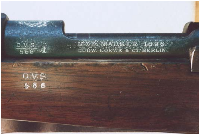
Side rail and receiver markings of the Ludwig Loewe & Co. Model 1896 Mauser Rifle.
