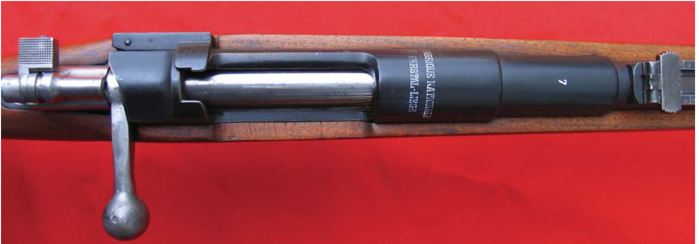
The top of the action of the Model 1889 Heavy Barrel Rifle made by FN, showing the serial number and the rifle's black enamel paint finish. (John Wall collection)
