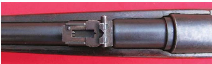
A top view of the receiver and barrel of the Spanish Model 1892 Navy Test Carbine shows a receiver ring without an identifying crest, and a rear sight leaf without range numbers. (John Wall collection)
