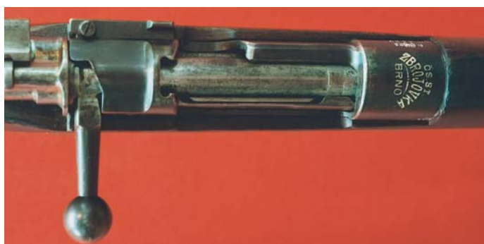
Full view of the action of the Czech Model 98/22 Rifle as used by Turkey. Note the arched Czech receiver ring marking.
