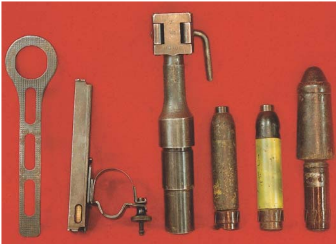
Grenade launcher and equipment used by the Germans with German Model 98k Carbine. From left to right: the launcher wrench, used to tighten or loosen the removable barrel; the inclinometer that attaches to the rifle to provide the proper level; two different style high explosive rifle grenades; lastly, an armor-piercing, shaped charge rifle grenade. (Henry Wichmann collection)
