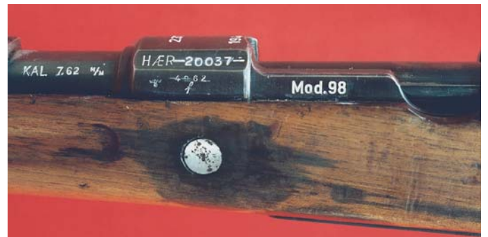
Stampings on the side of the barrel, receiver ring, and side rail of the Norwegian Reissue Model K98k Carbine. (Bob Bennett collection)
