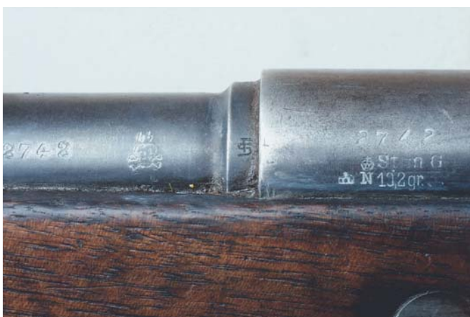
Barrel and receiver markings on a German Model 98k Carbine, showing an SS "Death's Head" on the barrel, indicating issuance to an SS unit. Note that the left side of the receiver ring bears commercial nitro proofs under the serial number. (Century International Arms, Inc.)
