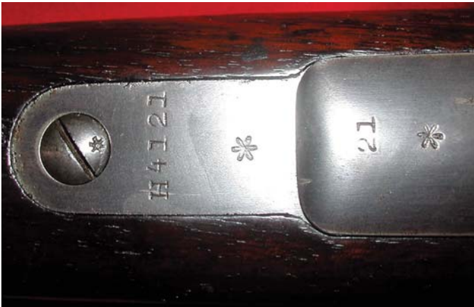
The trigger guard assemblies of original-condition German-made Spanish Model 1893 Mauser Rifles are fully serial numbered on the trigger guard tip, but have just the last two digits on the floor plate. Each screw is inspection stamped, but not numbered. (John Wall collection)
