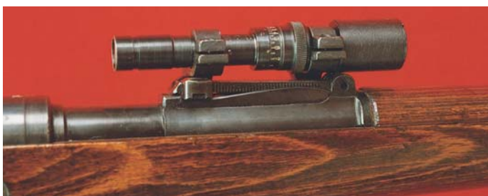
Right side view of the ZF-41 scope mounted on the German Model 98k Carbine.
