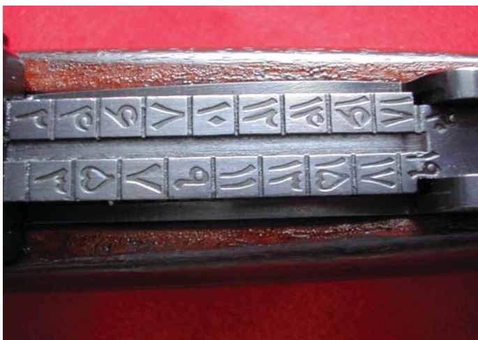
The Farsi numerals on the leaf sight of the M1924 FN Contract Rifle for Iran are graduated in 100-meter increments, from 200 to 2,000 meters. (John Wall collection)
