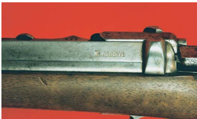
Model designation on the left receiver side rail of the German Model 71 Carbine.
