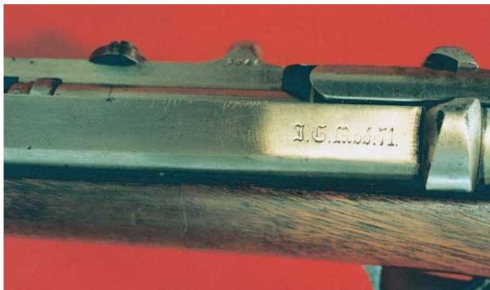
Regular G 71 markings on the left receiver side wall of the German Model 71 Short Rifle.
