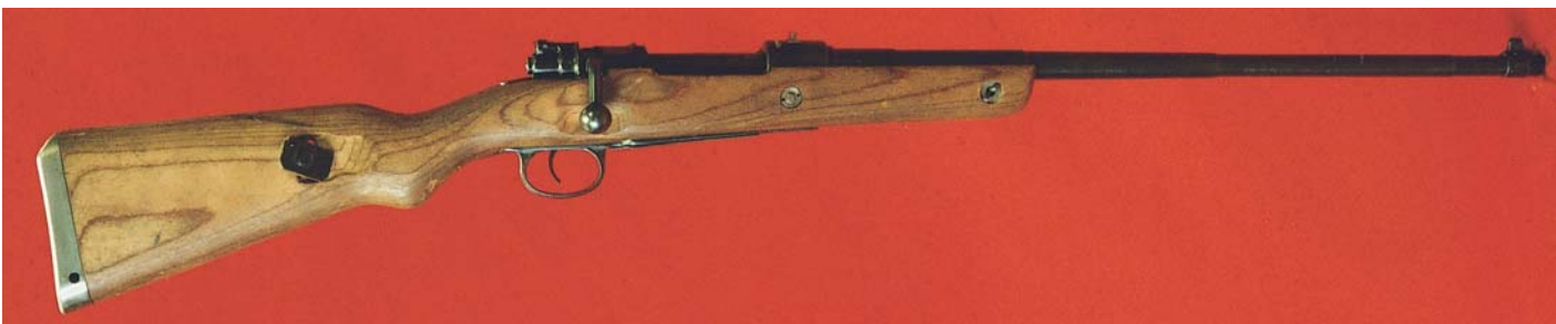
Full-length view of another German VK-98 Rifle. This rifle is fitted with a cupped buttplate with a hole in the side for bolt disassembly, a K98k barrel, a magazine floorplate, and provision for a sling.
