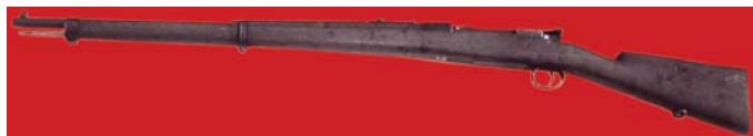
M1893 Spanish Mauser made by FN, serial number C6041. Several possible FN-made M1893 Spanish Mausers have surfaced in the none, A and C serial-number series, but all are unmarked except for FN address on ring. This example has a Spanish "R" (rebuild?) stamp on the left buttstock (matching), and the stock and handguard are also matched in pencil in the barrel channel, which is an Oviedo (Spanish Arsenal) practice. (Jack Carnahan collection)
