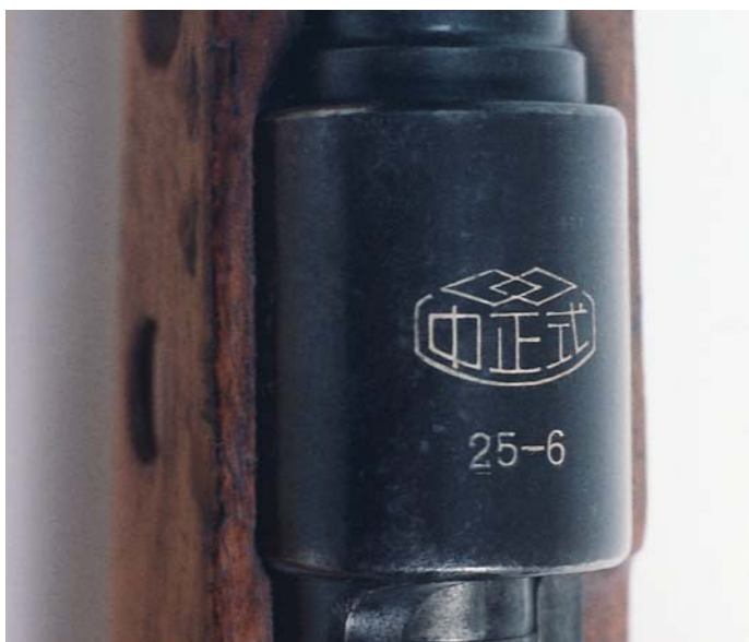
View of the Chinese markings on the receiver ring of the "Chiang kai-Shek" Model Short Rifle.
