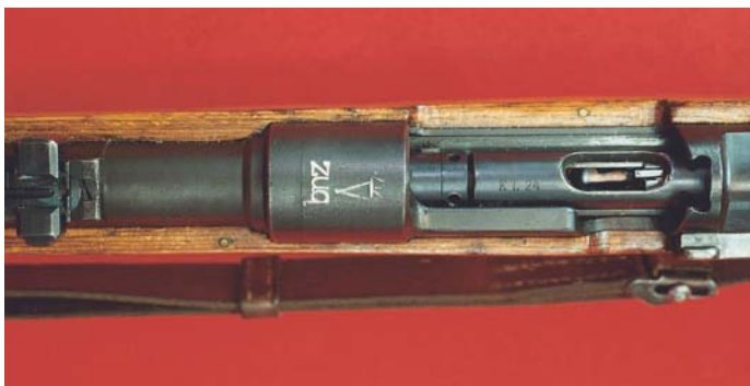
The action of the German Model 98k Carbine with the ERMA Model EL .22 caliber insert. Note the collar with holes for locking the insert into place with the aid of a short rod. Note also the port for ejection of the spent cartridge casing.
