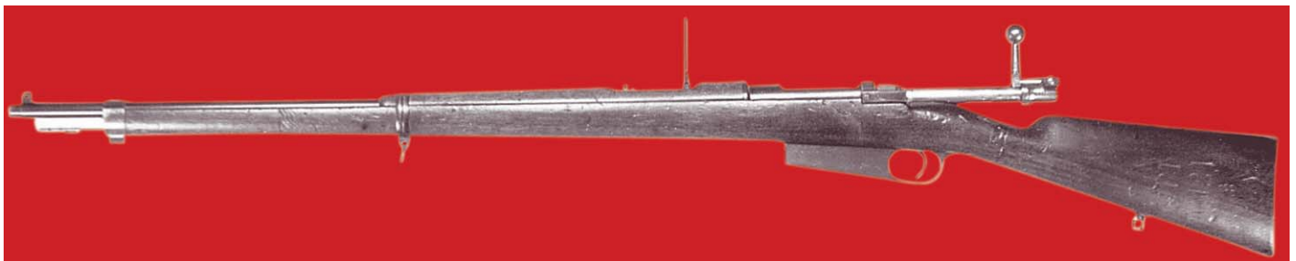
Left side view of the Model 1892-93 Experimental Rifle, with the bolt in the open position, and the rear sight extended. (John Wall collection)
