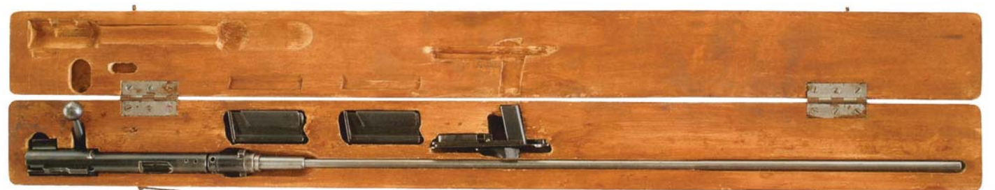
Pre-war .22 LR caliber conversion kit, manufactured by ERMA and used as a training tool with Mauser rifles. Marked ERMA, Erfurt, 1937. (Rock Island Auction Co.)
