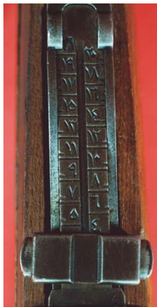
Turkish numerals on the rear sight of the Czech Model 98/22 Rifle in Turkish service.
