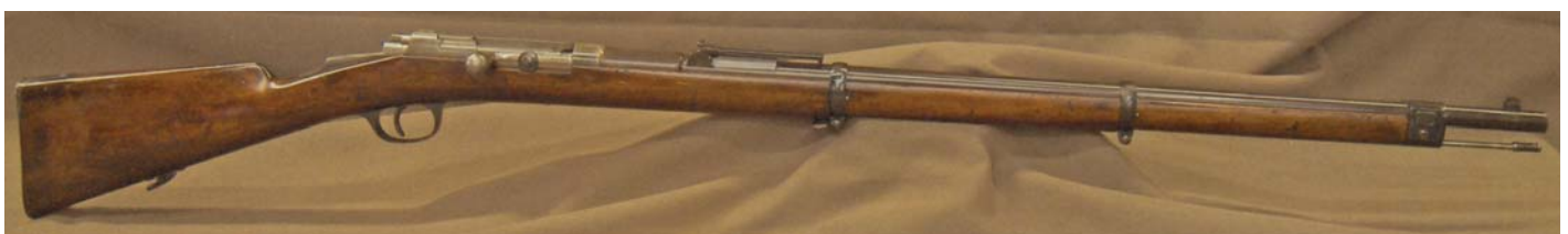
Model 78/80 manufactured pattern rifle for Serbian contract 10.15mm. Note third barrel band. (Private collection of Robert I. Landies)
