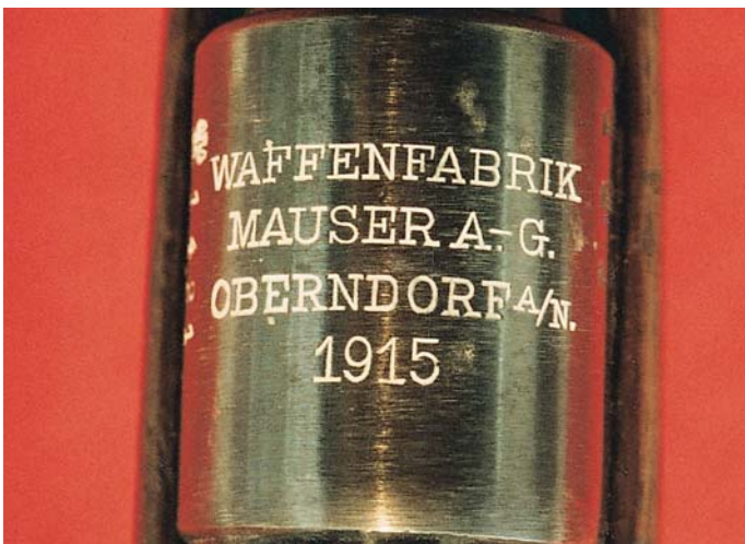
Receiver ring of the Danish Military Target Rifle made with a Model G 98 action, showing the original German markings.
