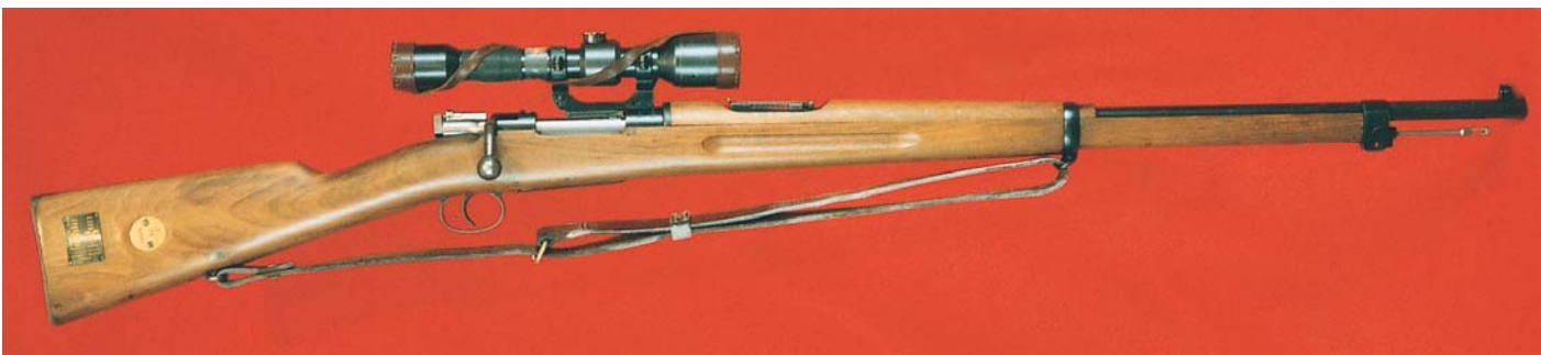
Full-length view of the Swedish Model 1896 Sniper Rifle fitted with the Model 41 AGA scope. Note the bent bolt for clearance.
