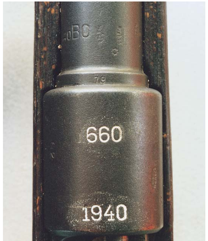
The receiver ring of the German Model 29/40 Rifle, showing the "660" code for the Steyr-Daimler-Puch factory over the date "1940."
