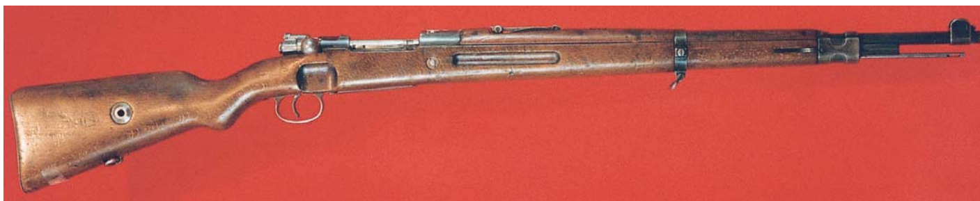
Full-length view of the Polish Model Wz 29 Training Short Rifle in .22 caliber. In all other respects, this is identical to the standard short rifle.
