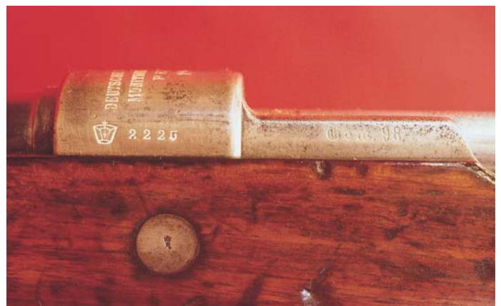
The left side of a naval issue G 98 Rifle, showing the naval acceptance mark on the side of the receiver.
