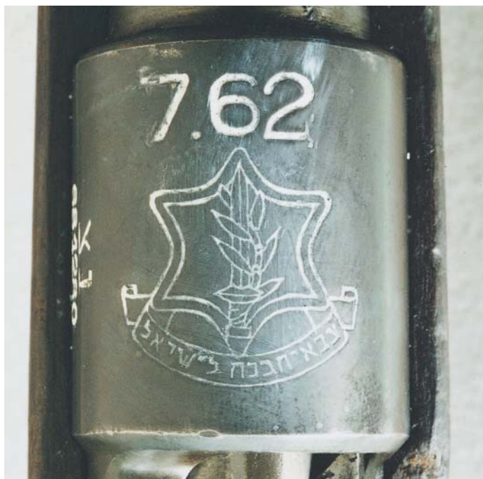
The Israeli crest and the caliber designation on the receiver ring of the Israeli Model 98k Short Rifle. FN proof marks are on the left side of the receiver ring.
