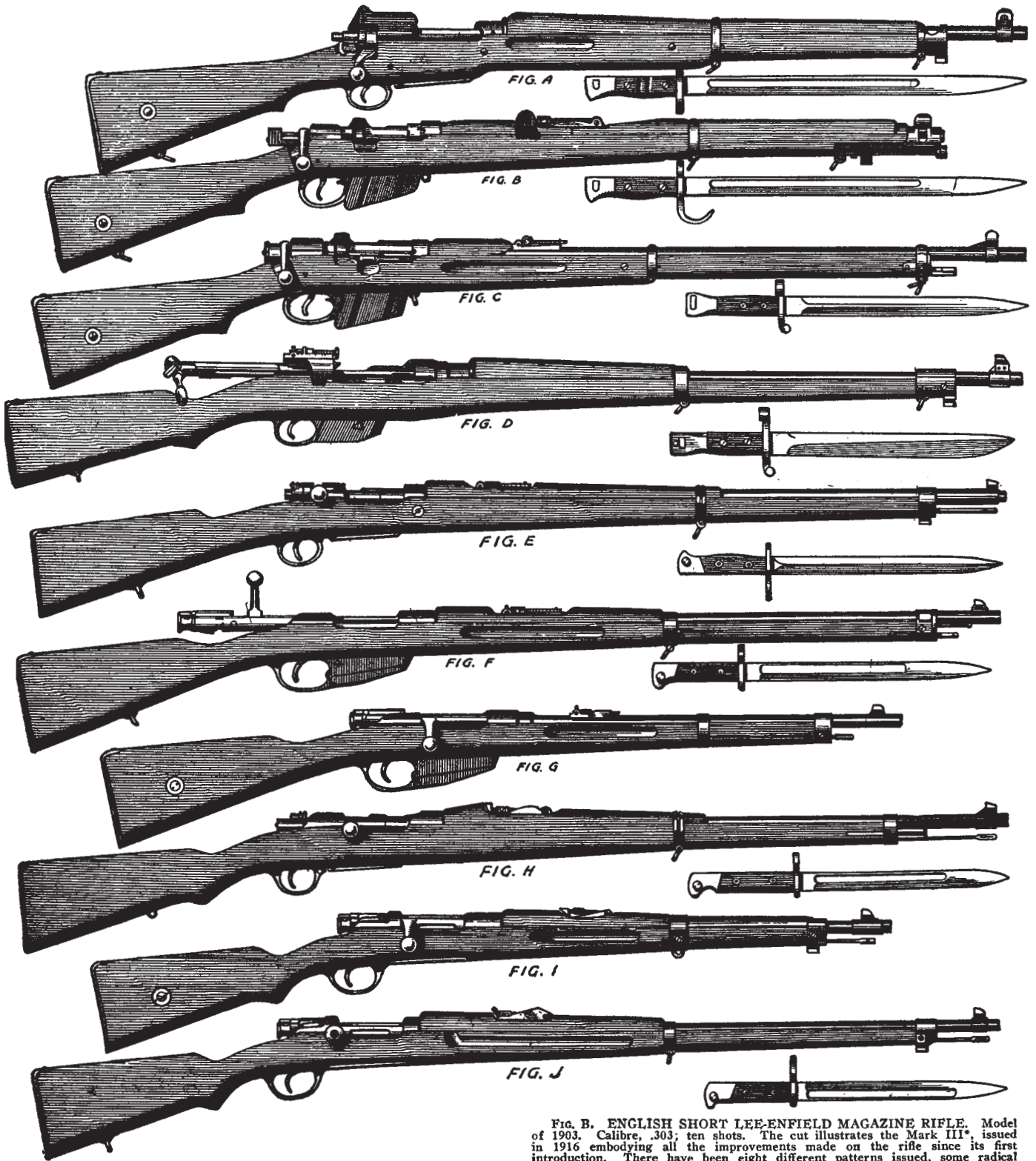
FIG. A. ENGLISH ENFIELD MAGAZINE RIFLE. Pattern 1914. Calibre, .303; five shots. The British government was experimenting with this rifle when the war broke out, it was however to be of a smaller calibre, i. e. .27. Thousands were made in this country for England in the early part of the War and as is well known, the U. S. adopted it in view of the fact that so many armories could produce it while but one could make the Springfield. This model differs from the U. S. in that it has a long range sight on the left side and the calibre being .303 instead of .30. Bayonets for both countries are the same. It will be noticed that there are 2 ribs cut into the wooden grips of the bayonet, this was done as a means of distinguishing this model from the model that fitted the 1903 short Lee-Enfield, the bayonets were very similar in looks. The rear sight being placed directly over the receiver and near the eye of the soldier is a new idea. The Ross of Canada, Mark III copied it. (See Fig. D.) In all the photographs of war scenes, the writer has never seen one of these rifles in the hands of an English "Tommy."
