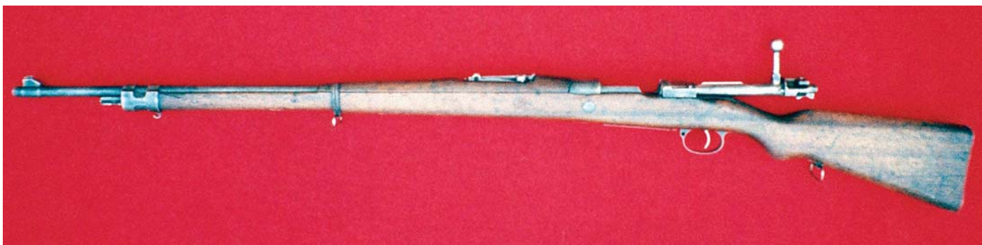
Left side view of the Austrian Model 1914 Mauser Rifle with the bolt in the fully open position. (John Sheehan collection)
