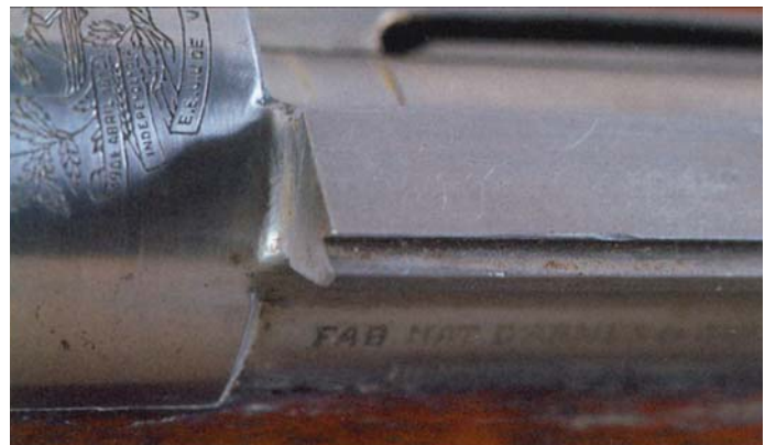
Left side view of the integral dovetailed scope base on the Experimental FN 24/30 Sniper Rifle. (Rock Island Auction Co.)
