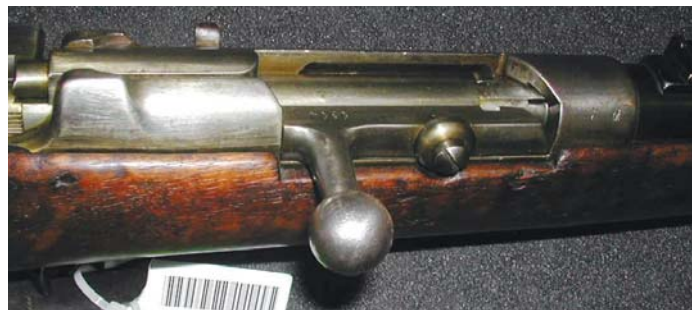
The right side of the action of the Serbia Model 1884 Artillery Carbine, which along with the Serbian M1884 cavalry carbine, is the only Oberndorf-made carbine version of the Model 1871/84 action. (From the former Pattern Room Collection now in the Royal Armouries Museum, Leeds, England)
