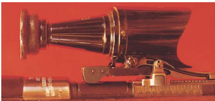
Right side view of the low light bifocal marksman scope mounted on the "Lange Vizier" rear sight. Note how the base of the scope conforms to the curvature of the rear sight ramp, while the spring-loaded mounting arms lock into the recessed bottom portion of the rear sight ramp. The eyepiece is molded leather.
