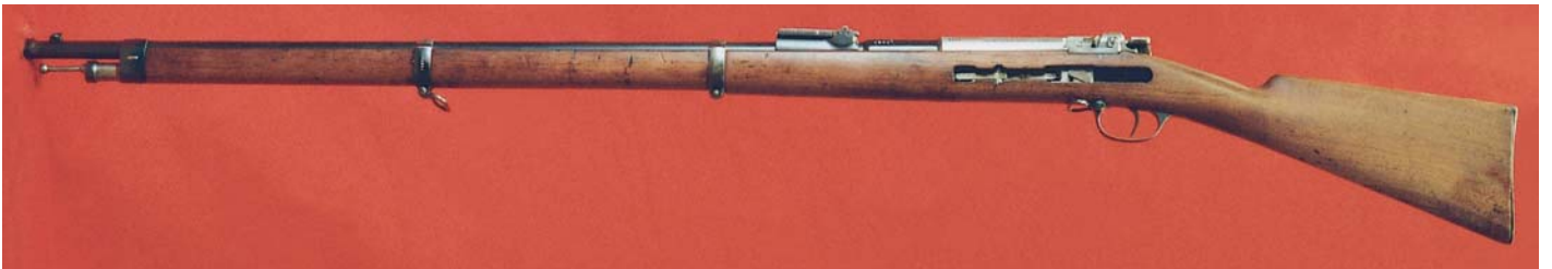
Left full-length view of the G 71/84 Cutaway Rifle, showing the cuts in the action area of the rifle.
