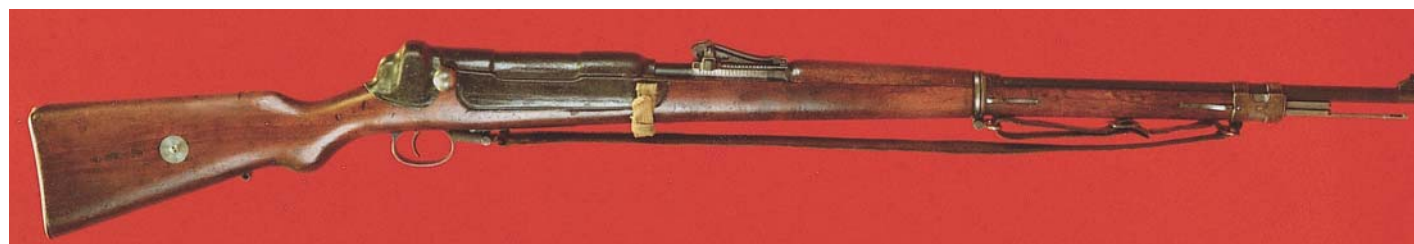
Right side view of a German Model G 98 Rifle with a most unusual pressed steel action cover, held in place by a buckle and strap arrangement at the front of the cover.
