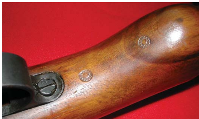
Inspection cartouches on the stock wrist area of an unissued Chinese contract Kar98k Service Rifle. Notice that, just as on Wehrmacht rifles of this era, the action screws are also numbered to the rifle. (John Wall collection)
