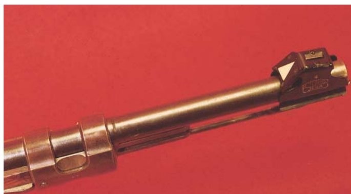
Close-up view of the auxiliary front sight used in conjunction with the low light bifocal marksman scope. This auxiliary sight with white diamond aiming point fits over the regular front sight and appears in the sight picture in the lower portion of the bifocal sight, with the target aligned with the top point of the triangle.
