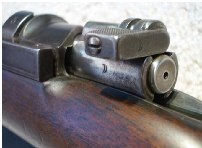
The bolt sleeve of the Spanish Model 1891 Cavalry Carbine dated "1894," showing the Turkish crescent inspection marks on the bolt sleeve and cocking piece. (Hans-Joerg Meyer collection)
