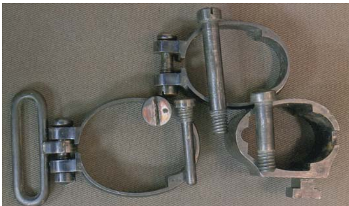
Barrel bands from the Serbian contract Model 78/80 SN 6 rifle. (Private collection of Robert I. Landies)
