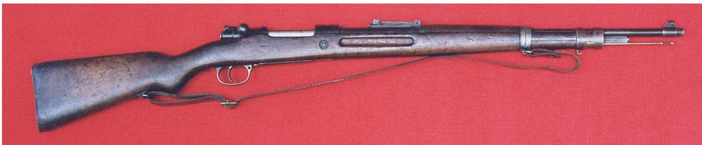
M1933 Standard Modell Short Rifle as used in Spain by the Condor Legion. This short rifle is in caliber 7.92 x 57mm.
