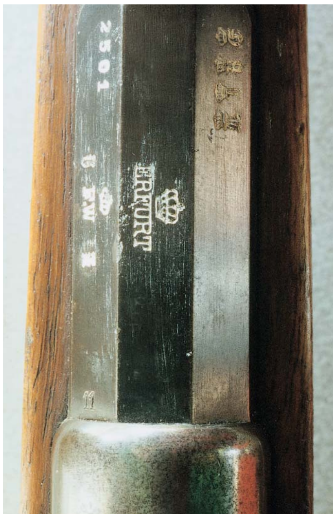
Markings on the chamber flats of the German Model 71/84 Rifle. This rifle was produced at Erfurt.
