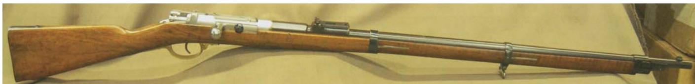
ABOVE: Mauser prototype Model 71/84 SN 14 tube magazine fed 11mm rifle. Right side full length view. (Private collection of Robert I. Landies)
