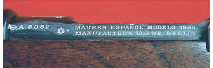
The left side rail of the Spanish Model 1893 Carbine, showing the manufacturer's markings stamped in Spanish. (Cliff Baumann collection)
