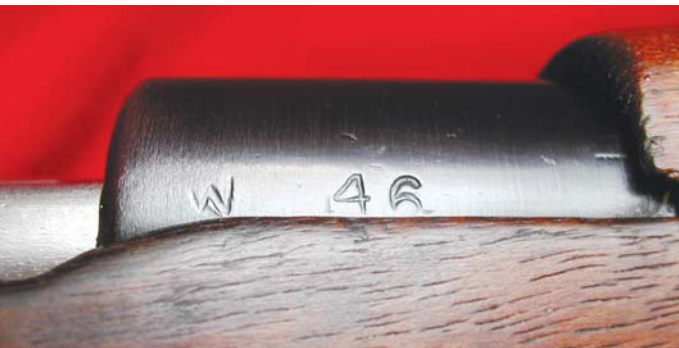
The action of the postwar Vz 23-type Yugoslav Mauser is almost totally unmarked: no receiver crest, no side rail markings, no proof mark. The sole exception is the application of a new serial number, in this case W46, to the bolt and receiver ring. (John Wall collection)
