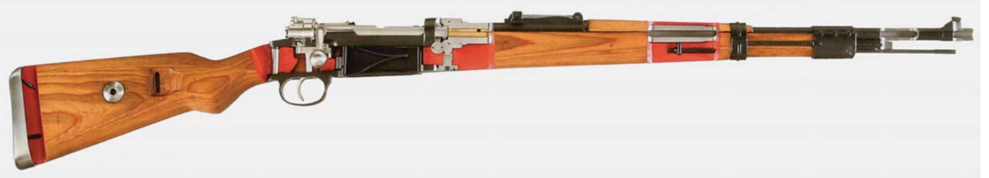
German K98k Mauser Cutaway Rifle. Right side view of a German Army training aide. (Rock Island Auction Co.)
