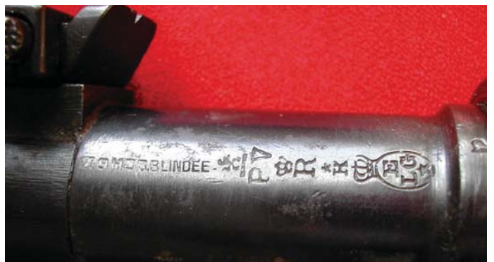
The marks of the Liege proof house found on the barrel under the handguard of the FN-made Model 1930 Short Rifle for China. The Controleur’s mark “star over-K” belongs to Walthere Delaaux, who worked at the proof house from 1929 to 1968. (John Wall collection)
