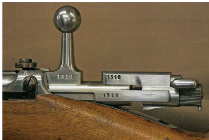
ABOVE: Left rear close-up of the 71/82 bolt showing bolt root, cocking piece and rear of extractor. (Private collection of Robert I. Landies)
