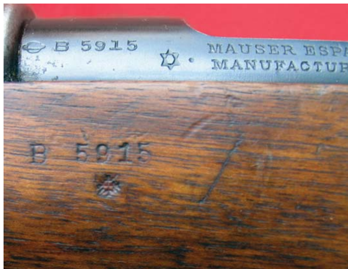
Spanish Model 1895 Carbines have the same Spanish inspection marks on the left side of the receiver as do the Spanish Model 1893 Long Rifles, even down to the curious punch mark to the right of the hexagram. Note the stock serial numbering convention directly below the receiver number on this 1896-dated Ludwig Loewe carbine. (John Wall collection)
