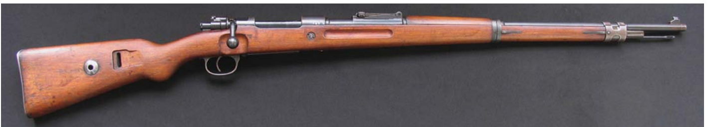
At the conclusion of WWII, a number of German service rifles were taken into service by the French Government. Among these were a number of 7.92mm Karabiner 98b Service Rifles, originally produced by Simson in Suhl for the Reichswehr during the Weimar Republic era. Shown here is one such rifle. Note the typical features of the Karab 98b; the turned down bolt handle, the flat tangent rear sight, the absence of the sling hook on the upper barrel band, the side mounted sling, bolt dismount tube and unit marking plate, as well as the 29-inch barrel. In his book, "Das System Adalbert Der 98k," the German writer Albrecht Wacker tells how, during the German Rifle Trials of 1929, Spandau Armory in Berlin modified several Karabiner 98bs by removing 5 inches of barrel from between the upper and lower barrel bands, and won the competition. This configuration was adopted as is by the Reichswehr. Five years later, the shortened 98b finally went into production with its new name, the "Karabiner 98k." The configuration of the French 98b is completely German, except for the recess cut into the left side of the buttstock to accommodate a MAS36 sling and sling bar. (John Wall collection)
