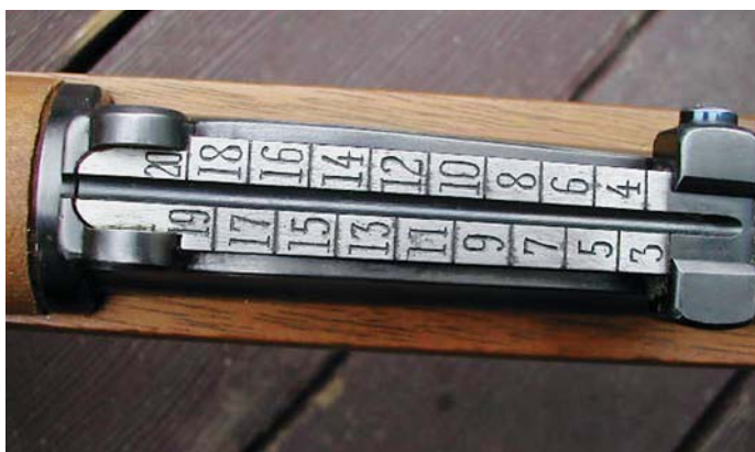
The rear sight leaf of the Mauser patented Model 1896 tangent rear sight assembly with sight graduations from 300 to 2,000 meters. (John Wall collection)
