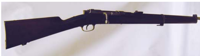
Right side view of the Turkish M1887 9.5x60mm Carbine. (Jan Gardiner collection)
