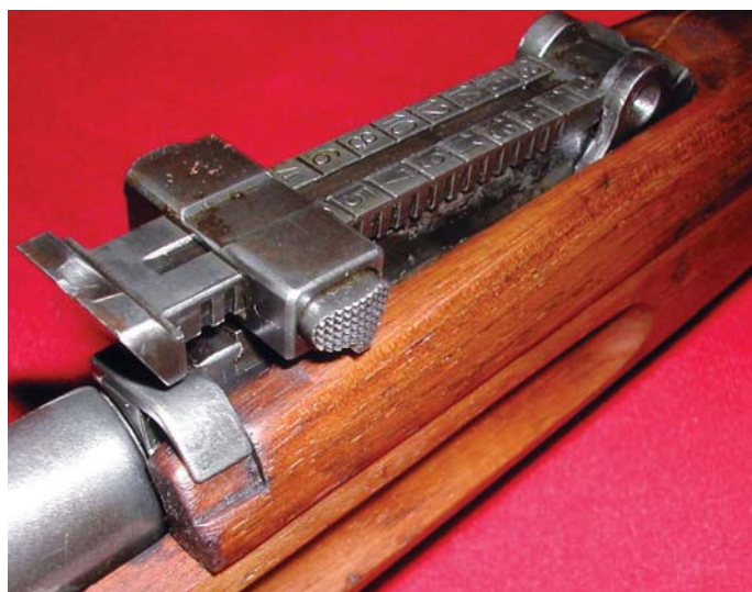
The double button rear sight leaf on the Steyr-made experimental Mauser Short Rifle as used on the Czechoslovak VZ.24. Note the manner in which the handguard surrounds the sight with a protective steel cap at the receiver end, a feature Steyr used on all M.95 Mannlicher straight-pulls made for the Austro-Hungarian and Bulgarian Armies. (U.S. Army Ordnance Museum, Aberdeen Proving Grounds, Md.)
