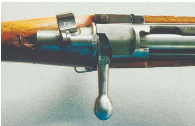
Overhead view of the Mukden Arsenal Mauser Rifle, showing the Japanese-style ovoid bolt knob. Note the safety is slightly bent on this specimen.
