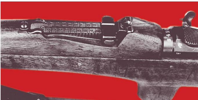
Left side view of the rear sight of the Flier's Rifle. (Robert Jensen collection)
