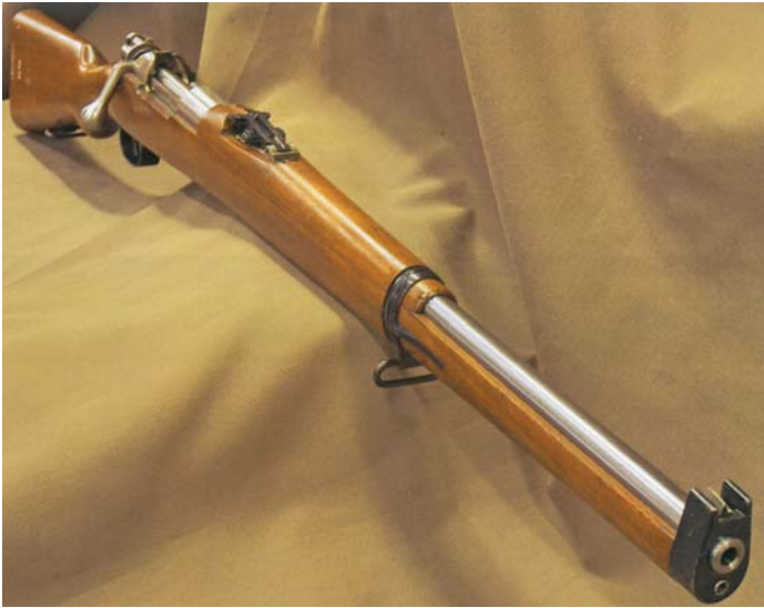
Full-length view of the Turkish Mauser Model 1905 Carbine, SN 5580, 7.65mm. Note the special dual caliber rear sight system, patented by Paul Mauser. (Private collection of Robert I. Landies)
