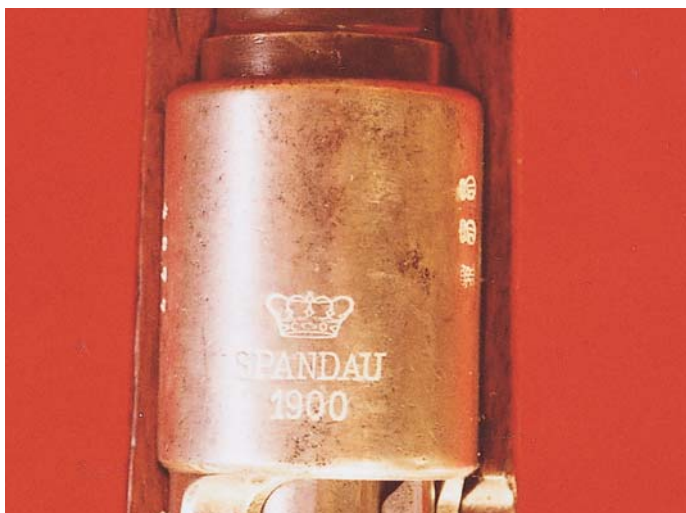
The receiver ring of the Colonial Service marked, modified German Model 98 Rifle, marked "S" on the barrel, and "Crown/SPANDAU/1900" on the ring.
