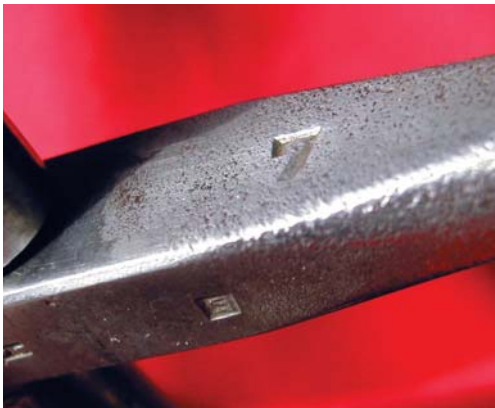
The bolt of the FN-made Model 1889 Heavy Barrel Rifle, showing the serial number "7" stamped on the bolt flat which faces the shooter, and various inspection marks. (John Wall collection)
