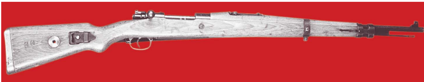
Full-length view of a German Model 24(t) Rifle fitted with a laminated stock.
