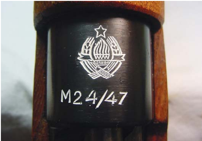
The Yugoslav Communist crest on a Kragujevac Model 24/47 Short Rifle. These rifles are refurbished Model 1924 FN and Kragujevac-made Yugoslav Army short rifles. Because these (and all FN M1924s) utilized intermediate length receivers which were 1/4-of-an-inch shorter than all other military Mauser rifles, parts from M24/47 and M48 will not interchange with other post-war Yugoslav rifles including the Model 24/52c and the reworked German Kar 98ks.
