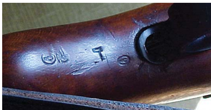
Unique style of Polish inspection marks on the small of a Wz 29 stock. (John Wall collection)
