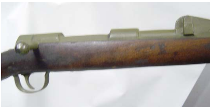
Close-up view of the simulated action of the Gew 98 Training Rifle. Note the simulated Lange-Vizier rear sight. (Jan Gardiner collection)
