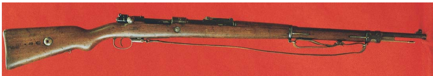
Full-length view of the German G 98 Transitional Model Rifle with the narrow lower barrel band.
