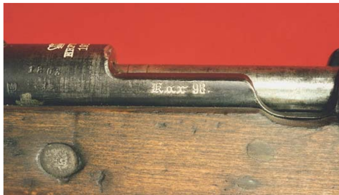
The left side rail of the German Model 98AZ Carbine, showing the model designation.
