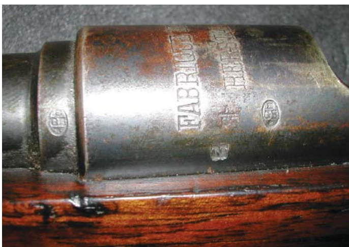
A side view of the Garde Civique Rifle showing the FN address and the "EGB," the official Government proof mark found on firearms accepted into Belgian military service. None of the FN Model 1893 rifles have been observed with this mark. (Pattern Room Collection, Royal Armories Museum, Leeds, England)
