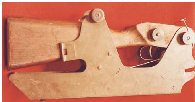
Right side view of the German Trench Rifle-firing Device in its folded, carrying position.
