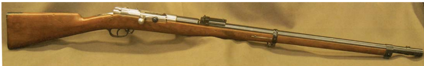
Prototype Mauser Turkish 1887 9.5mm rifle. Note that stock is not completed for the tube magazine feed. Also note the sleeve over the barrel, which is the same as for the Commission 88 rifle. (Private collection of Robert I. Landies)
