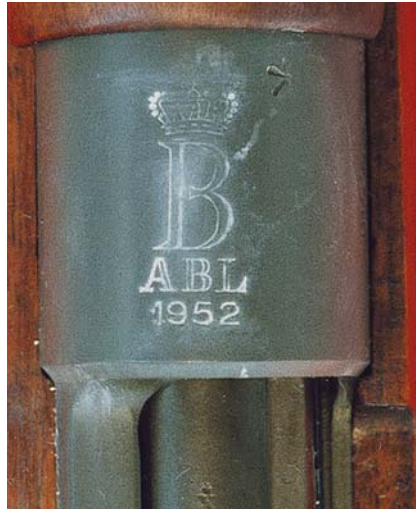
View of the crest of the Belgian Model 24/30 naval .22 caliber Training Rifle. This shows the crown/"B"/"ABL"/date of manufacture markings common to this rifle.
