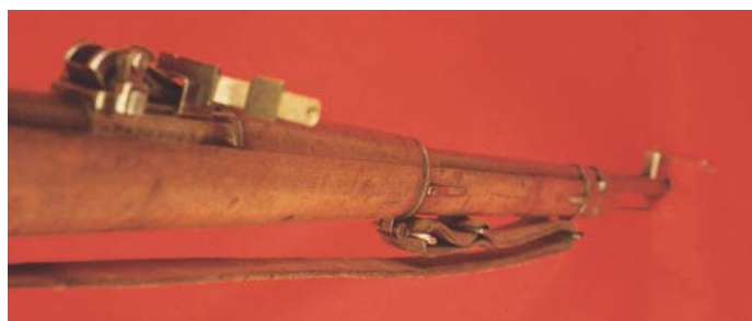
This close-up shows the attachment of the adjustable aircraft rear sight on the German Model G 98 Rifle.
