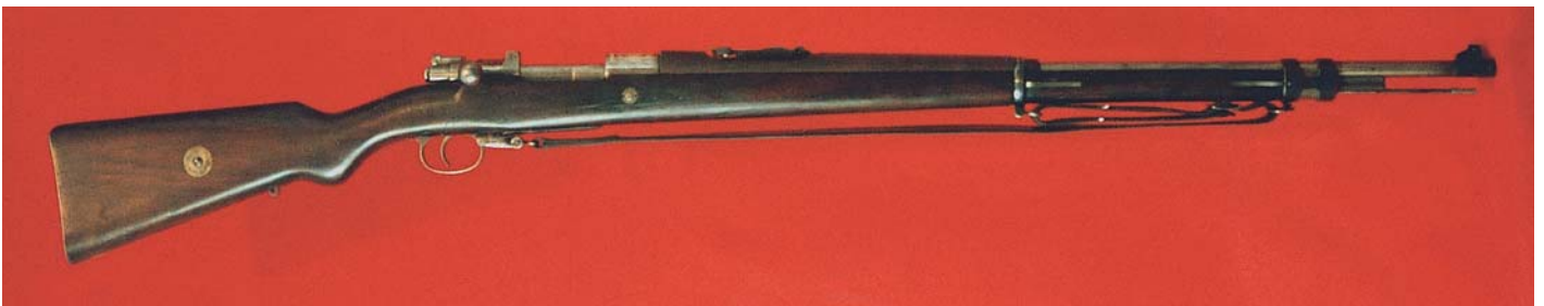
Full-length view of an unusual Peruvian Model 1909 Rifle. Note the tangent leaf rear sight rather than the usual "Lange Vizier" rear sight.
