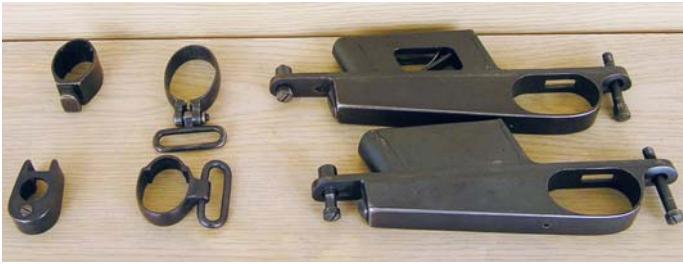
Shown here is a comparative view of the magazine assemblies and barrel bands of the Swedish Model 1892 Mauser Trials Rifle (above) and Carbine (below). Note the cutouts in the magazine walls of the rifle. (Jorma Seppanen collection)
