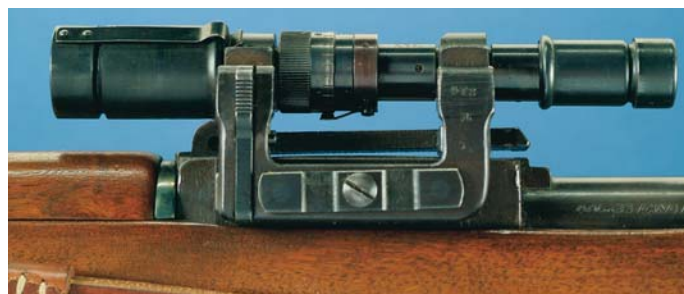
Left side view of KKW Training Rifle, with ZF41 scope, marked "CXN/serial number/ZF 41." (Rock Island Auction Co.)
