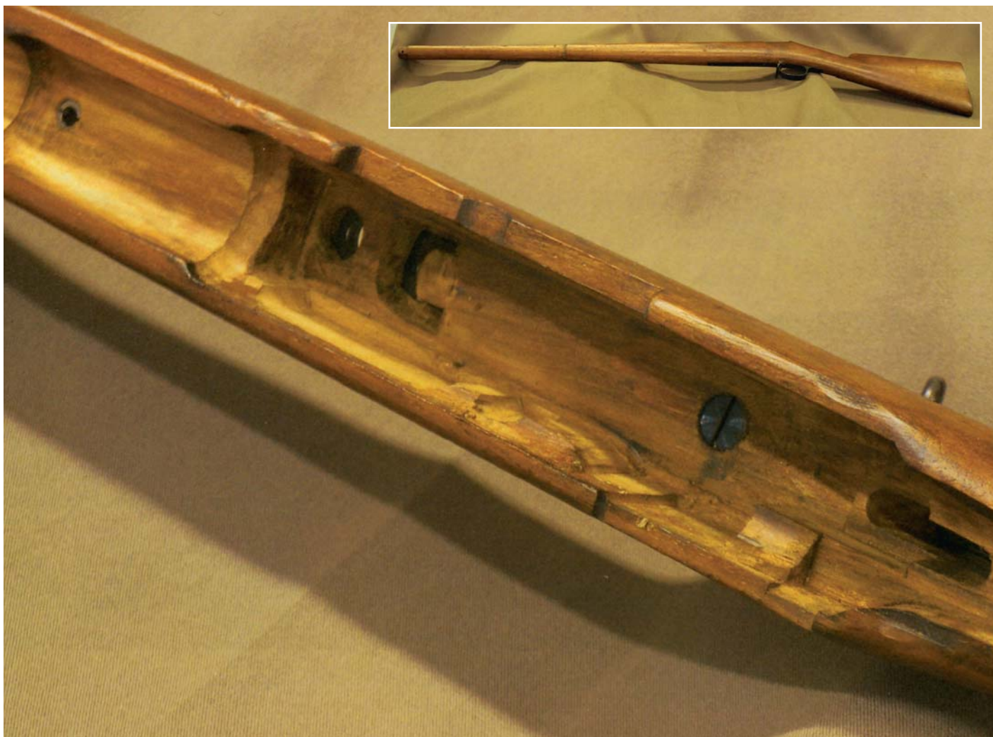
Another view of the inletting required to incorporate the tube magazine feed system in the prototype Mauser Turkish 1887 rifle. (Private collection of Robert I. Landies)
