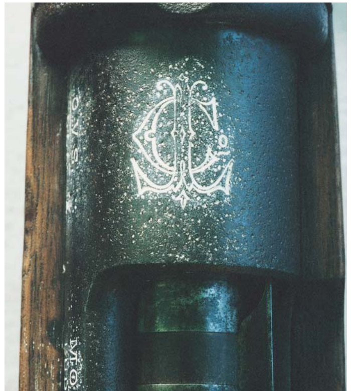
The Ludwig Loewe & Co. crest on the receiver ring of the Model 1896 "OVS" marked Mauser Rifle. The finish on this weapon is peppery due to exposure to the elements.
