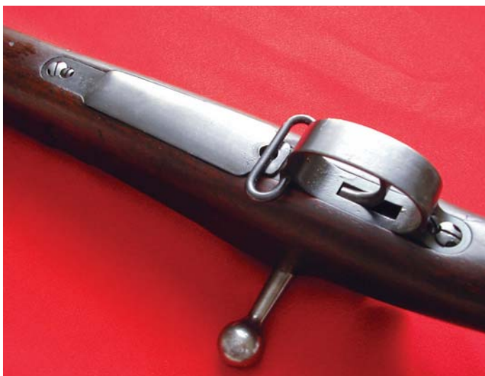
The trigger guard and magazine assembly of the FN-made M1924 Iranian Mauser Short Rifle features a permanently installed third sling swivel. (John Wall collection)
