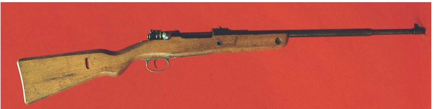
Full-length view of a variation of the German VK-98 Rifle. This weapon has a straight bolt handle, a machine gun barrel, a buttplate, and an internal magazine with floorplate, as well as provision for a sling. The bolt of this rifle was produced without a stop on the bolt sleeve.
