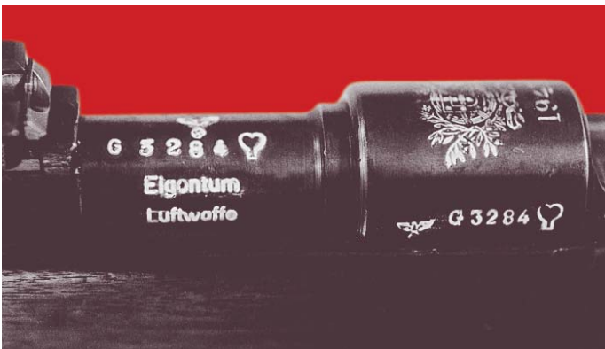
Left side view of the receiver markings on a Portuguese Model 1940 Kar 98k, which was never shipped to the Portuguese, but was remarked and issued to the Luftwaffe. Notice the Portuguese crest. (Robert Jensen collection)
