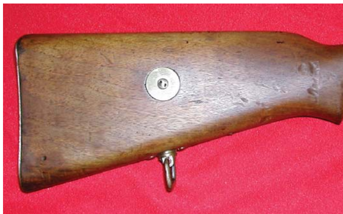
The right side of the Steyr Mauser Cut-away Rifle showing the distinctive pointed pistol grip, a feature often associated with stocks made at Steyr. (U.S. Army Ordnance Museum, Aberdeen Proving Grounds, Md.)
