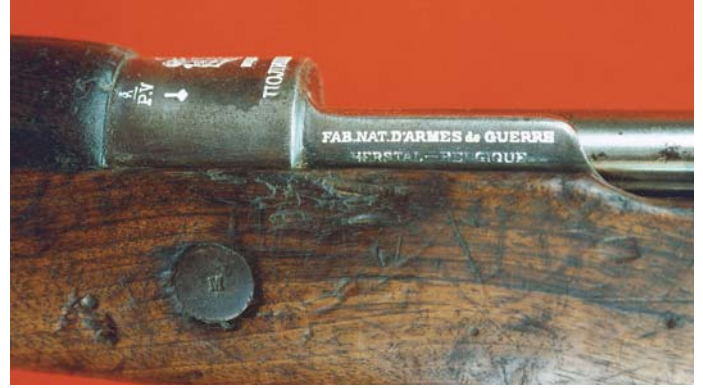
The Belgian proofs on the receiver ring and the manufacturer's markings on the left side rail of the Yugoslavian FN Model 24 Carbine. (Noel P. Schott collection)
