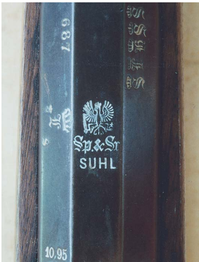
Receiver markings on the German Model 71 Carbine, showing the Spangenberg & Sauer markings.
