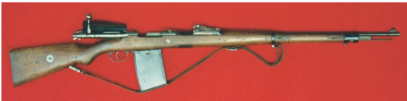
The German Model 98 Rifle with bolt cover and large capacity magazine, showing the action open, illustrating how the sliding bolt cover is attached to the bolt handle.
