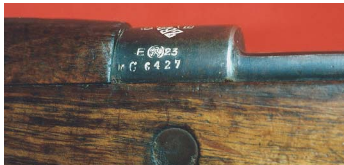
Close-up view of the left side of the receiver of the Czech Model 98/22 Rifle in Turkish service, showing Czech proof marks, as well as the rifle serial number.
