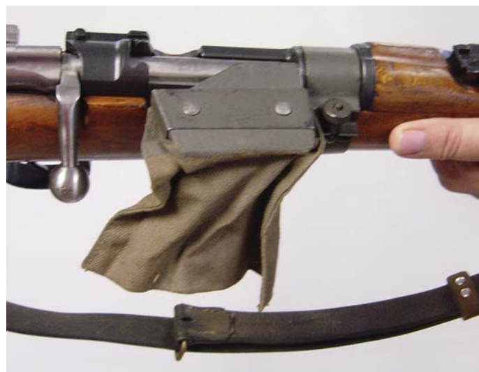
Swedish M1896 Rifle with "shell catcher" attached. (Jan Gardiner collection)
