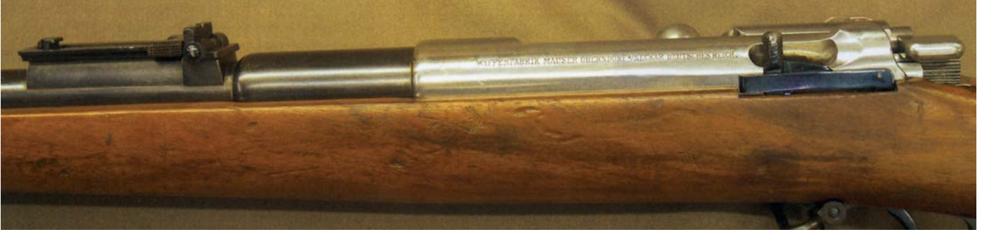
Close-up view of the left sidewall of the prototype Turkish Mauser 9.5mm rifle. Note lack of proofs, etc. (Private collection of Robert I. Landies)
