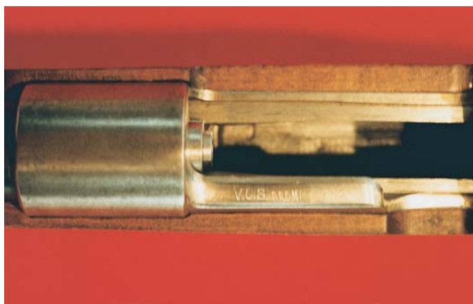
The chamber area of the German Model 98 .22 caliber Training Rifle. This view shows to advantage the spring-loaded chamber that extends into the magazine well area when the bolt is opened, allowing the single .22 caliber round to be loaded by hand. The only markings on the rifle are those seen on the top of the left side rail, in this case, "V.C.S." for Schilling, and "D.R.G.M."
