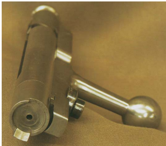
Front view of the bolt head and bolt for the 71/78. Note relief cut on bolt head face. (Private collection of Robert I. Landies)
