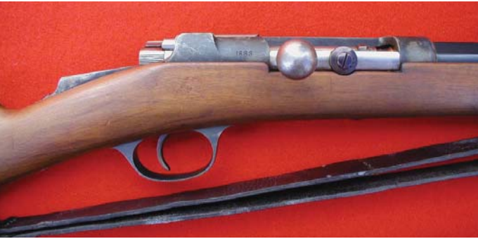
Right side view of the action of the Serbian Model 1878/80 Infantry Rifle, showing to good effect the long receiver tang projecting above the stock providing support to the bolt when it is operated. (John Sheehan collection)
