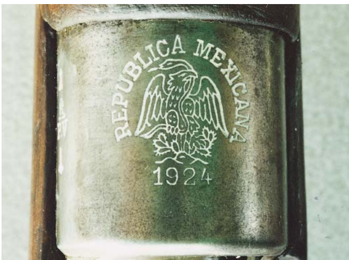
The receiver ring of the Mexican FN Model 1924 Short Rifle, showing the national crest and date of manufacture.
