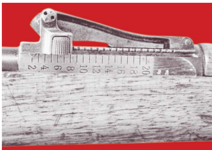
Rear sight of the Colonial Service marked, modified German Model 98 Rifle, showing it registering on 200 meters. This was probably a necessity due to the brush war nature of engagement with the Hereros during the uprisings.
