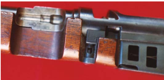
Close-up view of the lower left side of the action showing the cut-away chamber and stock of the Mexican Model 1910 training aide rifle. (R. K. Smith collection)
