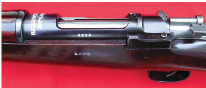
The left side of the action of the FN Model 1893 Carbine, possibly made for Spain. Note the serial number in the 4,000 range, which appears on the side rail and just below it on the stock. (John Wall collection)
