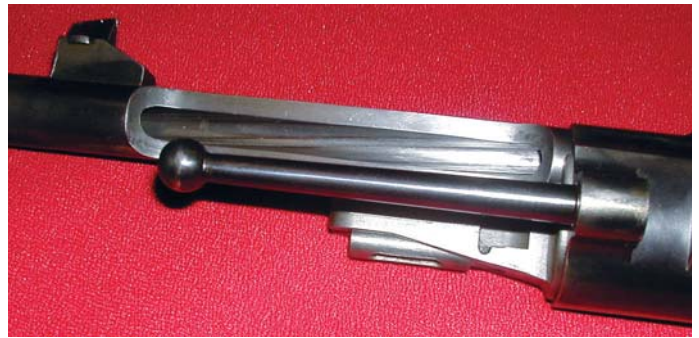
Cut-away section of the barrel and muzzle area of the Steyr-made Mauser 98 experimental Short Rifle. Note the Steyr Mannlicher M.95-type stacking bar next to a modified Mauser Gewehr 98 style bayonet bar, which almost fully conceals the tip of a Mauser Gewehr 98-type cleaning rod. (U.S. Army Ordnance Museum collection, Aberdeen Proving Grounds, Md.)
