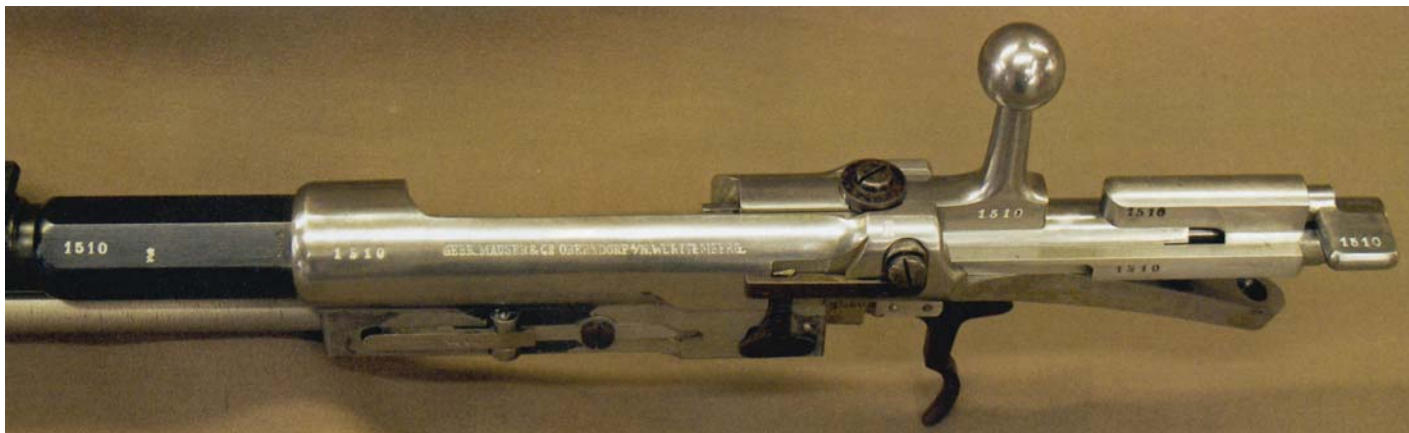
MIDDLE LEFT: Left side stripped view of the new 71/82 design feed tube and locking key for bayonet lug. (Private collection of Robert I. Landies)
