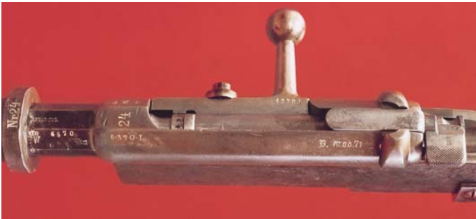
Top view of the action and markings of the German Torpedo Boat 5cm cannon subcaliber firing device.
