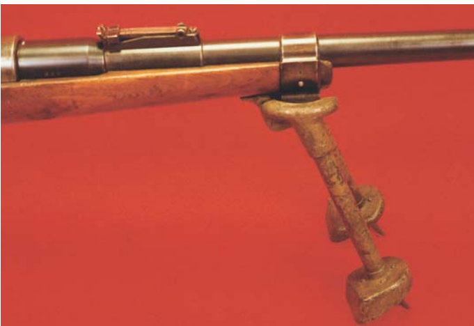
Close-up view of the right side of the purpose-made bipod of the German 13mm Anti-tank Rifle. Note that there is no supporting horizontal bracing bar between the legs as is found on the German 08/15 bipod.
