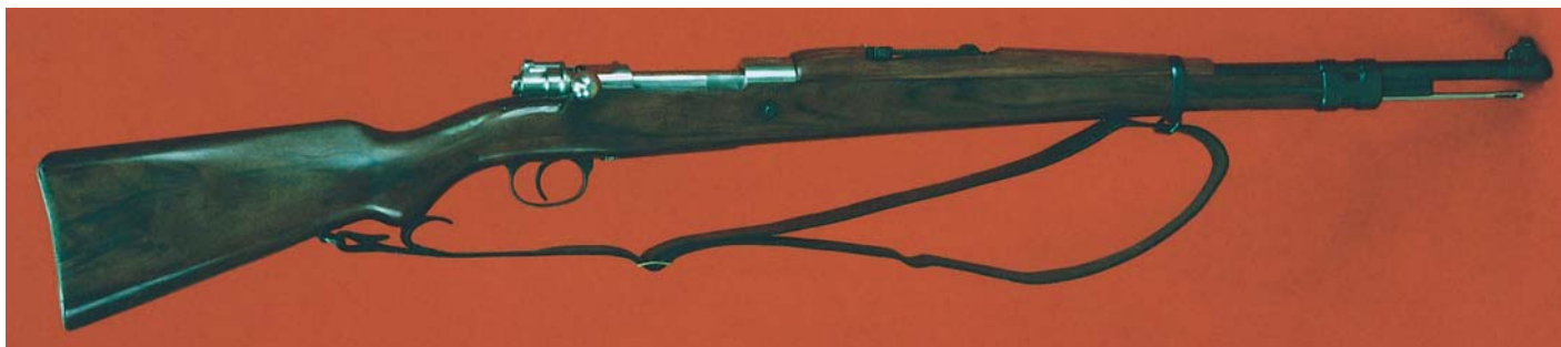
Full-length view of the Venezuelan FN Model 24/30 Short Rifle, but with slight variations. Note that the wrist of the stock is somewhat slimmer, with a less “chunky” look to it. Also note the location of the lower sling swivel in relation to the one shown previously. It is much closer to the wrist than normal. (Lothar Frank collection)
