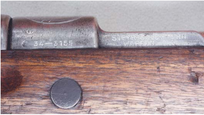
Manufacturer's markings on the left side rail, including the serial number on the receiver ring of the Colombian Steyr Model 1929 Short Rifle.
