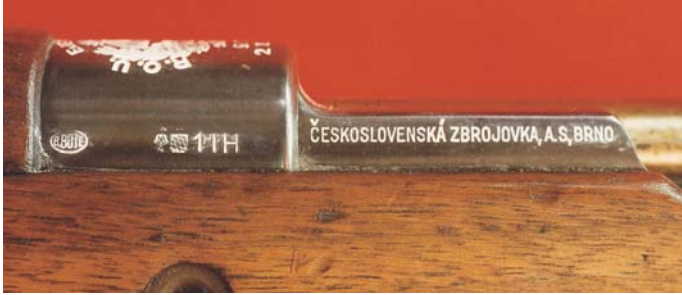
Left side of the action of the Uruguayan Model VZ 37 ("937") Short Rifle, showing the proof marks and the manufacturer's markings in Czech. (Noel P. Schott collection)
