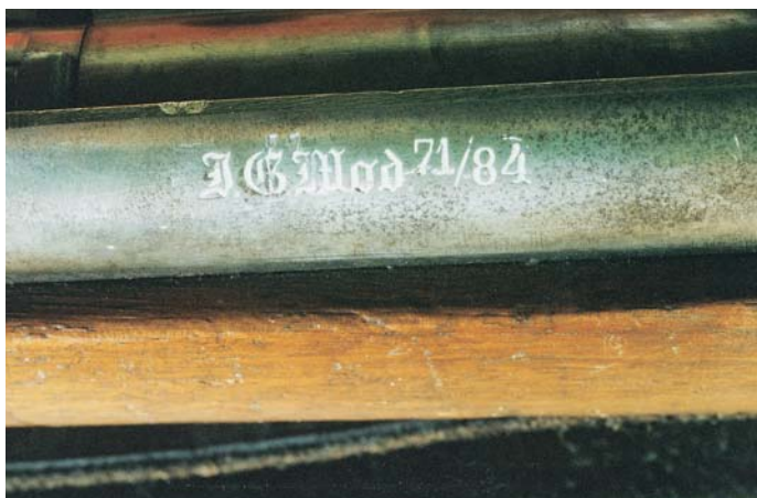
Model designation, "I. G. Mod 71/84" on the left side rail of the German Model 71/84 Rifle.
