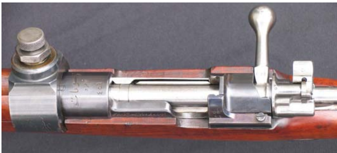
A top view of the Turkish “Customs Administration” Model 1903 Rifle. The top line of Turkish text translates as “Customs Administration” according to Terrence Lapin in his book “Mauser Military Rifle Markings.” Below this is the serial number of the pressure test rifle, 459. (John Wall collection)
