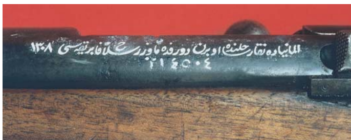
Manufacturer's markings in Turkish over the serial number on the left side rail of the Turkish Model 1887 Rifle. (Cliff Baumann collection)
