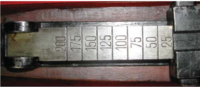
The rear sight leaf of the Model 1924 Belgian .22 caliber Mauser Training Rifle, showing range gradations of 25 to 200 meters. (John Wall collection)
