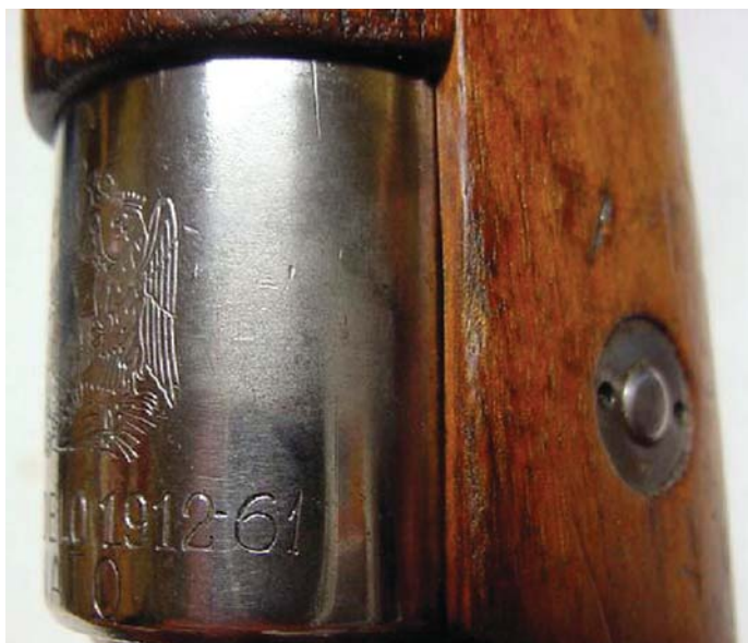
Many Chilean Model 1912 long rifles made by Steyr were converted to 7.62 NATO by being re-barreled with shorter 60 cm barrels. Some conversions have been noted without any identifying marks other than the short barrel. Others, as shown here, were re-marked on their receiver rings with the numeral "61" and the acronym "NATO," thus identifying the rifle by its new nomenclature, the "Modelo 1912/61." (Ed Parada collection)
