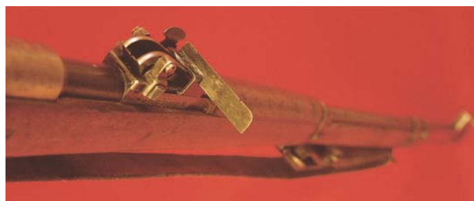
This close-up shows the attachment of the nonadjustable aircraft rear sight on the German Model G 98 Rifle.
