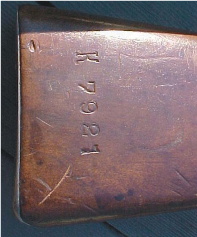
The buttstock of a "K" block Czechoslovak Army VZ 23 illustrating the stock-numbering convention for these rifles. Dr. Sada documents the Czechoslovak Army-authorized production of 130,000 VZ 23 rifles, which would account for 13 blocks of VZ 23s, serial numbered, 13-letter prefixes "A" through "M," with 9,999 rifles per production block. VZ 23 rifles in the "O" block with 1924 dates have been noted. (John Wall collection)
