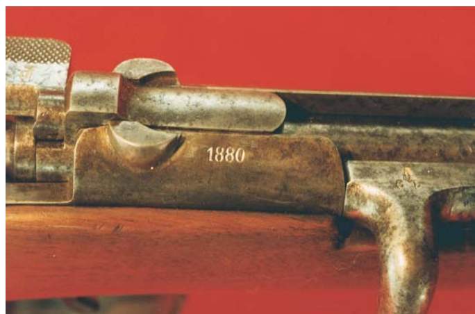
Right side wall stamping indicating date of manufacture of the German Model 79 Rifle. Note the serial number 19.
