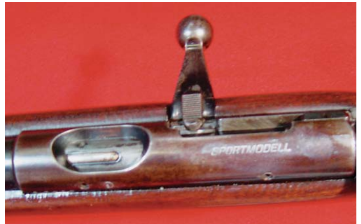
Close-up view of the action and receiver markings on the "PAAST/SPORTSMODELL" .22 caliber Training Rifle. Note the shape of the bolt handle.
