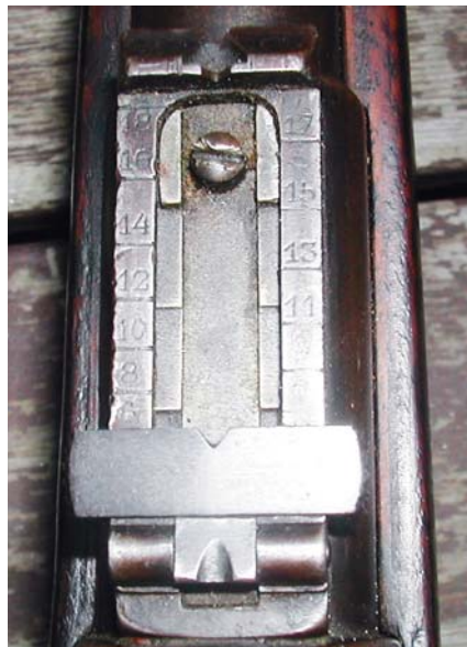
The rear sight configuration on the Model 1889 Mounted Gendarmes Carbine. (John Wall collection)
