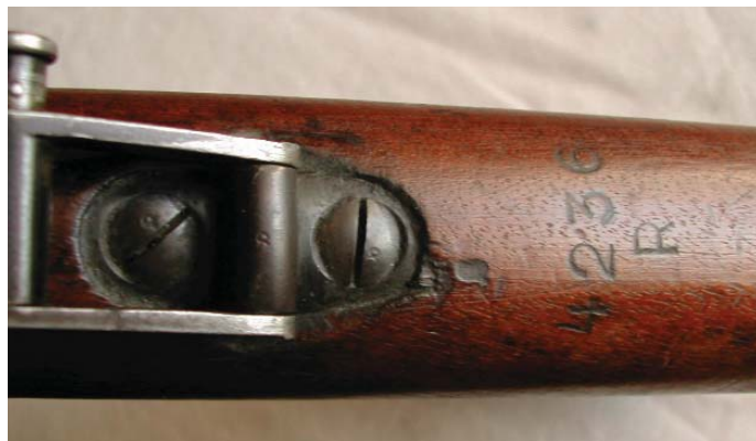
The CZB-made "Mod. 1908/34" Carbine uses the Gewehr 98-style quick detachable sling swivel and boss, and is numbered across the lower comb in the German style.
