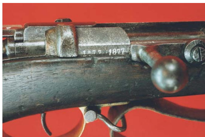
Year of manufacture on the right rear receiver flat of the German Model 71 Rifle.
