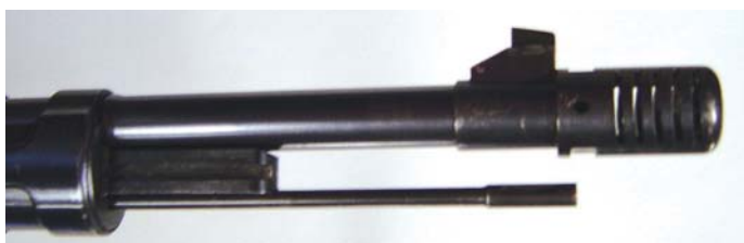
Close-up view of the M40 Swedish K98k Short Rifle muzzle brake.
