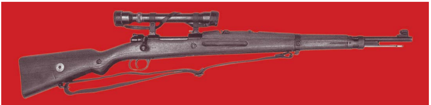
Czech VZ 24 Sniper Rifle, with turned down bolt handle for clearance of the claw-mounted Czech Sniper Scope. (Robert Jensen collection)
