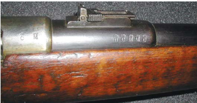
Another view of the right side of the Serbian Model 1884 Artillery Carbine, showing the barrel inspection marks next to the rear sight leaf. (From the former Pattern Room Collection now in the Royal Armouries Museum, Leeds, England)
