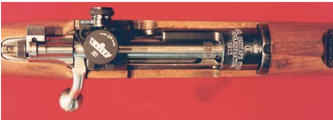
Top view of the action and special target rear sight of the Swedish Model 1896 Military Target Rifle.
