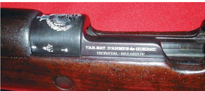
The left side of the receiver of the Model 1924 Mauser Rifle made for Iran. A unique characteristic of the Model 1924 series is the fact that they were all made with "intermediate length" receivers, and thus are an eighth of an inch shorter than the rest of the Mauser rifles of the day which used a receiver that was 8.75 inches long, called a "standard length receiver." Model 1924 rifles and carbines are also heavily serialized, and were seemingly not made under a system of manufacture that provided interchangeable components with a high degree of reliability. Because most of the components on this Iranian Short Rifle are not serial numbered, this likely dates this rifle to the post-1930 era, when the FN Model 1930 went into production, a rifle with a standard length receiver and whose manufacturing technology produced highly interchangeable parts without hand-finishing and fitting. Note the early side rail address written in a font with serifs, and the Liege proofing. (John Wall collection)
