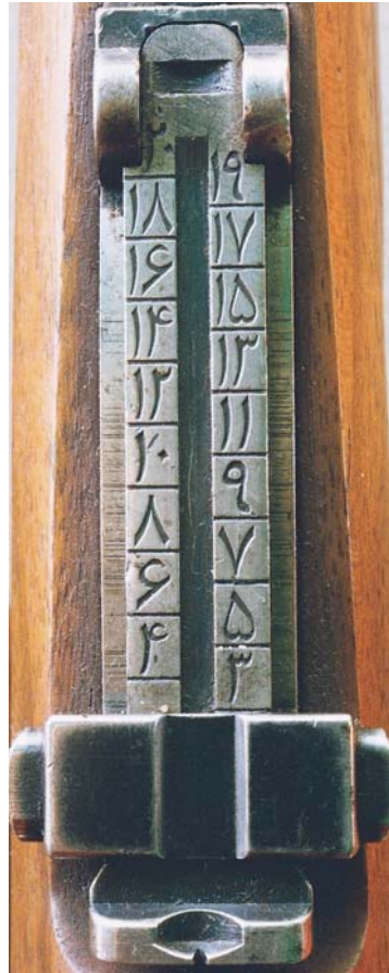
Rear sight graduated in Farsi of the Persian Czech Model VZ 24 Short Rifle.
