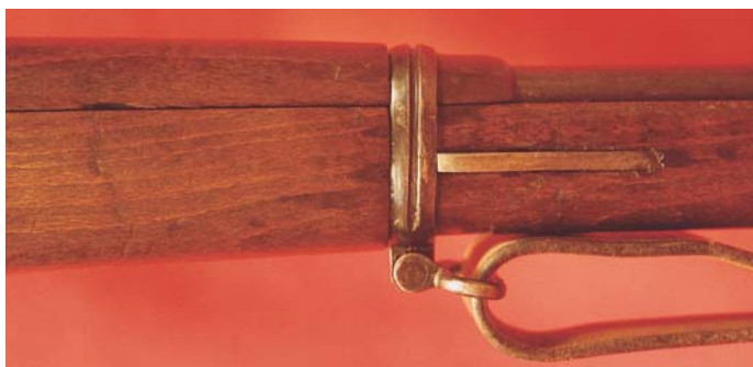
Close-up view of the narrow lower barrel band on the German G 98 Transitional Model Rifle.
