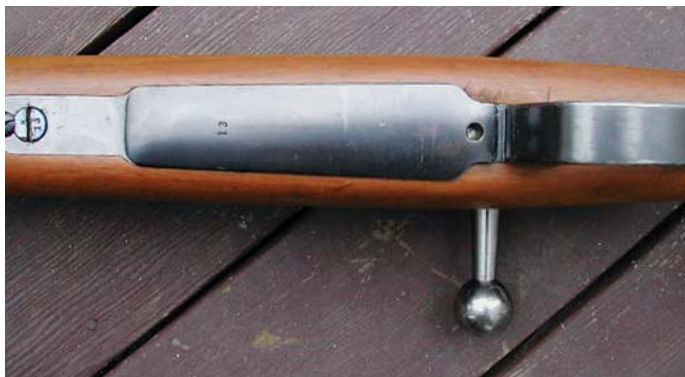
The magazine assembly and floor plate of the Mauser Model 1898 5.97mm Test Rifle. Note the absence of all proof and inspection marks, except for the serial number “13.” (John Wall collection)
