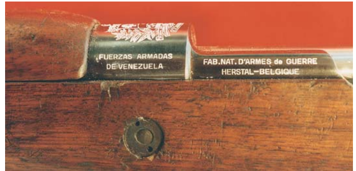
Venezuelan army markings on the left side of the receiver, and the manufacturer's markings on the left side rail of the Venezuelan FN Model 24/30 Target Rifle.
