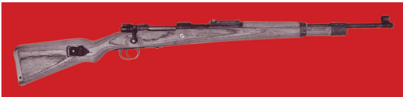
Right side view of the full-length of a late-war production Kar 98k Carbine, illustrating the gradual simplification and short cuts, i.e. lack of bayonet lug, take-down hole in the buttplate, omission of the stock washer, poorly finished laminated stock, etc. taken at the end of WWII in order to keep production as high as possible.
