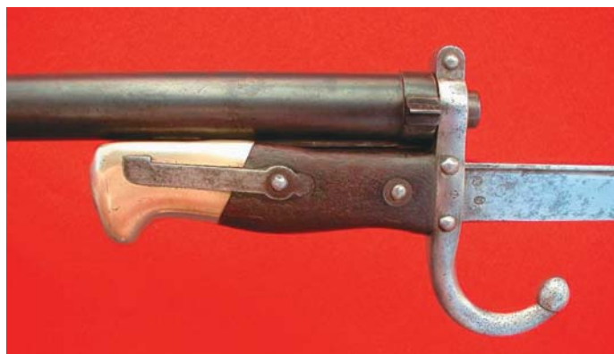
This carbine was adapted to utilize a surplus Model 74 French Gras bayonet. Gras bayonets were readily available, and a similar adaptation is known to have been added to a small number of Model 89 Infantry rifles. Bayonets were in short supply from time to time, and alterations such as this were to be found in nearly every army that fought in WWI. (John Sheehan collection)
