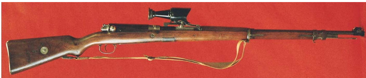
Full-length view of the German Model 98 Marksman Rifle fitted with a sliding bolt cover and a low light optics, bifocal marksman scope and front sight.
