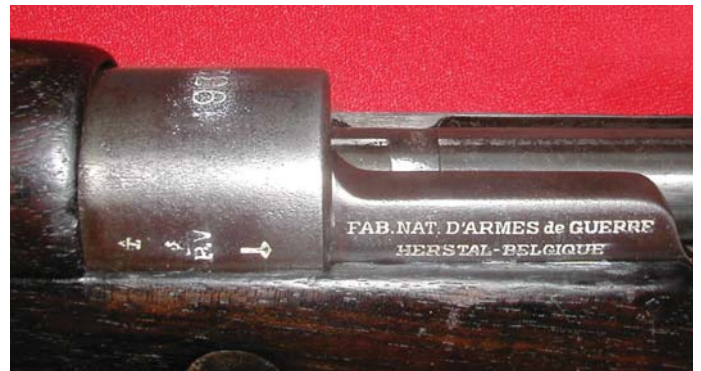
The action of the Model 1924 Chinese Short Rifle with the “1932” receiver crest, showing the FN side rail address using the serif font typical of rifles made at Herstal in the mid-1920s to the middle 1930s. (John Wall collection)
