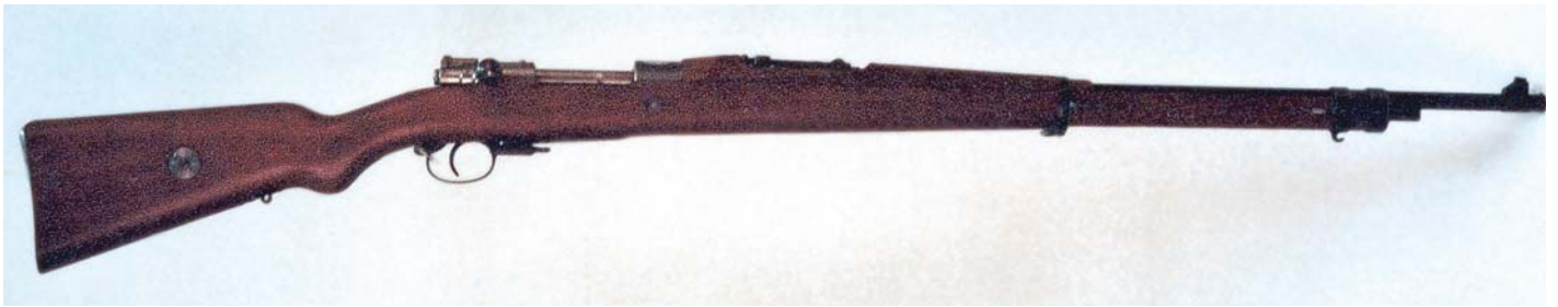
Full-length view of the Modelo 1907 Rifle. Note that this rifle is missing the lower sling swivel and cleaning rod. (Springfield Armory Museum)
