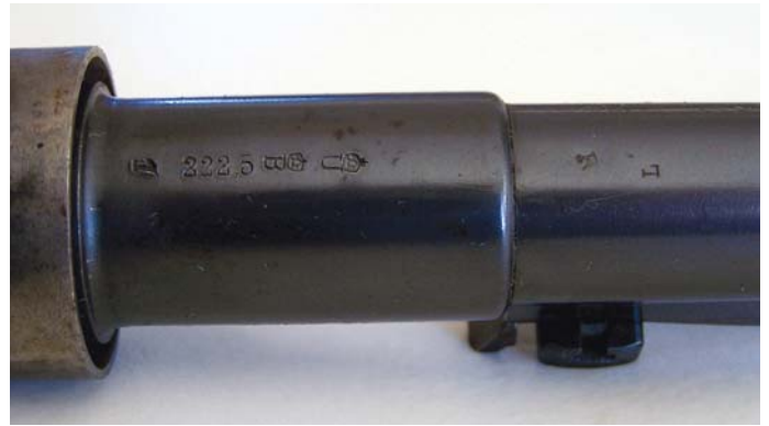
The underside of the barrel at the breech of the Serbian Model 1910 Short Rifle reveals the German commercial “B” and “U” definitive proof marks for shoulder-fired weapons. Many instances are known where a purchasing country acquired Mauser rifles in Germany and allowed the factory to proof test their arms using the German commercial proof standards established in the German proof laws of 1891 and 1911. (David Jonas collection)
