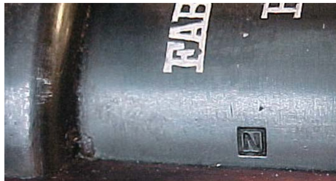
The boxed letter “N” mark seen on many Mauser components made by FN. Its meaning is still unknown. (John Wall collection)
