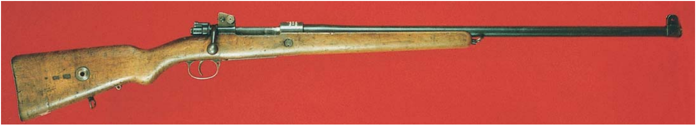
Full-length view of a Danish Military Target Rifle utilizing the action of a German G 98 Rifle. Note the bending of the bolt handle.
