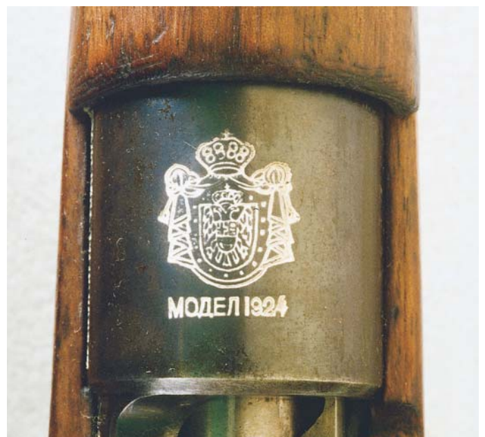
Yugoslavian crest over the model designation on the receiver ring of the Yugoslavian Model 24 Short Rifle.
