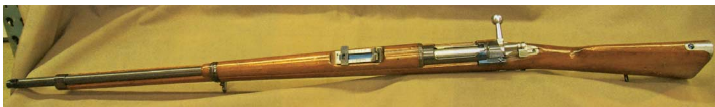
Full-length top view of prototype Spanish Model 1892 Troop Trials 7mm rifle, SN 2. Note 2-position magazine cutoff. (Private collection of Robert I. Landies)
