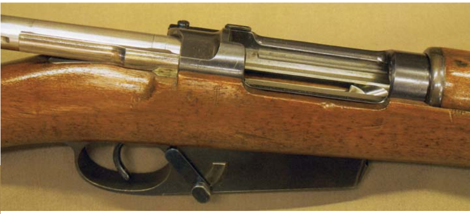
ABOVE: Mauser prototype Spanish Model 1892 SN 2 Troop Trials 7mm rifle with cutoff in the raised position.
