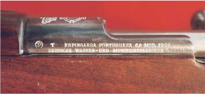
The left side rail of the Portuguese Model 1904 Mauser-Vergueiro Rifle, showing the model designation and caliber in Portuguese and the manufacturer in German.
