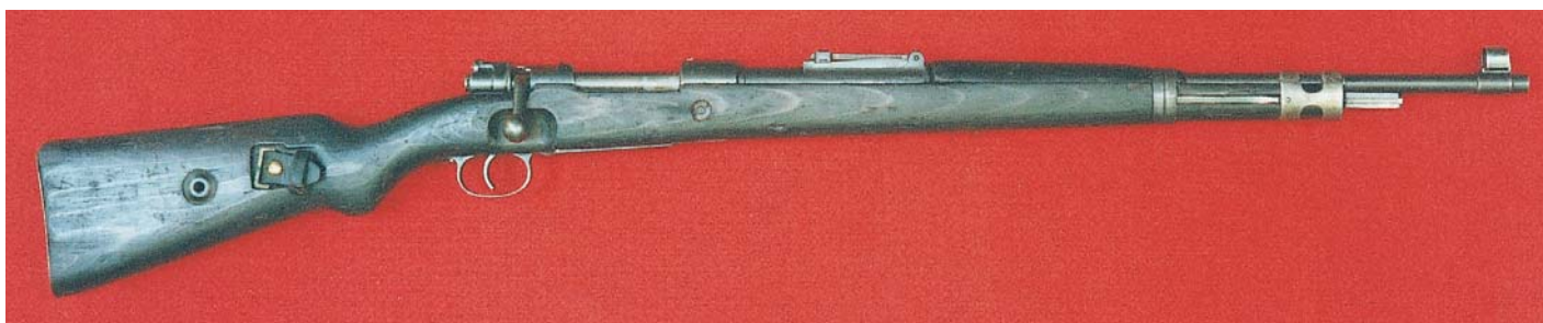
Full-length view of the later version of the German Model 29/40 Rifle, fully comparable to the German K98k Carbine except for the markings.
