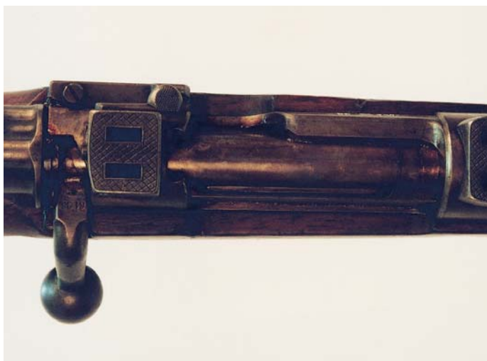
The German Model 98 Sniper Rifle as viewed from above, showing the location of the claw mounts. (Springfield Armory Museum)
