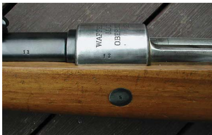
A close-up of the left side of the Model 1898 5.97mm Oberndorf “versuchsgewehr.” Note the absence of any proof and inspection marks, and the bare side rail. (John Wall collection)
