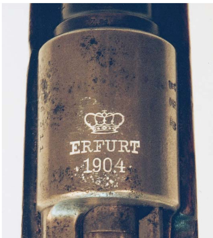
The receiver ring of the German Model 1898 Carbine (Kar 98A), showing the crown, the Erfurt arsenal marking, and the date "1904." (Springfield Armory Museum)
