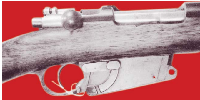
Close-up view of the right side of the special test Model #3 1892 Mauser Rifle, showing the cutoff lever pivoted upwards. (Springfield Armory Museum)
