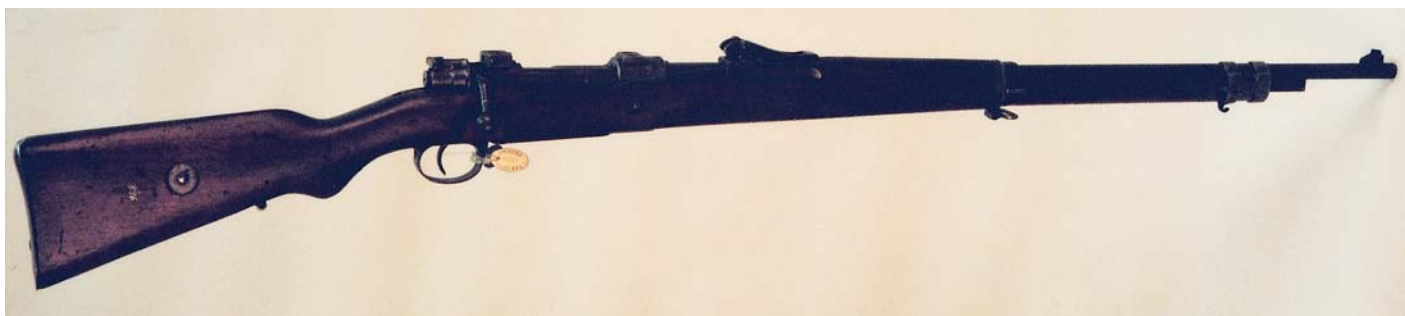
The German Model 98 Rifle modified in 1915 for use as a sniper rifle. The receiver and the receiver bridge have claw mounts for a 4 x Goerz or Zeiss telescopic sight. The scope mount would be offset to the left in order that the rifle could be used as a clip loader. The bolt handle is bent down, and there is a recess cut in the stock to accommodate the bolt knob. The rifle is otherwise identical to the standard issue Model 98 Rifle. (Springfield Armory Museum)
