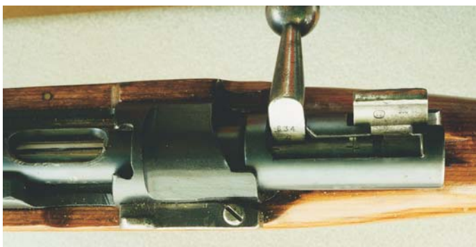
Another view of the German Model 98k Carbine with ERMA Model EL .22 caliber insert, giving a better impression of the bolt and the action itself. This was an inexpensive, as well as practical, method of training unskilled recruits in the handling of military weapons. The ERMA unit would normally be kept in a lidded wooden chest that had been machined to accept the various components of the insert.
