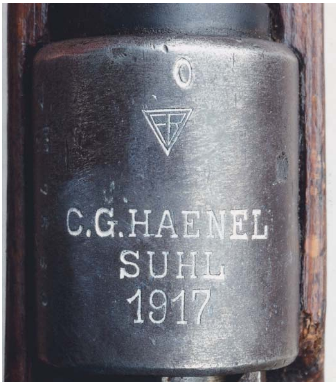
Markings on the receiver of the Wz 29 Short Rifle made from World War I reparation parts. Note the diamond-shape Radom symbol above the C.G. Haenel markings. (Century International Arms, Inc.)
