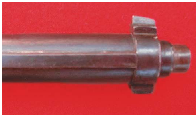
The bayonet lug and tenon added to this carbine were silver soldered and riveted to the barrel jacket. (John Sheehan collection)
