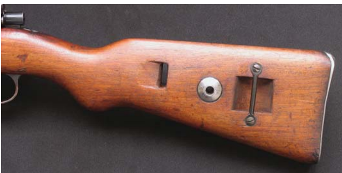
The buttstock of a German Kar. 98b modified post WWII by the French with a stock recess to accept the MAS36 sling and sling bar. The unit marking plate is stamped "5/R.R. 12.35," for the Fifth Reserve Infantry Regiment, 12th Company, rifle number 35. (John Wall collection)
