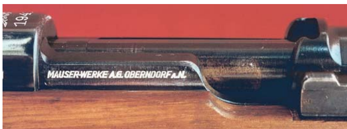
Manufacturer's markings stamped on the side rail of the Portuguese Model 41 Short Rifle.
