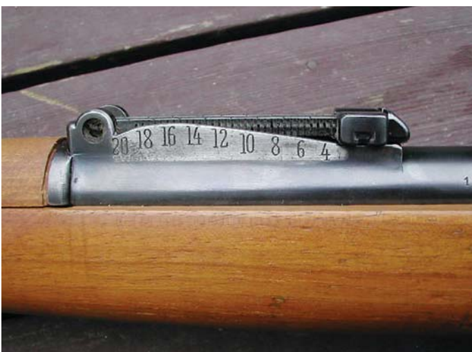
The Mauser patented Model 1896 rear sight assembly, reportedly (Gotz) used by Mauser on its test rifles as a preferred alternative to the Lange rear sight used on the German Model 88/97 test rifles. (John Wall collection)
