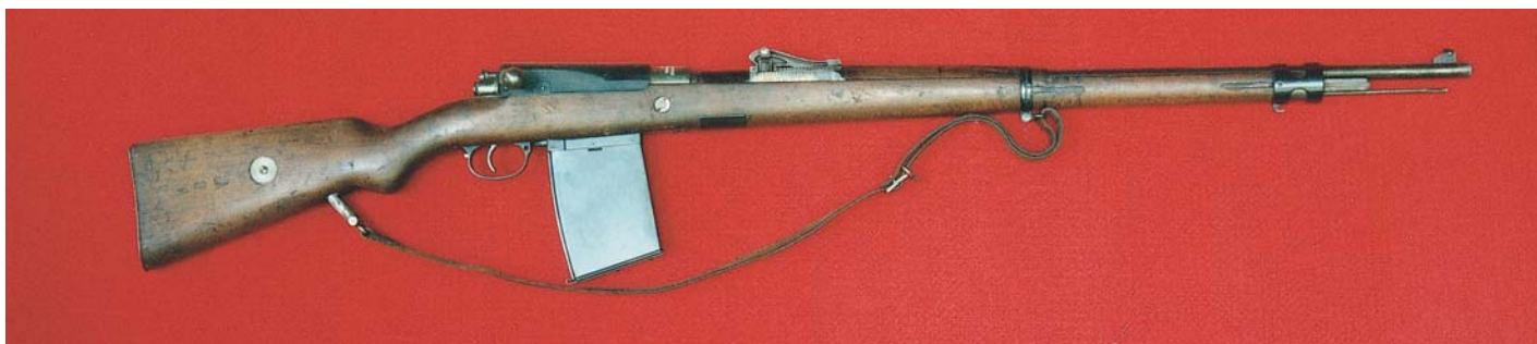
German Model 98 Rifle equipped with a sliding bolt cover designed to keep mud and debris out of the action of the rifle. The rifle is also fitted with a non-detachable large-capacity magazine, which increased the rifle capacity to 25 cartridges.
