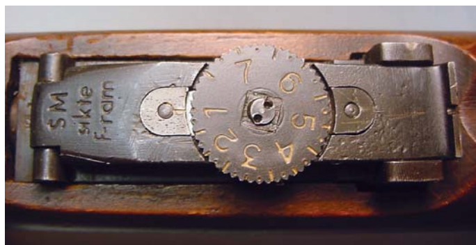
The SM Sikte F-ram sight, an experimental variation of the target shooter's SM Sikte M/58 military rear sight, but adjustable to 800 meters as opposed to the 600-meter up limit on the M/58 sight.
