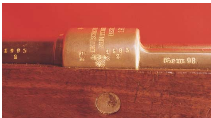
Side view of the receiver ring of the star-marked G 98 Rifle shown left. Another interesting fact is that these rifles had a numeral suffix, as opposed to alpha suffix. Note how the former serial number is canceled.
