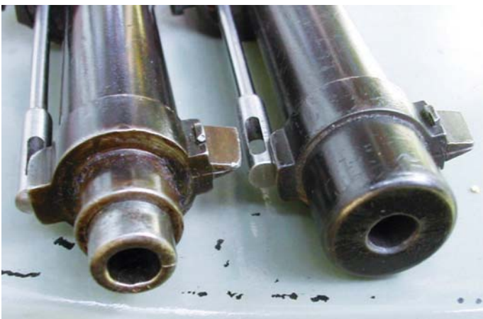
A comparison of the officially adopted 7.65mm Model 1889 Infantry Rifle muzzle on the left, with the blunt muzzle of the Model 1889 Heavy Barrel Rifle on the right. Although the upper band of the heavy barrel rifle does have a bayonet lug, the lack of the protruding muzzle and the associated extra barrel length means that the heavy barrel rifle prevents it from accepting a bayonet. (John Wall collection)
