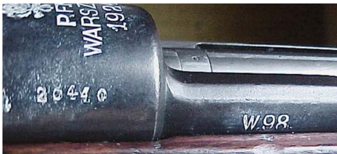
The serial numbering and side rail marking conventions used on the Polish W.98s (Gewehr 98) made at Warszawa in the mid-1920s. (John Wall collection)
