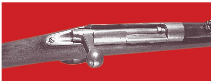
Top view of the receiver area of the Model 67/69 Mauser-Norris Rifle; note the mainspring incorporated as part of the bolt handle. (Springfield Armory Museum)
