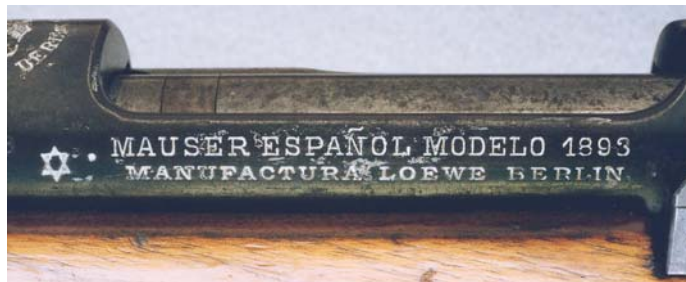
Manufacturer's markings stamped in Spanish on the left side rail of the Spanish Model 1893 Rifle.
