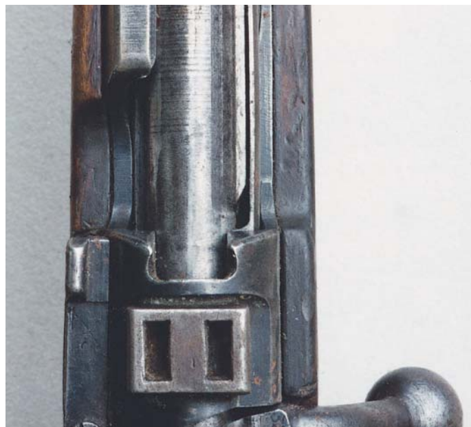
Top view of the claw mounts on the sniper model German Model 98k Carbine (bottom of page). Note the markings on the receiver both in front of and behind the front mount. (Century International Arms, Inc.)
