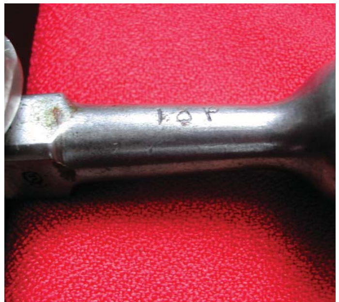
The straight bolt handle on the Iranian Model 1924. Note that the serial number is inscribed on the part of the handle facing the shooter's eyes. (John Wall collection)
