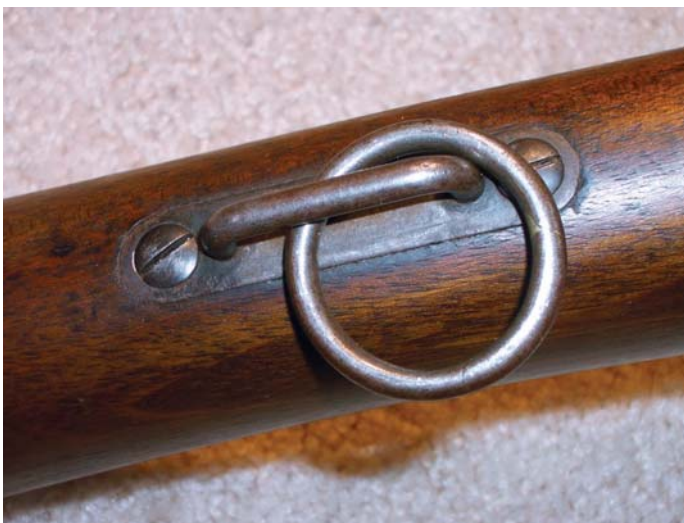
The cavalryman's lanyard ring found on the underside of the stock wrist of the 7.65mm Spanish Model 1891 Carbine. (Hans-Joerg Meyer collection)
