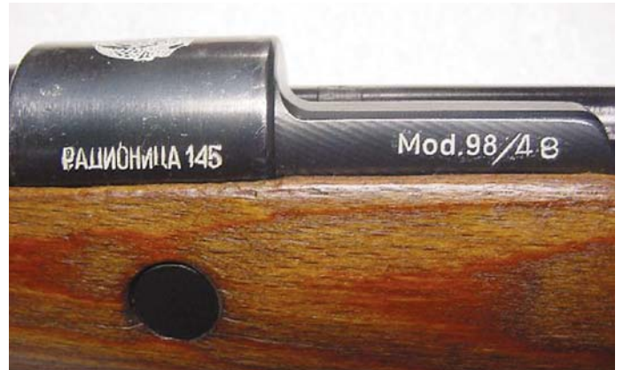
After WW II, the new Federated National Republic of Yugoslavia began a program of reworking and reissuing former Axis services rifles for their new army. The rifle shown above, originally built as a German Kar 98k, has had its original receiver ring markings removed, and has been reblued. First however, the crest of the new Communist Government and the Slavic phrase "Workshop 145" were applied to the receiver and the original German side rail marked "Mod. 98" was modified by having "/48" stamped next to it. 1948 was the year the refurbishing of the K98k's began. The location of Workshop 145 is unknown. (Ed Parada collection)
