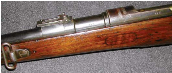
The side-mounted sling swivel of the Garde Civique Bicyclist's Rifle. Note that the earlier swivel was located closer to the rear sight. (Pattern Room Collection, Royal Armouries Museum, Leeds, England)
