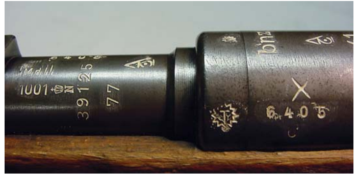
An ex-Wehrmacht, ex-Russian, ex-East German ex-Iraqi Kar 98k. BNZ 41 indicates manufacturer at OEWG Steyr, Austria in 1941. The "X" (crossed rifles) is the Red Army capture mark, the sunburst and crown over "n" are East German proof marks, and the Arabic letter in the triangle is an Iraqi Government property mark.
