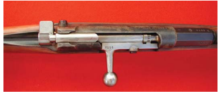
The Serbian Model 78/80 and Model 84 were the only Mausers designed with a bolt guide extension extending from the rear of the action into the stock wrist. (John Sheehan collection)
