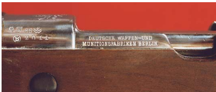
Left side of the action of the Uruguayan Model 1908 Rifle, showing the serial number and proofs on the receiver ring and the manufacturer's markings on the side rail. (Noel P. Schott collection)
