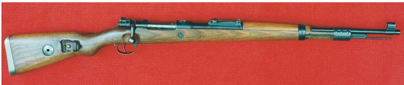
Full-length view of a late-war German Model 98k Carbine, FN manufacture. Note the laminated stock, the crude bands, and cupped buttplate.
