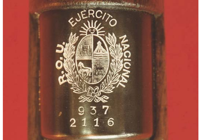
The top of the receiver ring of the Uruguayan Model VZ 37 ("937") Short Rifle, showing the national crest and other markings. (Noel P. Schott collection)
