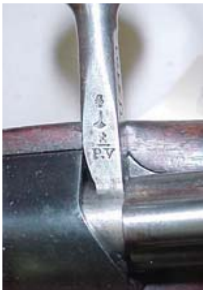
The action of the Pieper Model 1889/36 conversion. Note the checkered surface of the underside of the bolt handle, indicating that the bolt had originally been a turned down bolt for a Model 1889 Carbine, which Pieper straightened for the conversion. (John Litt collection)
