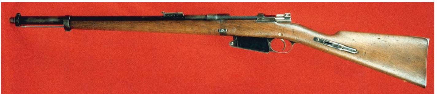
Full-length view of the left hand side of the Belgian Model 1889 Carbine, standard version converted for Cavalry use. Note the slotted sling attachment.
