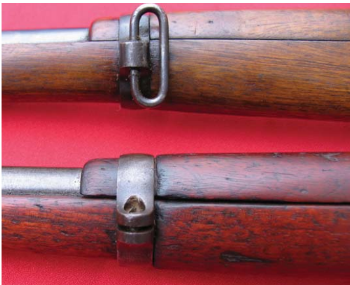
A comparison of the two varieties of German-made Ludwig Loewe Spanish Mauser carbine barrel bands. The lower band, on an 1894-dated Carbine can be adjusted by a screw and has no sling swivel, while the upper band, on an 1896-dated Carbine, is solid and has a side-mounted swivel attached. (John Wall collection)
