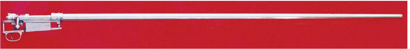
Ammunition test barreled action; action is a 98k with receiver code "S/42/1937." Serial number on barrel and receiver is #8. Barrel is chambered for 8x57mm. Barrel is 51-3/8" long, 1-3/16" at the receiver, with no German proofs on the receiver. (R. K. Smith collection)
