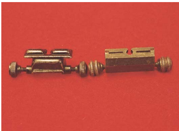
A comparison of the pressed steel auxiliary night sights on the left, as opposed to the machined steel auxiliary night sights at the right. Both sights were phosphorous coated in the two inset to either side of the sight notch.
