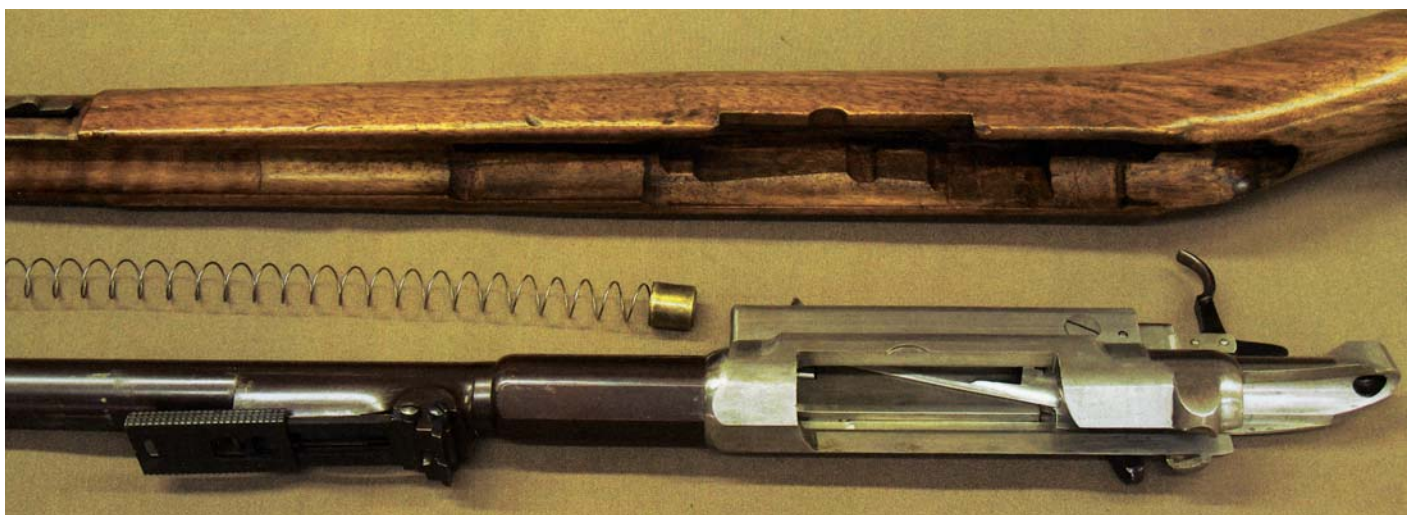
BELOW: Model 71/78 stock, tube feed spring and cap, and barreled action. (Private collection of Robert I. Landies)
