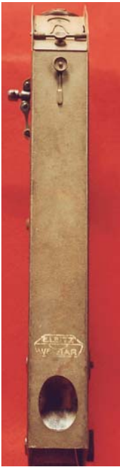
Left: The eyepiece of the periscopic viewfinder of the German Trench Rifle-firing Device.
