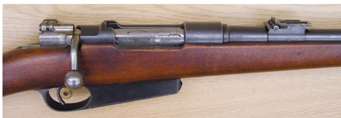
The right side of the action and rear sight assembly of the Swedish 8x58R Danish Model 1892 Trials Carbine. (Jorma Seppanen collection)
