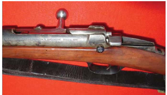
The siderail markings of this rifle are set against the backdrop of the original color case-hardening of the receiver. The markings are in Cyrillic and translated read as, "Mauser Oberndorf a'n Wurttemberg Model 1880." (John Sheehan collection)
