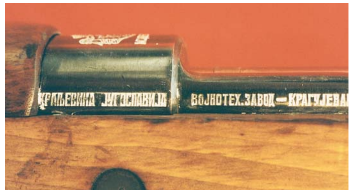
Manufacturer's markings stamped into the side of the receiver ring and the left side rail of the Yugoslavian Model 24 Carbine.
