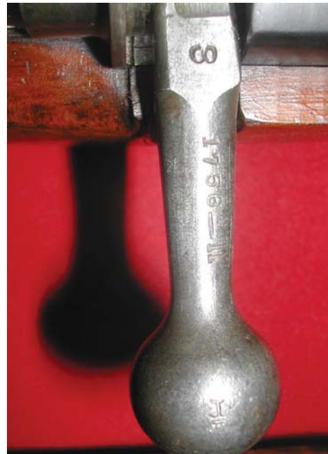
The bolt of the M1924 Yugoslav Short Rifle, showing the unusual serial number "1756-II", and the smokeless powder proof mark, crown over "T" on the bolt knob. (John Wall collection)
