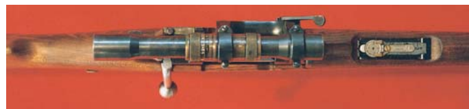
Top view of the Model 42 AGA scope, action, and rear sight of the Swedish Model 1896 Sniper Rifle.
