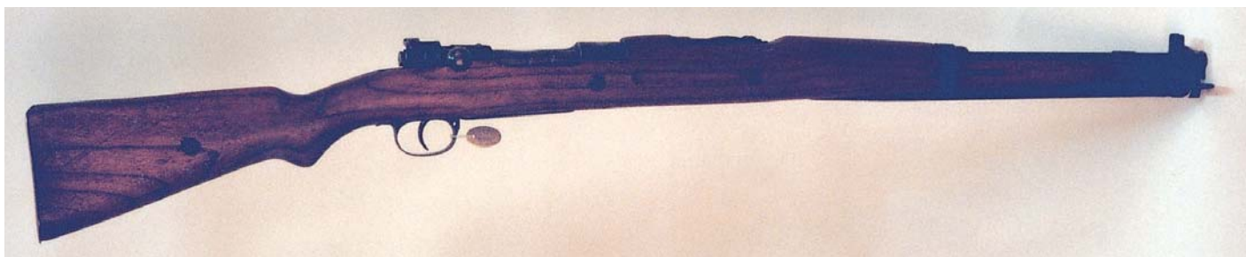
Full-length view of the modified Chinese copy of the Czech VZ 24 Short Rifle with folding bayonet. (Springfield Armory Museum)
