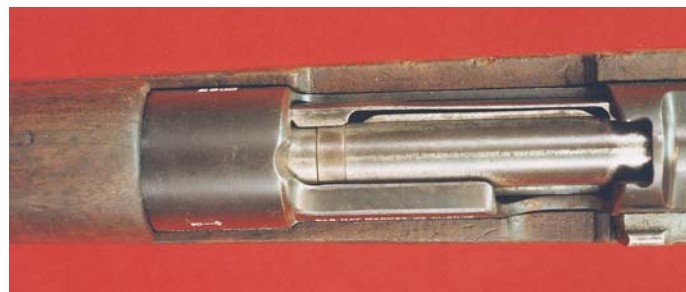
Top view of the action of the Haitian FN Model 24/30 Short Rifle showing the cut in the receiver face to accommodate the longer .30-06 caliber cartridge.
