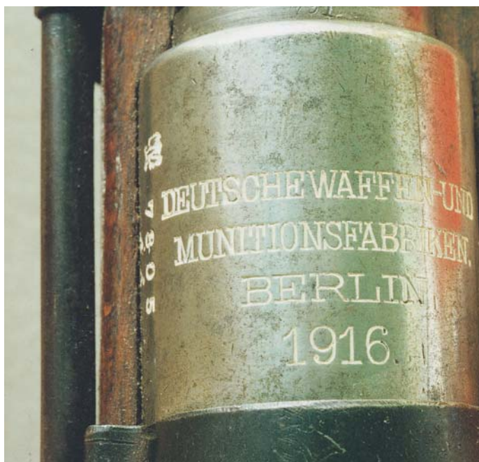
The receiver of the German Model 98 Rifle with sliding bolt cover (shown on previous page), showing how the forend of the bolt cover fits snugly up against the face of the receiver. This also illustrates how the bolt cover rides on a rod that is attached by a steel clip fitting just in front of the receiver.
