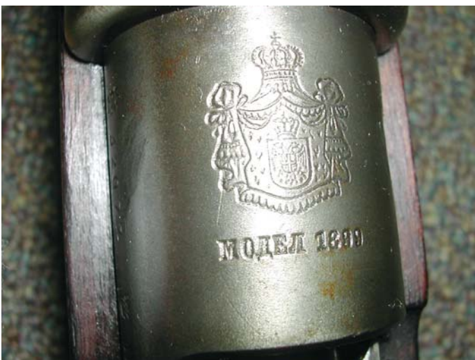
The Serbian Model 1899 receiver crest, one of 90,000 7mm Long Rifles made by DWM using the Mauser patented Model 1895 action, a variation of the Model 1893 updated to feature a round-bottom bolt face and a wide receiver tang which supports a third locking surface behind the bolt handle. The carbine version of this rifle was not made until 1908 when Steyr produced 10,000 M.1908 cavalry carbines. (U.S. Army Ordnance Museum Collection, Aberdeen Proving Ground, Md.)
