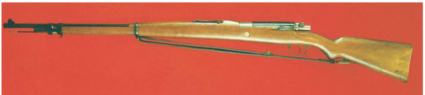
Left full-length view of the Manchurian Mauser Rifle. Note the streamlined appearance when the bolt cover is in place.
