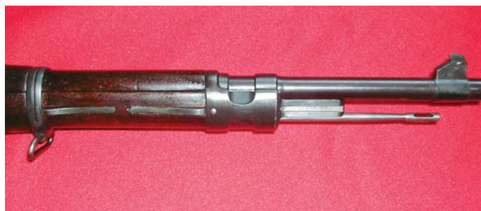
The front sight of the Iranian M1924 FN Contract Rifle is mounted on a barrel band, and features a full-length handguard. (John Wall collection)
