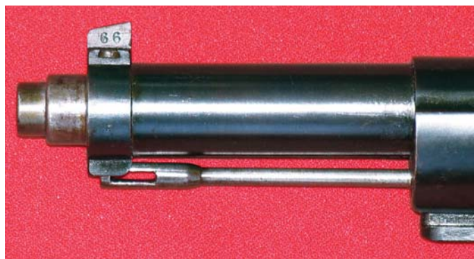
The muzzle, fore end and front sight of an MAE-made Belgian Model 1889 Long Rifle. Note that the last two digits of the rifle's serial number, "66" are also stamped on the front sight blade. (John Wall collection)
