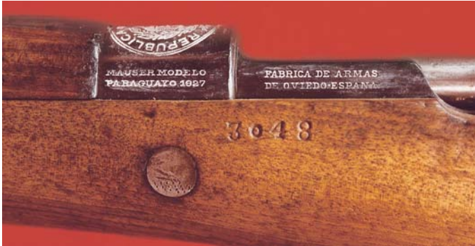
The left side of the receiver ring with model designation, and left side rail with manufacturer's markings of the Paraguayan Model 1927 Rifle.
