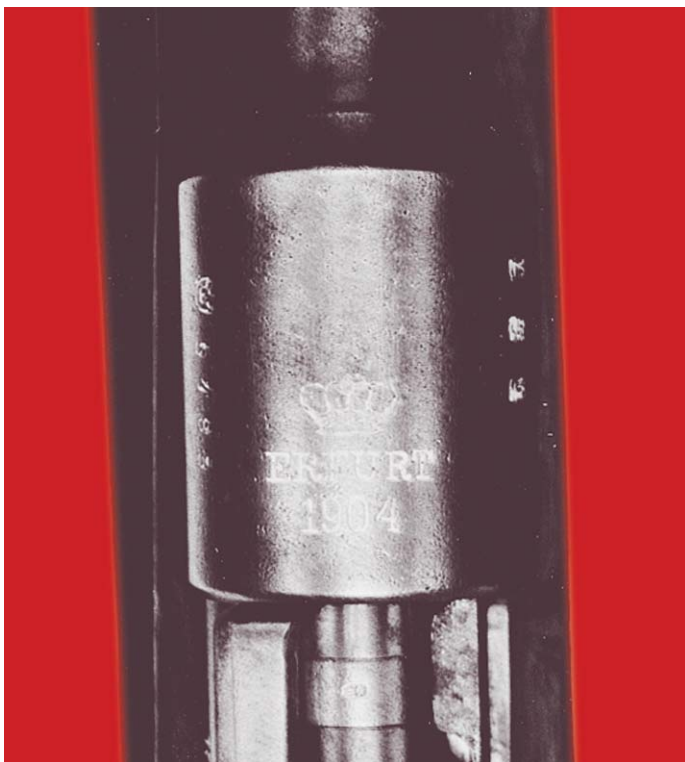
Crown/ERFURT/1904 markings on the receiver ring of the Model 98 Carbine, Second Pattern. (Robert Jensen collection)
