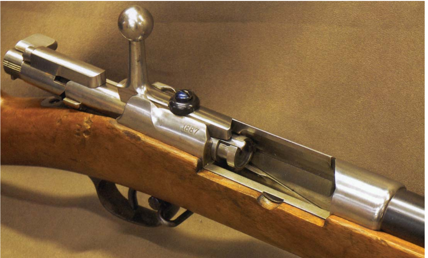
The open action of the prototype Turkish Mauser 9.5mm rifle. Note the position of the magazine elevator. (Private collection of Robert I. Landies)
