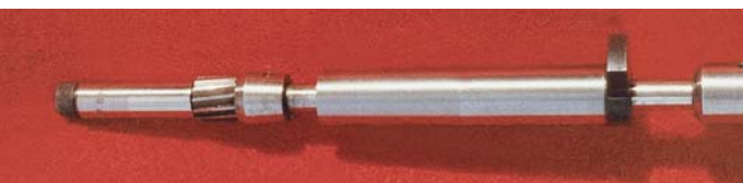
The reamer tip with pilot "7.89" in place. The black part to the right locks into locking lugs in the rifle receiver. (R. K. Smith collection)
