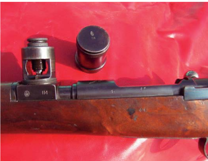
The test fixtures belonging to an Oviedo Pressure Test Rifle, manufactured circa 1913. (John Litt collection)
