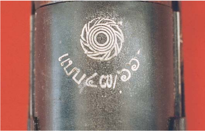
"Charkra" and model year in Siamese numerals on the receiver ring of the Siamese Model 1923 (Type 66) Short Rifle.
