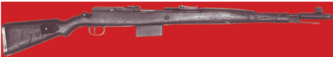
Right side view of the Gew 41M Semi-Automatic Rifle; note the bolt handle knob, as well as the awkward distance from the trigger guard to the fixed magazine. (Robert Jensen collection)
