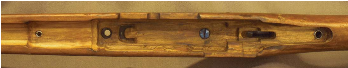
Intricacies of the inletting for inclusion of the tube magazine feed system in the Turkish Model 1887 prototype rifle. (Private collection of Robert I. Landies)
