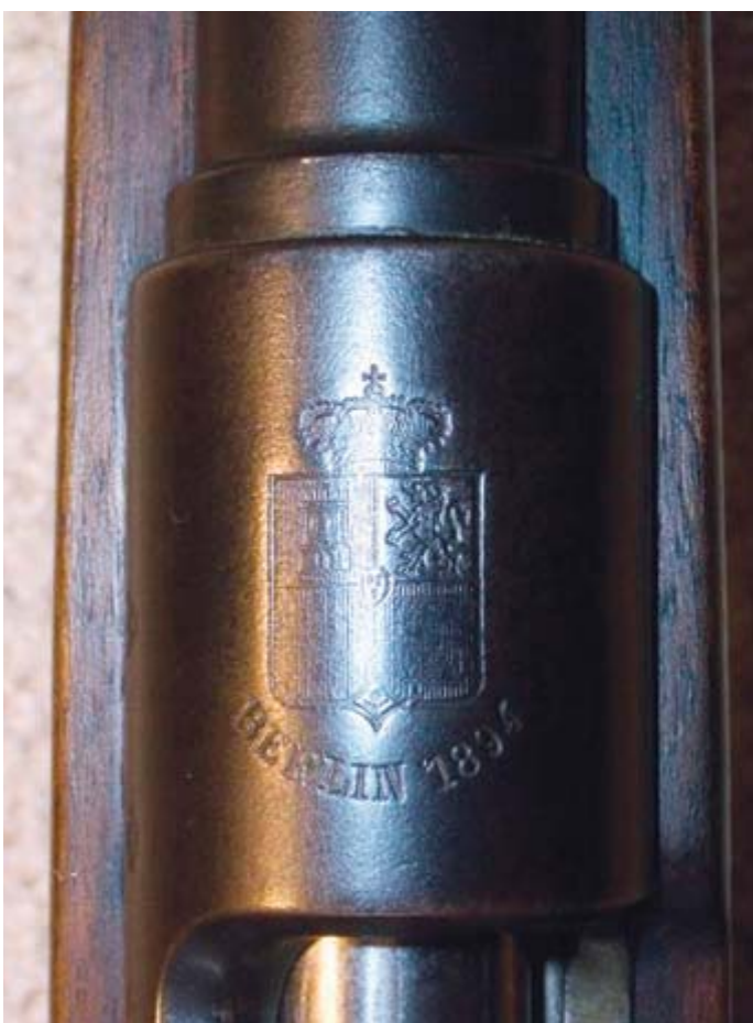
The Spanish royal coat of arms as it appears on the receiver ring of the Model 1891 Cavalry Carbine. The "Berlin 1894" inscription indicates the place where the Ludwig Loewe factory was located, as well as the year in which the carbine was manufactured. Later that same year, Spanish carbines using the Mauser Model 1893 bolt-action were also manufactured at Loewe's Berlin plant, so the same crest, city and year may also be found on the first production run of these carbines as well. (Hans-Joerg Meyer collection)
