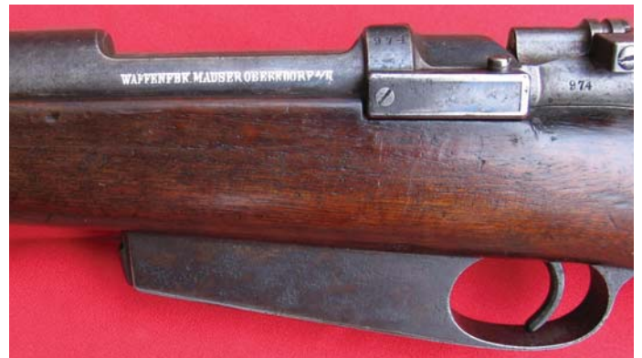
The left side of the Spanish Model 1892 Carbine, with the "Waffenfabrik Mauser a/N" address. The carbine must be disassembled in order to reveal the serial number "974," which is stamped on the receiver below the wood line. (John Wall collection)
