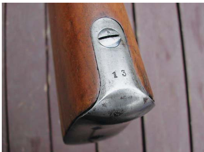
The tang of the buttplate of the 5.97 Test Rifle is the long type seen so often on the German Kar98 Carbine where it served as the location for the unit mark. Here the tang shows just the test rifle's serial number "13." (John Wall collection)
