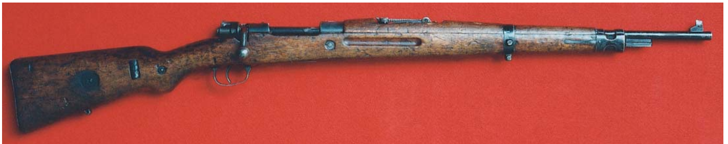
Full-length view of the Lithuanian FN Model 30 Short Rifle. Note that this version has the bent bolt handle. For some unknown reason, this specimen has a quick-release sling attachment on the right side of the stock, instead of on the left, as is usual. (Steve Kehaya collection)
