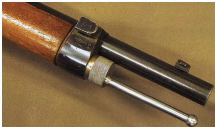
BELOW: Muzzle area showing magazine cap and stacking rod of the late production 71/84 rifle SN 17666. (Private collection of Robert I. Landies)
