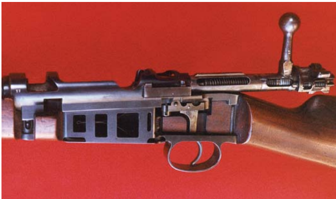
Close-up view of the left side of the Mexican Model 1910 Cut-away Rifle training aide, with the bolt open. (R. K. Smith collection)
