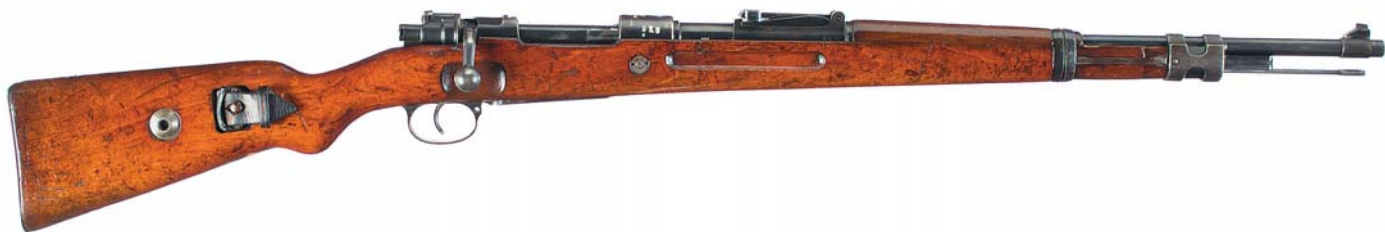
Right full-length view of an "SS" proofed K98k Short Rifle. This was a Gew 98 converted during the 1920s or 1930s. This is a late WWI production original issue 'SS' rifle. (Rock Island Auction Co.)
