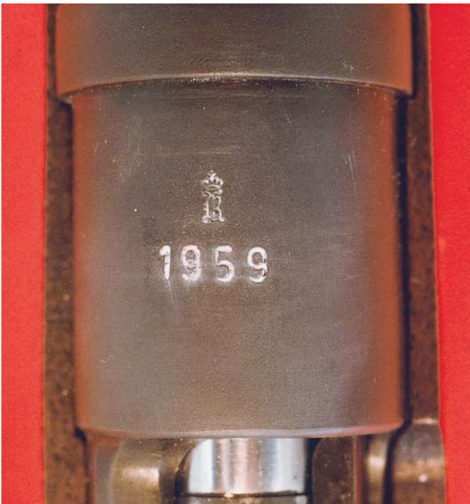
The receiver ring stampings on the Norwegian Army Target Rifle as modified from the Mauser K98k action.
