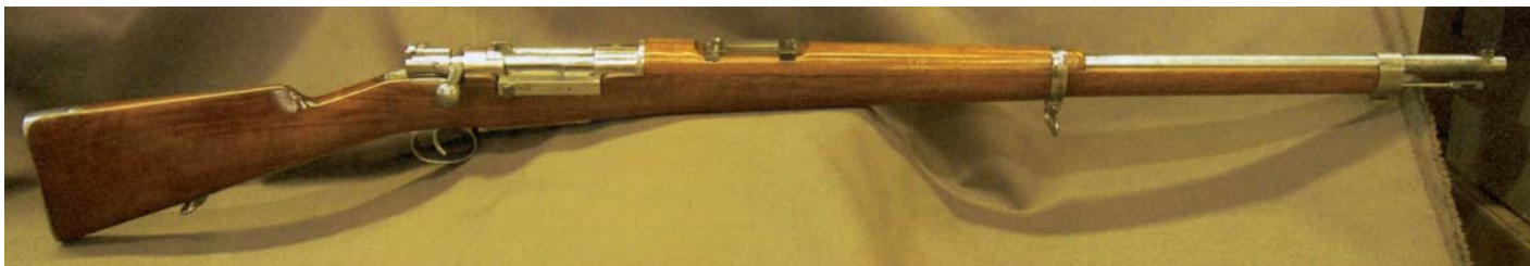
Mauser-manufactured Turkish Model 1893 7.65mm SN 111 rifle, nickel plated with magazine cutoff. This is one of 200 in the original contract for the Palace Guard of the Sultan of Turkey. (Private collection of Robert I. Landies)
