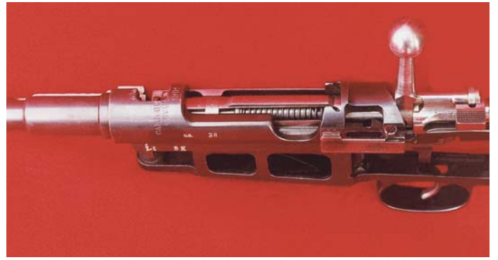
Left side, top view of Swedish M1896 barreled receiver cut-away. (R. K. Smith collection)
