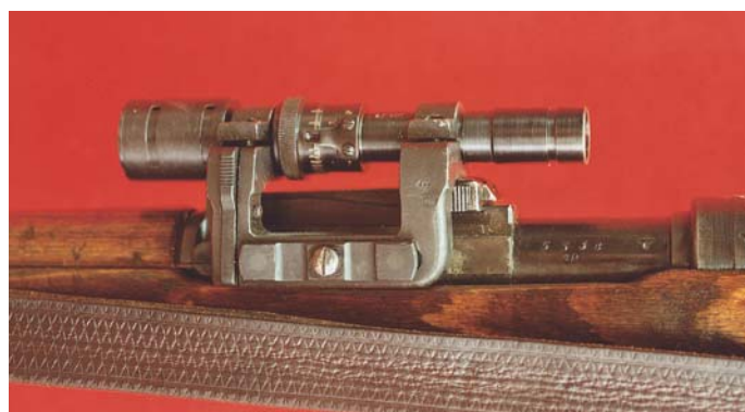
Close-up view of the left side of the mount and ZF-41 scope on the German Model 98k Carbine.
