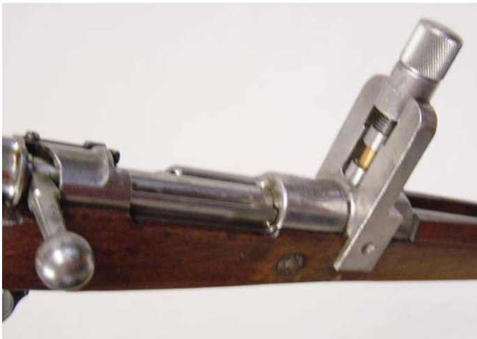
Chilean M1912 Pressure Test Rifle, close-up view of action. (Jan Gardiner collection)
