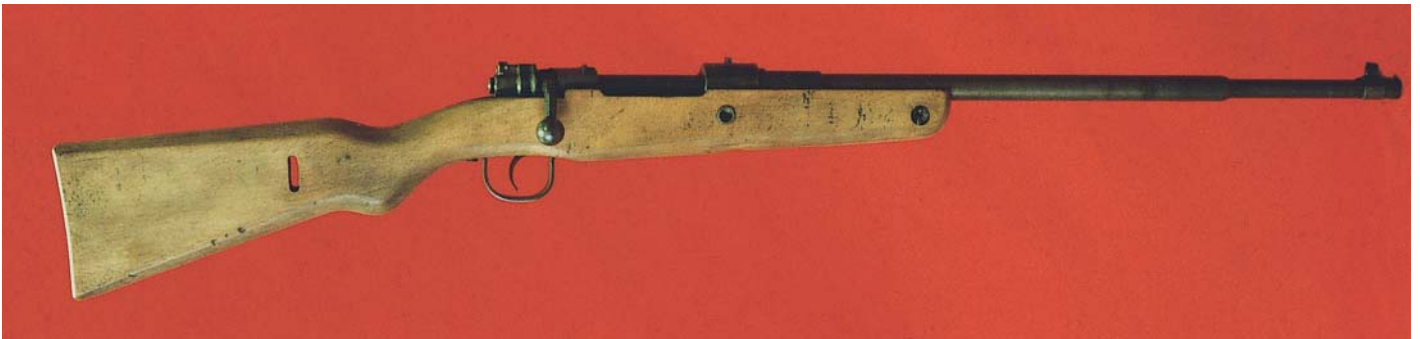
Full-length view of the German VK-98 Rifle. Note the fixed rear sight, the 5-shot internal magazine, and the machine gun barrel. This rifle is fitted with a buttplate and provision for a sling, with a swivel on the left front of the stock and a cut through the stock for a sling.
