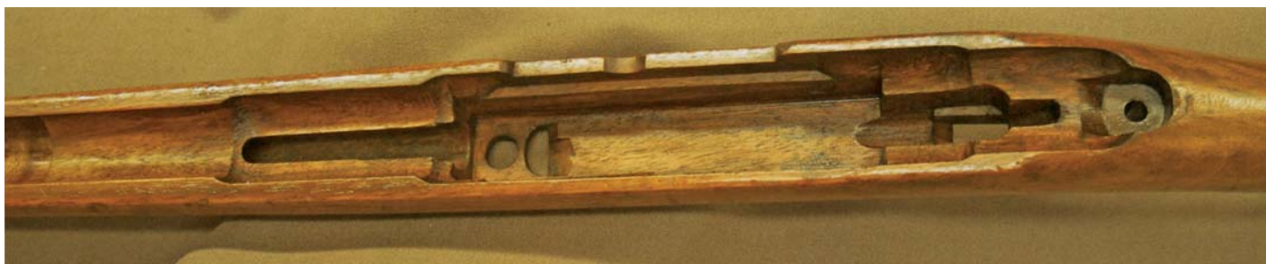
Standard Model 71 stock modified for tube feed. (Private collection of Robert I. Landies)
