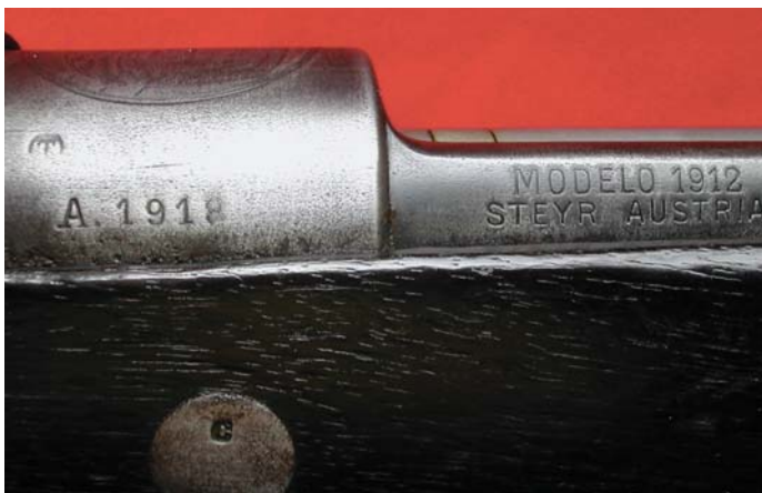
The side rail of the Colombian “Modelo 1912” Carbine made in Steyr Austria. Note the A.1918 serial number and the Steyr “T in a circle” proof mark partially visible above the serial number. (John Wall collection)
