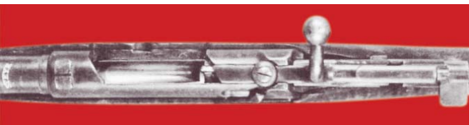
Top view of the Styer-made G 71/84 Short Rifle with the action open, showing the magazine ramp in the "up" position.
