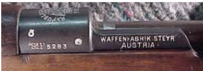
The Mexican Model 1912. This rifle is one of 70,000 Mexican M1912 long rifles made at Steyr in Austria that were brought into Austro-Hungarian Army service in 1914 as the "Repetiergewehr M.14 (Mexicanische)." Prior to issue to A/H troops, the receivers were blued. In Mexican service, the M1912 was issued with a bright, unblued receiver. (John Wall collection)
