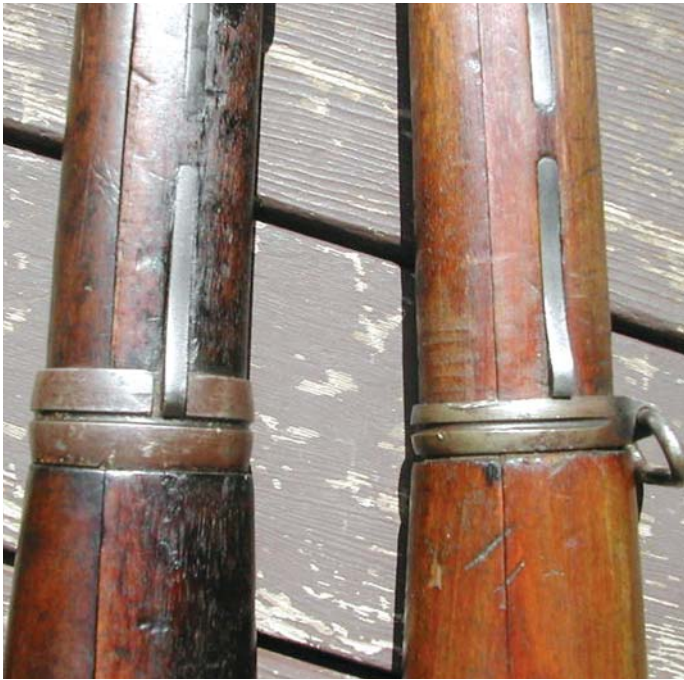
The German Army re-issued many Yugoslav M1924 Rifles which had been modified to accept their own Kar 98k sling. After they cut the sling slot in the buttstock, they removed the original upper sling band (right, above) and replaced it with a wider Kar 98k band with its side-mounted sling loop. The right side of the 98k band was then notched (above, left) to permit it to be re-installed on the M1924 with its original Yugoslav band spring still able to do its work of holding the band in place. (John Wall collection)
