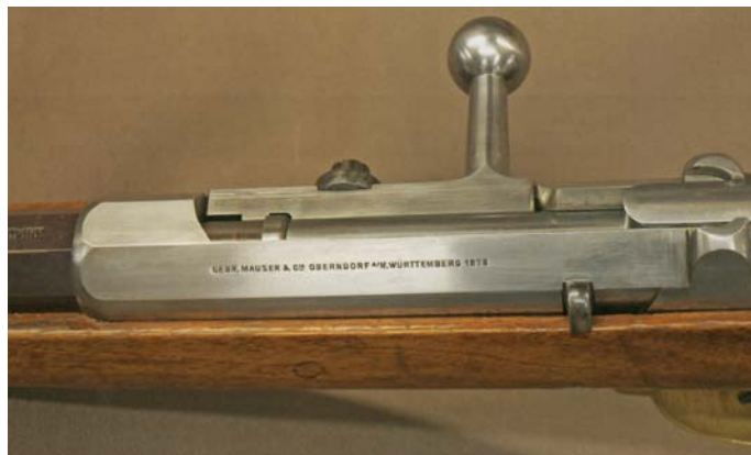
Left side view of 71/78 SN 14 prototype tube magazine fed 11mm rifle. (Private collection of Robert I. Landies)
