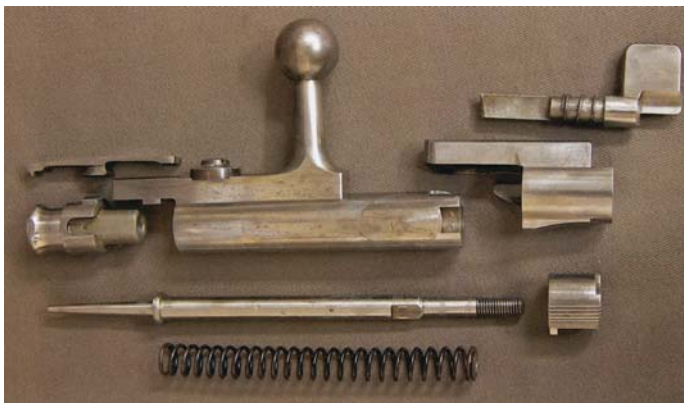
Model 78/80 Serbian contract pattern rifle bolt assembly, SN 6. (Private collection of Robert I. Landies)
