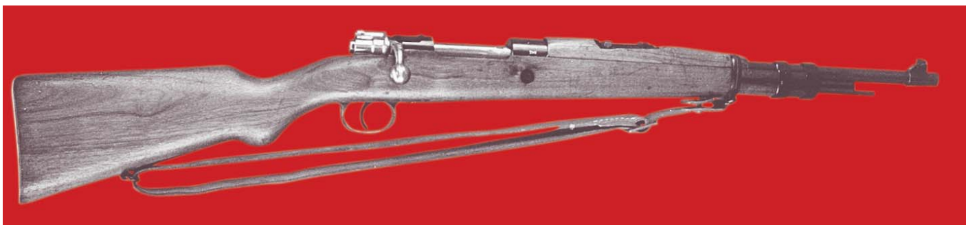
Full-length view of post-WWII FN-manufactured Carbine, possibly M1950. This carbine was produced in both .30-06 and .308 caliber, with all dimensions identical. It is believed, from what little information the author has been able to glean, that these carbines were used to arm the Moroccan gendarmerie. Information relative to these weapons is almost non-existent.
