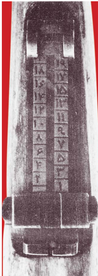
Rear sight with gradations marked in Farsi on the Persian Model 98/29 Long Rifle.
