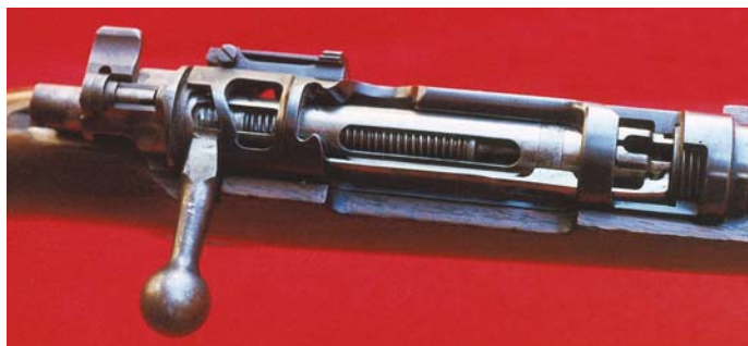
Mexican Model 1910 7mm Cut-away Rifle training aide. Close-up top right-hand view of the action. (R. K. Smith collection)
