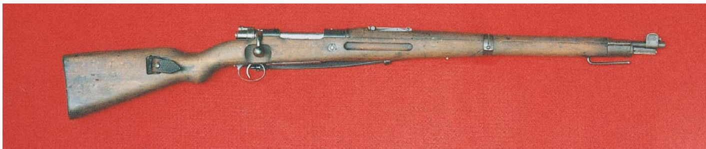
Full-length view of the post-1915 German Model 98AZ (98a) Carbine, with grasping grooves.
