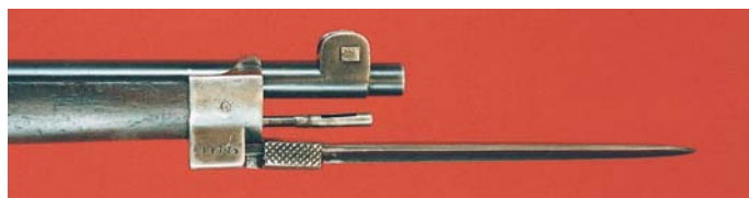
Close-up side view of the folding bayonet on the Turkish Model 38 Short Rifle.
