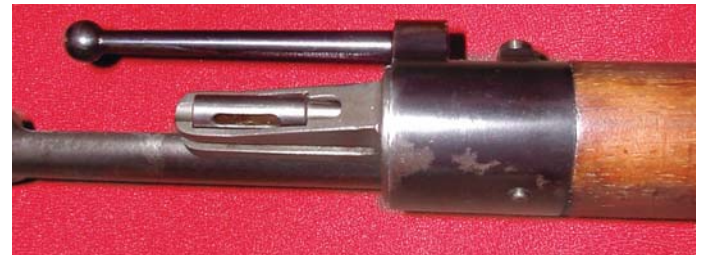
The view beneath the muzzle showing the stacking bar and the protected cleaning rod near the muzzle of the Steyr-made Mauser 98 experimental short rifle. (U.S. Army Ordnance Museum collection, Aberdeen Proving Grounds, Md.)
