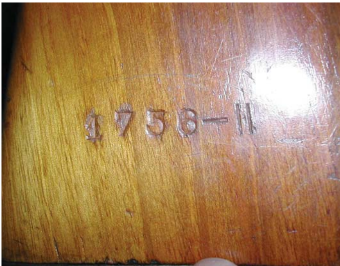
The buttstocks of Yugoslav M1924 Rifles made at Kragujevac Armory were numbered on the left side of the stock flat, about two inches above the buttplate. (John Wall collection)
