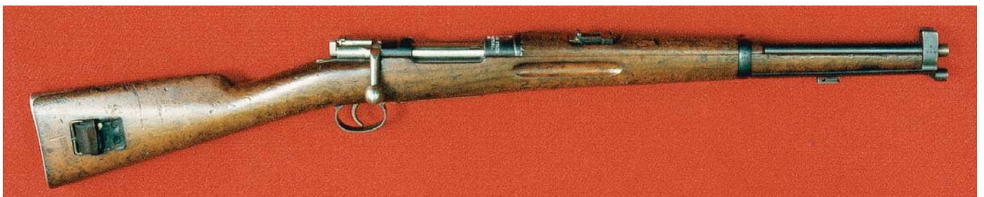
Full-length view of the Swedish Model 1894 Carbine as modified in 1917 by the addition of a bayonet lug. (Lothar Frank collection)
