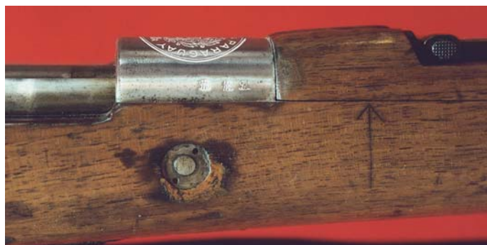
Right side of the receiver ring of the Paraguayan Model 1907 Carbine, showing proof marks. (Noel P. Schott collection)
