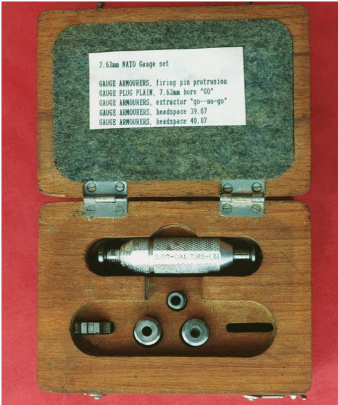
Israeli Armourer's Gauge Set, showing the open box with its tools. (R. K. Smith collection)
