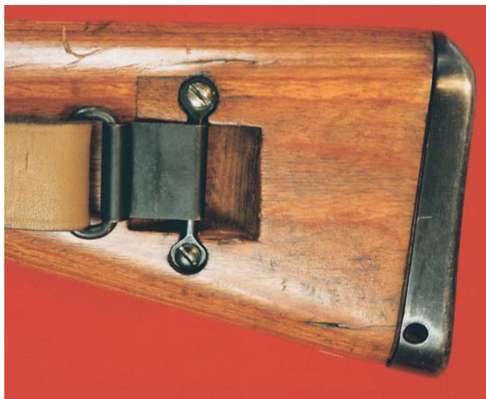
The left side of the buttstock of the French Model 98k Carbine, showing the crude bar-and-screws sling attachment. Note the hole in the buttplate for dismounting of the firing pin.
