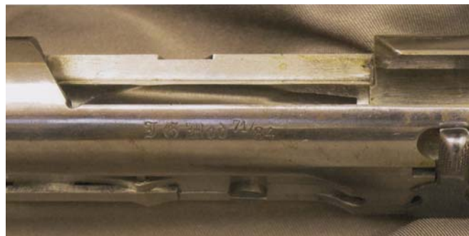
RIGHT: Barreled action of the Model 71/84 late production model 11mm, SN 17666, with second locking lug. Note the additional locking lug slot in the receiver. (Private collection of Robert I. Landies)
