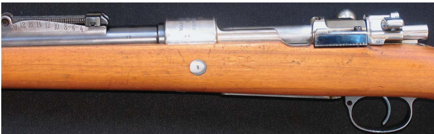
A close-up of the Mauser Model 1898 5.97mm Test Rifle. Note the use of the Mauser patented Model 1896 rear sight assembly which persisted on military bolt action rifles well into the 1960s. Note that this rifle has no visible proof marks, neither commercial nor military, and is serial number 13. (John Wall collection)
