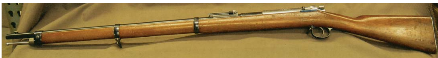
ABOVE: Left side view of Model 71/84 late production model 11mm, SN 17666, with second locking lug. (Private collection of Robert I. Landies)
