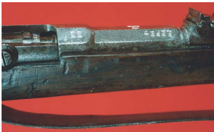
Proof markings on the right side of the chamber of the German Model 71 Rifle.
