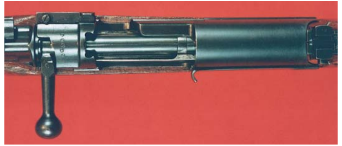
Full view of the action with open bolt cover of the Siamese Model 1923 (Type 66) Short Rifle.
