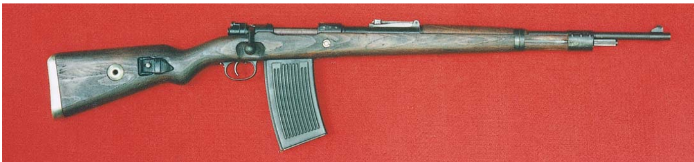
Full-length view of a German Model 98k Carbine equipped with an integral box magazine giving a 25-round capacity to the weapon. This carbine was captured on the Russian front, arsenal refinished, put into arsenal storage, and later shipped to Vietnam where it was used by the Viet Cong. This was its condition when captured, so one assumption is that the magazine, which is permanently attached to the trigger guard, was affixed experimentally by the Germans. It is also possible that this was done post WWII by the Czechs.
