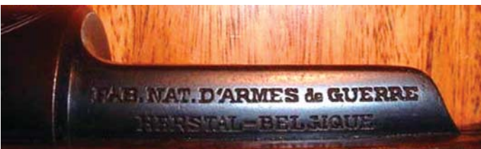
The side rail of the FN Model 1930 Short Rifle made for Paraguay. Note the use of a text font with serifs, typical of FN receiver side rail markings in the 1920s and 1930s.
