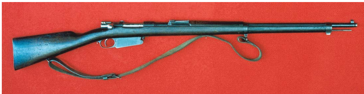
Full-length view of the Bolivian Modelo 1895 version of the Argentine Modelo 1891 Rifle.
