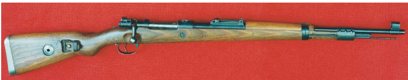
Full-length view of a late-war German Model 98k Carbine, FN manufacture. Note the laminated stock, the crude bands, and cupped buttplate.
