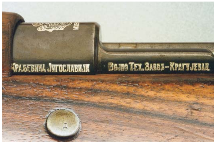
Manufacturer's markings stamped into the left side of the receiver and the left side rail of the Yugoslavian Model 24 Short Rifle.
