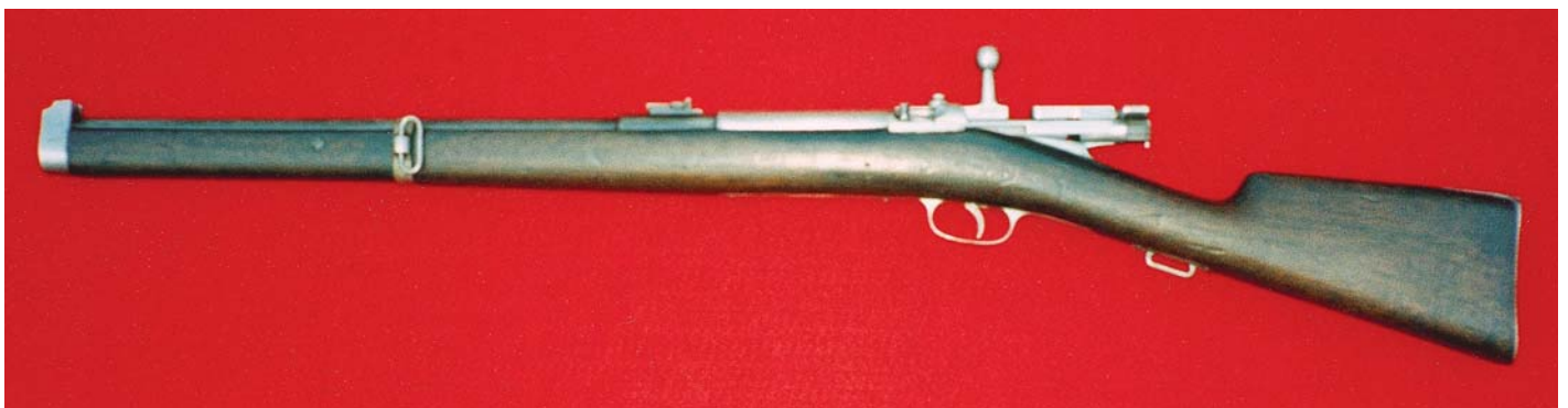
Left side view of the Serbian Mauser "Koka" Carbine with the bolt withdrawn; this shows the support to the bolt of the receiver extension. (John Sheehan collection)
