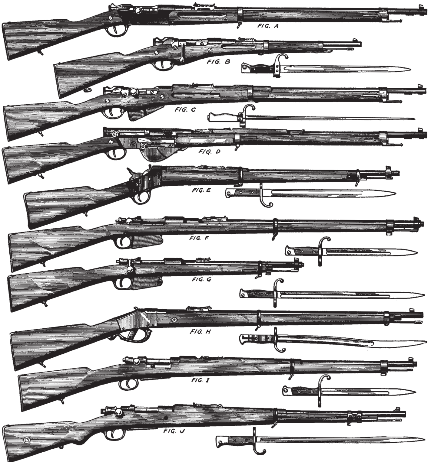
FIG. A. (FRANCE) LEBEL, MAGAZINE RIFLE, MODEL OF 1886. This weapon is distinguished by the fact that it was the first small-bore (8 m/m.) ever used and also, the first to use smokeless powder. The French were evidently satisfied with the two innovations for the arm remains unchanged today. The magazine, holding eight shells, lies in under the barrel, being simply a hole bored in the fore-end, the cartridges being fed into the magazine by the action of a long spiral spring. The Lebel is the standard arm of the French Army, it takes the bayonet shown between Figs. C and D.
