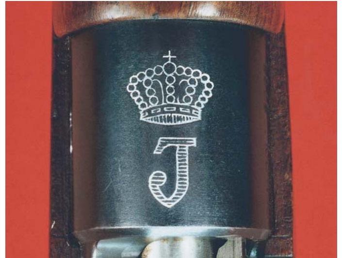
The receiver ring of the Dutch FN Model 1948 Carbine, showing the crest "J" for "Juliana." (Cliff Baumann collection)
