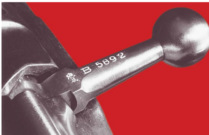
View of the German military quality inspection mark on the root of the bolt handle, with the serial number on the bolt handle of the M1896 ZAR Mauser Rifle. (John Wall collection, photo by John M. Leone)
