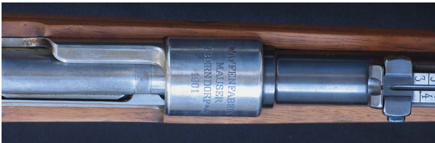
The receiver ring and sight leaf of the Model 1898 Mauser Test Rifle in 5.97mm (6mm) made at Oberndorf in 1901. (John Wall collection)
