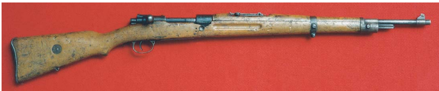
Full-length view of the unaltered Colombian Model 29 Rifle, redesignated the Model 29/40 as issued to the Luftwaffe. Note the sharp point to the pistol grip, the Austrian-style lower and upper bands held by screws, and the deeply cupped ends of the recoil crossbolt. This specimen has unfortunately lost a piece of the stock at the right side of the receiver ring. (Century International Arms, Inc.)
