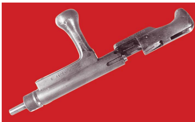
Figure 1.3 Details of the Chassepot Rifle bolt. The cocking piece has been retracted and rotated off-center to expose the three grooves on the bolt that retain it in a specific configuration (safe, half-cock, or fire).
