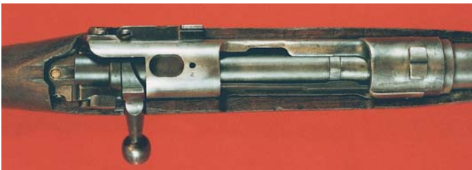
Top view of the action of the Hybrid Short Rifle built on the action of the Model 1917 Enfield.
