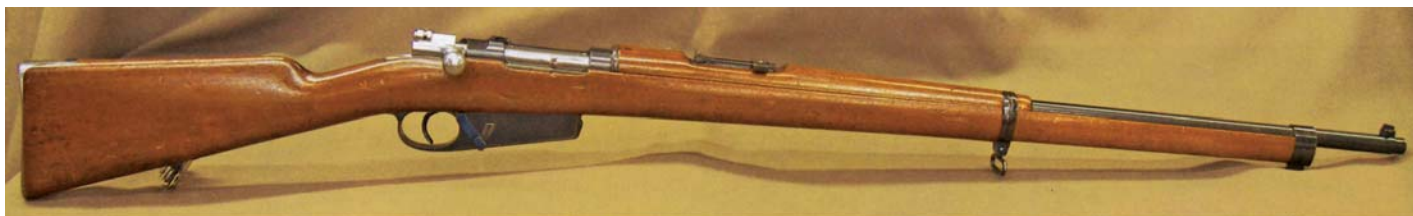
Mauser prototype Spanish Model 1892, SN 2, 7mm 2-position magazine cutoff. (Private collection of Robert I. Landies)
