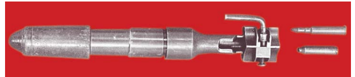
The grenade launcher for use with the German Model 98k Carbine, shown here with two propelling cartridges of differing strength, as well as the shaped-charge, armor piercing rifle grenade shown mated to the barrel of the launcher. (Henry Wichmann collection)
