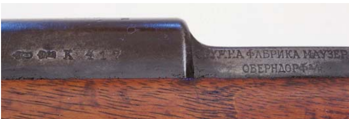
The left side of the receiver ring and side rail of the Serbian Model 1910 Short Rifle. Note the Mauser Oberndorf address in Cyrillic on the side rail and “B” and “U” proof marks. (David Jonas collection)
