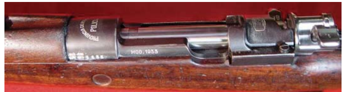
Left-side view of the receiver and side rail of the Argentine Model 1933 Short Rifle, showing the model number and part of the crest markings.
