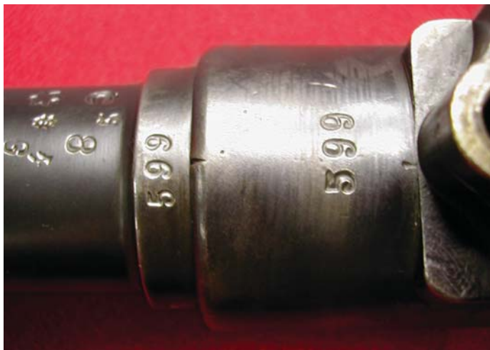
The underside of the 7.65mm M1892 Rifle at the U.S. Army Ordnance Museum. The serial number shown above, number 599, is stamped on the underside of both the receiver and the barrel, but is not visible on the assembled rifle. (U.S. Army Ordnance Museum, Aberdeen Proving Ground, Md.)
