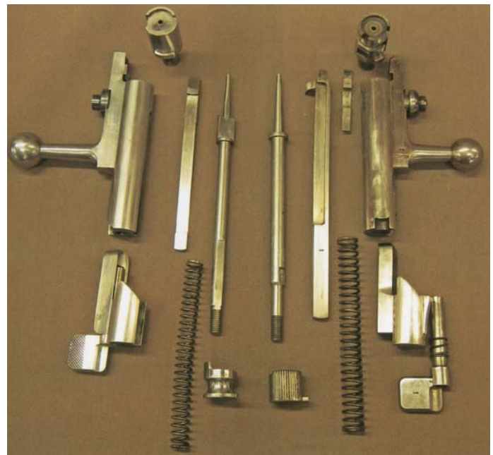
Comparison of the 71/78 bolt components to the 71/84 bolt, SN 1. (Private collection of Robert I. Landies)
