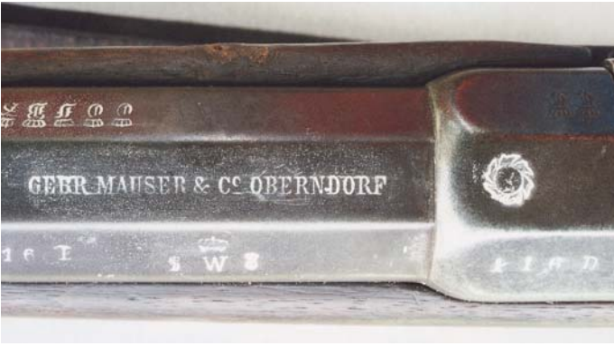
Siamese "Charkra" and manufacturer's markings and proofs on the receiver ring and barrel of the Siamese Model G 71 Rifle.
