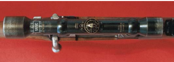
Top view of the Argentine Modelo 1909 Sniper Rifle; note the marking "Ejercito Argentino" over the scope number at the forward end of the barrel. The number visible at the rear of the scope is a collection identification number.
