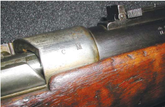
The right side of the receiver ring and rear sight of the Serbian Model 1884 Artillery Carbine. (From the former Pattern Room Collection now in the Royal Armouries Museum, Leeds, England)
