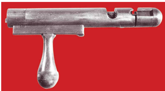
Figure 5.3 Mauser Rifle, Interim Model 1869/70 First Model. Details of the bolt.
