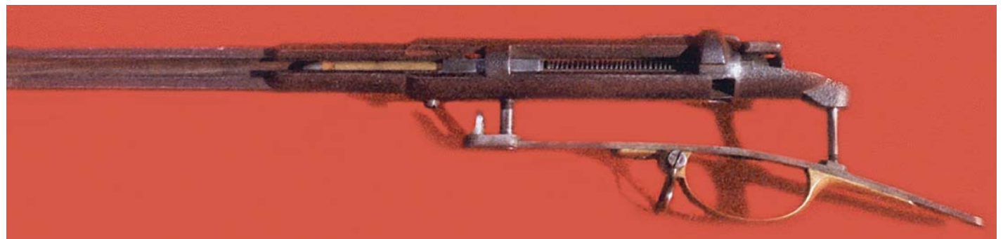
Left side view of barreled receiver cut-away M1871 Rifle, the barrel marked "AMBERG." (R. K. Smith collection)
