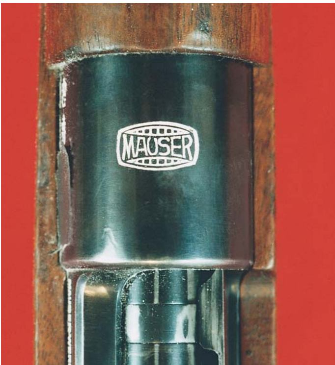
The receiver ring of the Standard Modell Model 1933 Carbine, showing the Mauser Banner legend.
