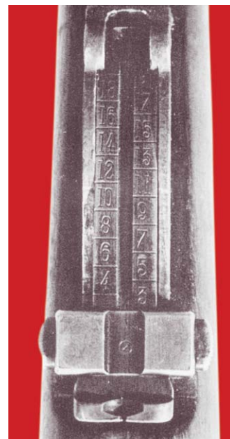
Rear sight leaf with Arabic numerals on the Czech Model 98/22 Rifle used by Turkey.
