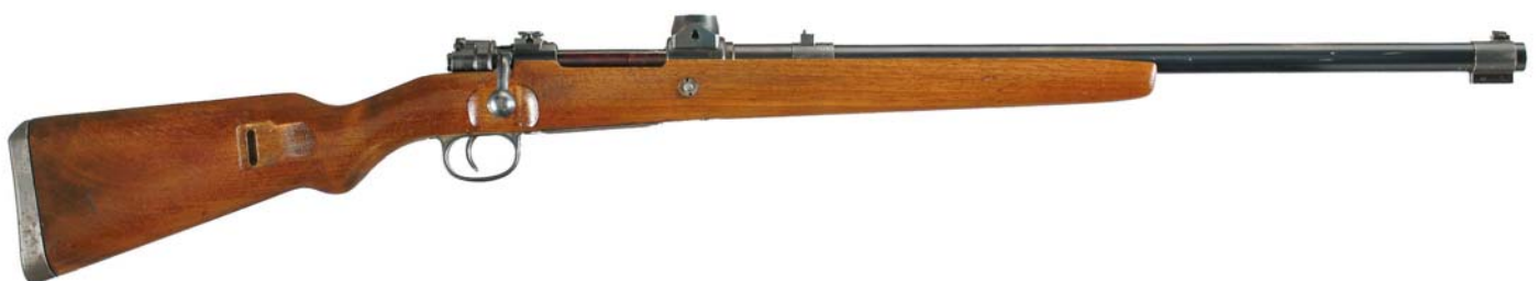
Right side view of rare German Mauser K98k Ammunition Test Rifle, with high-turret scope bases and a special heavy barrel. Note the removable iron sights clamped to the underside of the barrel. (Rock Island Auction Co.)
