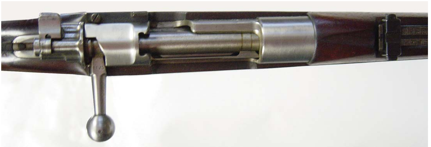
Brazilian M1908 Mauser Rifle, 8x57 J. Overhead view of the action. (Jan Gardiner collection)
