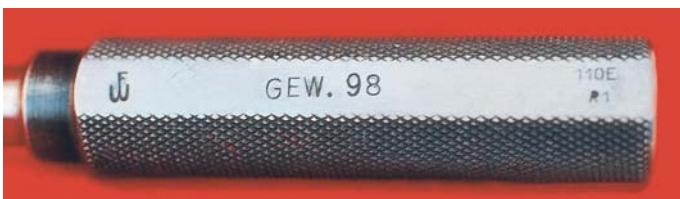
Close-up view of the handle included in the bore reaming kit, with proof, GEW. 98 and 110E/RI. (R. K. Smith collection)
