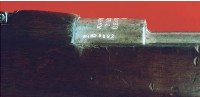
Left side of the receiver of the Siamese Model 1904 Rifle, showing the weapon serial number and the proof marks. (Noel P. Schott collection)
