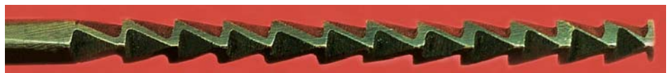
Mauser Banner Cleaning Rod. Made of .323 diameter brass, the overall length of the rod is 45.25 inches, while the rod length is 36.25"; the wooden handle is 9", and the saw tip blade is 4". The wood handle is long enough to allow use of both hands, and the spacer could be used to adjust for different length barrels. It is the owner's thought that this is a post-WWI item when Mauser was making everything except guns. The Mauser Banner Cleaning Rod shown here has a large wood handle with adjustable keeper. Note Mauser Banner in upper corner of handle. (R. K. Smith collection)
