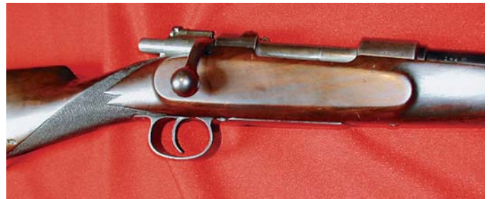
The receiver and action of a Model 1893 Mauser built as a Sporting Rifle by DWM for the South African market. note the turned-down bolt, the extra wood around the receiver, the straight-grip stock (many "Plezier" or sporting Mausers had pistol-grip stocks) and the typical action normally found on military M1893 carbines. (John Wall collection)
