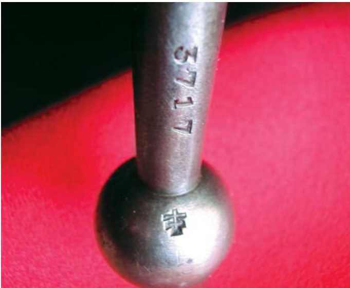
The bolt handle and knob on the Slovak VZ 24 Service Rifle also features the double-barred crucifix. On Czechoslovak VZ 24s, circa 1924-1939, this mark had been a small rampant lion stamp. (John Wall collection)
