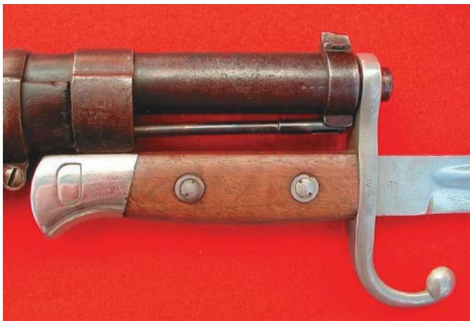
The Mounted Gendarmerie Carbine has a lower band mounted a scant 1" below the top band. This view shows both upper bands with the bayonet mounted on the carbine. This model is extremely rare. (John Sheehan collection)
