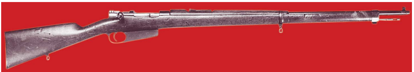
Right side view of an experimental Model rifle. This Mauser Model 1892-93 Experimental Rifle was manufactured in an unknown caliber 6.5mm, and has no markings whatsoever other than the serial number. The rifle has the standard fixed magazine, without a follower stop, and the action cocks on closing. The sights are adjustable from 500 to 2000 meters. The rifle weighs 8.11 lbs., with a barrel length of 29.125" and an overall length of 49.875". (John Wall collection)
