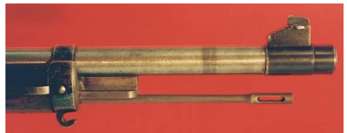
The muzzle and forend of the German Model 1904 "Salesman's Sample" Export Rifle, showing the short, simple upper band and the "T" shaped bayonet lug.
