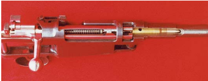
Right side, bolt closed view of the Swedish M1896 barreled receiver cut-away rifle. (R. K. Smith collection)
