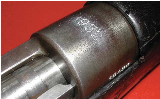
The “1932” receiver date crest of an FN-made 7.9mm Model 1924 Mauser Short Rifle made for China. As with all other known Mausers made by FN in the 1920s (China, Mexico, Brazil) this Model 1924 is characterized by an intermediate length receiver. Only this Chinese purchase and a small Iranian contract are believed to have occurred in the 1930s, when FN began producing their Model 1930 which featured a standard length receiver. (John Wall collection)
