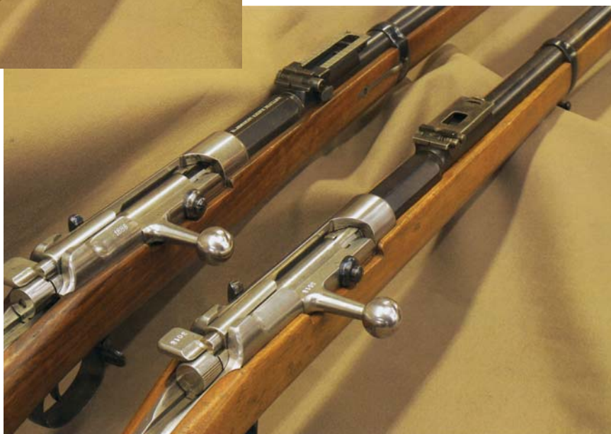
Close-up comparison of the 71/84 standard rifle to the 71/84 Jager rifle, with rear sight raised. (Private collection of Robert I. Landies)
