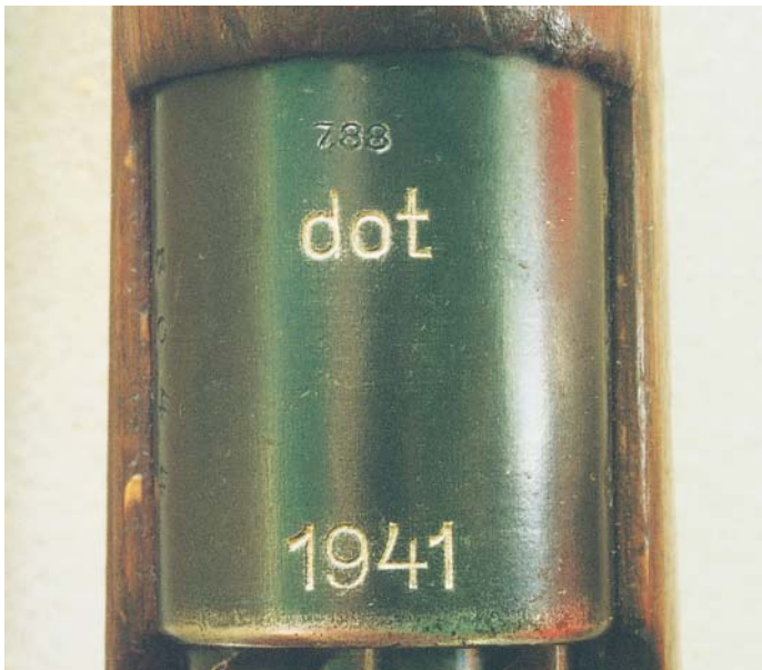
The receiver ring of the German Model 33/40 Carbine, showing the manufacturer's code over the date of manufacture.
