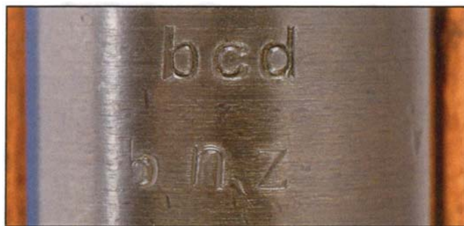
Close-up view of the receiver ring of dual-coded rifle, showing "bcd/bnz." (Rock Island Auction Co.)
