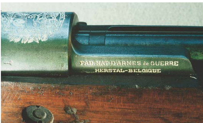
Manufacturer's markings stamped into the left side rail of the Venezuelan FN Model 24/30 Short Rifle.
