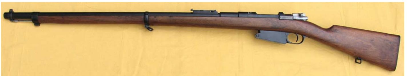
The Belgian Model 1889 Heavy Barrel Rifle. The illustrated example has no stock cartouches, and lacks the muzzle protrusion that holds a bayonet-locking ring. The factory finish on the heavy-barrel Model 1889 is black enamel, suggesting that it was made in the 1920s or 1930s. No record of rifles of this type has yet been uncovered in Belgium, so its tactical purpose, if any, is unknown. (John Wall collection)
