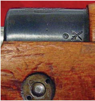
The right side of the receiver of the Teheran-manufactured Model 1309 (Model 98/29) Long Rifle. (Darryl Beck collection)
