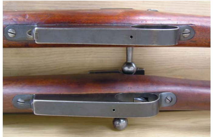
A comparative view of the M1892 Swedish Trials Long Rifle (below) and Carbine (above) showing the un-numbered bottom of both magazine assemblies, and a drain hole. The one observed Spanish Model 1892 also has the drain hole, but does have a serial number stamped on the bottom of the magazine assembly. (Jorma Seppanen collection)
