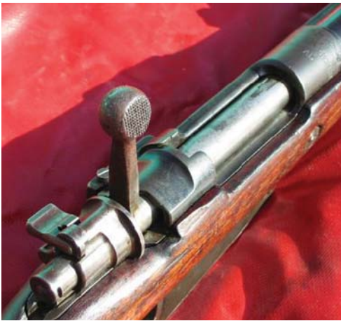
The action of the Pieper Model 1889/36 conversion. Note the checkered surface of the underside of the bolt handle, indicating that the bolt had originally been a turned down bolt for a Model 1889 Carbine, which Pieper straightened for the conversion. (John Litt collection)
