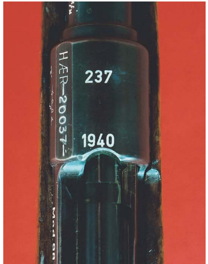
Receiver markings on the Norwegian Reissue Model K98k Carbine. Note how the face of the receiver has been milled to accept a different size cartridge. (Bob Bennett collection)
