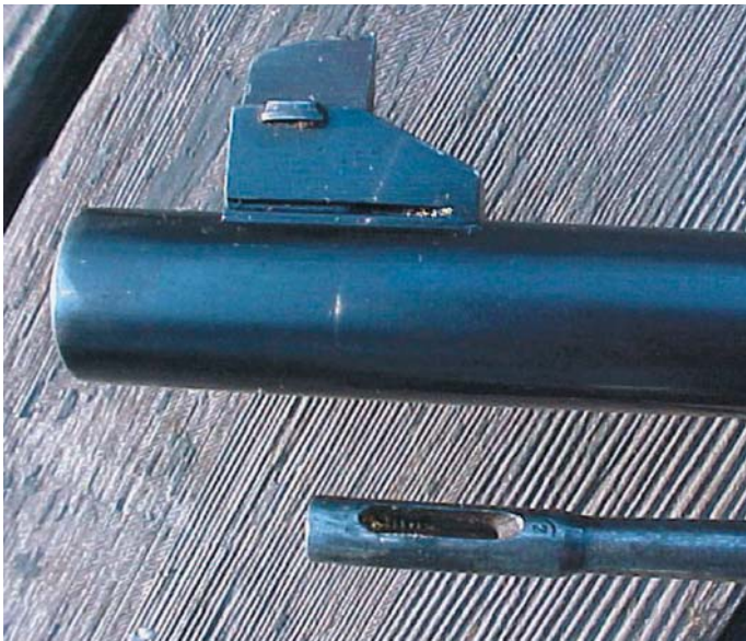
The front sight of a VZ 23 Czechoslovak Army Short Rifle. The VZ 23 featured a highly distinct slot for a sight hood cut in its sight base. Note that the rear of the slot is deeper than its front. VZ 23 sight hoods themselves are extremely rare. When transitional production of the VZ 24 began in 1924, this slot and its hood were some of the first features of the VZ 23 to be eliminated. (John Wall collection)
