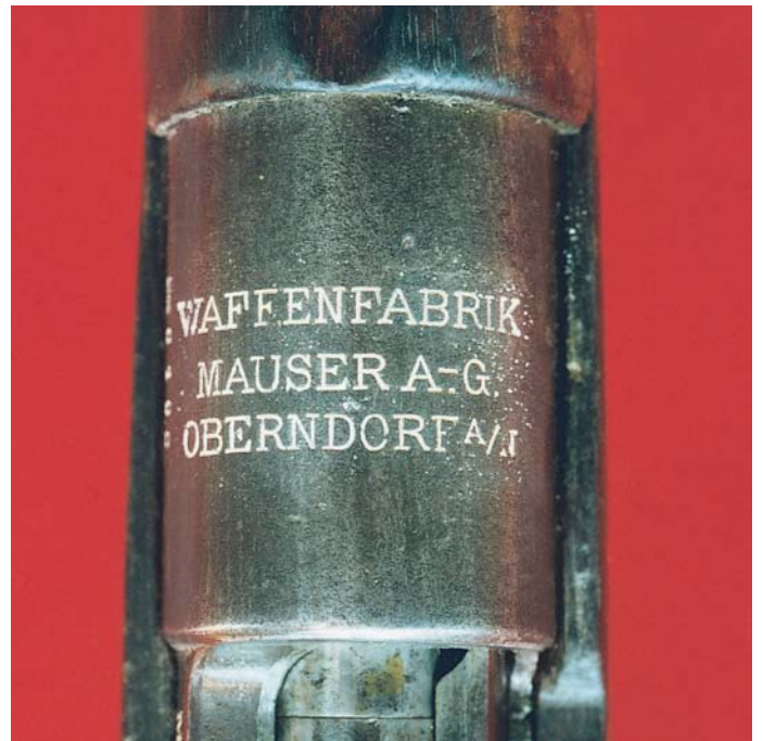
The receiver ring of the Costa Rican Model 1910 Rifle. This particular specimen has the Waffenfabrik Mauser Oberndorf markings instead of the Costa Rican national crest.
