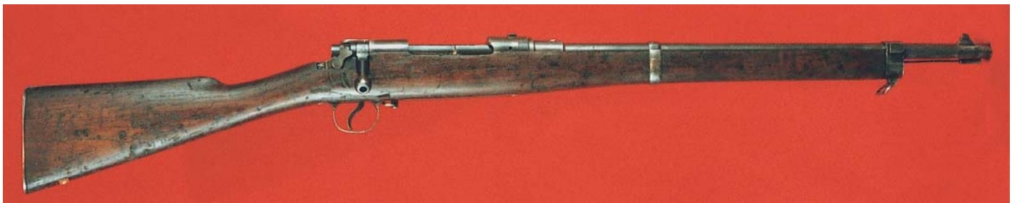
Full-length view of the Hybrid Short Rifle built on a Model 1917 Enfield action with a Steyr barrel.
