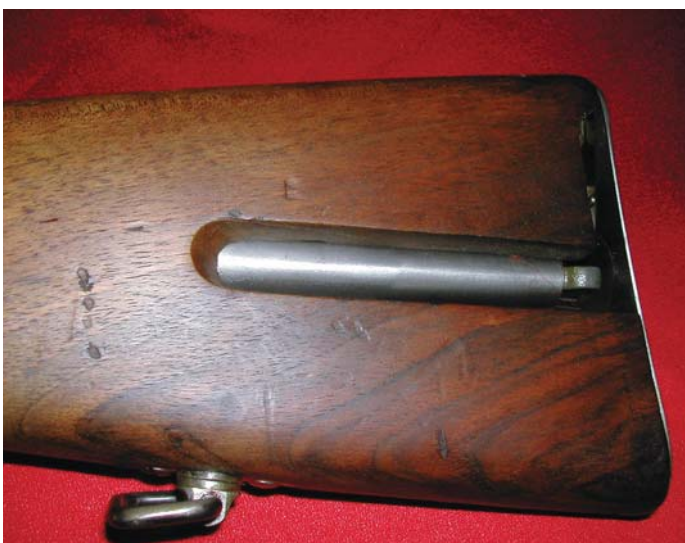
Cut-away buttstock of the Steyr-made Mauser 98 experimental Mauser Short Rifle, showing a cleaning kit accessible through a butt trap. Note the large sling swivel, used earlier on certain Austro-Hungarian M.95 straight pull carbines and the Czechoslovak VZ.23. (U.S. Army Ordnance Museum collection, Aberdeen Proving Grounds, Md.)
