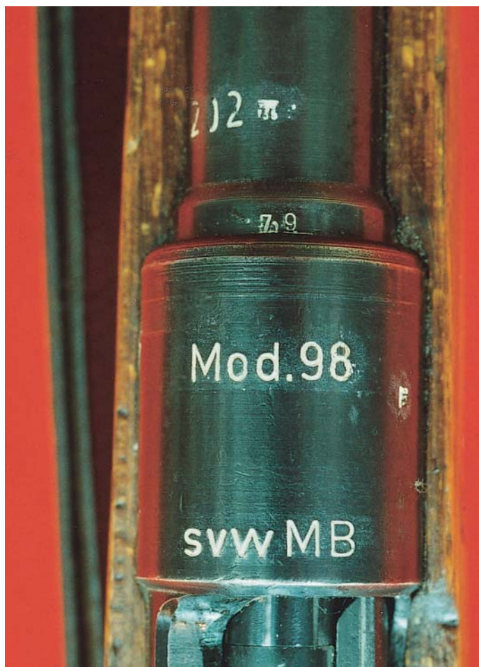
The left side of the receiver ring with serial number and "star" French proof mark for an arm of foreign origin of the French-modified German 98k Carbine. (Bob Bennett collection)
