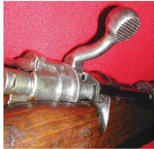
The underside of the M1924 Yugoslav Mauser Cavalry Carbine reveals its unusual shape, stock groove and knurled grasping surface. The rifle's stock bears the cartouche of King Peter II, indicating that it was made between 1934 and 1941. (John Wall collection)
