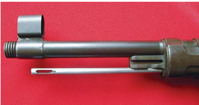
The Brazilian M954 (Model 1954), an updated version of the Czechoslovak-made Brazilian 1908/34 Carbine, is distinctive for its incorporation of several features from German WWII arms. The muzzle area, shown above, features a slotted front sight base that accommodates a German-type 98Kk sight hood. Additionally, the muzzle is threaded for what is assumed to be a grenade launcher and/or muzzle brake. The finish has been changed from bluing to a dark, olive colored Parkerizing. (John Wall collection)
