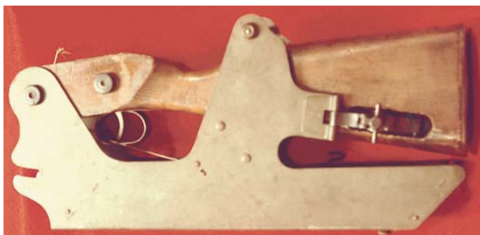
Left side view of the German Trench Rifle-firing Device in the folded, carrying position. Note how the rifle clamping attachment is housed in the cutout on the left side of the auxiliary stock.
