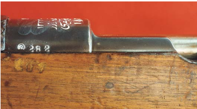
Left side view of the Yugoslavian Model 03(T) Short Rifle, showing the new serial number on the side of the receiver ring. (Noel P. Schott collection)
