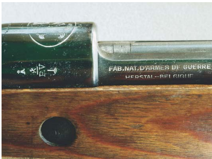
Side view of the receiver area of the FN-made German Model 98k Carbine, showing the original FN markings on the side rail and the Belgian proofing on the side of the receiver ring.
