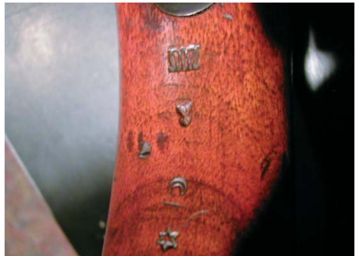
The area beneath the stock’s wrist of the M1903 Customs Administration Rifle was the site of many inspection marks and cartouches seen on most Ottoman Mausers. The upper stamp is the intertwined letters “W” and “M” of “Waffenfabrik Mauser.” (U.S. Army Ordnance Museum, Aberdeen Proving Ground, Md.)
