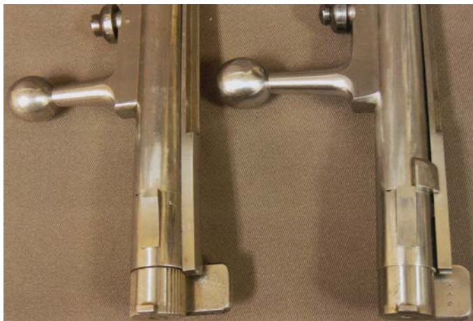
Two-thirds view of the Model 71/84 First Model bolt, SN 1 compared to 71/84 Late Model bolt showing no splines on firing pin retainer. (Private collection of Robert I. Landies)
