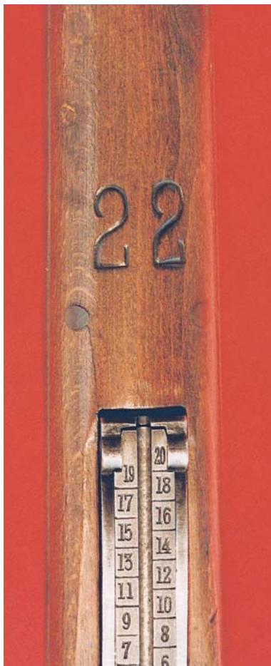
Twenty-two caliber designation burned into the upper hand guard of the Polish Model Wz 29 Training Short Rifle.
