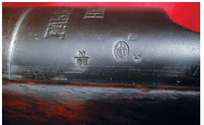
The left side of the receiver of the Model 1889 Gendarmes Carbine showing the "EGB" Belgian Government proof mark, in addition to earlier proof marks which appear to have been partially removed, perhaps during a conversion process. (John Wall collection)
