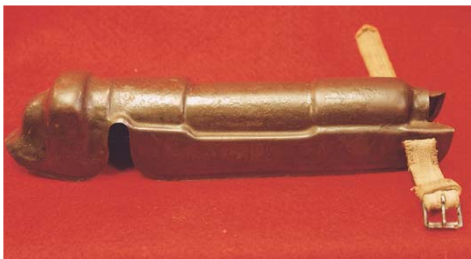
Right side view of the German Model G 98 Rifle action cover, showing the slot for the bolt handle and the cloth strap and buckle.
