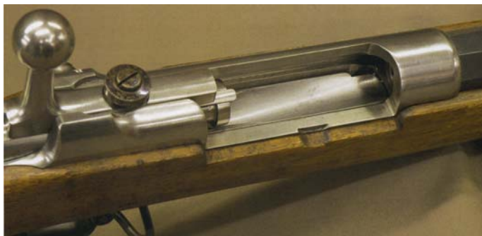
ABOVE: Left rear close-up of the 71/82 bolt showing bolt root, cocking piece and rear of extractor. (Private collection of Robert I. Landies)
