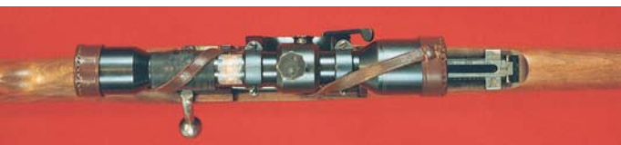
Top view of the scope and action of the Swedish Model 1896 Sniper Rifle fitted with the Model 41 AGA scope.
