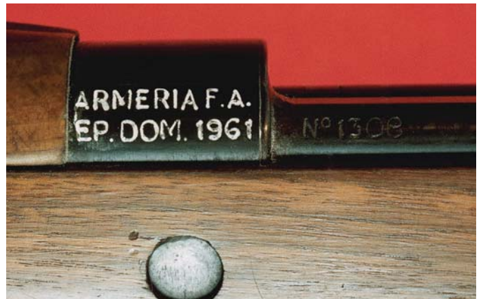
Stampings on the left side of the receiver ring of the Dominican Republic Model 1953 Rifle.
