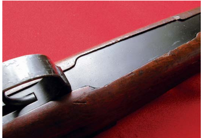
The flat single piece side plate covering the area which on the standard large bore Model 1924 Mauser Service Rifle accommodates the five round magazine. On .22 caliber training rifles, the plate simply covers stock wood since this trainer is single shot and has no magazine well. (John Wall collection)
