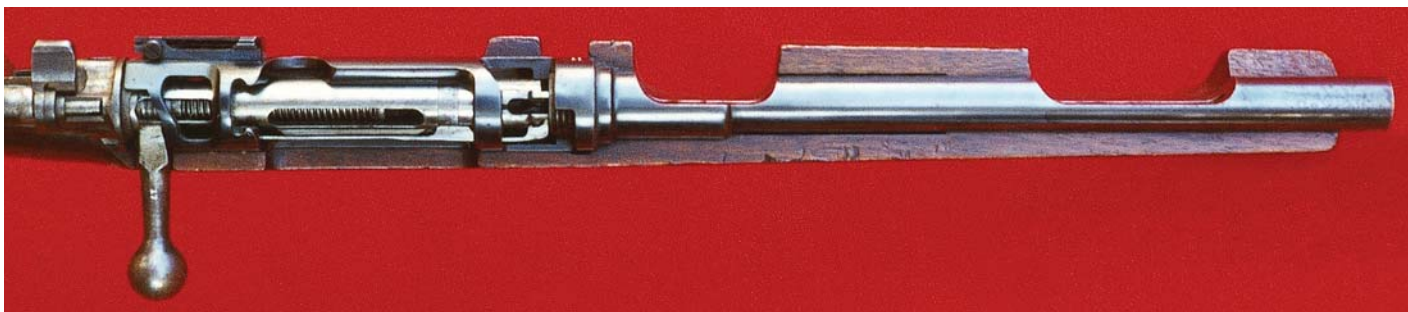
Mexican Model 1910 7mm Cut-away Rifle training aide. Top view of the action with the bolt closed. (R. K. Smith collection)
