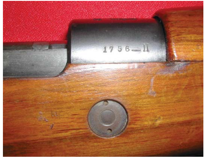
The serial numbers on Yugoslav M1924 Short Rifles made at Kragujevic Armory were always applied to the right side of the receiver ring just above the wood line, such as on number: "1756-II" shown above. Interestingly, Branko Bogdanovic's reported Kragujevac serial number ranges for the M1924 do not include any with letter suffixes. The meaning of the "-II" is not presently known. (John Wall collection)
