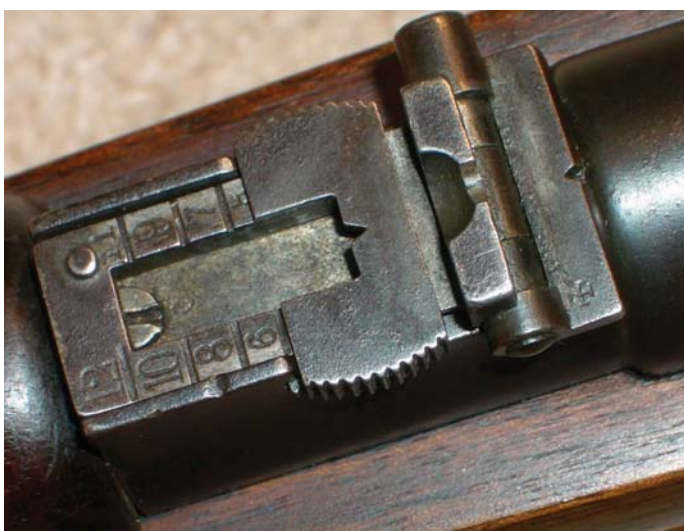
The rear sight assembly of the 7.65mm Spanish Model 1891 Cavalry Carbine purchased from Ludwig Loewe in 1893/94. (Hans-Joerg Meyer collection)
