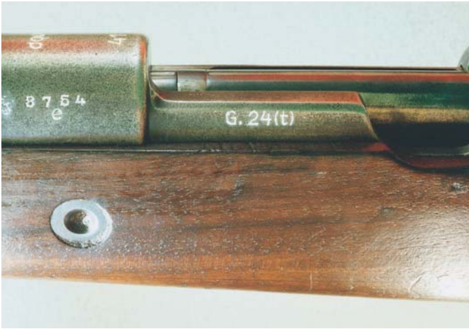
The side rail of the German Model 24(t) Rifle, showing the model designation. Note the typical deep-dished recoil crossbolt.
