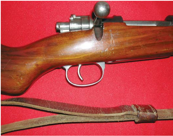
The breech area of the M1924 Rifle stock has been notched so that the stock could be issued with the uniquely configured turned down bolt commonly used on Kragujevic M.1924 cavalry rifles and the M.1924CK Assault Carbine. The left side of the receiver has the standard Yugoslav post-1931 mark: "VOJ. TEH ZAVOD KRAGUJEVAC", which Bogdanovic translates as the "Military Technical Institute, Kragujevac". (John Wall collection)
