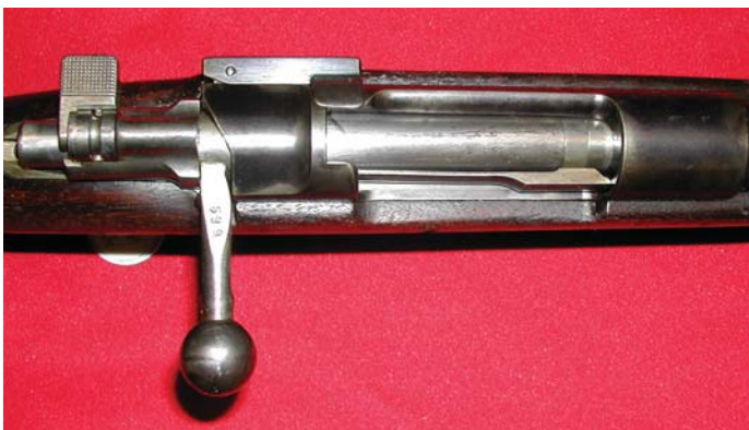
A top view of the Spanish-type M1892 Long Rifle's action. Note the long non-rotating extractor on the lower side of the bolt body, and the bolt release with its curved arm that supports a charger clip during loading. (U.S. Army Ordnance Museum, Aberdeen Proving Ground, Md.)
