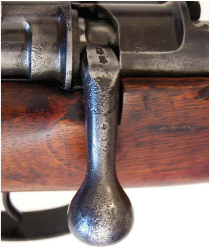
The receiver bridge and bolt handle of the Mauser Oberndorf-made Serbian Model 1910 Short Rifle. German commercial “B” and “U” proof marks, as well as the serial number, K417, appear to be period markings. This rifle was previously undocumented, so we do not know for sure if it is a purpose-made weapon or a factory conversion of an original M1910 Long Rifle. (David Jonas collection)
