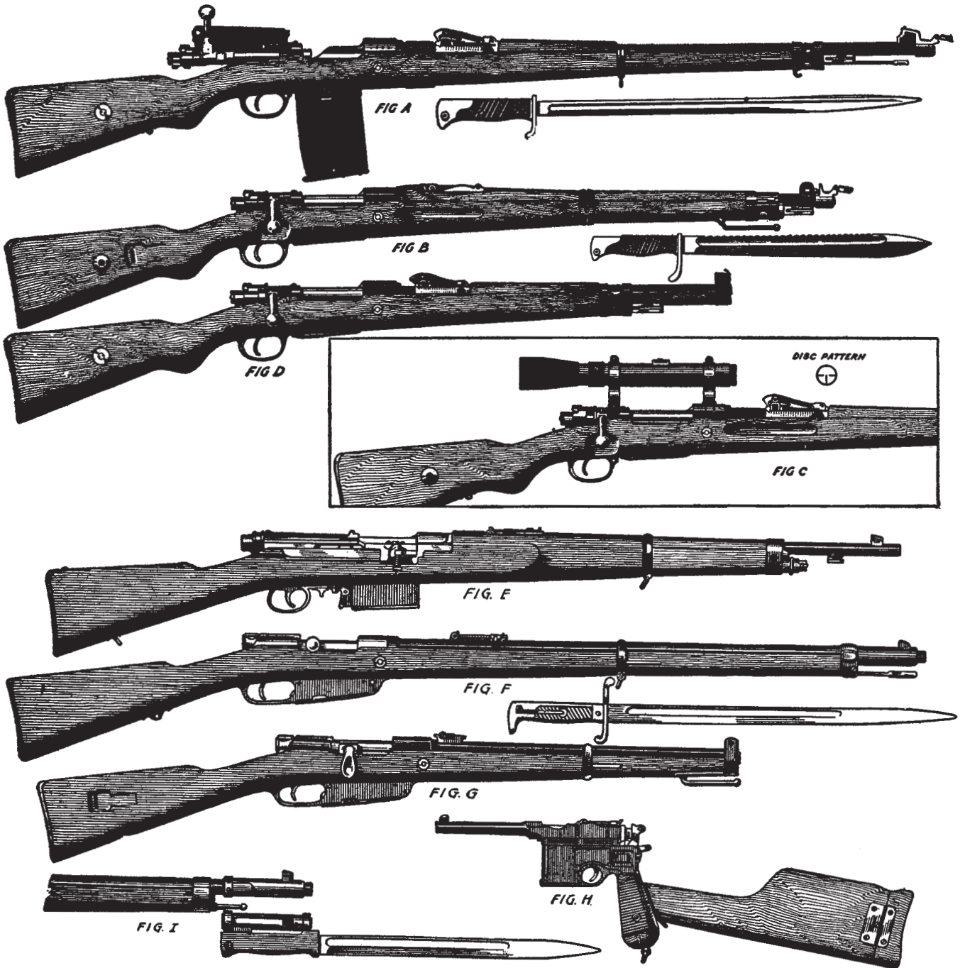
FIG. A. (GERMANY) MAUSER RIFLE, the infantry arm of the German Army. Stamped on the left of the receiver "GEW 98" meaning Gewehr (weapon) of the year, 1898. The rifle is shown with the action open and bolt withdrawn to the rear, equipped with the breech-cover, designed to keep wind and dirt out of the mechanism while in use in the trenches. It will also be noticed that the extra magazine, made to hold 20 cartridges, is attached. A muzzle cover is in its proper place as well. The bayonet shown is the model brought out with the gun in '98, but during the War over forty different designs were made; these are shown in a book we have on sale, see notice elsewhere. The calibre of GEW '98 is .31 and the magazine holds five shots.
