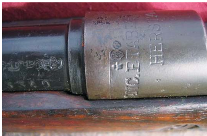
The left side of the Pieper M1889/36 conversion. Note the Liege proof marks in combination with the faint "EGB" oval Government proof mark. (John Litt collection)
