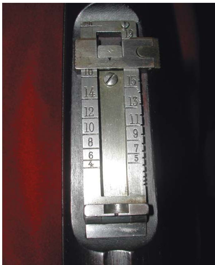
The rear sight leaf of an original Loewe Model 1893 Spanish Army Long Rifle, graduated from 400 to 2,000 meters and using a distinctive sight slide which has a single catch located on the right side of the ladder. Later Oviedo rifles used a unique slide of heavier construction that was adjusted by a button instead of the slider shown here. (John Wall collection)
