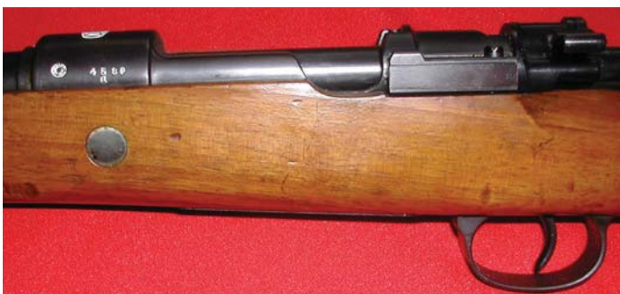
The left side of the Chinese Kar98k contract Mauser. Although this is the German Service Rifle reborn for sale in Asia, it lacks the normally seen "Md. 98" side rail markings found on the Wehrmacht version. Note the second Chinese Nationalist sunburst emblem on the left side of the receiver ring. (John Wall collection)
