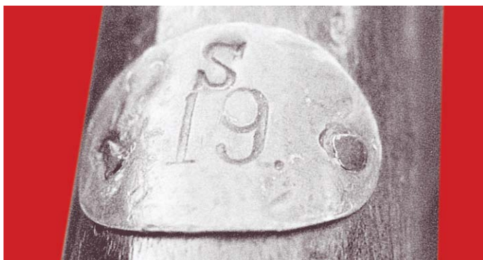
Property plate on the bottom of the stock of the Swedish Navy Model 1894 Carbine. (Noel Schott collection)
