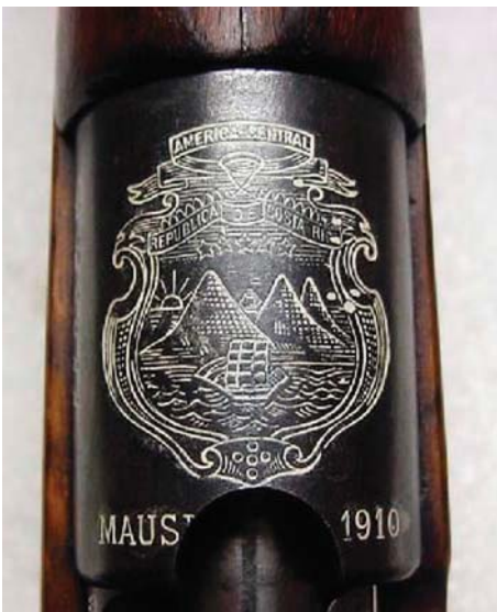
A small number of Costa Rican Model 1910 Long Rifles have turned up with barrels cut down to approximately 22 inches. Several of these have been further converted to chamber the .30-06 U.S. service cartridge. The Model 1910 rifle shown here is one such conversion; note the deep notch machined into the receiver ring to accommodate the extra length of the .30-06 round. (Ed Parada collection)
