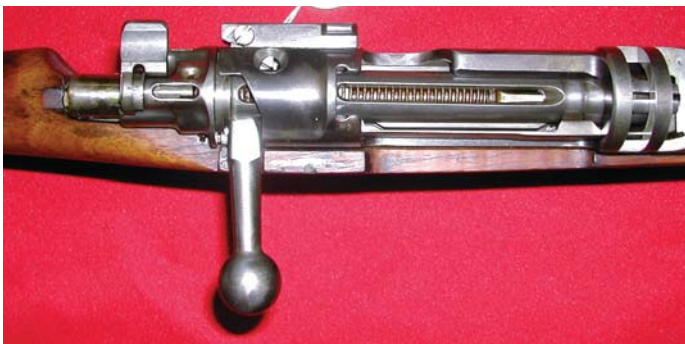
Top view of the Steyr Mauser Short Rifle with cut-away areas showing key areas of Mauser Model 1898 functionality. (U.S. Army Ordnance Museum, Aberdeen Proving Grounds, Md.)
