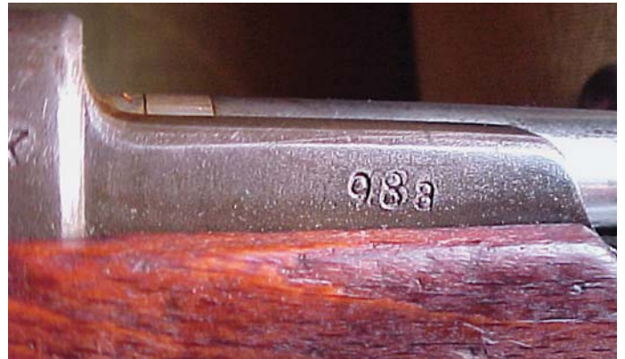
The side rail of a W.98 converted to Wz 98 configuration, remarked "98a." New barrels with flat tangent sights were added during this rebuild. (John Wall collection)
