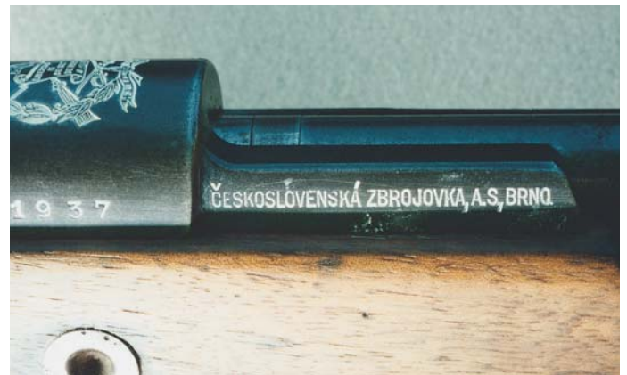
The side rail of the Guatemalan VZ 24 Short Rifle showing the manufacturer's markings—in this case, in Czechoslovakian. The number on the side of the receiver ring is not the date produced, but the serial number.
