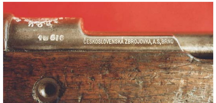
The left side of the action of the Uruguayan Model VZ 37 ("937") Carbine, showing the proof marks and the manufacturer's markings in Czech. (Noel P. Schott collection)
