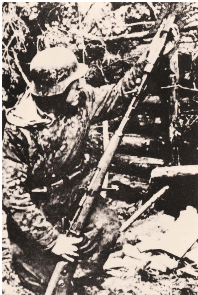
German soldier with German Model 98k Carbine with grenade launcher attached. The soldier is shown matching the grooves of the rifle grenade to the lands of the grenade launcher. (Signal)
