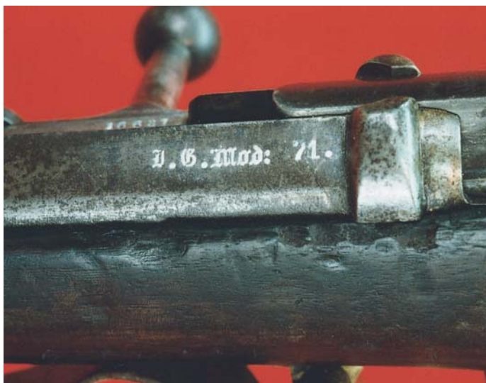
Left rear flat of the receiver showing the model designation of the German Model 71 Rifle.
