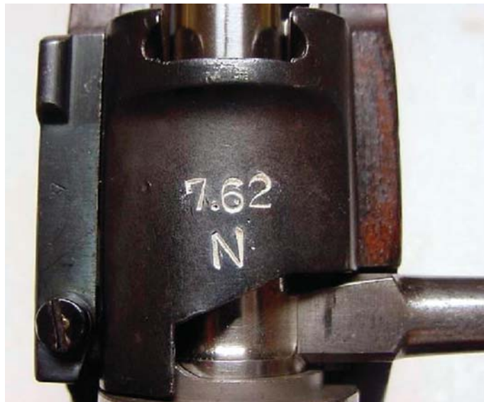
After the adoption of the 7.62 NATO cartridge, Chile converted a number of its Steyr-made Model 1912 rifles to the new standard caliber. Converted long rifles, which came from the factory with receivers in the white, were blued and marked "7.62" over "N" on the receiver bridge. Note the absence of marks on the receiver ring to the left. (Ed Parada collection)
