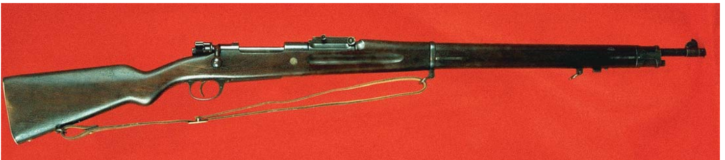
A full-length view of a most unusual variation of the Modelo 1909 Rifle. This rifle has been experimentally restocked in a Springfield Model 1903-style "C" stock with grasping grooves, a Springfield-style rear and front sight, and a most unusual stud-type bayonet lug. The receiver ring is marked in the conventional manner.
