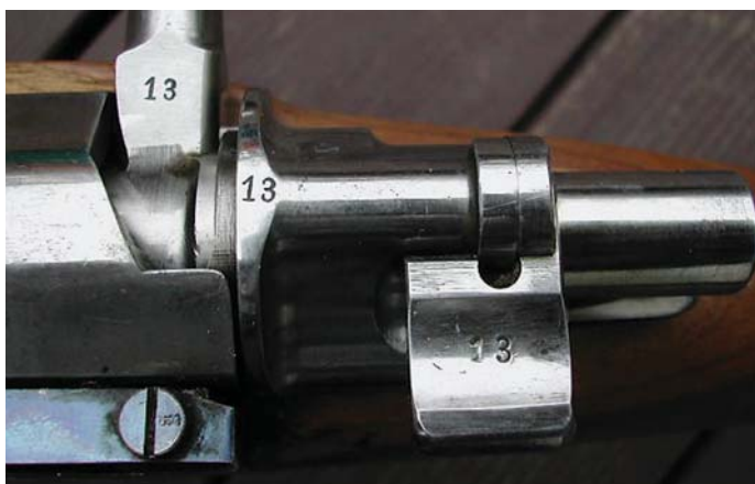
All components on the bolt shroud and firing pin assembly of the 5.97mm Test Rifle are finished in the white and are serial numbered "13." (John Wall collection)
