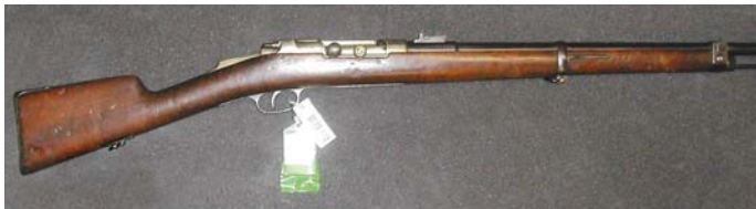
The Serbian Model 1884 Artillery Carbine shown is one of only 4,000 made by Waffenfabrik Mauser in 1884-85. This repeating carbine was fed from a six-round tubular magazine of the same style used in Mauser's Model 71/84 rifle for German infantry. The artillery carbine has a 21-inch barrel, almost 3 inches longer than the M1884 cavalry carbine, and is chambered for the Serbian 10.15mm blackpowder service cartridge. (From the former Pattern Room Collection now in the Royal Armouries Museum, Leeds, England)
