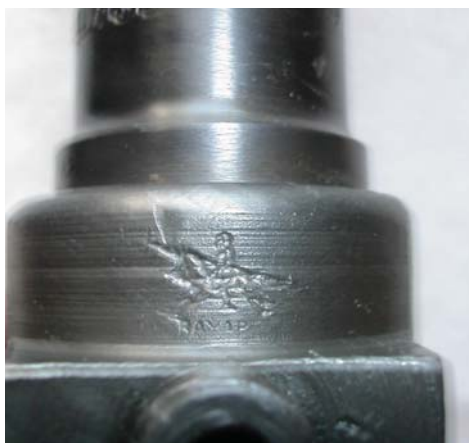
The cavalier on horseback is the traditional trademark of the Pieper firm of Liege, Belgium. This particular stamp was found under the receiver of a German Gewehr 98 bearing a Crown-over-Spandau, 1916 crest. It is believed that the Imperial German national armory at Spandau subcontracted the manufacture of a number of Gew 98 receivers to both Pieper and the German industrial firm of Siemens and Halske. A firm noted for its industrial dynamos, Siemens and Halske made receivers that were stamped with their stylized overlaid "S and H" trademark (right). This particular receiver is a 1917 Spandau Sterngewehr. (John Wall collection)
