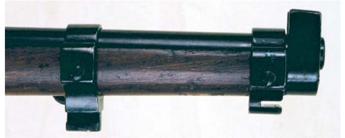
Close-up view of the bayonet's lugs permanently attached by screws on the M1891 Engineer's Carbine.
