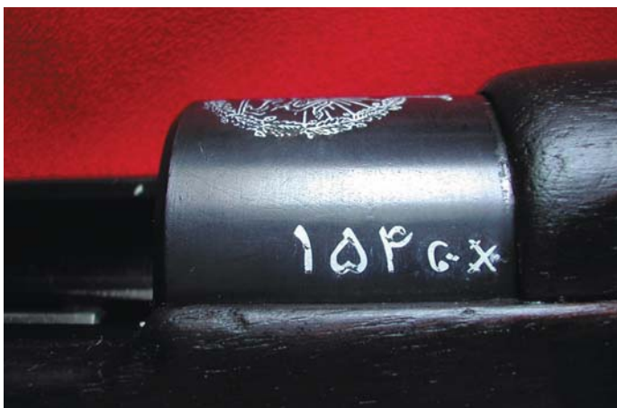
The serial number of the FN Model 1924 made for Iran was stamped on the right side of the receiver. (John Wall collection)
