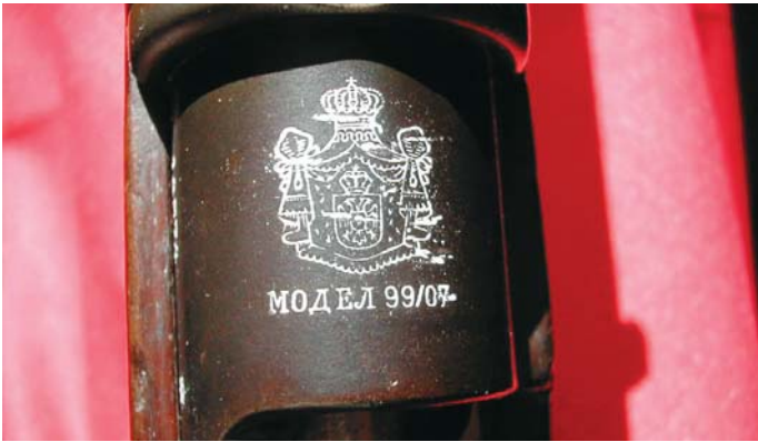
The receiver crest of one of the 30,000 Model 1899/07 Serbian Infantry Rifles made in 7mm Mauser by the Austrian Arms Company (OEWG) of Steyr, Austria. (John Wall collection)
