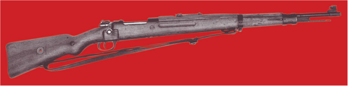
Full-length view of the right side of the Slovak Republic VZ 24 Short Rifle with variant turned-down bolt handle and inletted stock. (Robert Jensen collection)
