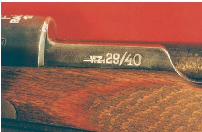
Side rail of the converted Polish Wz 29 Short Rifle. Note the crossed-out model number "wz," and the addition of the "/40" behind the "29."
