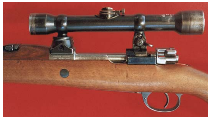
The scope and scope mount from the left hand side of the Argentine Modelo 1909 Sniper Rifle.
