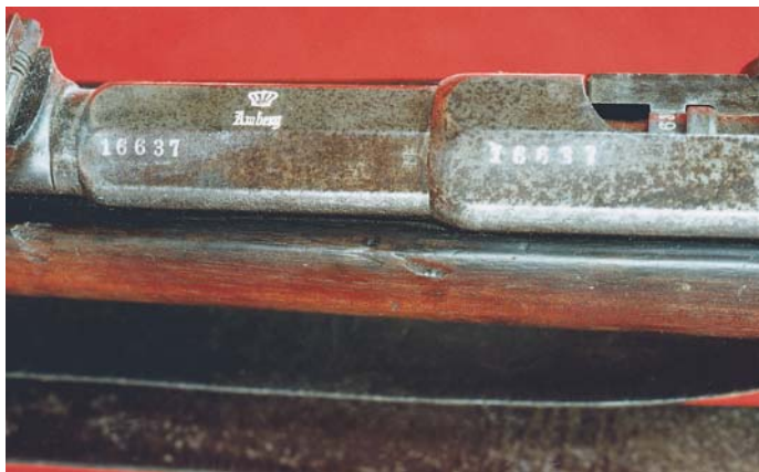
Marking of the royal arsenal at Amberg on the top flat of the chamber, with the serial numbers on the left flats of the chamber and the receiver of the German Model 71 Rifle.
