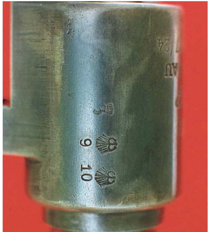
Right side view of "Zn" Spandau 1917/24 receiver showing proof marks; these are early Waffen Amt, with unit marks 9 and 10. (R. K. Smith collection)
