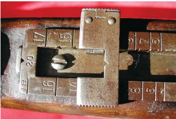
The top of the rear sight of the Serbian Model 99/07 Long Rifle has a unique sight slide which features two large screws securing the sight's range slide to the sight ladder. (John Wall collection)
