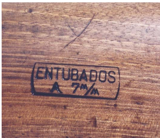
Marking on both sides of the buttstock of the Standard Modell Short Rifle used by Spain. This warns users that the rifle has been rebarreled for the 7 x 57mm cartridge.
