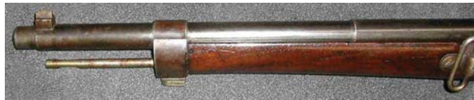
The forestock, muzzle and cleaning rod of the Garde Civique Bicyclist's Rifle. (Pattern Room Collection, Royal Armouries Museum, Leeds, England)
