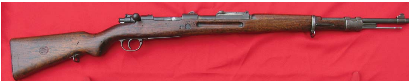
A Chiang kai-Shek (Zhong Zheng Shi) pattern Mauser Short Rifle modified after the Standard-Modell Mauser Oberndorf rifle of the early 1930s, made at Guangdong (Kwantung) Arsenal during WWII when it had been moved inland away from Japanese Forces to the Province Guizhou, where it was known as the 41st Arsenal. According to the 1997 (page 152) Military Rifle Journal article by Stan Zielinski "Chinese Military Rifle marks: Part 5, The Kwantung (Canton) Arsenals," rifles made by the 41st. Arsenal are undated and marked only with this crest. (John Wall collection)
