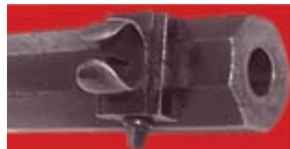
Boer “Plezier” hooded, windage-adjustable front sight. (Jack Carnahan collection)
