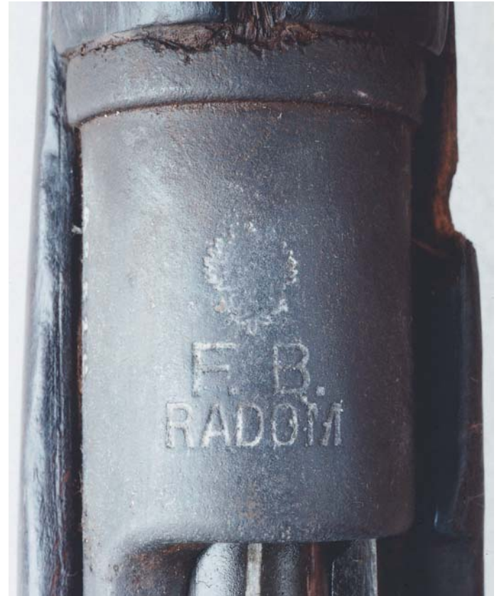
Polish markings on the receiver ring of the Polish version of the Model 98AZ Carbine. Note the lack of a date on this specimen. (Century International Arms, Inc.)
