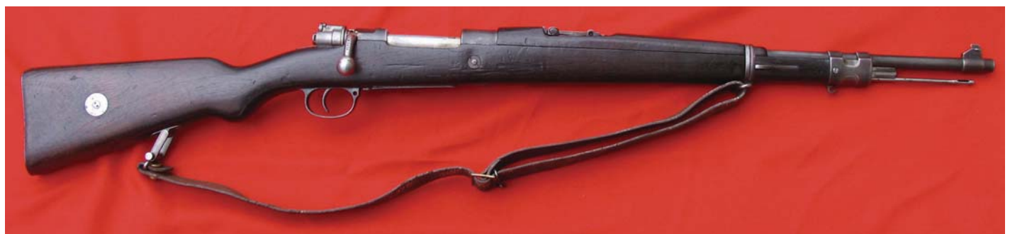
Between 1912 and 1914, Oesterreichische Waffenfabriks-Gesellschaft, (OWEG) the Austrian Arms Company of Steyr, Austria, produced a number of Model 1912 Long Rifles and Carbines for the Colombian Army. The Carbine version, shown here, was made with a 55cm (21.5 in.) barrel. Note the use of the Gew98-like quick detachable sling swivel, the short bayonet bar, and the presence of the unit-marking disc in the buttstock. (John Wall collection)
