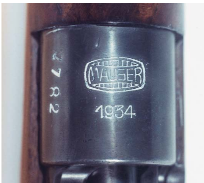
Markings on the receiver ring of the Standard Modell Short Rifle as used by Spain.
