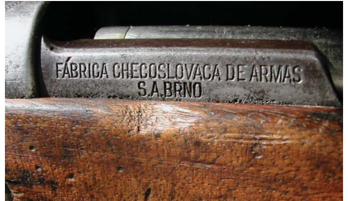
The receiver side rail with Czechoslovak Brno markings in Spanish on the Colombian VZ 24 Service Rifle. (John Wall collection)
