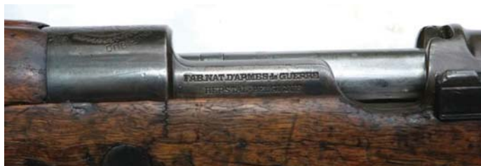
The FN side rail address text on the Argentine-San Juan Province police carbine. Note the serifs on the font, used on FN rifles from the mid-1920s to the mid 1930s. (John Wall collection)
