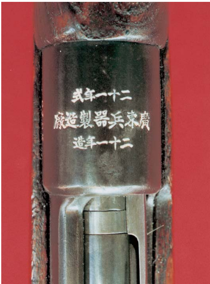
Markings on the receiver ring of the Chinese Model 21 Short Rifle. (Noel Schott collection)
