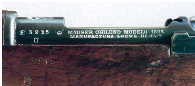
Manufacturer's markings on the side rail of the Chilean Model 1895 Rifle. Note that the manufacturer is Ludwig Loewe & Co., Berlin.
