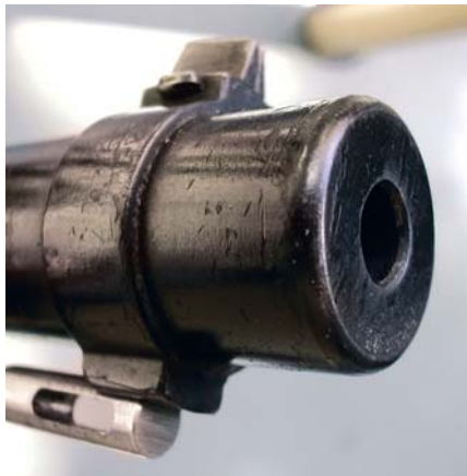
The crown and the muzzle of the Belgian Model 1889 Heavy Barrel Rifle. (John Wall collection)
