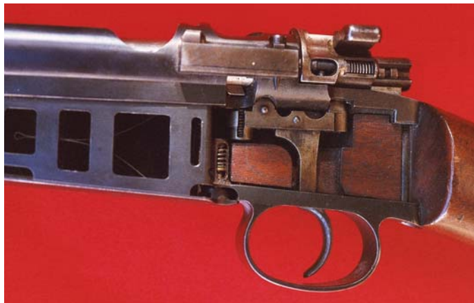
Close-up view of the lower left side of the Mexican Model 1910 Cut-away Rifle training aide, with the bolt closed. (R. K. Smith collection)
