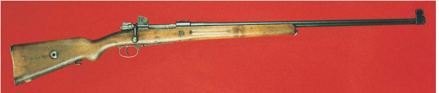
Full-length view of the Danish Military Target Rifle made with the action of a German Model 98k Carbine.
