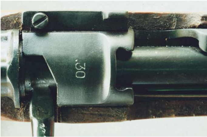
Caliber marking on the receiver bridge of the Colombian Model 1950 Short Rifle.
