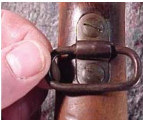
The lower sling boss on the Mexican M1912 was, in Austrian service, replaced by a large swivel design to accommodate the wide Austrian M95 rifle sling and its thick metal buckle. (John Wall collection)
