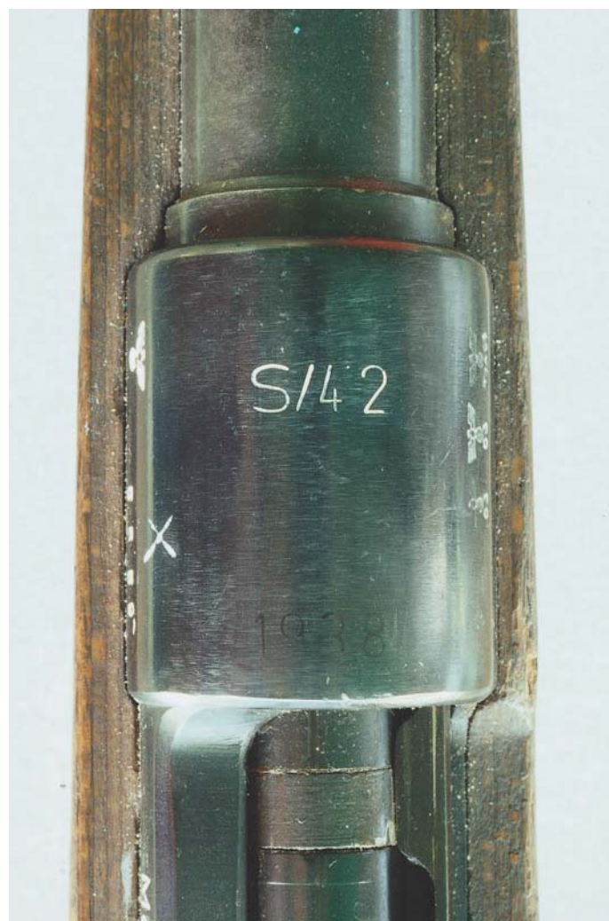
Receiver ring of the German Model 98k Carbine, showing the code "S/42" over the barely-discernible date "1938." What is interesting is that this carbine bears the crossed Russian rifle mark on the left rear of the receiver ring, indicating capture and later reissue by the Russians. This particular specimen was captured from the Viet Cong in 1968!
