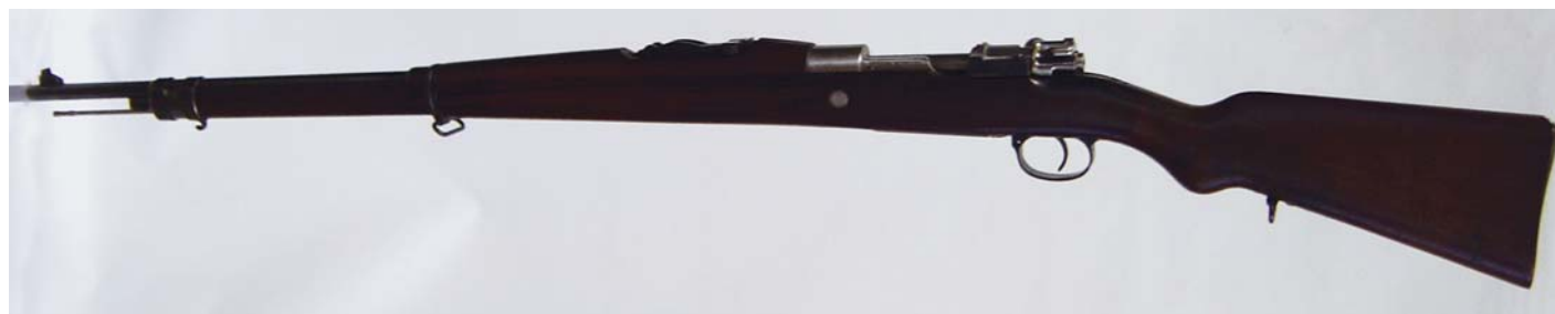
Brazilian M1908 Mauser Rifle, 8x57 J, left side full-length view; note the high hump to the tangent rear sight. (Jan Gardiner collection)
