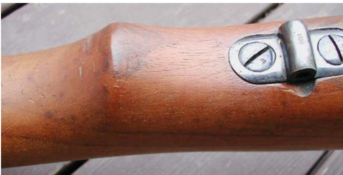
The underside of the small of the 5.97mm Test Rifle's stock is also devoid of markings. Note the pointed pistol grip, a feature rarely seen on Oberndorf military rifles, and the base for a quick detachable sling swivel. (John Wall collection)
