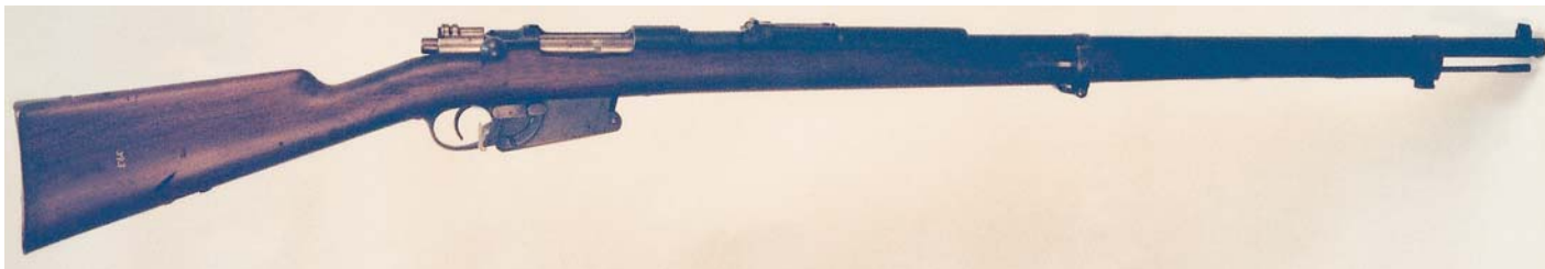
Full-length view of special test Model #3 1892 Mauser Rifle. Note that the rear sling swivel is missing from this rifle. (Springfield Armory Museum)
