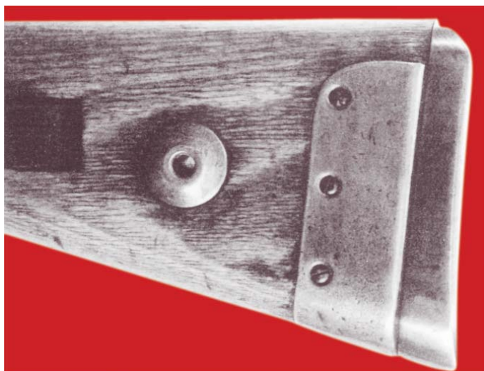
The left side of the German Model 33/40 buttstock, showing the sheet steel protecting plate adjoining the cupped buttplate.
