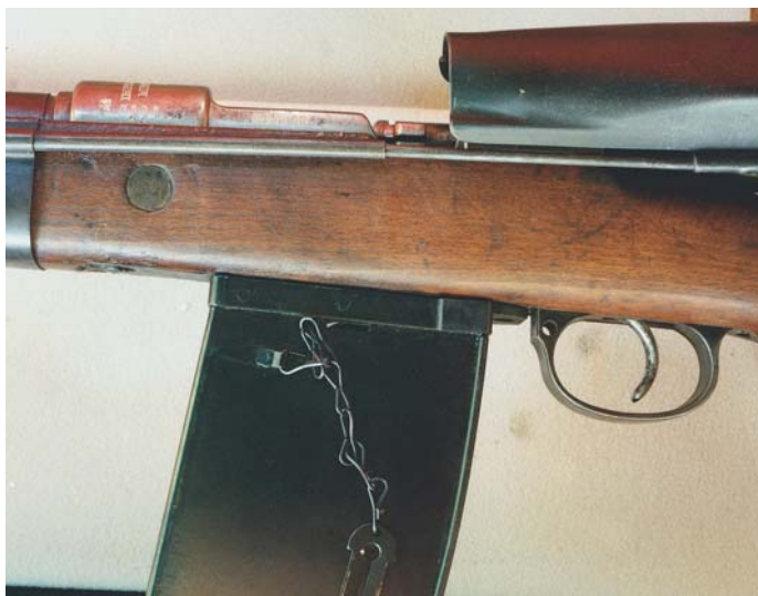
Left side view of the action of the German Model 98 Rifle with extended magazine and sliding bolt cover (see next page, top). This picture clearly shows the clip and rod that allows the bolt cover to slide back and forth with the action of the bolt, as well as rotating into position with the closing of the bolt. Also shown is the chain and key attachment used to hold the spring and follower in position during installation and removal of the extended magazine.
