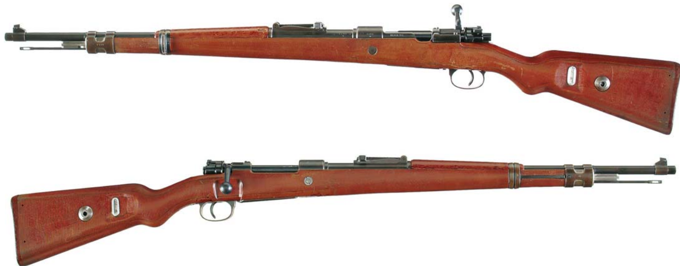
Right and left side views of K98k Mauser Rifle with experimental resin stock and handguard. Numbered "22" out of only several hundred produced for testing. The stock is made of red resin, composed of a hollow fabric base, laminated with plastic resin strips molded to the shape of the stock, with a lacquer finish. To strengthen the stock, an aluminum liner has been inserted in the sling slot and a flat buttplate screwed to the molded-in cupped butt. (Rock Island Auction Co.)
