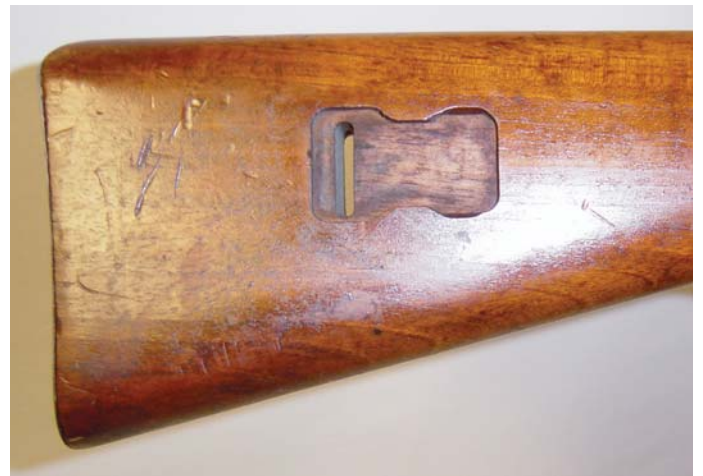
View of stock, showing cut for German-style sling attachment. (Jan Gardiner collection)
