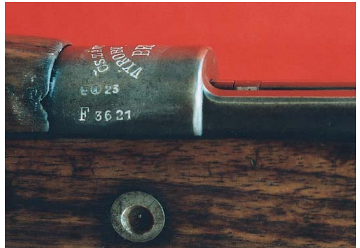
Left side view of the receiver ring showing Czech acceptance marks and the rifle serial number of the Czech VZ 23 Short Rifle. (Bob Bennett collection)
