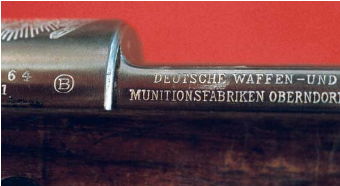
Manufacturer's markings on the side rail of the Brazilian Model 1908 Short Rifle.
