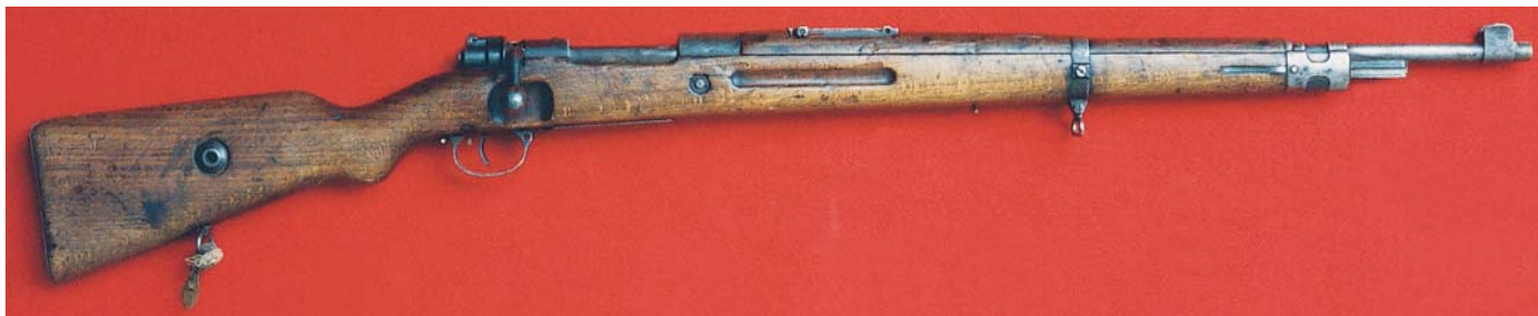
Full-length view of the Polish Wz 29 Short Rifle as issued for cavalry. Note the bent bolt handle.
