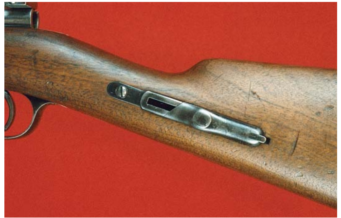
Close-up view of the slotted sling attachment on the left side of the wrist of the stock of the 1889 Carbine, lightened version.
