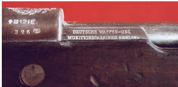
The left side of the action of the Uruguayan Model 1908 Short Rifle, showing the proofs and serial number on the side of the receiver and the manufacturer's markings on the left side rail. (Noel P. Schott collection)
