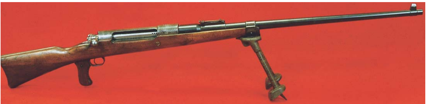
Full-length view of the German 13mm T-Gewehr, bolt action, single shot, Anti-tank Rifle.
