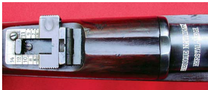
The action of an un-issued Model 1893 FN Cavalry Carbine, showing the rear sight ladder and slide, and the generic FN receiver marking: “Fabrique Nationale” over “Herstal, Liege.” (John Wall collection)
