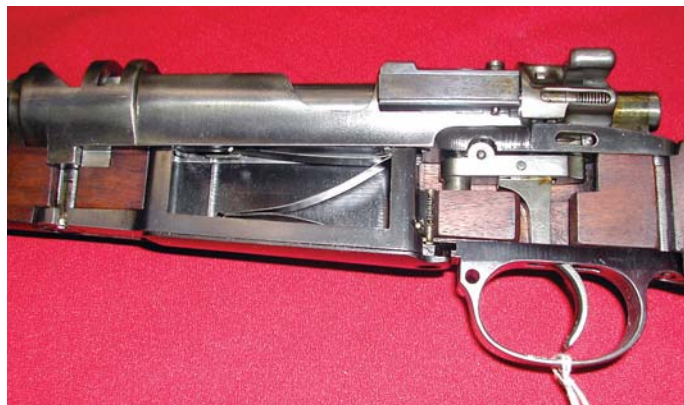
Cut-away section of the full left side of the Steyr-made Mauser 98 action. (U.S. Army Ordnance Museum collection, Aberdeen Proving Grounds, Md.)
