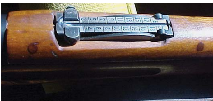
The rear sight leaf and handguard of a Polish Wz 29. Note the distinctive Polish practice of strengthening the front and rear sections of the handguard with horizontal dowels. (John Wall collection)
