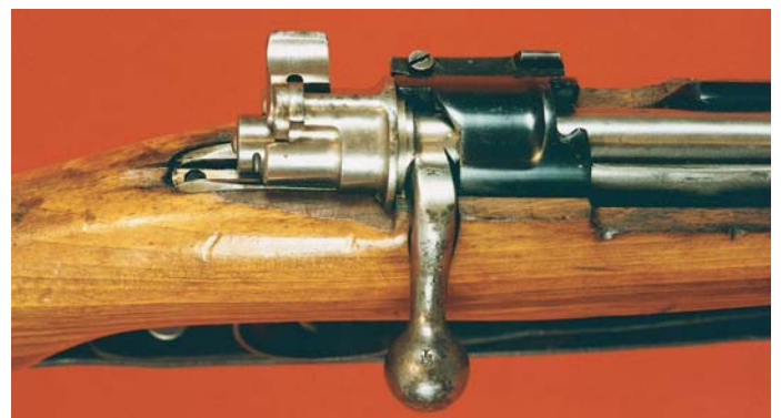
The action and the slightly recurved bolt handle on the Yugoslavian Model 24 Carbine.
