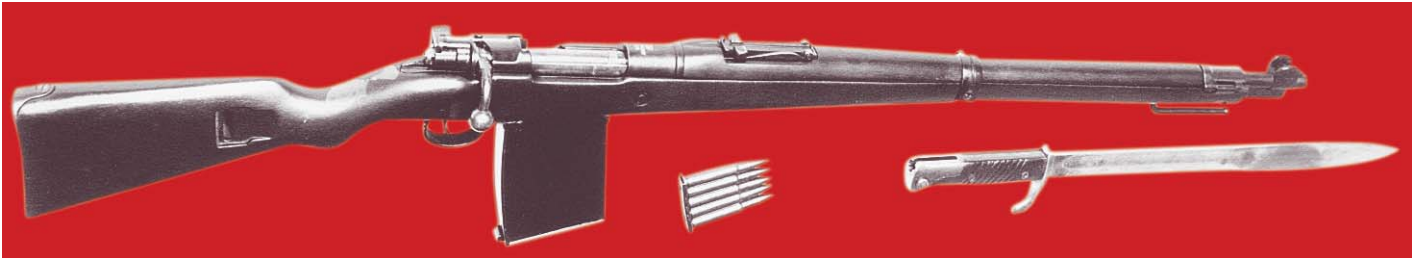
Full-length view of the right side of a German Model 98a Carbine fitted with an extended 20-round magazine, also showing a clip of cartridges and the customary bayonet. (John Wall collection)
