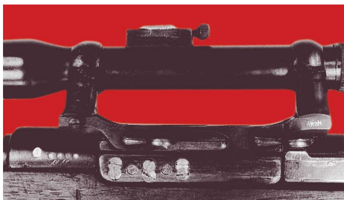
Left side of the police-issue Kar 98a Carbine, showing the side mounted sniper scope. (Robert Jensen collection)
