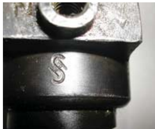
The cavalier on horseback is the traditional trademark of the Pieper firm of Liege, Belgium. This particular stamp was found under the receiver of a German Gewehr 98 bearing a Crown-over-Spandau, 1916 crest. It is believed that the Imperial German national armory at Spandau subcontracted the manufacture of a number of Gew 98 receivers to both Pieper and the German industrial firm of Siemens and Halske. A firm noted for its industrial dynamos, Siemens and Halske made receivers that were stamped with their stylized overlaid "S and H" trademark (right). This particular receiver is a 1917 Spandau Sterngewehr. (John Wall collection)
