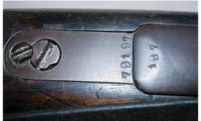
Serial number font and convention used on the trigger guard assemblies of Kunghsien Arsenal Chiang kai-Shek Mauser rifles circa 1937. (John Wall collection)
