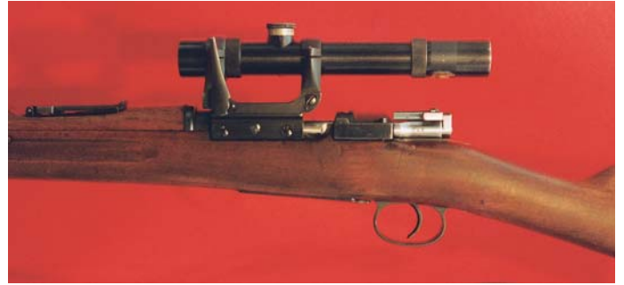
Close-up view of the left side of the Swedish Model 1896 Sniper Rifle fitted with the Model 44 AGA scope.
