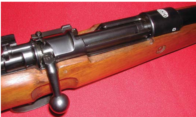
The right side of the receiver area of the Chinese contract Kar98k Mauser Rifle. Note the presence of the famous Mauser Banner trademark on the receiver, and the distinctive K98k style curved bolt, stock recess, bluing, and the single Chinese government sunburst emblem used as an acceptance and inspection mark. (John Wall collection)
