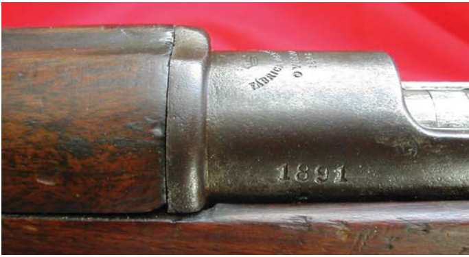
The side rail of the Model 1896 Oviedo Long Rifle is blank. Unlike later Spanish M1893s, which are serial numbered on the side rail, this early rifle is serial numbered on the left side of the receiver ring. (John Wall collection)
