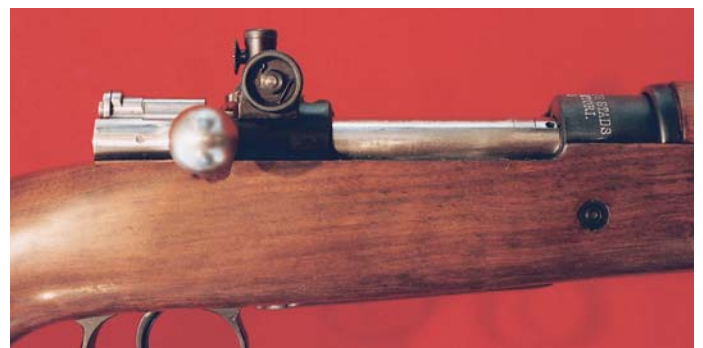
Close-up view of the action and receiver bridge sight on the heavy-barreled version of the Swedish Model 1896 Target Rifle.
