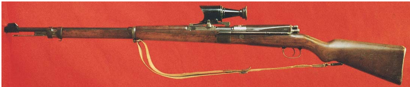
Left side view of the German Model 98 Marksman Rifle fitted with the low light bifocal marksman scope and front sight, as well as with a sliding bolt cover.
