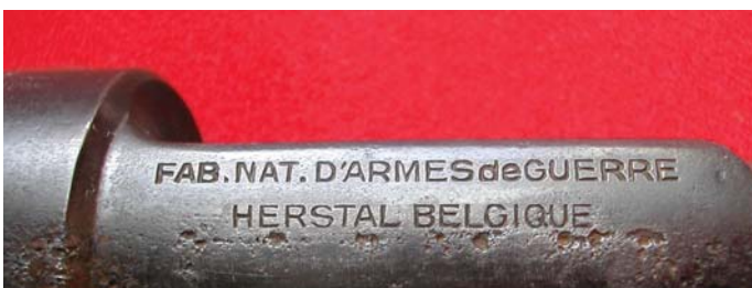
The side rail text of the FN Model 1930 Short Rifle dated “1938” Note that the letter font is without serifs, and characteristic of FN rifles made from the last of the 1930s to the early 1950s. (John Wall collection)
