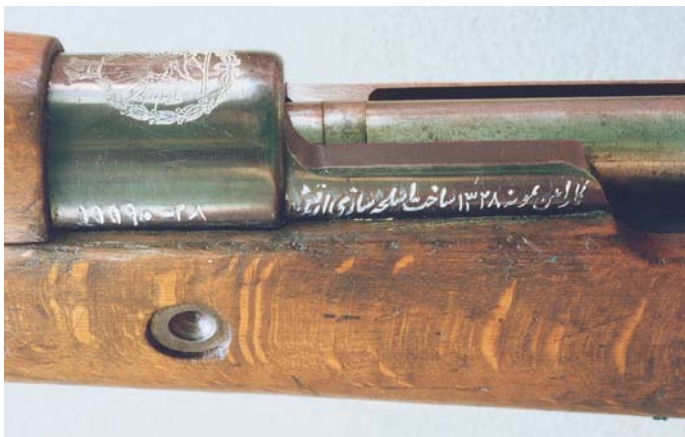
Left side view of the receiver ring and side rail of the Iranian Model 49 Carbine, with the manufacturer's markings stamped in Farsi.
