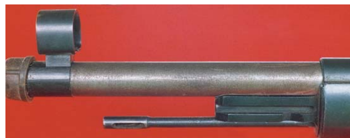
A virtually brand new G33/40 Mountain Carbine! A vet bring-back, this carbine was assembled from un-numbered parts at the factory when Americans pulled back to allow Russians to come in. Note that the front sight is not silver soldered on, nor is the bolt or receiver numbered! (R. K. Smith collection)
