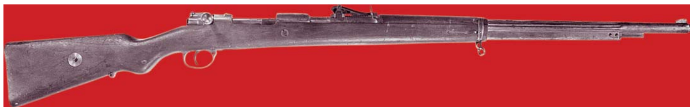
Full-length view of the right side of an experimental version of the German Model 98 Rifle with a fluted cooling jacket and shortened forestock. (John Wall collection)
