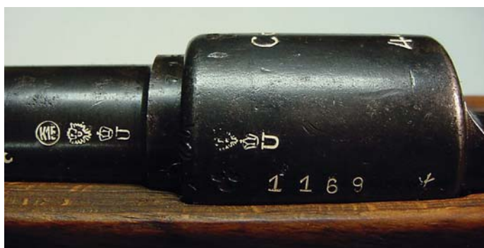
The spread wing eagle and the crown-over-N are definitive smokeless powder proofs used in the German Democratic Republic after 1950.
