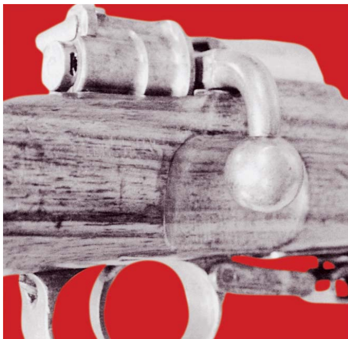
Close-up view of the professionally bent bolt handle and recessed stock of the Colonial Service marked, modified German Model 98 Rifle.
