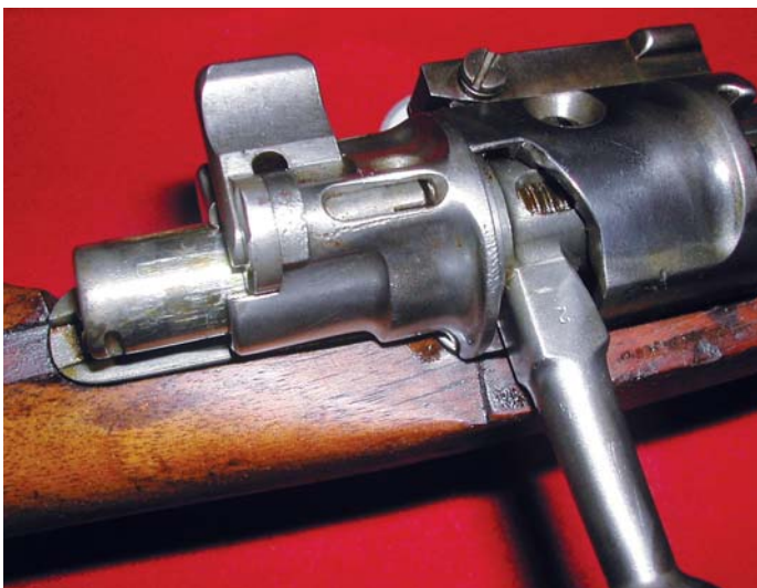
Cut-away bolt sleeve illustrating the operation of the Mauser Model 1898 safety on the Steyr-made experimental Mauser Short Rifle. (U.S. Army Ordnance Museum, Aberdeen Proving Grounds, Md.)
