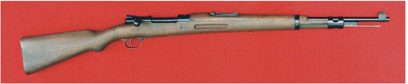
Full-length view of the Spanish Model 1944 Short Rifle as made for the Spanish Air Force. Note that the air force model does not have the auxiliary bayonet lug.
