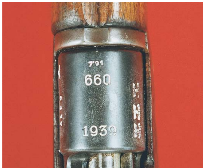
Steyr code "660" over "1939" on the receiver ring of the German Model 29/40 Rifle. Note the German waffenamt proofing on both sides of the receiver ring.
