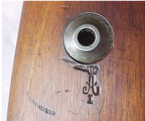
A close-up of the bolt dismount tubes and unit marking plates on the two Yugoslav M1924 captured and re-issued by German forces during WW II. (John Wall collection)
