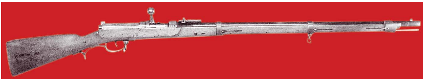
Figure 1.2 Dreyse Needle Rifle M1862 produced by the Danzig Arsenal. Double dated 1862 and 1871 indicating modification to provide obturation using the Beck System.
