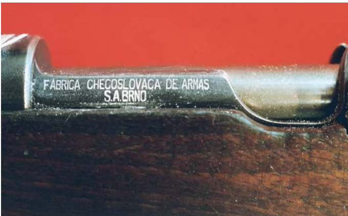
Czech manufacturer's markings in Spanish on the side rail of the Czech Model VZ 12/33 Carbine as used by Nicaragua.
