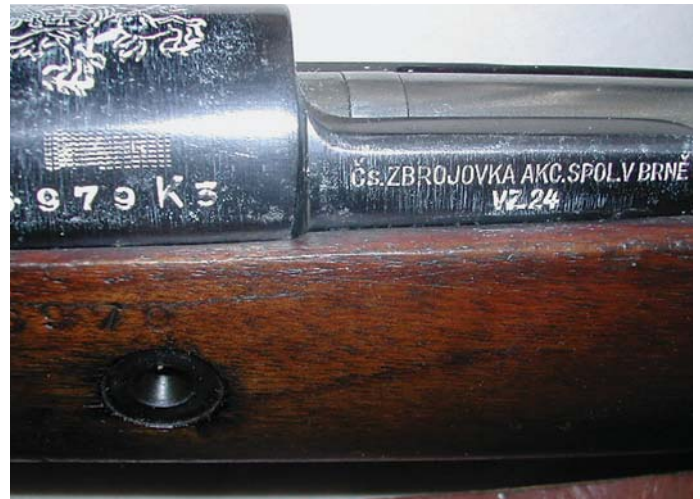
Markings on the receiver ring of the Czech VZ 24 Short Rifle.
