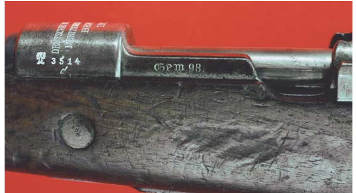
The side rail markings on the converted German Model Kar 98b Rifle. Note that this is marked "Gew. 98."
