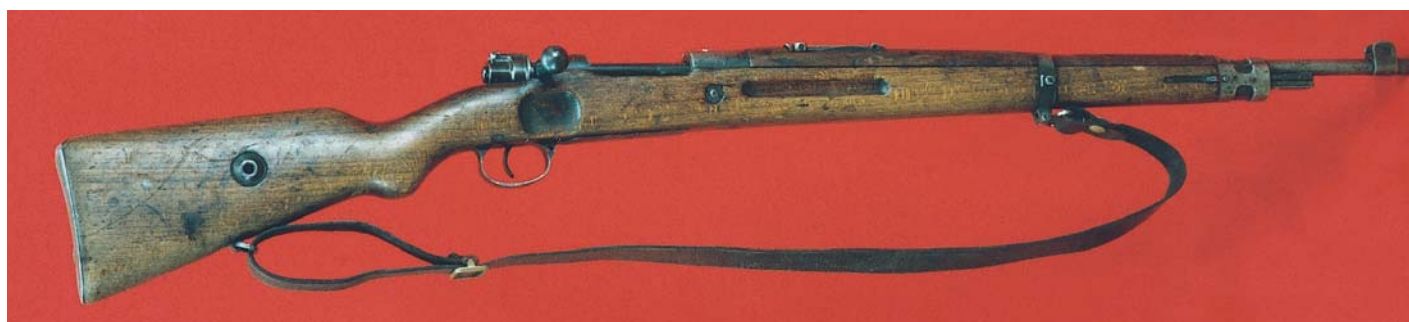
Full-length view of the Polish Wz 29 Short Rifle as issued for infantry. Note the straight bolt handle.
