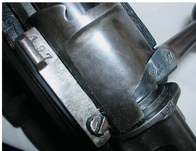
The receiver bridge of a Chinese-made Mauser "Standard Modell" (Chiang kai-Shek) Mauser Service Rifle. This particular rifle was manufactured at Kunghsien Arsenal in Honan Province in 1937. Note the untouched original serial numbers and the numbering convention on this unissued rifle. (John Wall collection)
