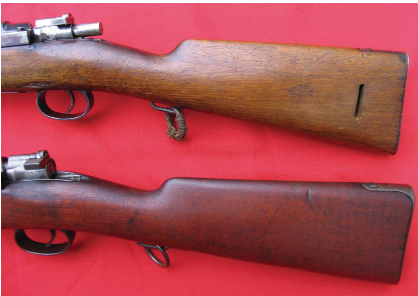
A comparison of the buttstocks of the two varieties of German-made Spanish Mauser carbines: the 1894 version, lower, without a slot for a sling loop, and the upper carbine, made in 1896, with the sling slot. Note that the sling loop "key" for this carbine has been lost. (John Wall collection)
