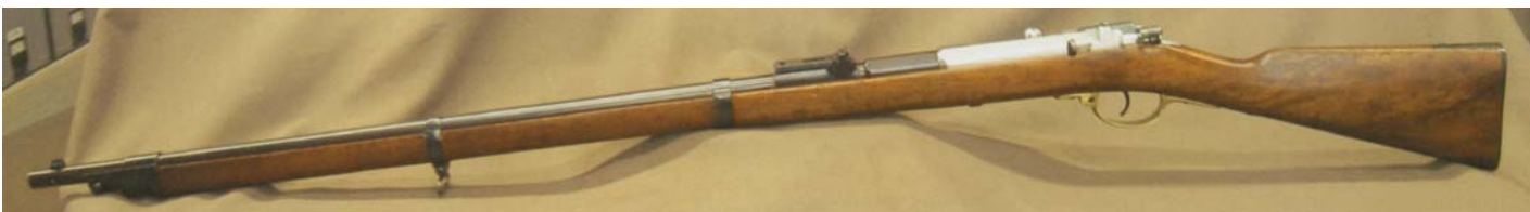
BELOW: Left side view of the prototype Model 71/78 SN 14 tube magazine fed 11mm rifle. (Private collection of Robert I. Landies)
