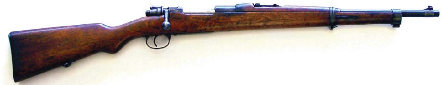
This Serbian-crested Model 1910 7mm Short Rifle was recently discovered. Previously, no short rifle or carbine variations of Model 1910 were known, and this rifle may be unique. A record of this variety being an official Serbian pattern has not yet been discovered. Although the history of this particular rifle is uncertain, the rifle features carbine sights, a front sight mounted on a barrel band, a turned down bolt handle, and German commercial proof marks on the top of the handle, receiver ring and the underside of the barrel. The Cyrillic text on the side rail indicates that the rifle was made at Mauser Oberndorf. No other information on this rifle is known. The work appears to be of factory quality. (David Jonas collection)
