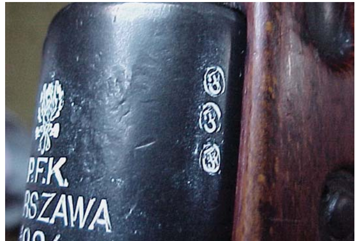
The right side of the receiver of a Polish Army "W.98" (Gewehr 98) Service Rifle made at "P.F.K. Warszawa" in 1924. Note the oval inspection marks. (John Wall collection)
