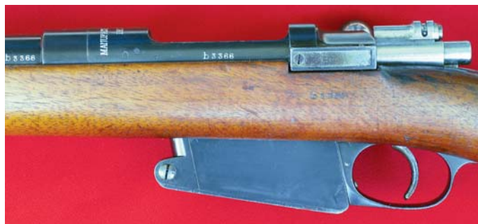
The left side of the action of the MAE Model 1889 Long Rifle. The serial number, b3366 is stamped on the stock below the ejector box, barrel jacket and receiver side wall. Note that the serial number prefix is a lower case letter. Observed newly-manufactured Model 1889 Long Rifles appear to use a serial number prefix unique to manufacturers; the FN serial number prefix is a capital letter, the MAE rifle uses a lower case letter, and the Hopkins and Allen-marked rifles use a cursive letter. (John Wall collection)
