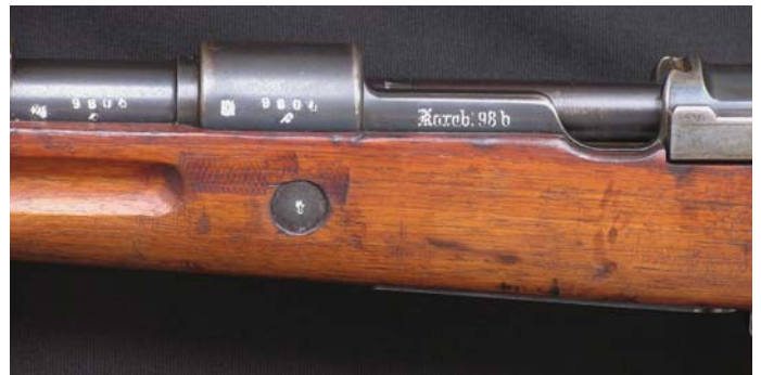
The left side of the receiver of the German Karabiner 98b as used in France after WWII. Note that all German marks remain intact, including the squared images of the German Imperial eagle, the "Reichsadler" that served as the Reichswehr firing proof. (John Wall collection)
