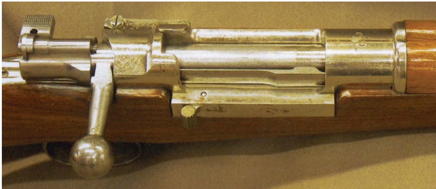
Close-up of the bolt and receiver of the Mauser Turkish Model 1893 7.65mm nickel plated with cutoff rifle. Note the clear view of the magazine cutoff, and the Turkish Toghra crest on top of the receiver ring. (Private collection of Robert I. Landies)
