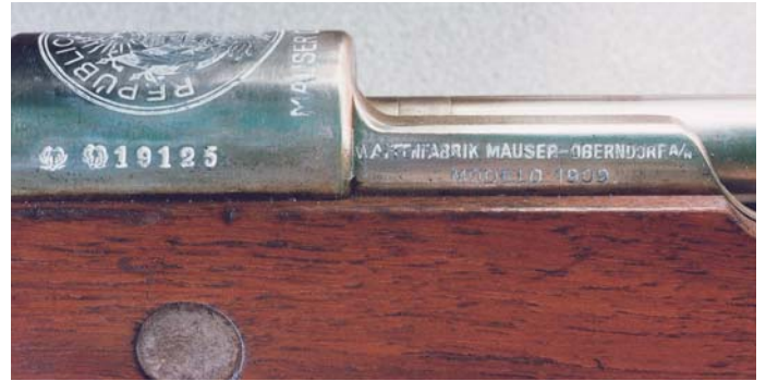
Manufacturer's markings stamped on the left side rail of the Peruvian Model 1909 Rifle. (Lothar Frank collection)
