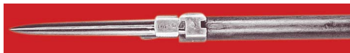
Bottom view of the folding bayonet on the Turkish Model 38 Short Rifle. Note the fluting on the bayonet blade.
