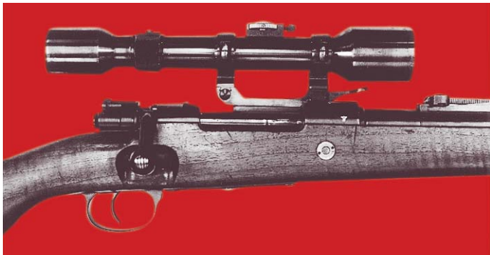
Right side view of a Kar 98k Carbine with a variant side rail mount incorporating a 4x scope. (Robert Jensen collection)
