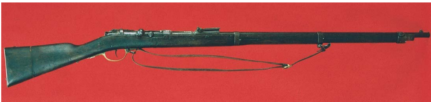
Full-length view of the German Model G 71 Rifle, as used for Japanese troop testing. All specific data on this rifle will be found in the section on Germany.
