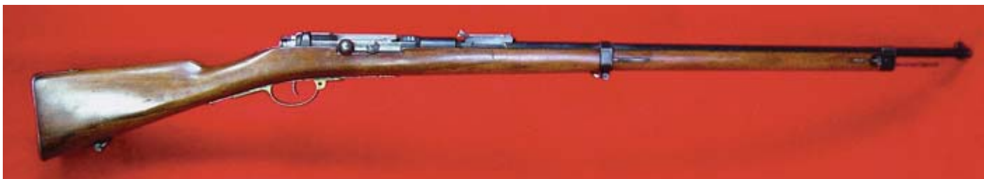
Full-length view of the Uruguayan Model 71/94 French-converted Model 1871 Mauser single shot Rifle to 6.5mm Daudeteau.
