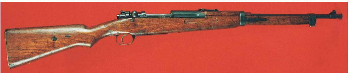
Full-length view of the Siamese Model 1923 (Type 66) Short Rifle, with the bolt cover open.
