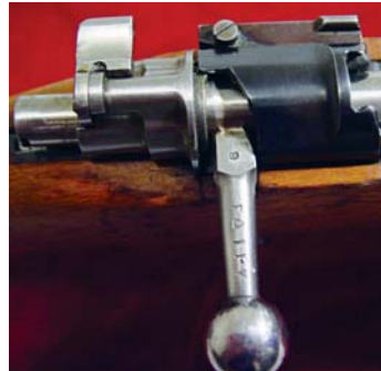
The bolt shroud and handle of the Teheran-made Model 98/29 (Iranian Model 1309) Long Rifle, showing the serial number 25147. (Darryl Beck collection)
