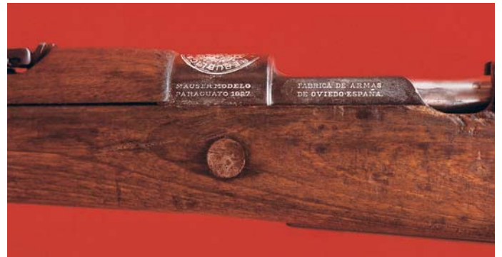
The left side of the action of the Paraguayan Model 1927 Short Rifle, showing the model designation and the manufacturer's markings.
