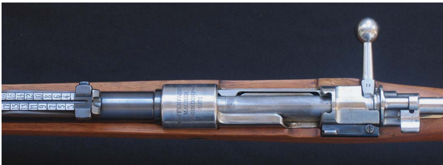
The action and rear sight assembly of the Mauser Oberndorf ballistic Trials Rifle ("versuchsgewehr") used to test the 5.97mm cartridge. (John Wall collection)
