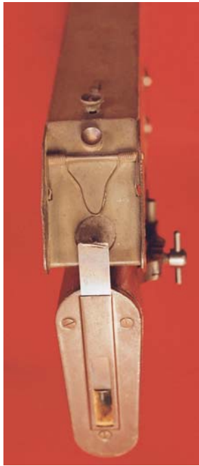
Right: The storage trap in the butt of the auxiliary stock of the German Trench Rifle-firing Device.
