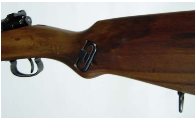
Left side view of the Bolivian Serie B-50 buttstock, showing alternate sling swivels. (Jan Gardiner collection)
