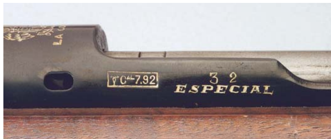
Caliber designation and "ESPECIAL" marking on the left side rail of the Spanish Modified Model 1916 Short Rifle. Note the low serial number 32.
