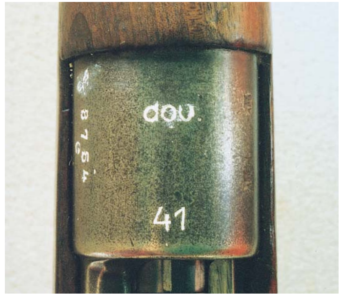
The receiver ring of the German Model 24(t) Rifle, showing the code “dou,” for Waffenwerke Brunn, A-G, Bystrica, over the date of manufacture.
