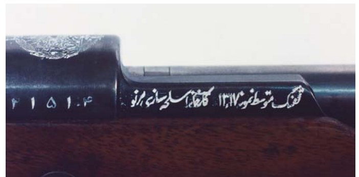
Manufacturer's markings stamped in Farsi on the side rail of the Persian Czech Model VZ 24 Short Rifle.
