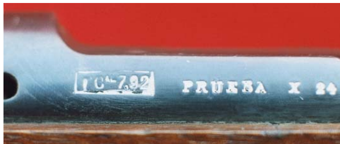
Markings on a Second Pattern M1916 Short Rifle, that has been converted to 8x57mm. built at La Coruna, the left side wall shows first "New Marking," followed by "PRUEBA," or "Test," followed by serial number x24. (R. K. Smith collection)
