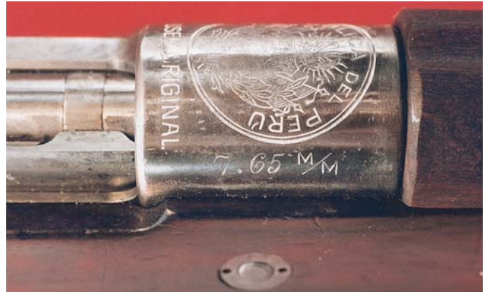
Caliber markings in electric pencil on the right side of the receiver ring of the above Peruvian Model 1909 Rifle.
