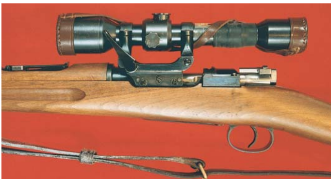
Close-up view of the left side of the Swedish Model 1896 Sniper Rifle fitted with the Model 41 AGA scope.
