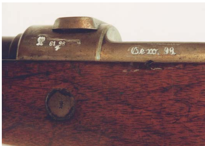
The left side of the German Model 98 Sniper Rifle, showing the model designation on the side rail, and the proof marks and serial number on the left of the receiver ring. (Springfield Armory Museum)
