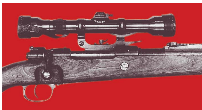
Right side view of a Kar 98k Carbine with a side rail mount with 4x scope. (Robert Jensen collection)
