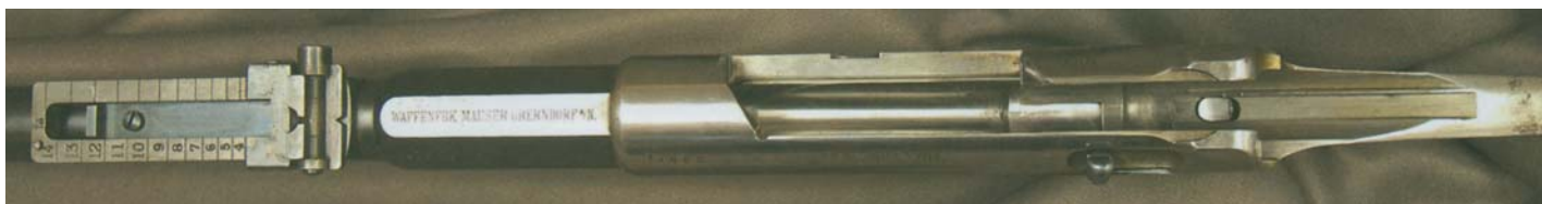
Close-up of top view of barreled action of Model 71/84 late production model 11mm, SN 17666, with second locking lug. (Private collection of Robert I. Landies)
