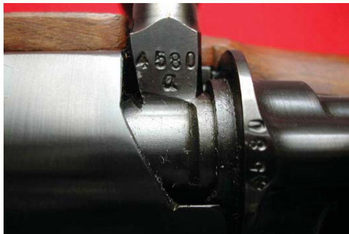
The Chinese contract Kar98 serial number 4580a. Notice that the numbering of all bolt parts is done in the front, format and location of comparable model rifles in German service. (John Wall collection)
